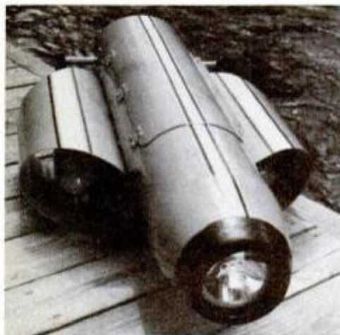
PM's electric diving scooter is easily guided through the water with bicycle-like hand grips. New features include headlight in nose (lower left) and instrument panel in stern (lower right). Hinged hatch cover opens for access to batteries and trim adjustments.
