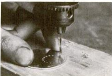
Center-punch lightly and bore holes through the soft metal. Clean off any burrs with sandpaper; solder to cylinder top.
