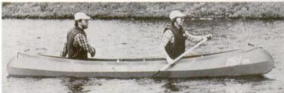
A canoe you can fold up into a 31-pound backpack unit, the Ally Collapsible from Vogue Industries, LaSalle, Que., uses aluminum ribs, PVC skin, assembles in 20 minutes.
