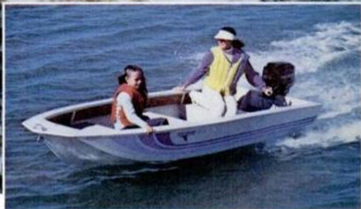
Lightweight hulls need less power, are easier to cartop and launch. Grumman's 12½-foot aluminum 3.8 weighs 170 pounds, can do 22 mph, is rated for 10-hp motors, like this Mercury 9.8.
