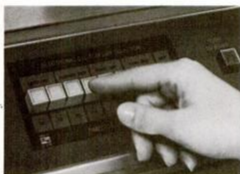
New microcomputerized clothes dryer doesn't have timer either. Buttons are pressed to select length of drying period and temperature and to start the unit.
