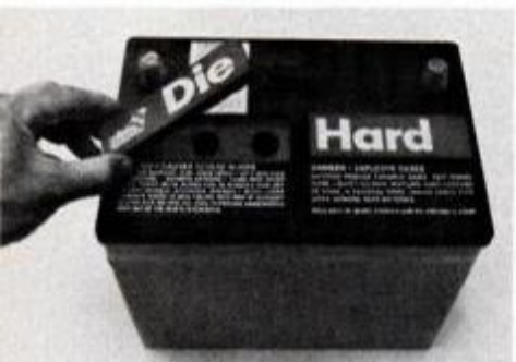
Replacement DieHard is maintenance-free, but caps come off for hydrometer checks.
