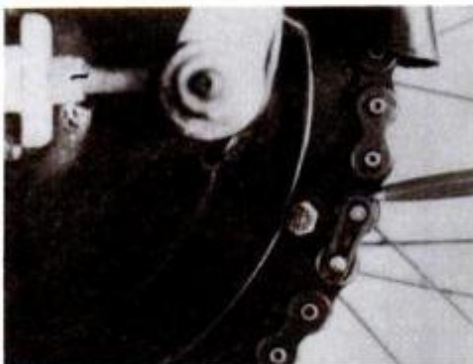
Closed end of spring clip on master link should lead in direction of travel chain, so it's less likely to be knocked off.
