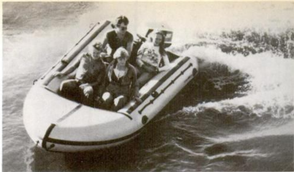
Bonair Boat's 16½-foot Brute 500 mounts up to 60 hp, has vee bottom for smoother ride, can even be ordered with a scuba diving window mounted in the boat's bottom.
