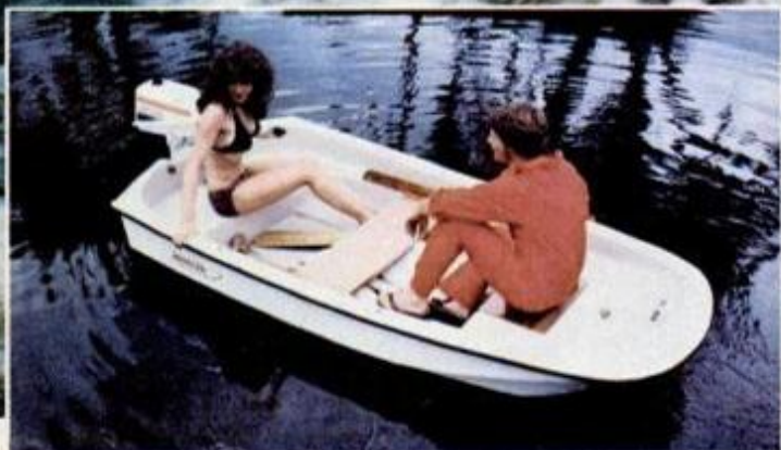
Broad beam and stable ride of wide multi-keel designs like the Boston Whaler make a good fishing boat or swimming raft. The 11½-foot hull, rated to 20 hp, easily handles Johnson 4.5.
