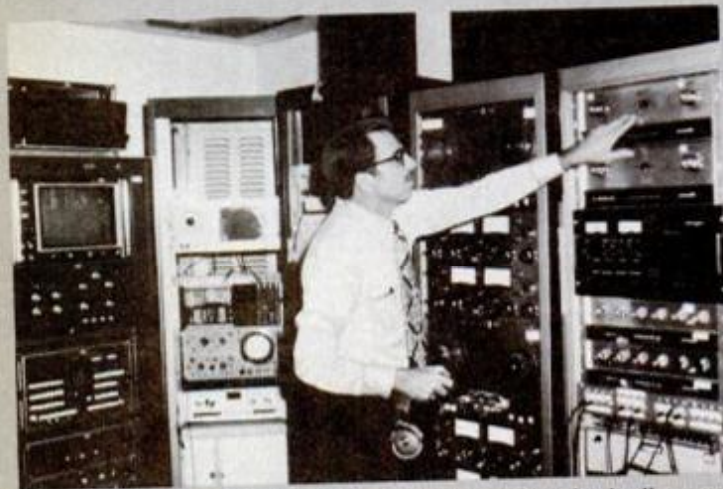
Cockpit voice recorder expert Paul Turner at work: Audio gear helps him dissect clicks, hums, rattles, engine roar for clues.
