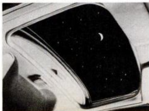
Sunshade (above) is operated manually. When it's pushed back, the power-operated moonroof (below) is exposed.
