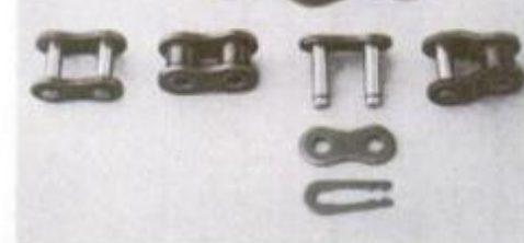
Roller chain links (from left): pin link, roller link, master link (pin link with removable linkplate and clip) and half link.
