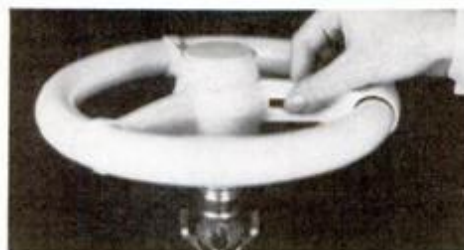
Light "wheel" fits over adapter. Plug-in spoke slides forward to engage adapter.
