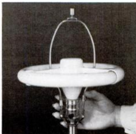
Harp is replaced to fit between spokes. Light may be rotated slightly to suit.
