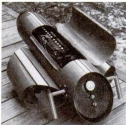
PM's electric diving scooter is easily guided through the water with bicycle-like hand grips. New features include headlight in nose (lower left) and instrument panel in stern (lower right). Hinged hatch cover opens for access to batteries and trim adjustments.
