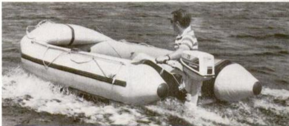
Low center of gravity for passengers and gear, plus independent flotation chambers in case of puncture, make quality inflatables like this, with Chrysler 7.5, extra safe.
