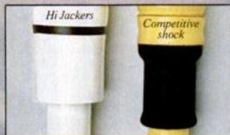
The rubber diaphragm on the shock at right can be damaged by road debris and gravel. The Hi Jackers' diaphragm is protected.
