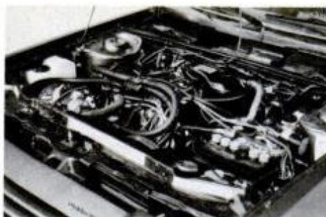
024 and TC3 use 70-hp, Volkswagen-based Four mounted transversely.
