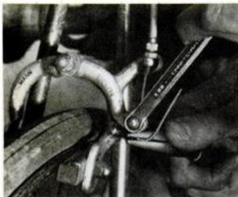
5 To tighten a brake cable, use needle-nose pliers to twist it. Tighten the cable anchor bolt with a wrench.
