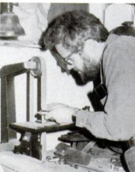
Use a belt sander-grinder to smooth rough castings more quickly than by hand.
