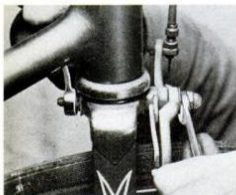
8 By turning the nuts at the front and rear of the brake in unison, you can easily center the brake over the wheel.
