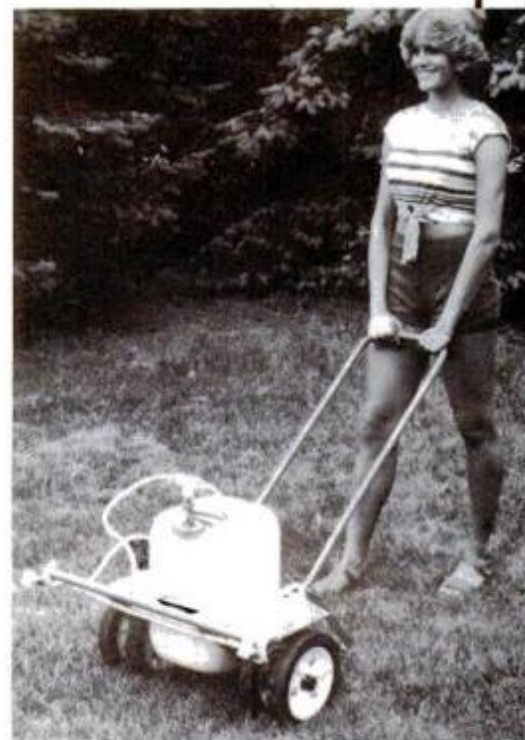
Broyhill's 2200-H holds 5 gal. of solution in a corrosion-resistant container, rolls easily on 10-in.-dia. wheels.
