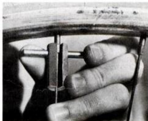
16 Inexpensive spoke wrench eases wheel truing. Tighten or loosen opposing spokes in half-turn increments.
