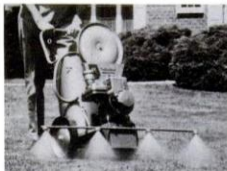
Hudson's 42025 sprayer, with 12½-gal. capacity, sprays a 5-ft.-wide swath per pass. It sells for about $415, and comes with electric power or as a towable unit.
