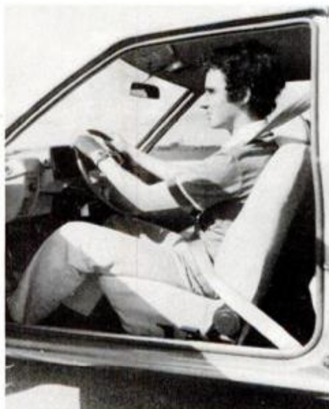
Front seating, legroom get good marks, but pedals are small for big-foot drivers.
