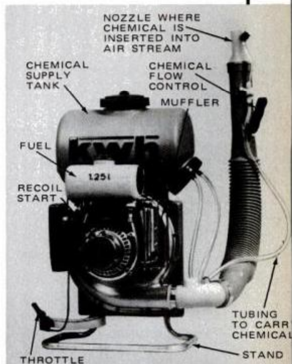
Compact mist blowers, such as Vandermol's KWH Model 44MP (about $400), feed chemical by gravity from top tank into blowpipe nozzle for best results.
