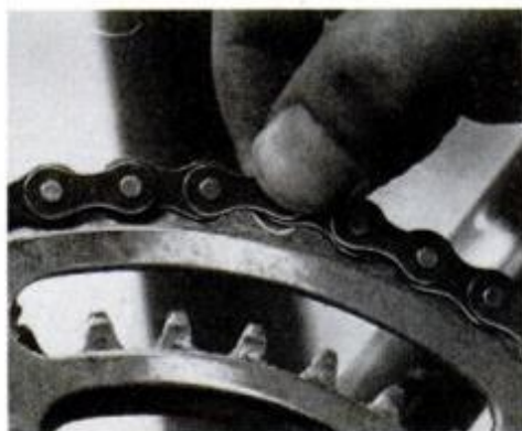
9 Chain should be cleaned and lubricated or replaced. If you can pick up a link this much, you should replace chain.
