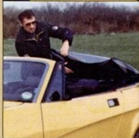
Two latches are undone and soft top is partially folded (top), final fold is made (above) and boot is attached to result in the TR-7's clean wedge shape (below).
