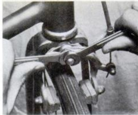
7 First step in centering a side-pull brake is to tighten the two nuts in front of the brake against one another.
