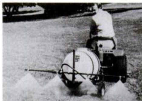
Larger units, like a Might Mac Model PS 350T, save time on large expanses of sod. It can treat a 10-ft.-wide area in one pass and sells for approximately $570.
