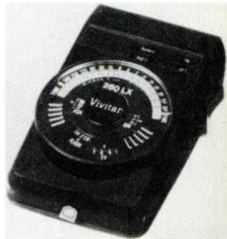
Servo-controlled dial on Vivitar 260LX hand-held meter omits moving needle.
