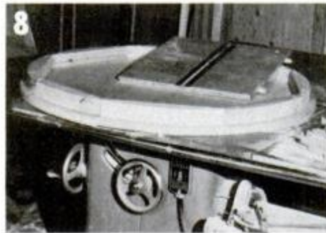
7. With apron assembly on sliding jig base, straight cuts form half circle. 8. Sliding jig base can cut many sizes.
