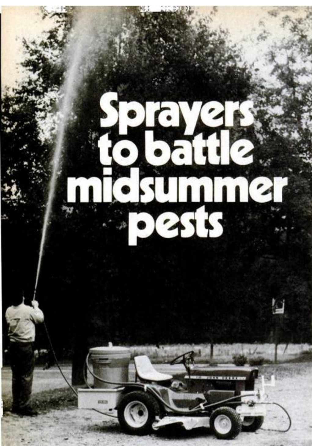
Get added use from a garden tractor with Marlen sprayer, Model 105, and a 30-gal. plastic garbage container. Combination lets you treat trees and turf. About $235.
