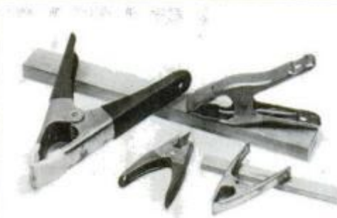
Spring clamps come in a variety of sizes and are perfect for light clamping tasks. You squeeze handles to open jaws.
