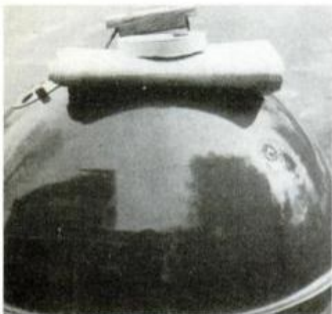
Chipped enamel surface of barbecue will accelerate spread of rust if untreated.
