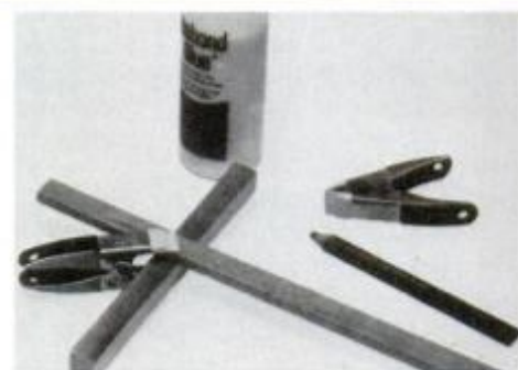
Spring-tensioned jaws are fine for holding small parts until glue dries. Pair here has plastic on jaws to prevent marring work.
