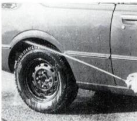
Wheel wells, car underparts should be washed frequently, especially where snow-melting chemicals are used on roads.
