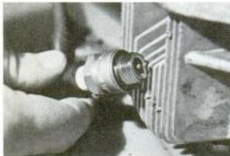
To check spark strength, grip plug rubber cap and hold plug in contact with engine while pulling on starter rope.
