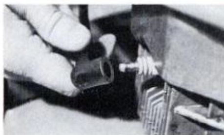
Before you begin any work on your mower, disconnect the sparkplug wire so the engine can't accidentally kick over.
