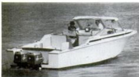
After cutting down transom to mount a pair of 200-hp outboards on a Bertram 28, Evinrude engineers found they added 14 mph, raised miles per gallon 83 percent.
