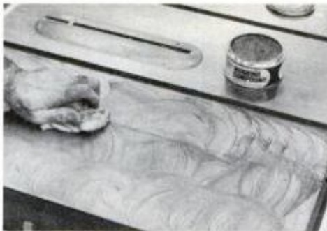
Use auto rubbing compound to remove rust, stains without marring saw table.
