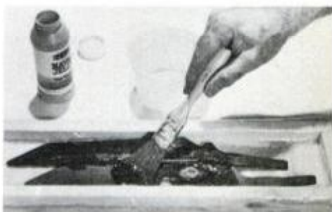
Brush was used to apply remover with disassembled tool held in plastic container.
