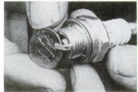
If the sparkplug is burned or otherwise damaged, it is best to gap and install a new plug at the season's start.
