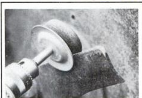
Sharpen the blade's cutting edge with a file or emery wheel. Inspect for signs of danger, such as cracks or severe bends.
