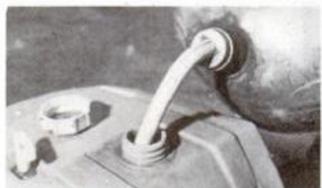
Fill the fuel tank with fresh gasoline or oil/gasoline mix, replace the sparkplug wire and test-pull the starter cord.
