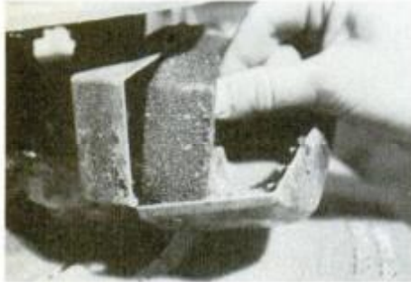
Lift out the air filter element and wash it in low-suds detergent or in kerosene. Squeeze it dry and re-oil it.
