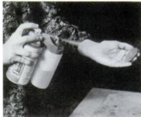
Spray gum binder on the metal to hold the enamel. To get a fine, even coat, hold the sprayer about a foot from the piece.
