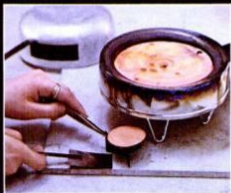
1 After sifting clear flux on face of a candle cube disc, put it on stilt; use spatula and tweezers to put in kiln.
