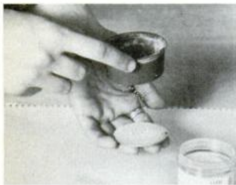
Sift a thin, even coat of any color enamel (it won't show) over the back of the metal. Make sure the metal is entirely covered.
