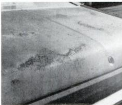
Surface condition shown can be a result of infrequent washings and waxing, particularly in seacoast or industrialized areas.
