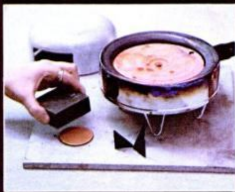
2 Each time you fire an enamel, cool 15 seconds on the stilt then flatten with a steel block or other weight for 10 seconds.
