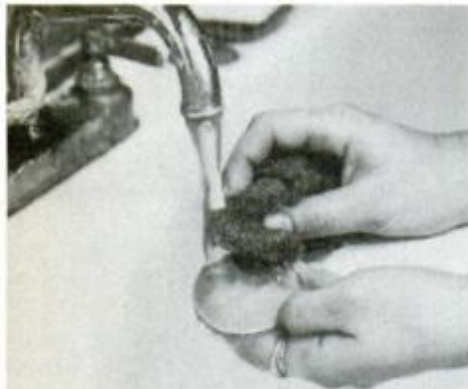
Clean the metal piece under running water using steel wool that doesn't contain soap. Grease may remain on the metal.
