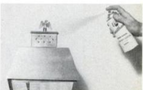
Protect brass or copper surfaces from corrosion with clear polyurethane finish. Apply it until the metal tone suits you.
