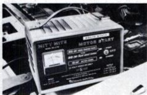
Special charger can put out 50 amps.
