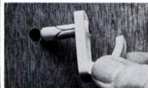
Plug is pushed firmly into 5/16-in. hole.
