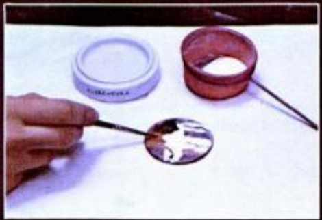
4 Dip brush in gum binder and remove enamel dust. Repeat step 3 with raspberry and white enamels, firing each one.
