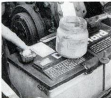
Heavy coat of grease or petroleum jelly on battery terminals resists corrosion.
