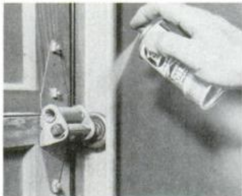
To apply protective coating in hard-to-reach places (such as obstructed side of garage-door roller), use oil in spray can.
