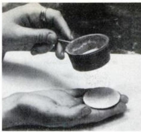
Sift bluebell over the fired white after spraying binder. In sgraffito it is very important to sift a thin, even layer.
