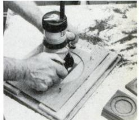
A jig holds the coaster blocks for routing. Each block gets a router pass using template X and a pass using template Y.
