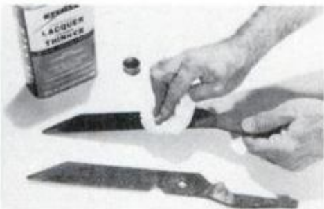
First, all grime and oily residue was removed using lacquer thinner and rags.
