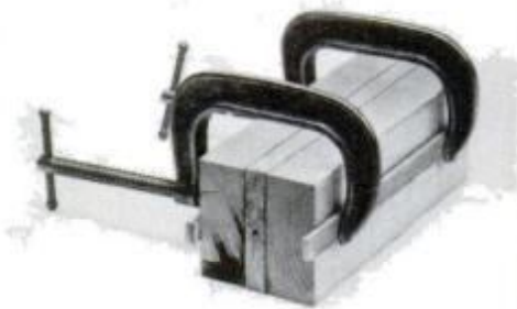
C-clamps are probably the most-used type in the home workshop. Here a pair holds glued-up stock for a lathe turning. Note protective wood strips under jaw pads.
