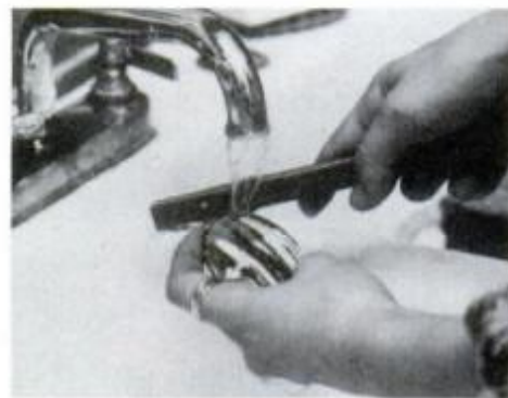
Hold the finished piece under running water and file firescale off the edges. Stroke file away from the top side of the piece.
