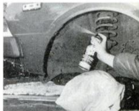
Small cracks, peeling in undercoating cause crevice corrosion. To remedy, first cover wheel with plastic. Then patch affected areas with a spray undercoat.
