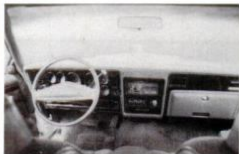
Instruments are hard to read because they're in recessed, poorly lit tunnels.
