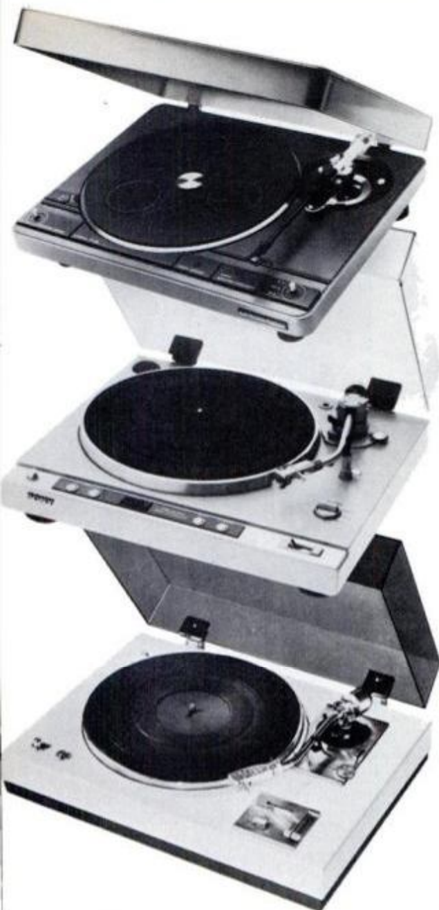
New ADC turntables have bases of two dissimilar substances; not only does this increase mass, it filters resonance. Sony's new cabinets use a nonresonant material and fluid-filled feet to dampen rumble. Kenwood uses a heavy base and highly damped rubber feet in its attempt to avoid turntable vibes.
