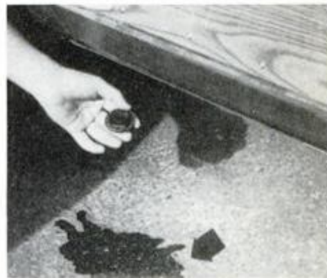
Water trapped in car doors (arrow) rots metal. Remove plug to speed drying, check doors often for clogged weep holes.
