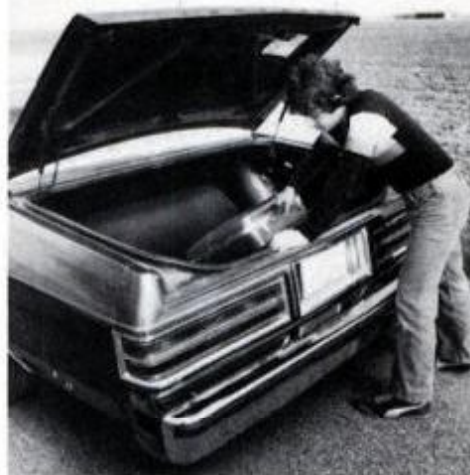
Gas cylinders prop up decklid, which lifts slowly. High loading sill is irksome.
