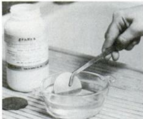
To remove grease, immerse the metal in a solution of Sparex and water. When grease is removed, water won't bead on the metal.
