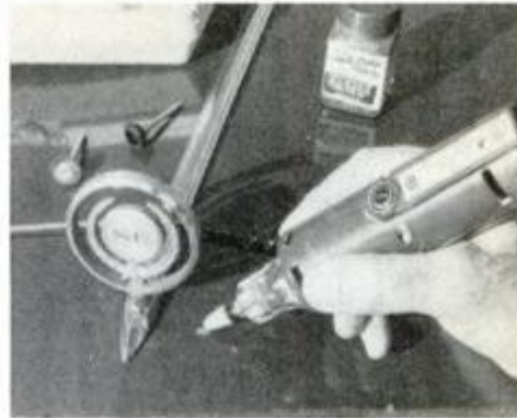
Small hand grinder with conical stone is perfect for removing rust from nicks and chips prior to touchup painting.
