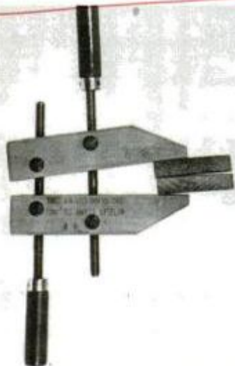
Wrong way to grip work with hand screws—nonparallel jaws mean work will dry as shown (in this exaggerated view).
