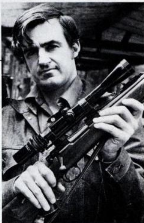
Leatherwood ART II (automatic ranging telescopic sight, above) is a sophisticated scope that figures range and bullet drop in one adjustment. Inventor James Leatherwood holds an early military model.
