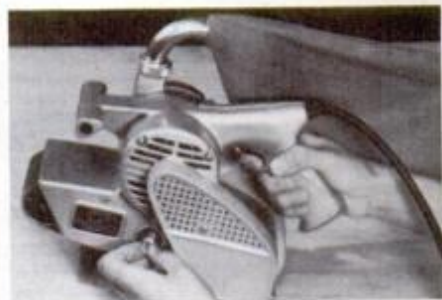
Belt-adjusting knob is used—with belt running—to get belt back on track.
