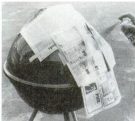
Use high-temperature-resistant enamel to touch up damaged spot. Mask surrounding surface with newspaper.
