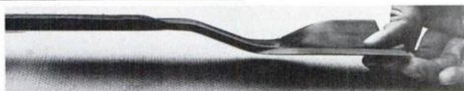
It's important to check the configuration of your mower blade. A good blade will have its outer tips at least 1/2 in. lower than the center mounting hole.
