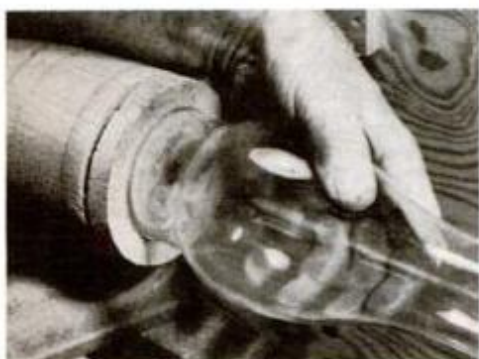
Periodically check globe in the groove. Stop lathe and back off tailstock to do it.
