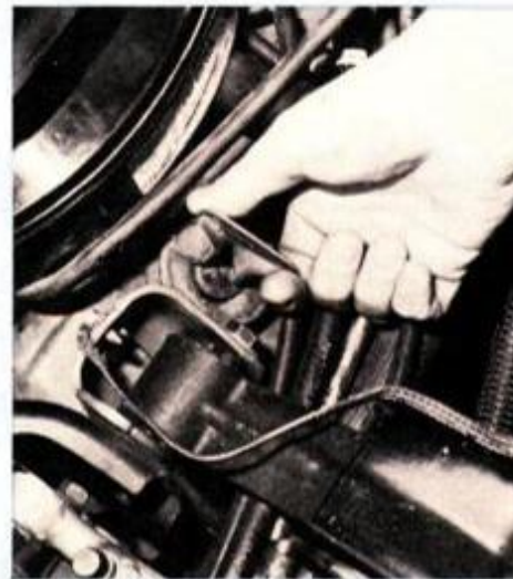
Dipstick for engine-oil level is right up front on V6 and has convenient handle.
