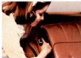
Push-Button Seat Conversion. Release the second seat with a touch of a button as you glide it down.
