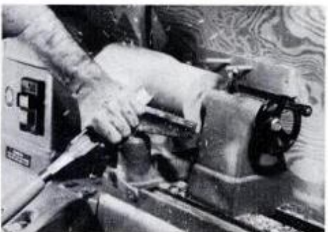
Start lathe and use gouge to make a series of 1 1/2 to 2-in.-long shearing cuts back to the right. Beginners should use light cuts and low speed to rough-round the stock.
