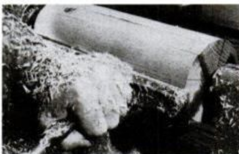
Or, make smoothing cut using skew in scraping position (better for beginners).
