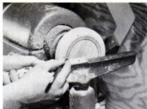
After smoothing face with square-nose chisel, use pencil to mark cuts on face.
