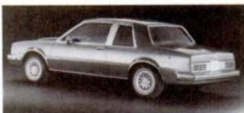
Pontiac Phoenix Coupe, like all the new GM compacts, is on a 104.9-in. wheelbase.
