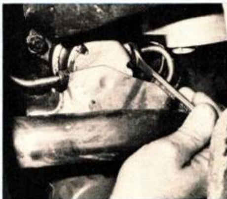
Fuel pump on V6 is next to oil filter; both are reached from front underside of car.
