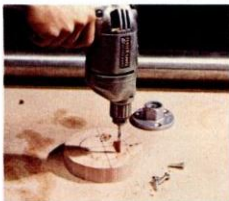
Bore pilot holes for faceplate screws; use tape stop on bit at desired depth.
