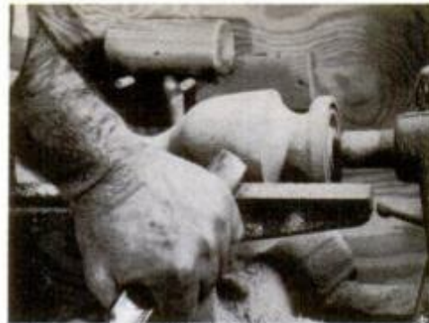
Sharp gouge with shearing cut produced desirable results on upper shoulder.
