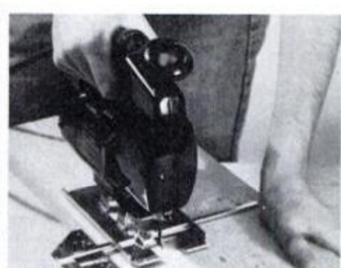
When accuracy is a must on a long rip, use the guide that comes with the kit. Make certain it is securely fixed to the shoe.
