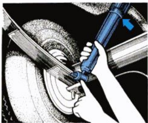
Damaged bottom and top bushings loosen shocks, causing loss of effective action.
