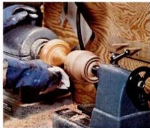
Apply by moving rag across work with lathe at slow speed. Replenish rag as needed.
