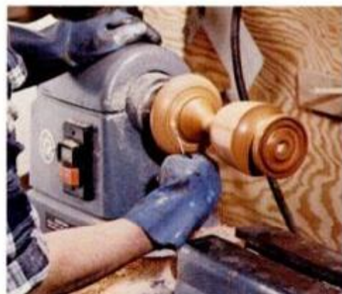
Repeat procedure on base; keep rag moving or you may create burn marks.
