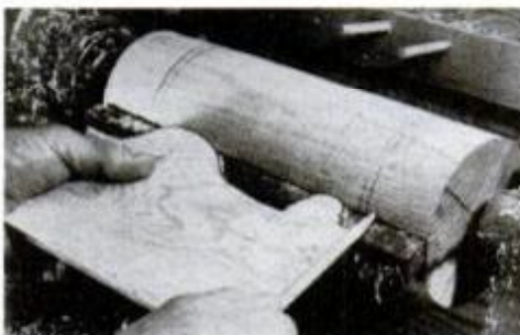
Cut a template and use it to lay out the basic shape on the smoothed cylinder.
