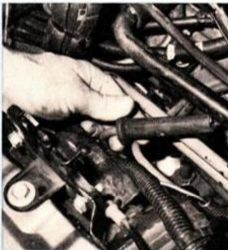
Sparkplug boots' built-in grips make it easy to remove ignition cables.
