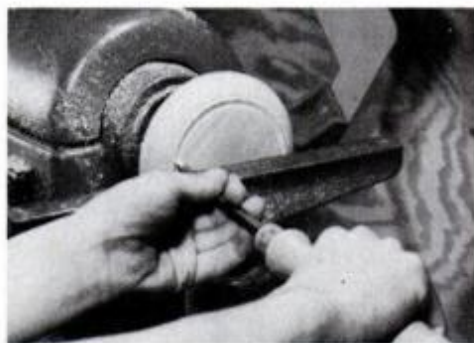
Small round-nose chisel is used to turn the decorative half-round groove.
