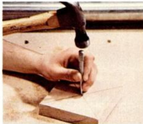
Make a permanent mark at the center by tapping a punch lightly with a hammer.
