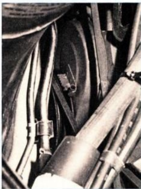
Timing marks on Four are easy to read; distributor-lock bolt is hard to reach.
