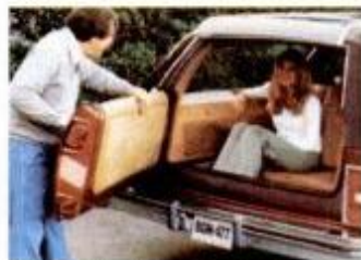
Three-Way Door-Gate. Opens like a door for people, like a gate for cargo.
