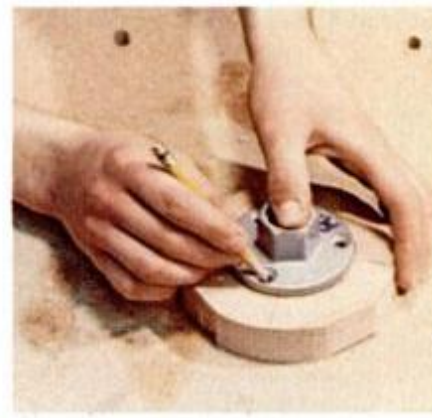
Center faceplate on stock, line up two screws with grain, mark for screwholes.
