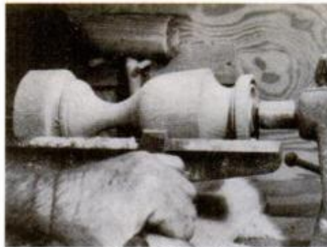
Skew in scraping attitude is an effective way to control shape on spinning work.
