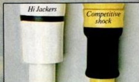
The rubber diaphragm on the shock at right can be damaged by road debris and gravel. The Hi Jackers' diaphragm is protected.
