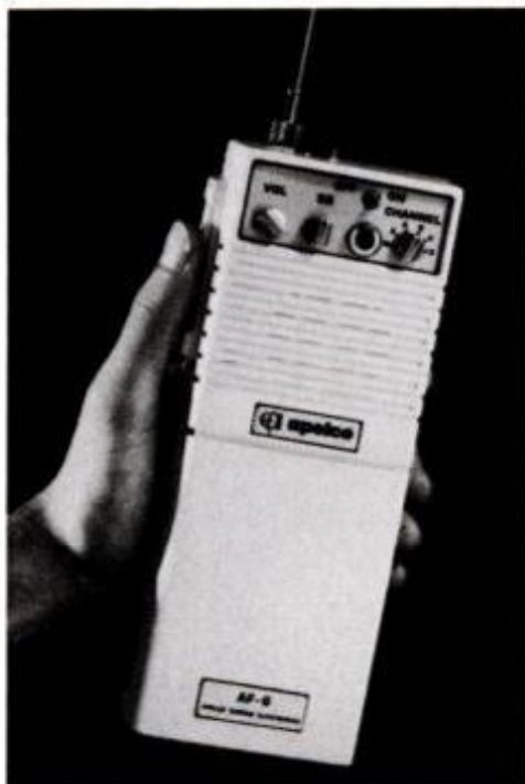
Useful hand-held VHF transceiver for boatmen is Apelco's $300 six-channel AF-6. Its five-mile range and two-pound weight makes it handy for small-craft harbor use.
