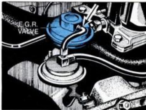
Disconnect the EGR hose at the near end (arrow) and plug hose to sustain vacuum.
