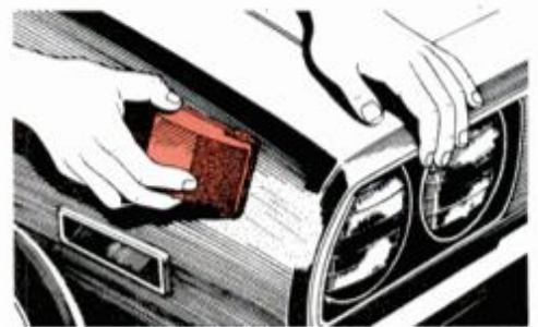
Meticulous sanding is critical and you should use a block to prevent raggedness.
