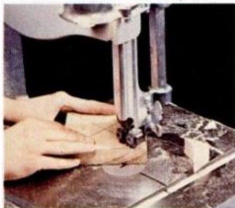
Use bandsaw to cut stock to rough dimension; cut on the waste side of line.
