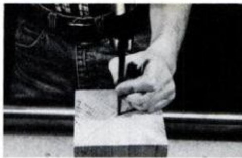
On both ends of the stock, center-punch holes at exact center (about 1/16 in. dia.) Use a wood mallet (right), which won't damage center, to drive the center into stock.
