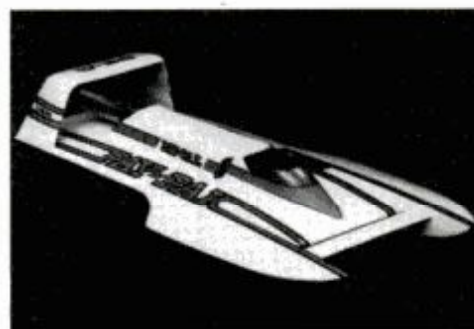
A first for unlimited competition, next year's Pay 'N Pak will have turbine power.
