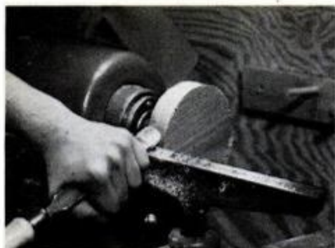
Set machine at low speed, and scrape across edge of stock with gouge or chisel.
