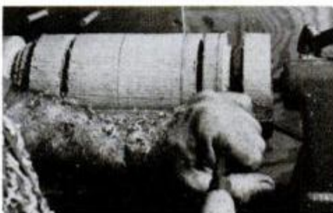
Cut various segments to correct diameter using the parting tool fed straight in.
