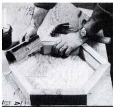
10 Fasten the stool edges together using glue and nails. Then repeat the procedure for the remaining five stools.
