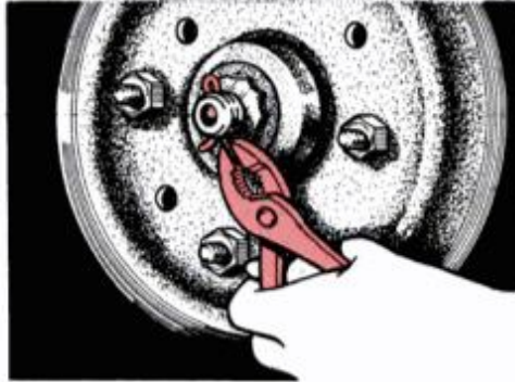
Align slots in the locknut with slots in the spindle and insert the cotter pin.
