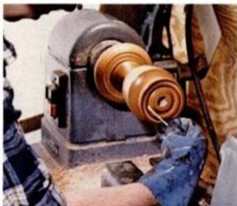
To work finish into valleys and crevices, wrap rag around small-diameter stick.
