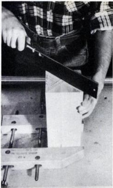
On spur center end of work, saw 1/8-in.-deep kerfs along both diagonal lines.
