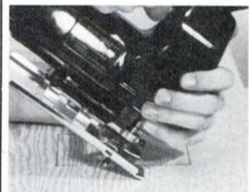
Slowly lower blade until shoe rests flat on work. If saw has variable speed, as here, use a slow blade speed, too.
