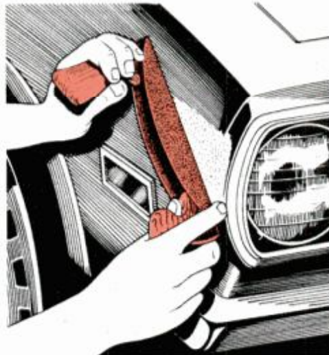
Apply plastic body filler and use a Surform to mold materials and remove excess.
