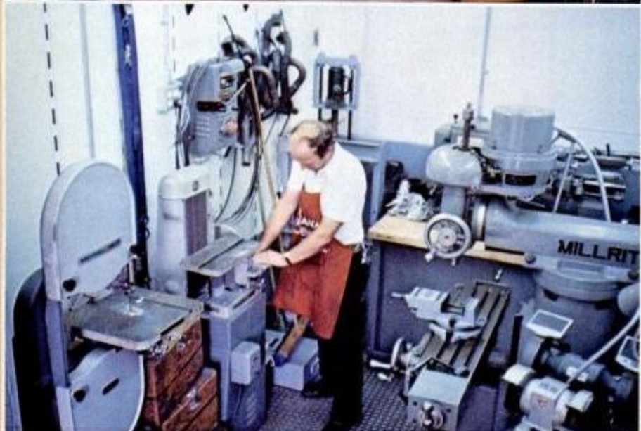
Colorful fleets of mobile machine shops pull into the infield during the mad month of May. The huge, 40-foot trailers are decked out with lathes, milling machines, drill presses, electric welding equipment and tons of tools. Dan Gurney's Eagles are borne to the Speedway in this big rig where his mechanics spend hundreds of hours in pursuit of the Indy 500 win. All photos are of Dan's rig except for the Parnelli Jones "pit wagon" (middle left) which has translucent roof for good light inside.
