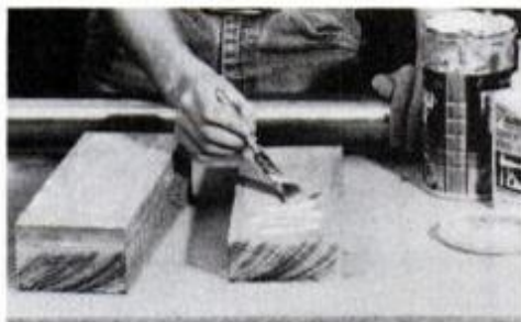
To glue up stock for a spindle turning, apply liberal amount of glue to mating surfaces (above). Use a number of clamps (right) to hold work until glue dries.
