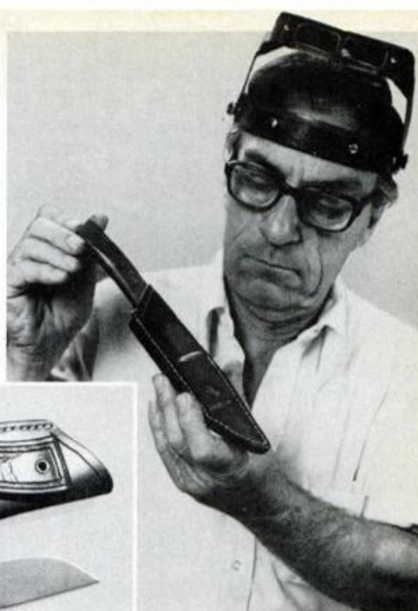
Art and craftsmanship combine in knives and sheaths made to order by Jack Barnett (above). Sheath (left) has hand-tooled decorations, molded front for snug fit for the knife, grommet at bottom of back for a rain drain and hole in belt loop for hanging it in display case.
