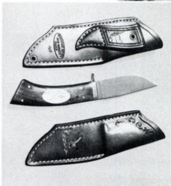
Art and craftsmanship combine in knives and sheaths made to order by Jack Barnett (above). Sheath (left) has hand-tooled decorations, molded front for snug fit for the knife, grommet at bottom of back for a rain drain and hole in belt loop for hanging it in display case.
