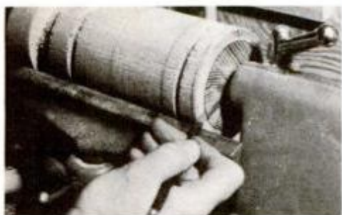
Lay out and cut groove for chimney using a small round-nose chisel with slow feed.
