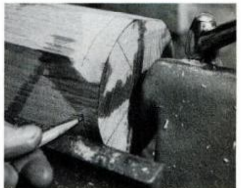
Using gouge, rough-round right end, mark with pencil to determine cylinder size.
