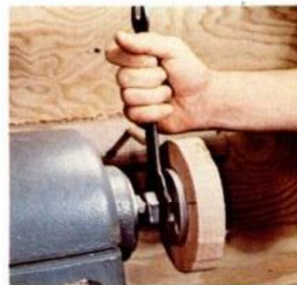
Holding lathe spindle rigid, mount the workpiece on lathe, tighten with a wrench.
