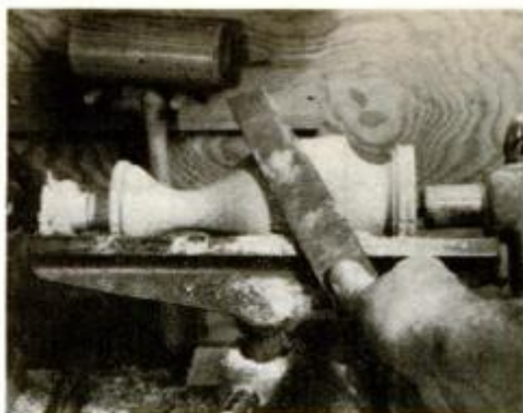
File, supported by toolrest, is an excellent way to start the smoothing step.
