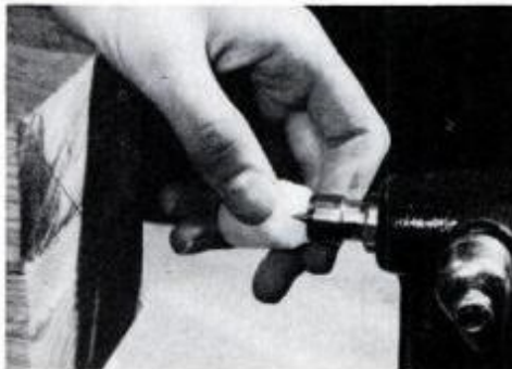
Mount work in lathe; before advancing cup center, apply lubricant to the cup center.
