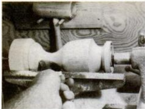
Shape cove portion by working from both shoulders down to the cove's center.
