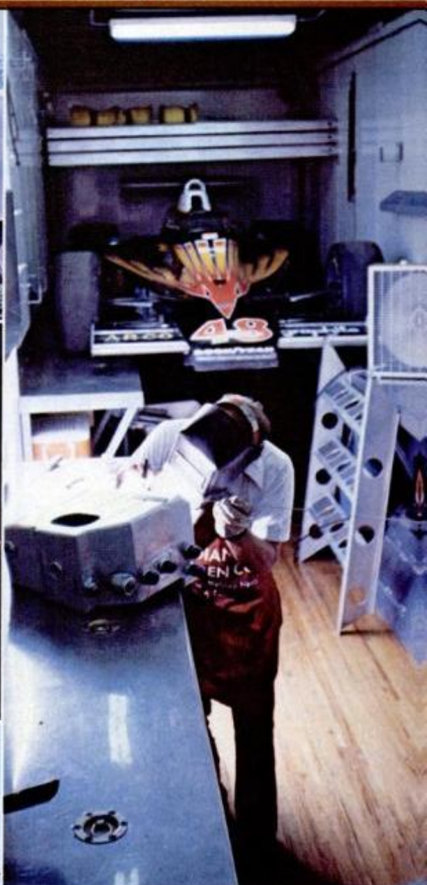
Colorful fleets of mobile machine shops pull into the infield during the mad month of May. The huge, 40-foot trailers are decked out with lathes, milling machines, drill presses, electric welding equipment and tons of tools. Dan Gurney's Eagles are borne to the Speedway in this big rig where his mechanics spend hundreds of hours in pursuit of the Indy 500 win. All photos are of Dan's rig except for the Parnelli Jones "pit wagon" (middle left) which has translucent roof for good light inside.
