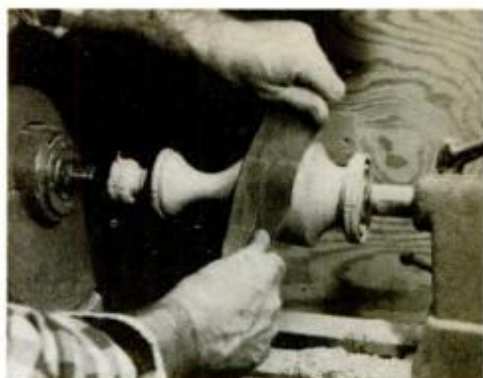
For final smoothing, use 220-grit paper (or fine emery cloth) shoeshine fashion.
