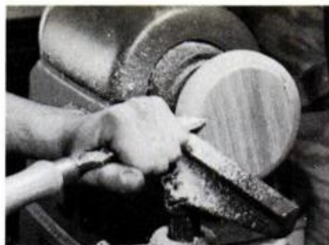
To shape the outside corner, a skew can be used in a scraping fashion.
