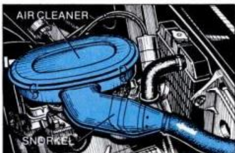
With this carb, tube can be disconnected at clamp (arrow) and snorkel is blocked.
