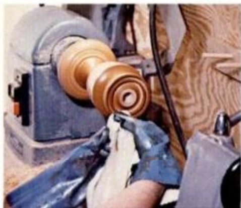
Apply rag to all wide, easy-to-get-at surfaces on the cylinder's top and base.
