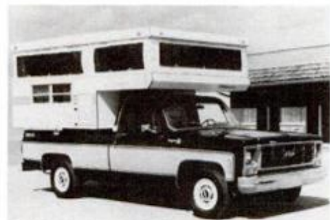
Bronco truck camper, at light 970 pounds, mounts on half-ton pickups and sleeps four with roof cranked up. It's new from Vanguard Industries, Colon, Mich.
