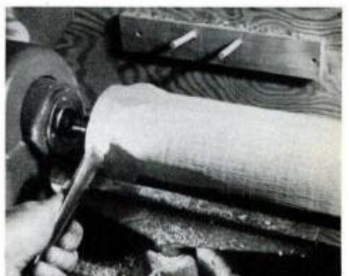
When you're about 2 in. from left end, roll gouge over and work toward the left end.
