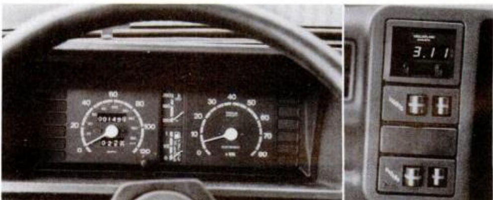
Dash layout includes temperature and fuel gauges set vertically between speedo and tach, both easy to read through wheel. Unique rocker switches for lights are under clock.
