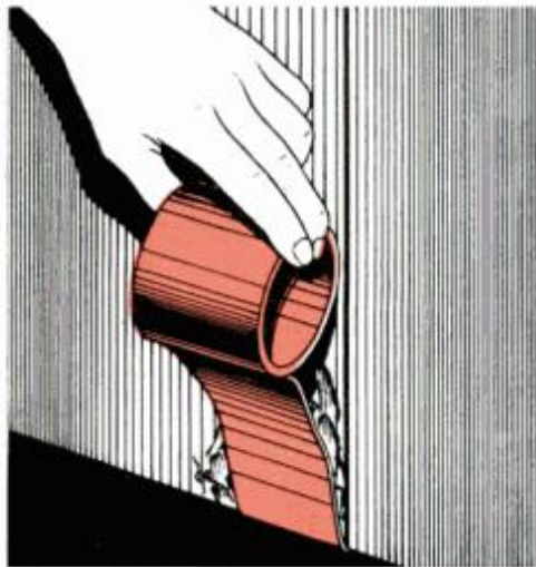
Aluminum tape and other material make possible body repair in the home garage.
