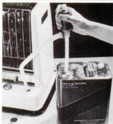
Siphon that comes with unit makes it a snap to refuel heater without spills.
