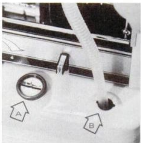
Gauge (A) gives tank reading. Filler tube is secured over clip in tank (B).
