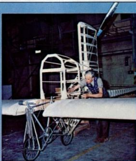
Britain's Newbury Manllier utilizes the power of two pilots pedaling in separate pods; while airframe-to-crew weight ratio is about the same as that for one-person Gossamer Albatross (below), a single, longer wing (138 feet) can be slightly more efficient.
