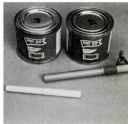
Four-inch plug, cut from solid white fiberglass blank, has been sanded; larger taper will be epoxied into hollow blank.
