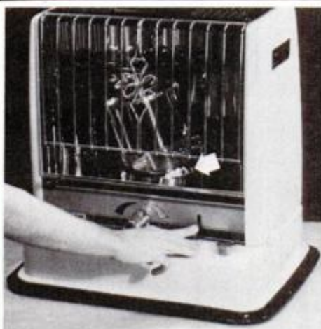
When lever is depressed, mantle tilts, battery-powered igniter lights wick.
