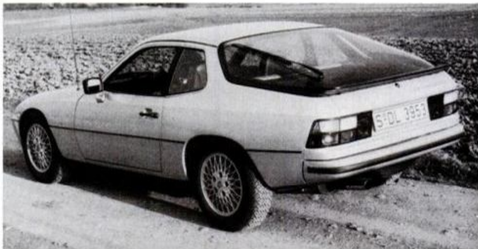
Rear spoiler aids aerodynamic flow over the turbo to reduce coefficient of drag. It's attached to the hatch lid and is soft rubber so it doesn't get nicked.
