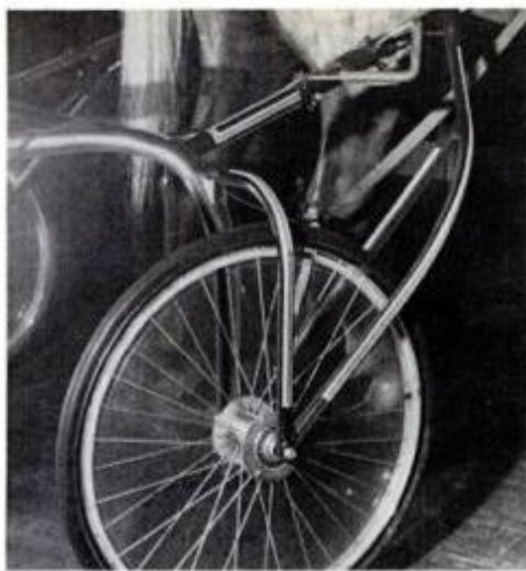
Conventional sulky (above) looks well put together, but modified makers claim added stiffness cuts down wheel "wandering."
