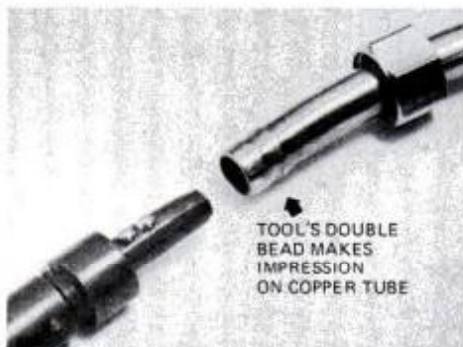
Bead mechanism on the tool forms a double bead on 3/8-in.-dia. copper tubing.
