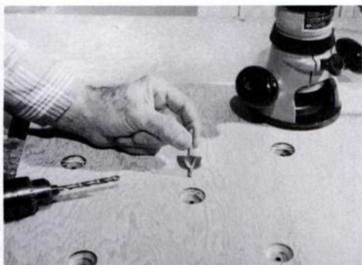
Cover router bit is used to make depressions in field. A clearance/guide hole for the bit's pilot end must be pre-drilled.
