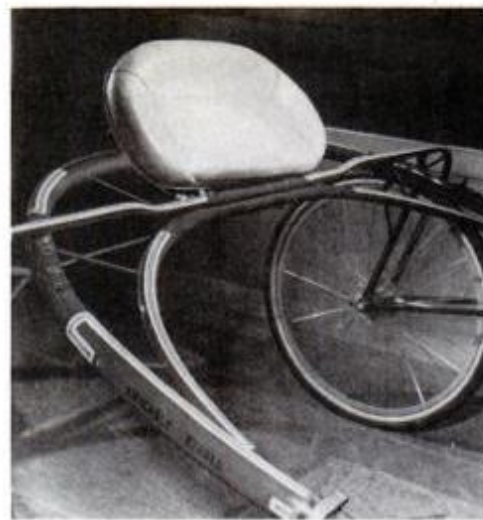
Lift from seat leverage in modified (below) is obvious. But many drivers discount the importance of the streamlined frame.
