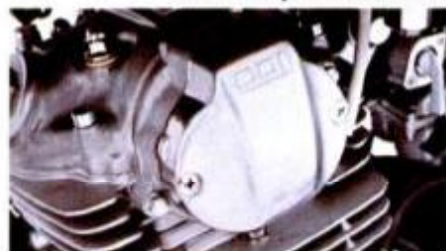
Hot-sparking Capacitor Discharge Ignitions fire the XLs (except XL75 and 100S).
