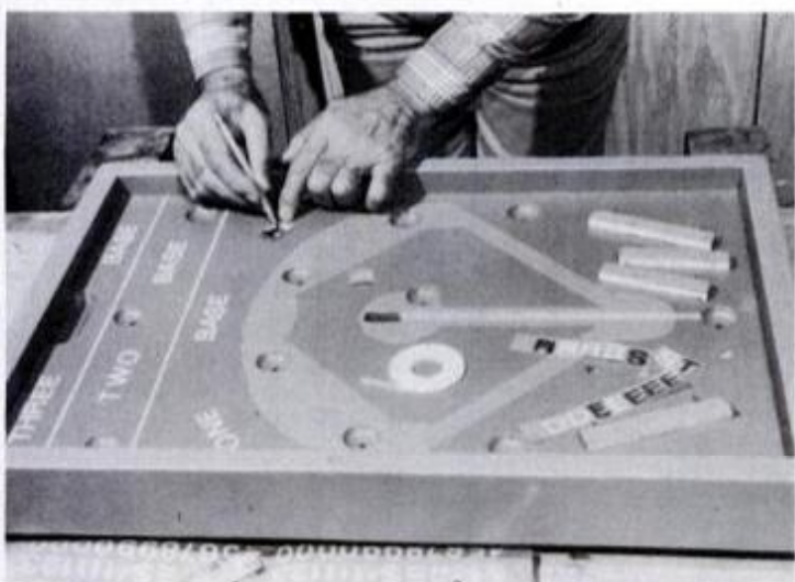
Press-on white letters, available in art supply stores, are applied by rubbing back of decal sheet with soft-lead pencil.
