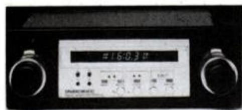
Electronic controls and digital readouts contribute to the new design "feel" of Sparkomatic's 22½-w.p.c. Model SR-3400.
