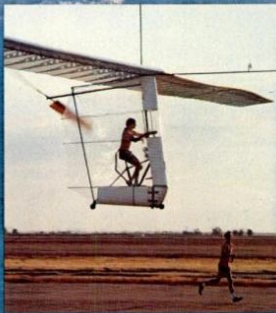
Paul MacReady's new Gossamer Albatross has pilot Bryan Allen sitting upright rather than semi-reclining as in the pioneering Gossamer Condor . Experience is the reason experts think MacReady will take the Channel prize, but logistics are tough.
