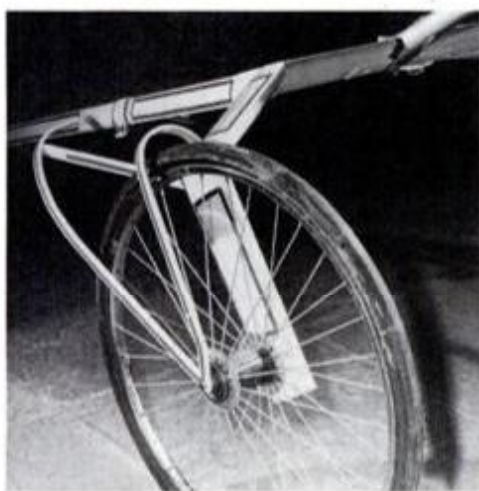
Conventional sulky (above) looks well put together, but modified makers claim added stiffness cuts down wheel "wandering."
