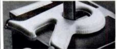
Idler wheel accessory aids grinding, finishing of areas like closed circles.
