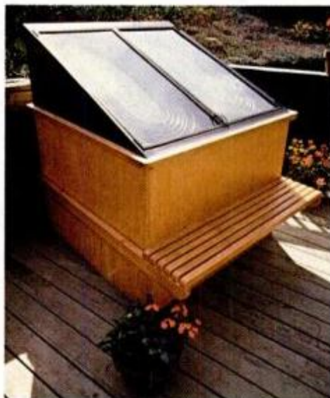
The top-cover doors (left) are framed fitted with clear acrylic and black polyethylene. Black plastic irrigation pipe (above) is sandwiched in between these layers.
