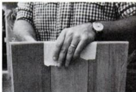
As each stave is placed, masking tape is used to hold a member temporarily.
