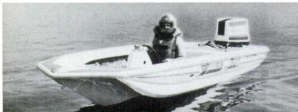
How fast will a bass boat go? This one, rigged for speed by Allison Craft, Louisville, Tenn., and with Benny Robertson driving, set a record of 107.4 mph, and then added another at 79 mph towing a water skier. Power was from the big 235-hp Johnson.
