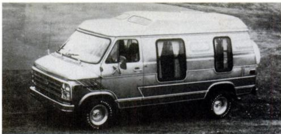
Raising the roof without shutting your rig out of the garage is possible with Viking's low-profile, add-on insulated fiberglass Sports Tops with roof racks for vans.
