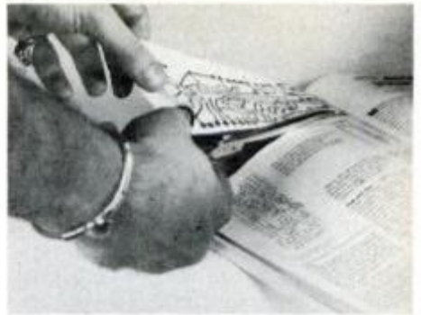
When you use a photographic-type PC-board kit, the first step is to cut out the PC template from page 18.
