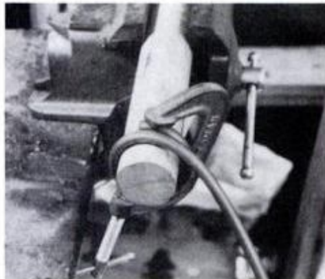
Tires are copper tubing shaped around a dowel. Shape seven tires, keeping them tight against each other; cut and solder.
