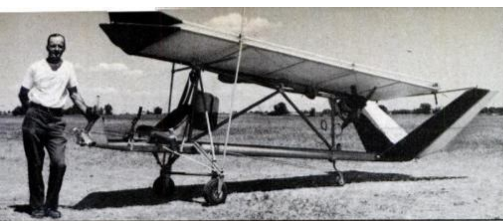
With wings removed and folded, Hummer (shown in flight on first page) is ready for trailering. At right is close-up of pilot seat, main wheels, foot pedals for ground steering.
