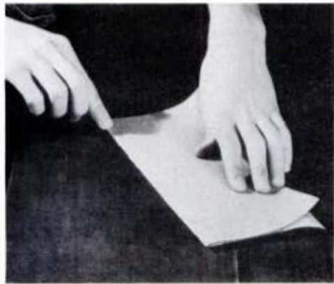
To tear sandpaper to size, fold neatly and press firmly along the line to be torn.
