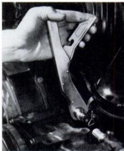
Lever can deliver torque of 450 in.-lbs.
