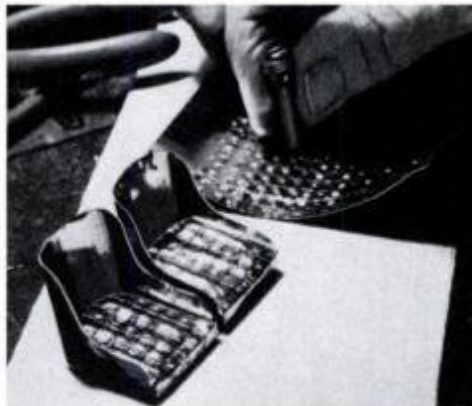
Seat bottoms and backs have textured upholstery made by scribing squares, then pressing with a punch or a stovebolt.
