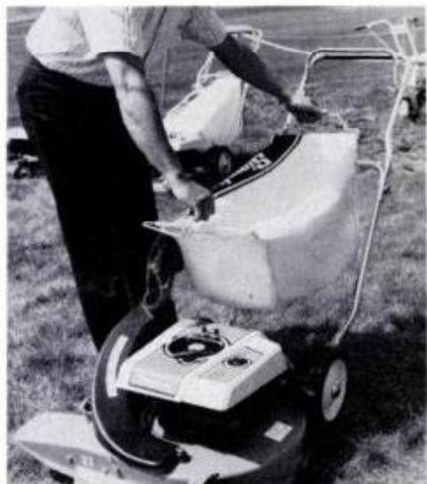
Turn this 21-in. Simplicity mower ($200) into a mulcher, side discharger, rear bagger or side bagging unit without tools.
