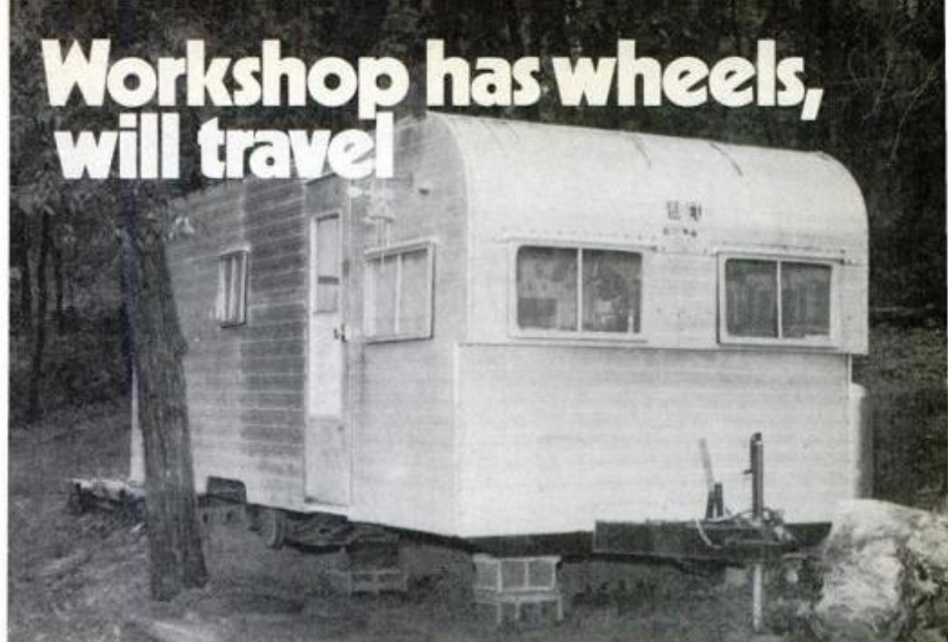
Exterior view shows trailer/shop with the wheels removed, positioned on cement blocks.
