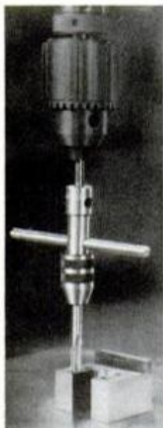
Lathe or drill-press chuck is used to guide, support and maintain alignment while tap is being turned by hand.
