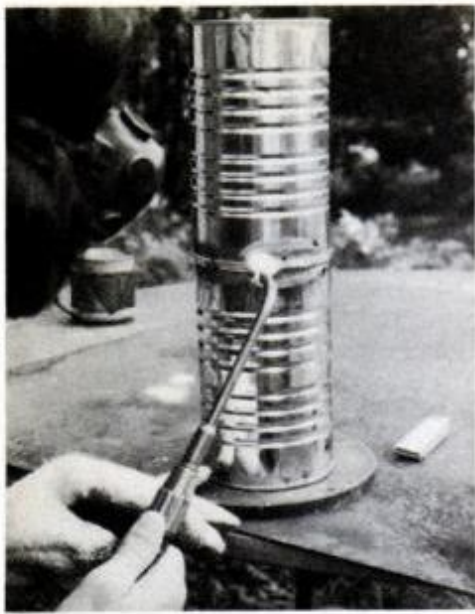
Cans are tack-welded in four spots to prevent warping, then seamed together by moving torch in small circles (see text).
