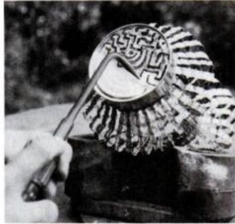
Top decorative design is cut. A lighted candle under it will cast this pattern on ceiling. Side bands, angles are final cuts.
