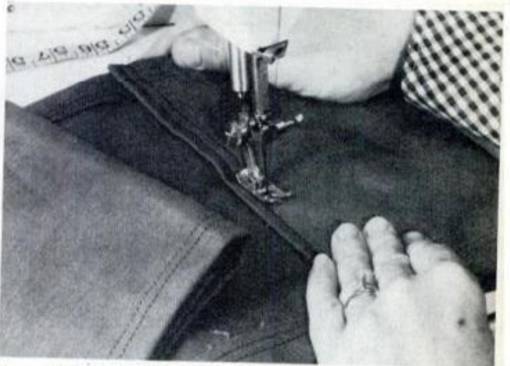
Sew a \frac{1}{2} -in.-wide hem with a double row of stitching on both edges of canvas parts. We used a No. 18 needle for this work.
