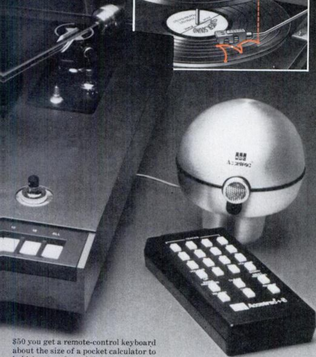
The Accutrac's tone arm uses laser technology to sense when it reaches the end of a selection. Grooves on the record disperse the beam but the blank areas between the songs will reflect it back like a mirror.
