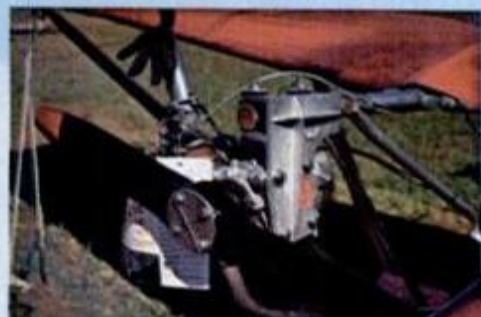
Weedhopper is patterned after traditional aircraft design with nose-mounted prop, tricycle gear and airplane-type tail. Engine (left) is 22-horse Yamaha snowmobile mill.
