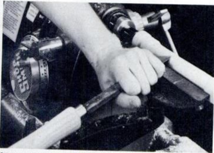
Several pieces require simple turning on lathe. Make the rough cuts with gouge, cut and trim shoulders with skew.
