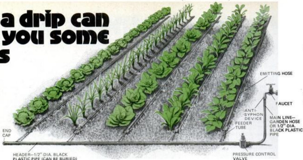
This diagram shows a basic trickle irrigation system. Antisiphon device prevents back flow.
