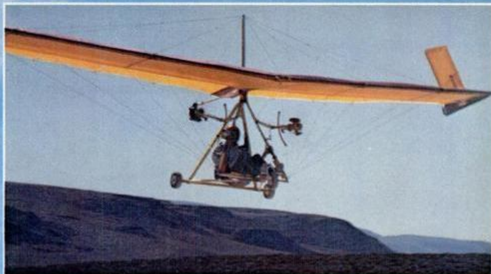
A twin-engine hang glider? Yep—it had to come! This Manta sports pair of 5½-hp chain-saw engines said to give 51-pound thrust. Dual system holds 40 minutes' fuel, weighs 26 pounds, will be sold under Gemini name as add-on power pack to fit most hang gliders.
