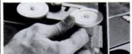
Flat or convex metal platens support grinding of curves, intricate shapes.
