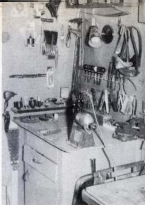
Tools hang on perforated hardboard in easy reach. "Bench" is a kitchen cabinet.
