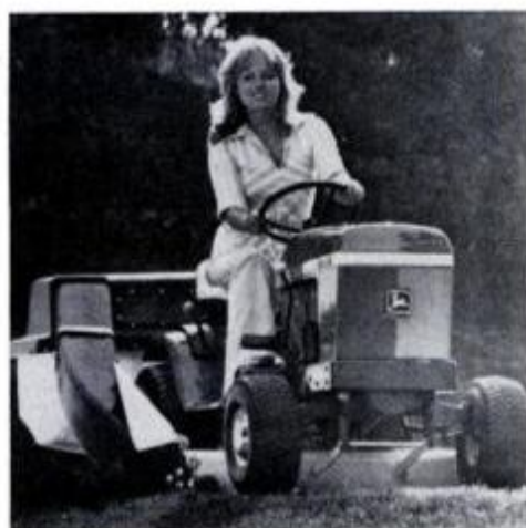
John Deere 108 ($1350) has an 8-hp engine, 5-speed transmission, 30-in. mower.
