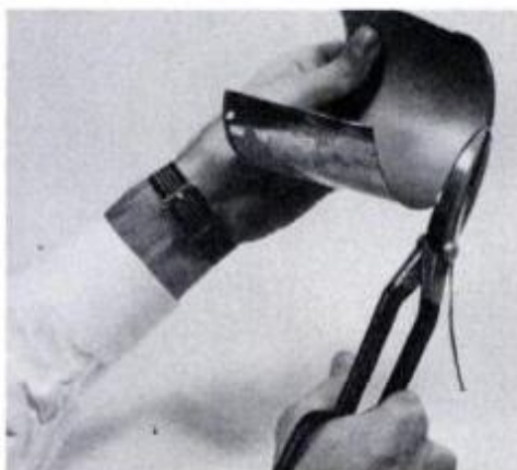
Cut rims from a can after slitting it at the seam. Next, tack the can to plywood with the inside surface facing outward.
