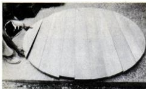
Factory-numbered boards prevent chance of assembling the tub bottom improperly.
