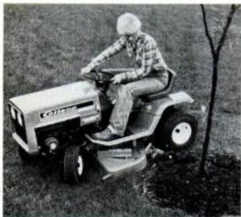
Gilson's 11-hp lawn tractor ($1280) has tight turning radius needed on home units.
