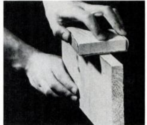
Use a backup block when sanding narrow edges to avoid rounding the corners.
