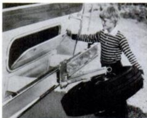
Blocked by a spare tire, a motor home's rear storage compartment is useless unless a hinged, spring-loaded tire carrier like Kenco Engineering's is bumper-mounted.
