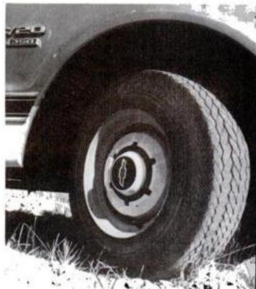
Conventional heavy-duty truck tire is a good on and off-road compromise.
