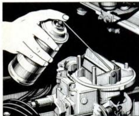
Keeping the choke valve clean and working freely is basic preventive maintenance.
