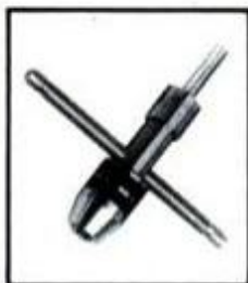
Lathe or drill-press chuck is used to guide, support and maintain alignment while tap is being turned by hand.
