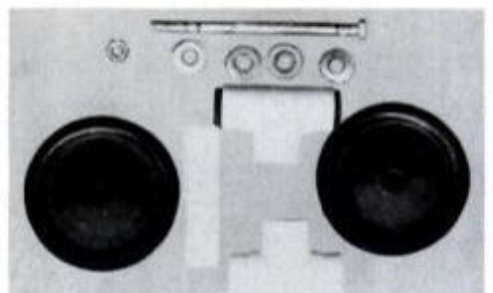
Wheel assembly includes tees, 3-in.-long PVC, 7/16-in. axle/bolt, washers, nut and 1 1/4-in. wood plugs cut with hole saw.
