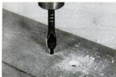
Bit shown in drill bores pilot and shank holes and countersink in one operation.
