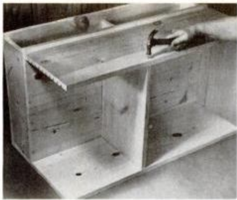
Divider (H) is butt-joined to front and back of chest, held with nails and glue.
