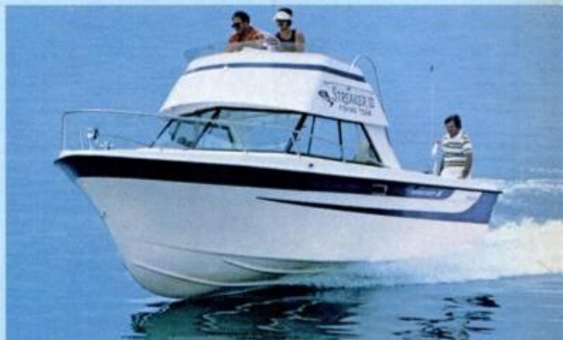
First Starcraft with extra-wide 9¼-foot beam, the 25-foot Star-Cruiser Flybridge has cabin, flying-bridge steering.
