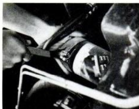
Wrench removes stuck-on oil filters.
