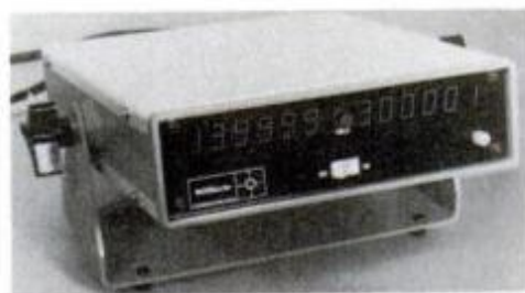
Teledyne's Loran C receiver can automatically track and display two signals.
