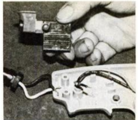
Note wiring pattern before removing faulty switch. Rewire replacement accordingly.
