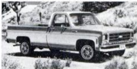
Chevrolet's 1979 light-duty pickups have revised grille, radial tires as standard equipment and 250 Six as the base engine.
