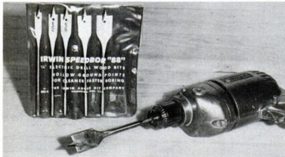
Handy set of spade bits in a pouch lets you bore \frac{1}{4} , \frac{1}{2} , \frac{3}{8} , \frac{1}{2} , \frac{3}{4} and 1-in. holes.
