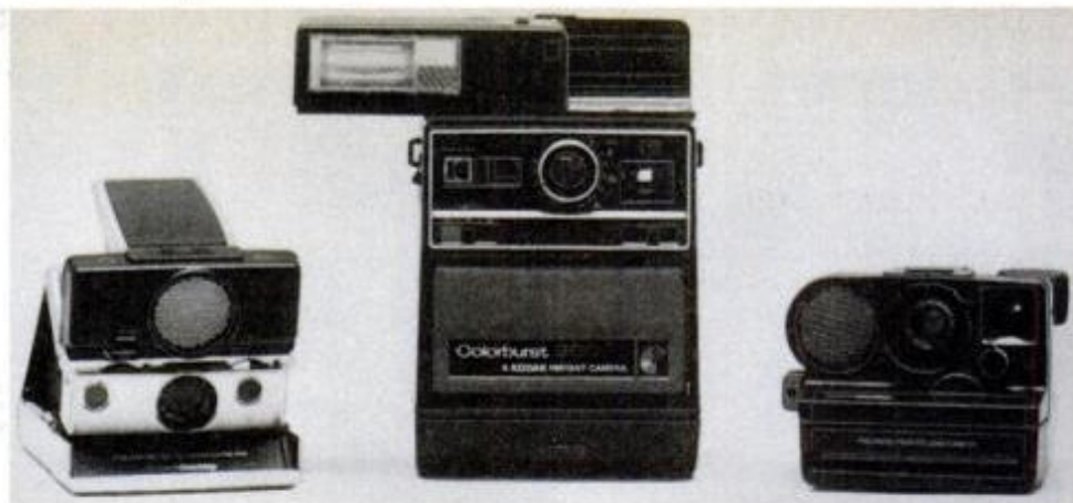
A trio of instant cameras: The Kodak Colorburst 300 is flanked by two Polaroids. Motorized Colorburst features built-in flash. SX-70 Sonar One Step (left) and Pronto Sonar One Step have automatic focusing. SX-70 also has a focusing preview.
