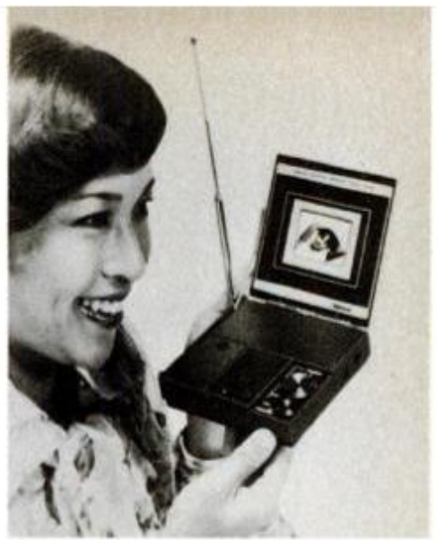
Matsushita of Japan recently showed this new, flat-screen TV. The picture is formed by an array of liquid crystal black and white "dots," much as photos in a magazine are produced by dots of black and white.
