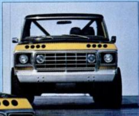
Don Kuster's 100-mph Ford F350 Camper pickup sports Cat diesel turbobed to 325 hp, four-speed Allison AT540 auto trans and 3.73 rear with Detroit Locker differential gears out back.
