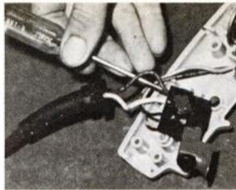
Switches with spring-connected wires are disconnected with thin-pointed tool. Wires may be attached to some switches with screws; loosen the screws to disconnect.
