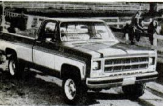
GMC half-tonners for '79 continue the diesel engine option, get more corrosion-resistant steel in doors, hood, fenders.
