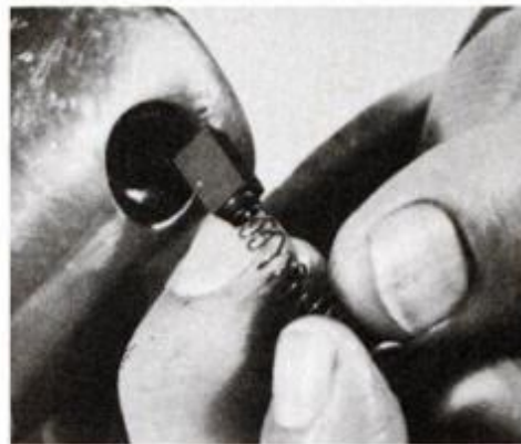
To remove a brush from metal-case drill, unscrew slotted retainer on housing. Release it slowly to avoid losing the spring.
