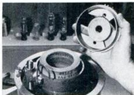
Center guide ring prevents centrifugal force from spraying water. Ring height adjusts so the stone can be used until it wears down to the last 1/16 in.
