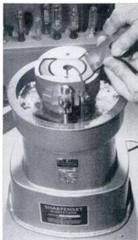
The grindstone is water-cooled, making this English unit a joy to use. Switch (above) sets direction of wheel's spin.
