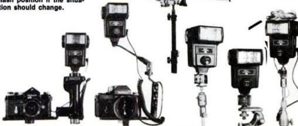
Three flashes set up for slave operation: Rollei/Honeywell Fotoeye II (left), a Vivitar slave (center) and the ingenious Leki Slave Trigger (right) made with a long cable to allow positioning of the slave away from the flash unit.
