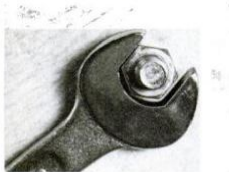
Wrong. Oversized open-end wrench will slip off, cause severe knuckle damage.
