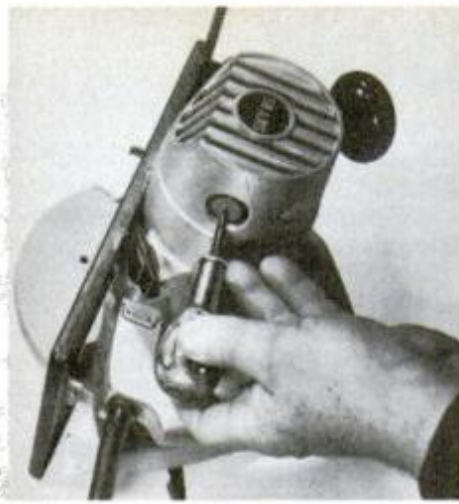
Brushes can be checked and changed in some tools like this Sears circular saw without opening the motor housing. Caps unscrew to allow brush removal.
