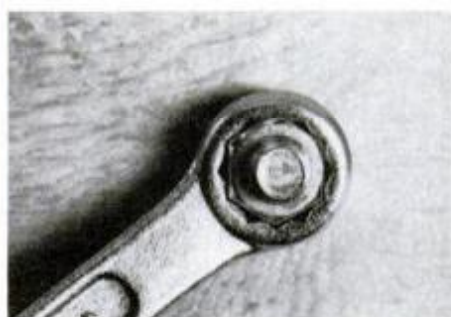
Right. Correct size fully engages nut and will not slip off under pressure.
