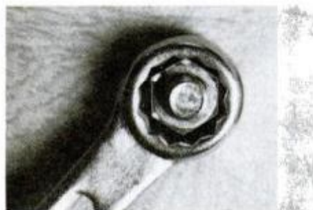
Wrong. Oversize box wrench will round nut corners and make it nonremovable.
