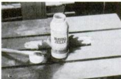
Clean rust from tool tables and lathe ways with rust remover. The right side of this saw table has been restored.
