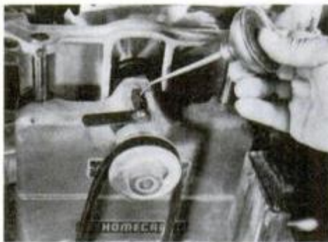
Clean sawdust from table saw with vacuum. Dirt can pack against stops and affect depth of cut and angle-cutting accuracy.
