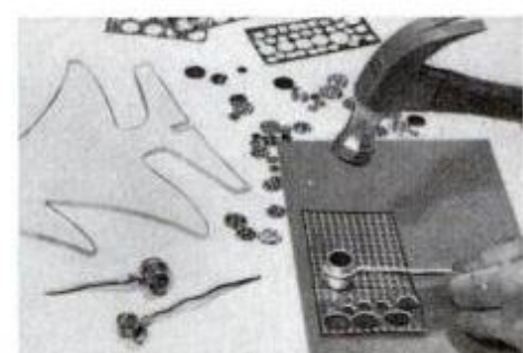
Add wire handles to clicker punches and cut film discs. Work on hardboard to get clean cuts.
