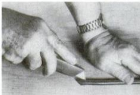
2 Make a slit in new cord's cover and bare enough wire to make connection. Trim off excess cover with scissors.
