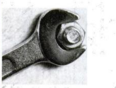
Right. Nut is fully seated in wrench; both wrench and nut will be spared damage.
