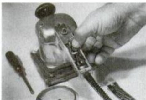
4 Use screw-on connectors or pigtails and tape insulation when rewiring. Fold wires into handle to avoid pinching.
