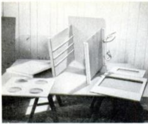
Main stove parts during assembly. Cleats permit using 1/4-in. plywood members.
