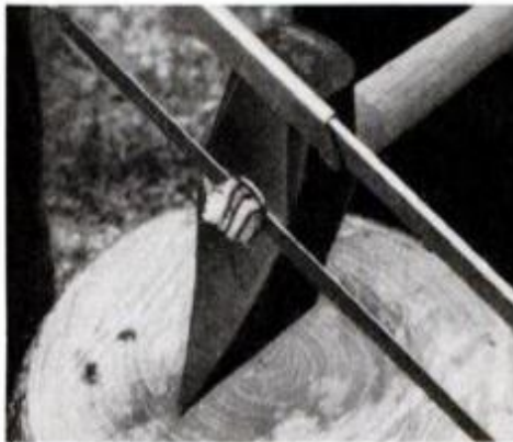
7 When tight, use the hacksaw to trim the new handle and wood wedges flush with the top of the tool eye.
