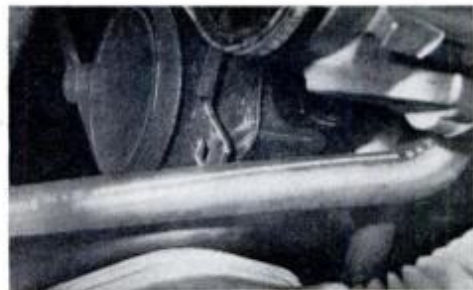
Power-steering drive belt is adjusted with breaker bar in square hole on bracket.
