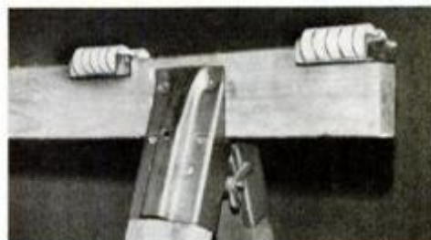
Appliance rollers are installed as shown on sawhorse that serves for rip support.
