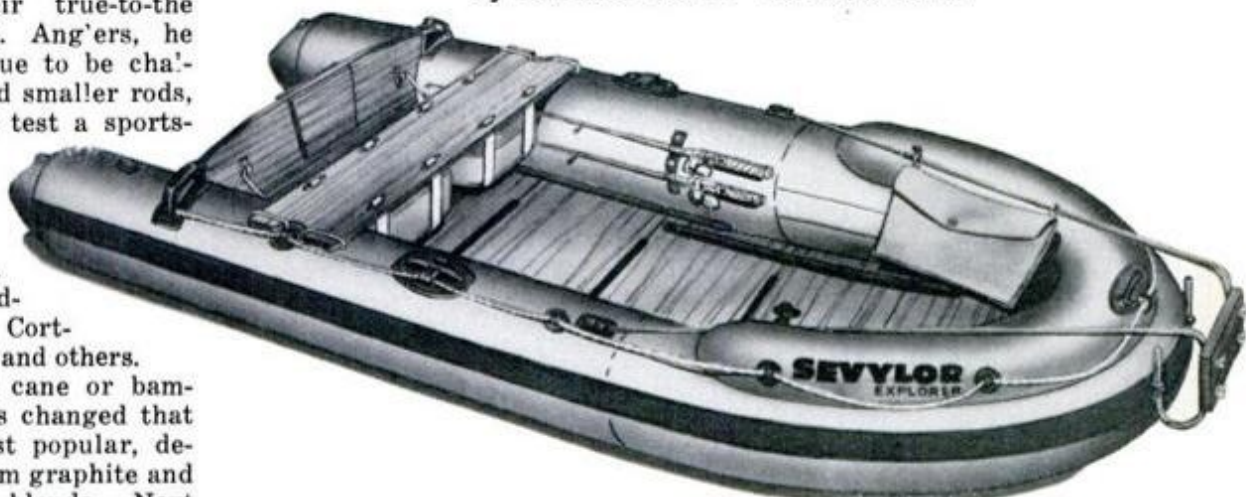
Is it the first inflatable bass boat? The 11-foot, 110-pound Sevylor Explorer has an electric trolling motor in front, up to 7½-hp aft, and can carry 650 pounds.
