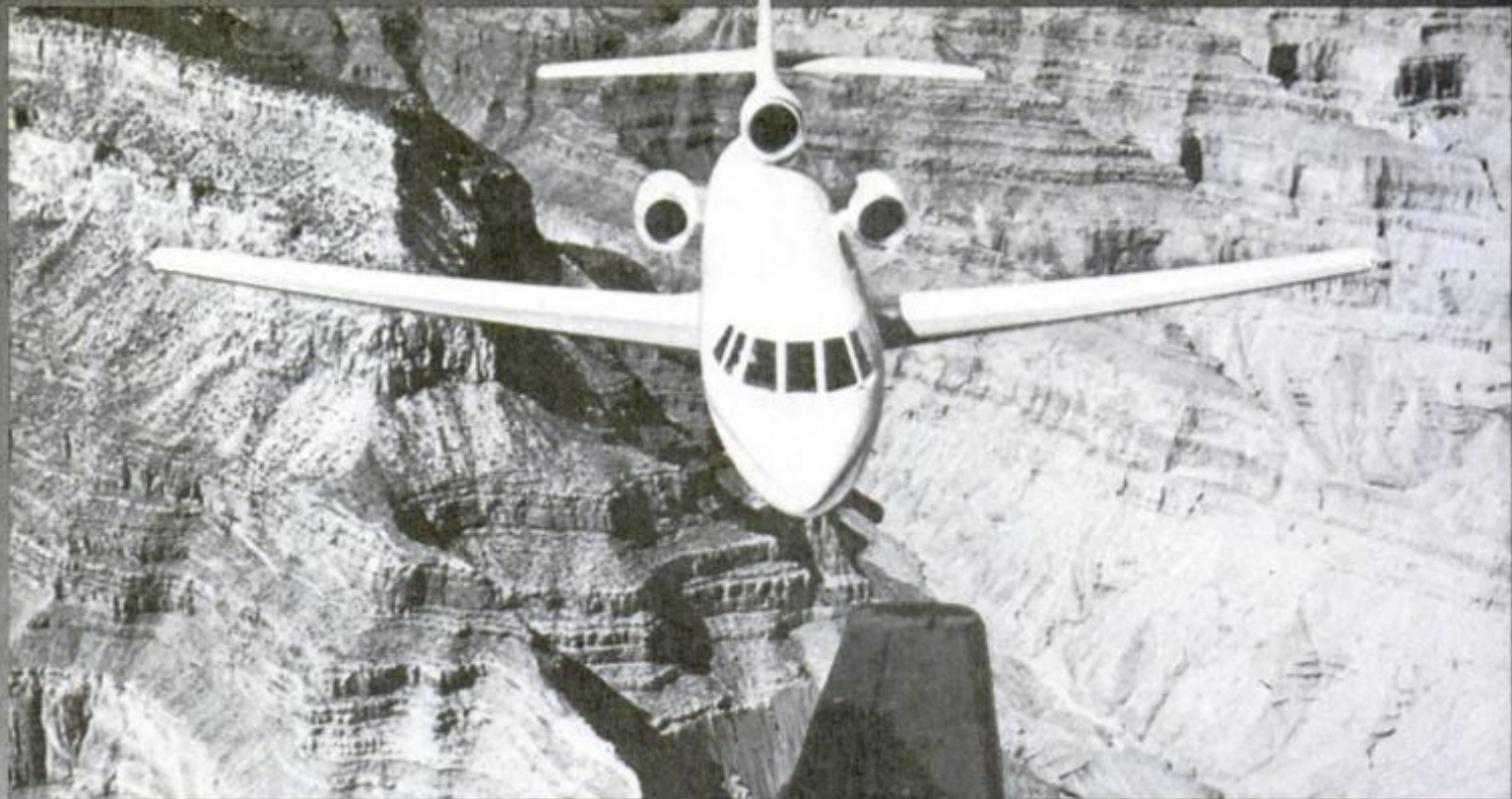
Dassault's Falcon 50 (above) is unique trijet design among the new-generation business aircraft. Grumman's Gulfstream III (right) employs nearly vertical "winglets" to help convert drag from tip vortex formation into useful lift.
