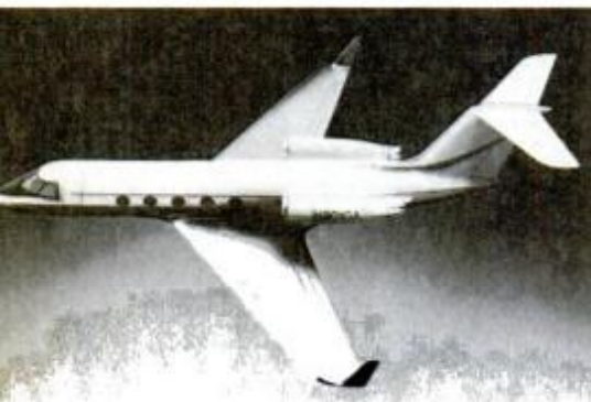
Now being built in prototype, Gates Learjet's new Longhorn model uses winglets similar to those of Gulfstream III.
