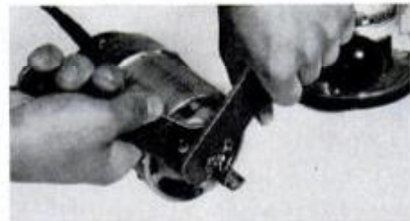
Most routers require the use of two wrenches to tighten collet, as here. Some makers offer models with built-in shaft-holding devices that permit changing cutters with only one wrench.
