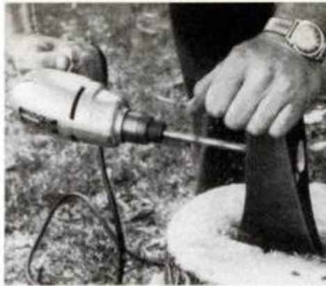
3 If the handle is exceptionally tight in the eye, bore several holes, then drive out the rest of the material.
