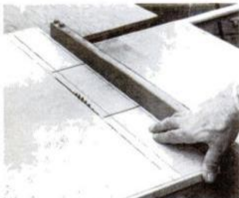
1 Elevate table-saw blade into work-piece to make internal cut for goal-end cutouts. Let blade stop, remove work.
