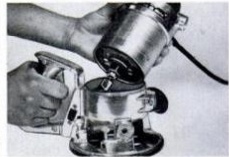
Next, router body is inserted in base, bit is set at approximate cutting depth.
