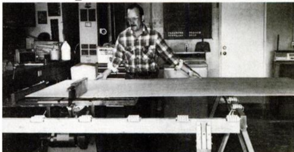
Install rollers on two sawhorses for easy, safe cutting of 4x8-ft. plywood.
