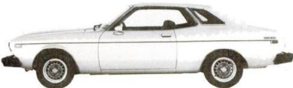
Two-door hardtop is added to 810 line; it, too, mounts the 2.4-liter, ohc, f.-i. Six.
