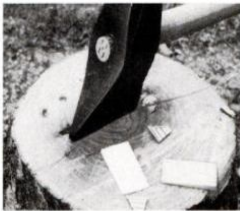
5 After making initial fit, check that wedges are large enough to expand the wood to fill the eye completely.
