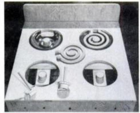
Close-up of burner assembly and knobs. Knobs are attached to snug-fit dowels.
