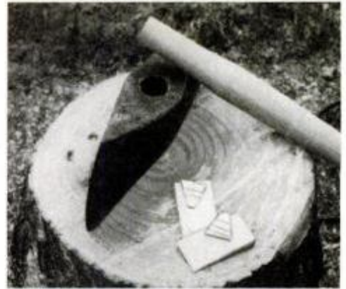
4 Fit new handle to tool eye. In some cases, excess wood will have to be removed to achieve proper fit (see text).
