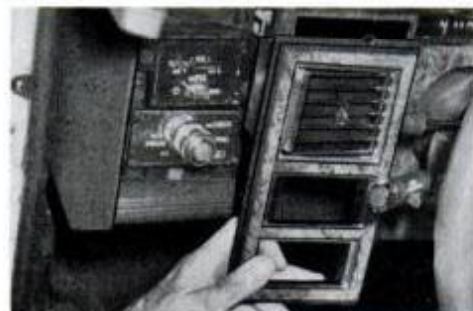
Behind-dash servicing is easy with removable bezels. At top, rear defogger switch is removed from the front. Access to left side of dashboard is shown above.
