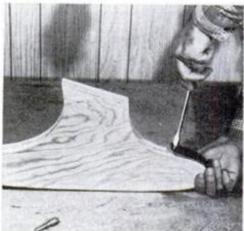
Countersink screwholes so screwheads are flush when runner is fastened to body.
