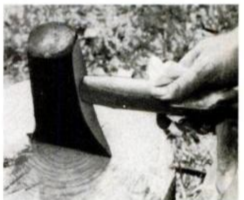
10 Rub down handle with boiled linseed oil, taking care to coat top of the eye and spots where trimming was done.
