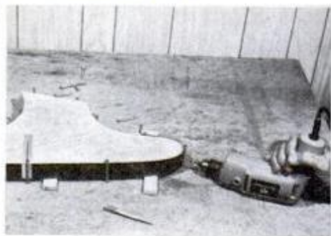
To use drill along centerline, elevate work-piece by placing 1 x 1-in. blocks below.
