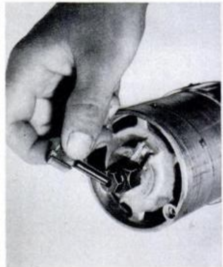
Collet is loosened and cutter is inserted fully, then withdrawn about 1/16 in.
