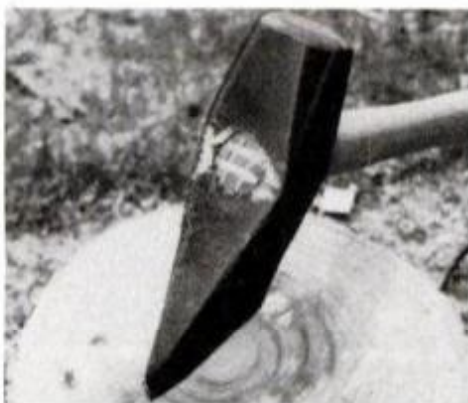
9 If job is done right, the new handle will be tight. Don't rely on wedges to correct mistakes made in fitting.
