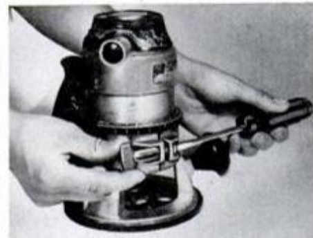
Use the micrometer collar—or a ruler—to set cutter depth accurately. Finally, secure body by tightening clamp screw.
