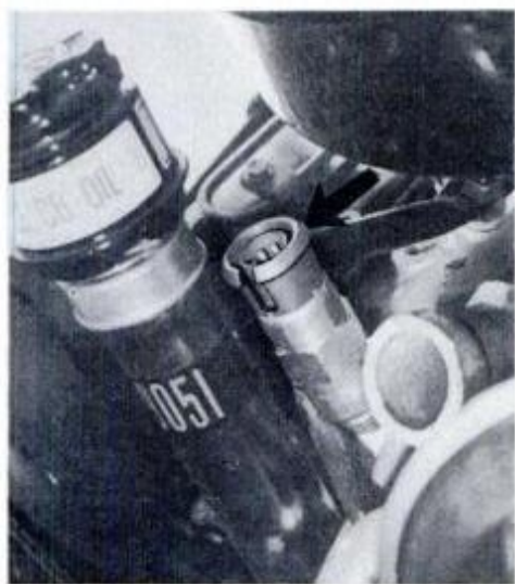
Controller (arrow) for fast-start glow plugs is threaded into the water jacket.
