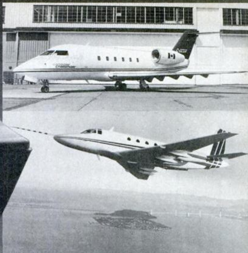
Canadair's Challenger (top) and Rockwell's Sabreliner 65 will vie for corporate sales. Note that both make use of pronounced fence array on underside of wings. Performance specs are on following page.
