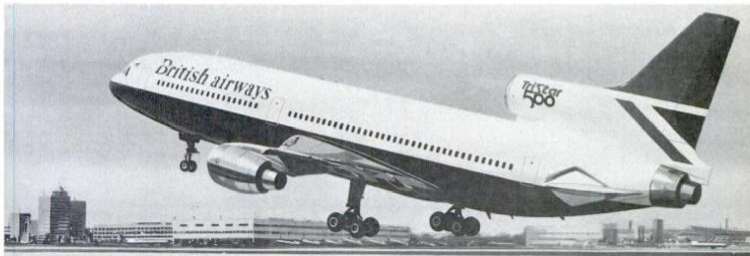
Lockheed's L1011 Dash 500, some 13 feet longer than the initial version, typifies the evolutionary airliner approach.
