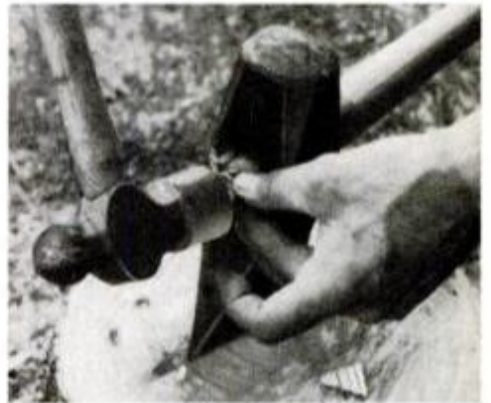
8 Drive metal wedges perpendicular to wood wedges. Small, almond-shaped ax eyes may need only one metal wedge.
