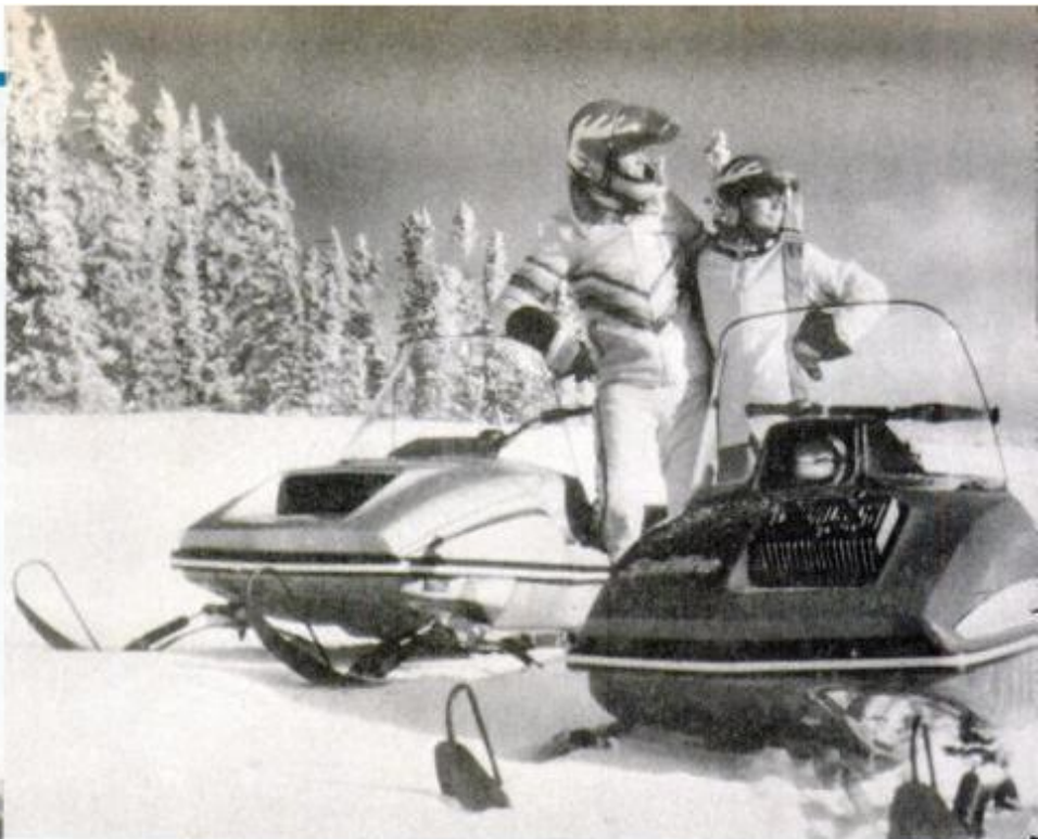
Newer Trailfires weigh 370 pounds for the 440, 364 for the 340 model. The Splitfire 338-cc (right), however, is a full-size lightweight of only 275 pounds.
