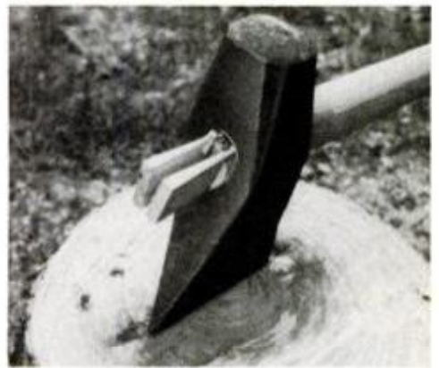
6 After opening up the wedge slots with a chisel, insert wood wedges (as shown) and drive in as far as possible.
