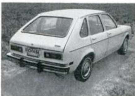
Rear hatch lifts on preloaded gas cylinder, gives good access to cargo area.
