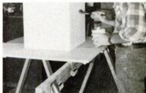
Sawhorses convert for regular use by simply flopping 2x4 cross member.
