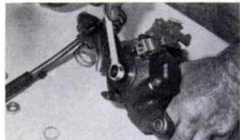
Rear disc brakes on E-bodies are new, can be serviced without use of special tools.
