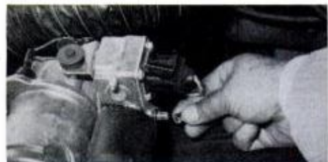
Airlift shocks can be inflated or deflated manually through the Schrader valve.
