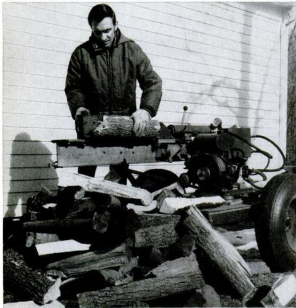
Plans call for 3-hp or greater gasoline engine, plus readily obtained stock parts.
