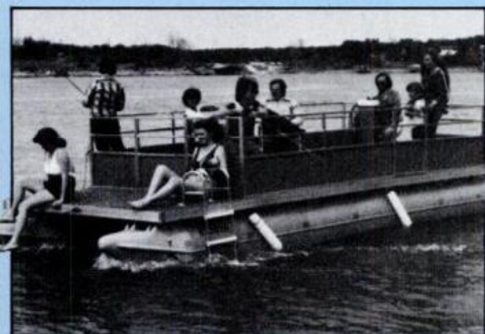
Pontoon deck boat uses Rotocast plastic units for flotation. The same floats can support a home-designed dock or swimming rafts of various dimensions.
