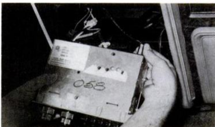
Bin-type glovebox is removable for access to behind-the-dash plumbing and wiring (left). It's easy to take out the radio. Just unscrew four retainers to remove the bezel, then remove two screws on radio (below, left) and pull it out. Disconnect the leads (below).
