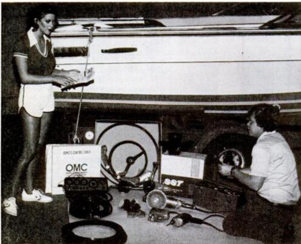
For a good job—and this is a job for a good mechanic—first assemble all parts and have an assistant inventory them by size and number on an installation checklist.
