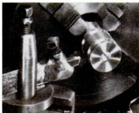
Cut grooves in the piston with a 1/4-in. tool bit ground to groove contour. See the groove-forming tool detail below.
