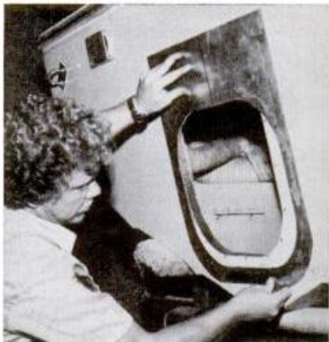
To alter the transom cutout, owner Ray Lind used a 3/16 x 20 x 24-inch aluminum plate. After marking the plate with a template supplied with the sterndrive, he cut the required opening with a sabre saw, then checked it against the old cutout.
