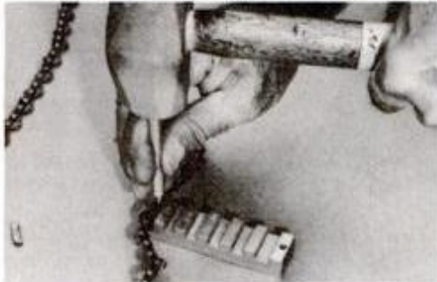
Two tools from Stihl that help repair saw chains are the pocket breaker ($3) (above, left), and the bench rivet spinner ($50). Breaker drives out rivets on chains from 1/4 through 1/2-in. Spinner makes easy work of replacing links. Adjustable guides hold the chain properly centered while you rotate the handle to form and seat rivets.
