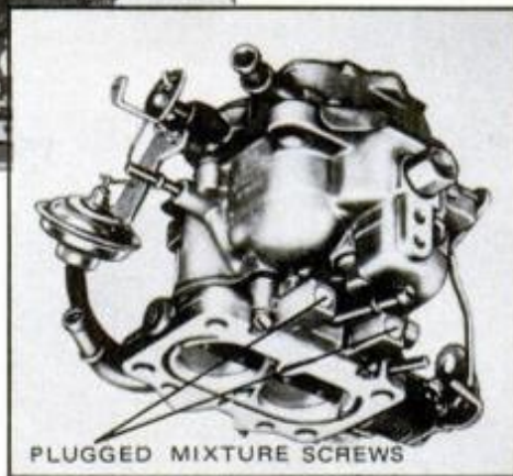
Slant Six engine installed in downsized Newport, New Yorker and St. Regis leaves good engine compartment room for do-it-yourself service. The two-barrel carburetor (below) does use mixture screws, but they are recessed and the bores are plugged.
