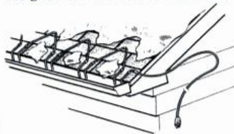
Tapes melt roof snow, prevent ice dams.
