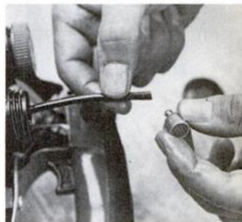
Also inspect the screen-type oil pickup filter which hangs inside the chain oil tank. Clean whenever it seems necessary.
