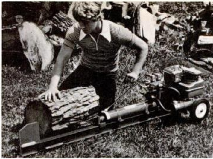
Wood splitter, model DB 19 priced at $500, splits a 19-in.-long log using seven tons of pressure. It's from Didier Manufacturing, 8630 Industrial Dr., Franksville, Wis. 53126.
