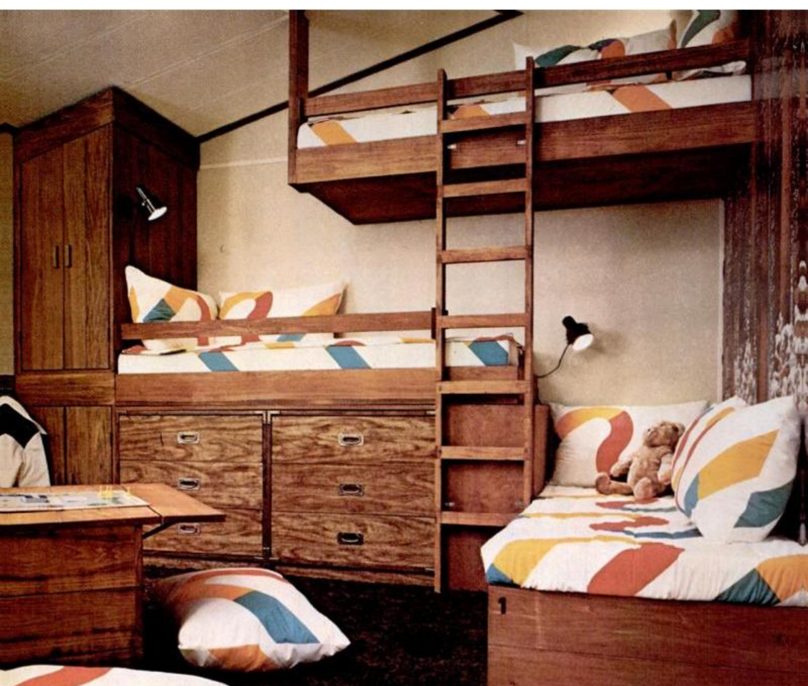
1 Ski-Trek room with its triple-deck bunks will please most youngsters. 2 The wall scene is a photo mural glued to foam-core board which, in turn, is affixed to wall with double-faced tapes. 3 Ladder to middle and upper bunks is permanently installed with wood screws.
