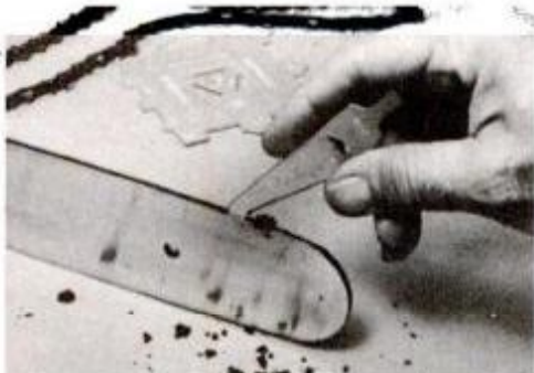
These tools from Stihl keep the bar in shape. The $1.25 Hook-N-Adjust (above, left), scrapes out packed, oily sawdust from the bar groove which can otherwise cause chain wobble and premature wear. The 50-cent test gauge (above, right), checks groove width of guide bar, chain and sprocket pitch and chain's drive link thickness.
