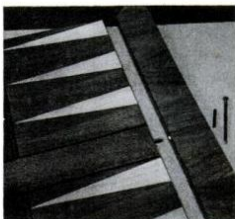
Insert nail pivots in gameboard (without glue) before assembling the frame.
