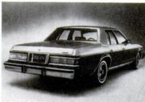
Dodge St. Regis is now lighter, 220.2 in. long, 77.1 in. wide and 54.4 in. high.
