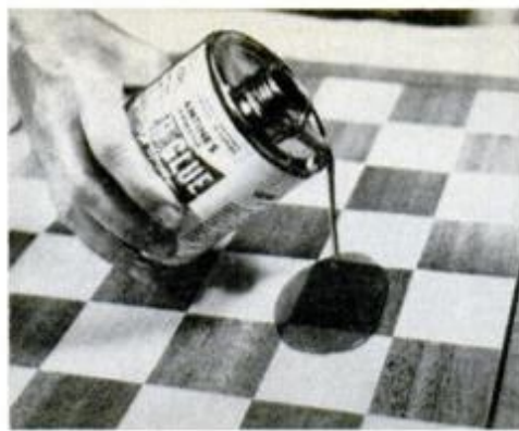
Spread veneer glue on back of veneer and on plywood; recoat one hour later.
