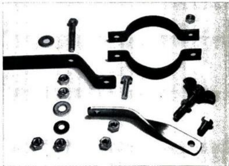
Bend your own column clamp for drill press lifter by using a form made from 2x4 scrap and applying pressure with a vise (above). Unassembled parts for lifter are at right.
