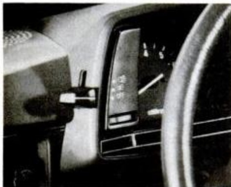
Light switch on instrument pod can be flicked while hands stay on steering wheel.
