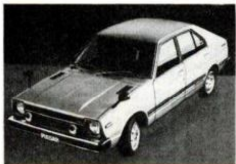
Pulsar uses 1400-cc transverse Four.
