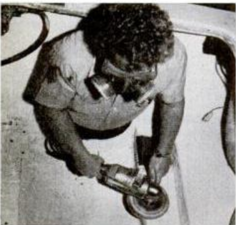
Fiberglassed engine mounts were discarded before stringers were widened with 2x6s bolted and fiberglassed in place.
