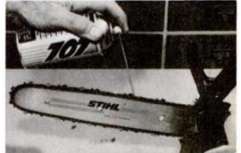
Apply 707 lubricant to a chain to minimize sawdust buildup, prevent binding. An 11-oz. can is $5.20. 707 Co., Inc., 405 Lexington Ave., New York, N.Y. 10017.
