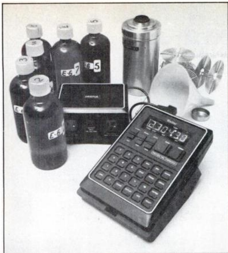
Process Time Commander is ready to control an E-6 run for Ektachrome transparencies. The timer's display has been set for program 2, step 3: 4 minutes and 30 seconds. Since the E-6 process requires that steps be of widely varying times, the PTC greatly simplifies the job when you're doing it at home.
