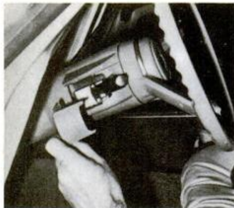
Stalk switch cover plate on steering column lifts off after removing single screw.
