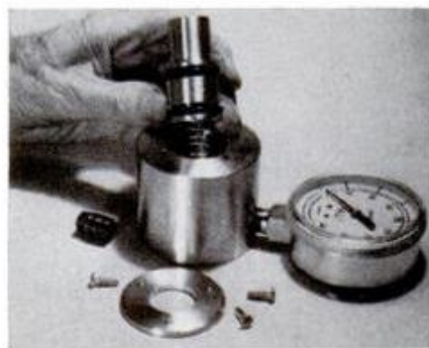
Complete assembly of scale by inserting piston; secure with retaining ring. Add oil through pipe plug and seal.
