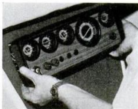
Full instrument panel is available with the new engine. Wiring connections are simplified with plug-in harness hookup.
