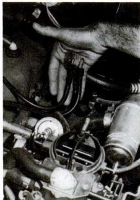
Vacuum spark advance regulator is used on all Sixes and 304 V8 with automatic.
