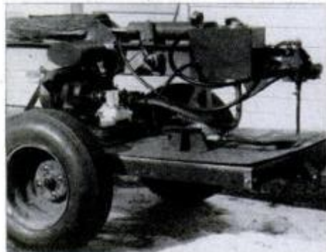
For best results, mount the log splitter on a two-wheel trailer and tow it to the cutting site with a garden tractor.
