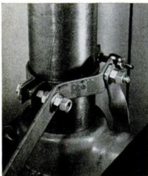
Locked nuts (two nuts jammed together) prevent loosening at pivotal connections.
