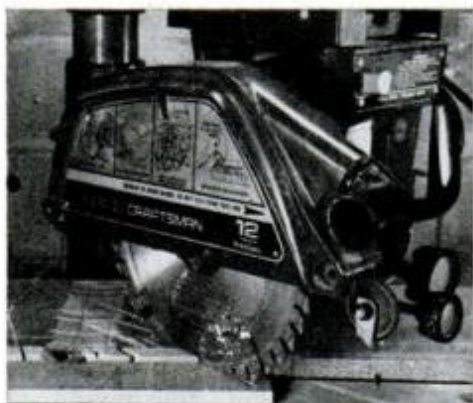
Miter frame members after measuring gameboard and providing for clearance.
