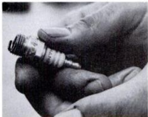
Check the gap and condition of sparkplug electrodes. Typical gapping is .025 in., but check recommendations in your manual.
