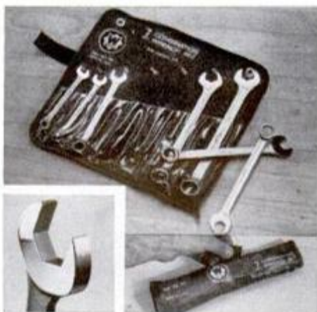
The wrenches come in a handy pouch. The V-notch design (inset) assures that you will have a good grip.
