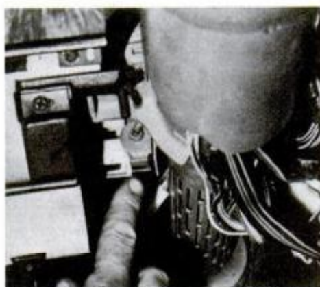
Dimmer switch, located lower on the steering column, is operated by linkage.
