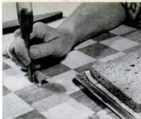
To remove gum paper on veneer, moisten small area with water; scrape with chisel.
