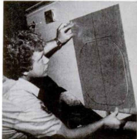
To alter the transom cutout, owner Ray Lind used a 3/16 x 20 x 24-inch aluminum plate. After marking the plate with a template supplied with the sterndrive, he cut the required opening with a sabre saw, then checked it against the old cutout.
