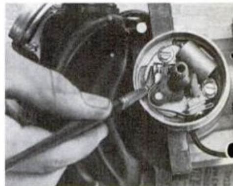
Clean breaker box and area around points with oil-free brush. Cardboard may be run between points to polish them clean.
