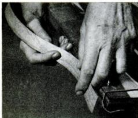
Bond veneer trim to gameboard edges with veneer glue, slipsheet. Trim overhang.
