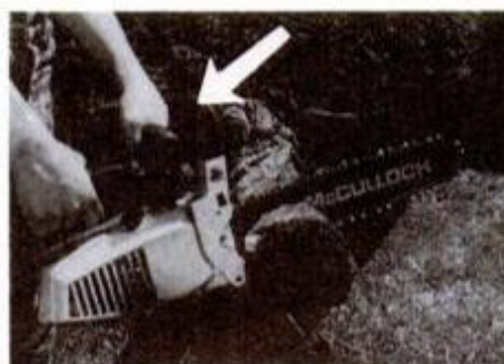
In normal use, the brake handle tilts toward the rear; the chain runs freely.
