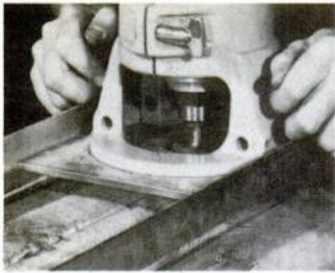
Even end grain can be surfaced to produce one-of-a-kind lumber finishes every time.
