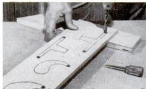
Bore saw-blade entry holes. One at each end makes it easier to cut narrow slots.
