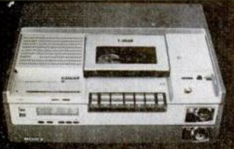
Tracking adjusts VCR to play tapes made on other machines. Tracking control on this Sony Betamax is hard to find and use.
