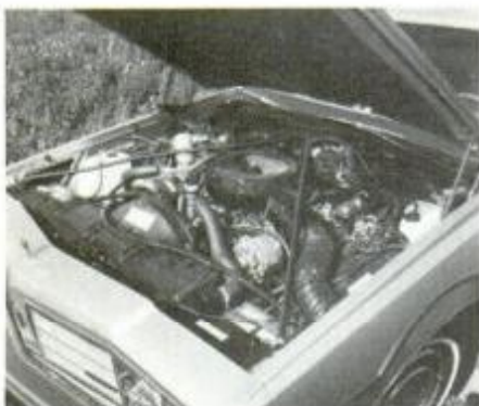
Oldsmobile's 350-cu.-in. V8 diesel is derived from the 350 gasoline V8.
