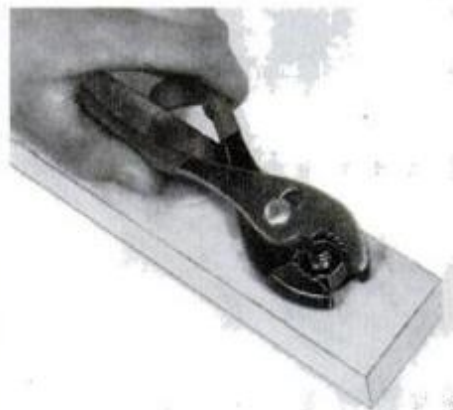
To remove small nail, pull at same angle it was driven, use block for leverage.
