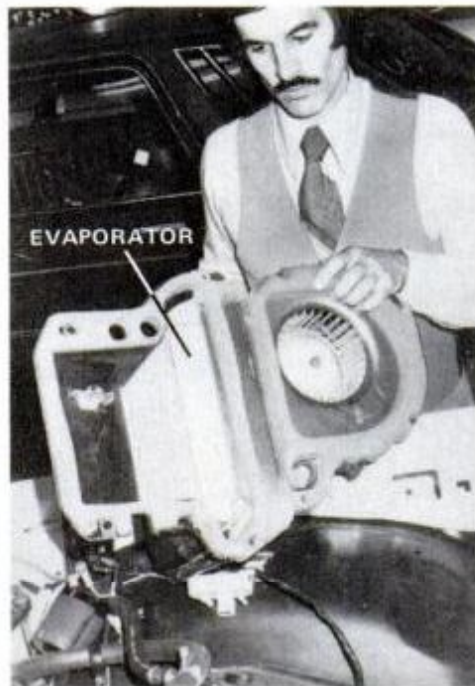
Evaporator is easily changed if necessary after duct section is removed from the car.
