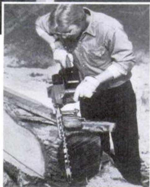
Large chunks of hardwood, such as parallel-cut log sections, are sliced using the Haddon Lumber/Maker guide. After air drying, wood is ready for surfacing.
