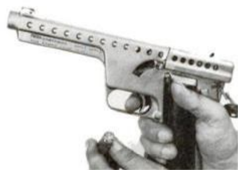
Rocket pistol made by American manufacturer fired tiny missiles with four venturis. It became an Air Force flare gun.
