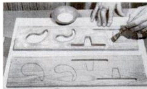
Use two nails to prealign shelf parts. Apply glue sparingly to mating surfaces, nail.
