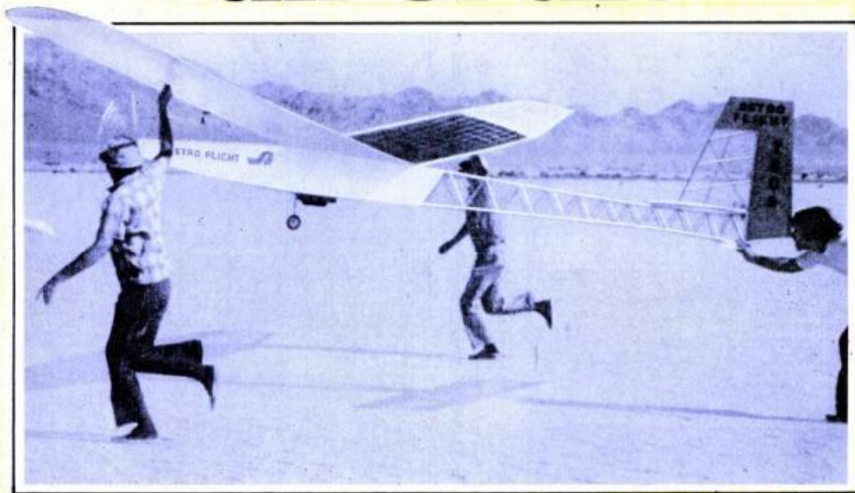
A remotely-piloted, solar-powered aircraft, built under an Air Force contract, Astro Flight 7404 takes off with help of runners on wings and tail. It can climb at up to 400 f.p.m., to altitudes of over 17,000 feet. But solar cells alone (dark areas on wings, right) cost $40,000.
