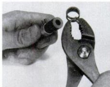
Pliers can be used to compress small spring clamp for hose installation.
