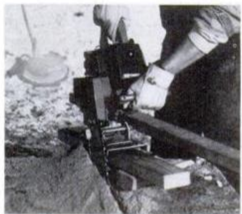
Lumber/Maker is also used to cut off log end sections to be surfaced in the jig.
