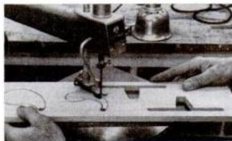
For precise cutouts, use set-tooth blade. For parts fit, remove line when cutting.
