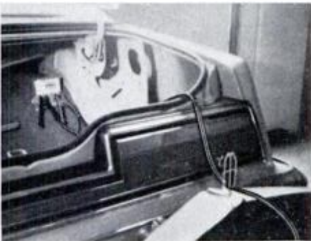
Battery posts mount at remote location.
