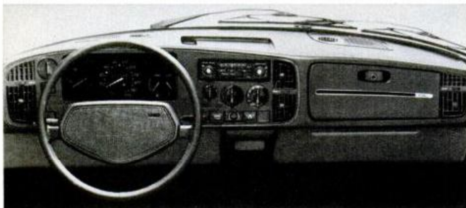
Saab 900 speedometer has electronic pulse transmitter to operate cruise control.
