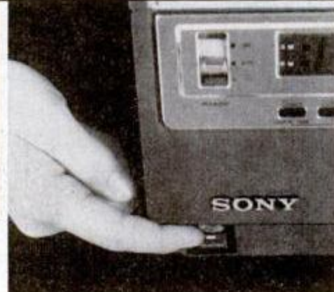
Tracking adjusts VCR to play tapes made on other machines. Tracking control on this Sony Betamax is hard to find and use.
