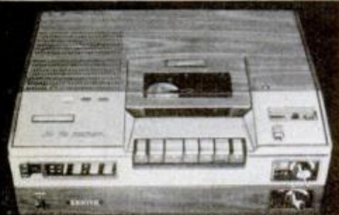
You won't run out of outlets near the TV set if your recorder has an auxiliary socket like this Zenith Beta unit.
