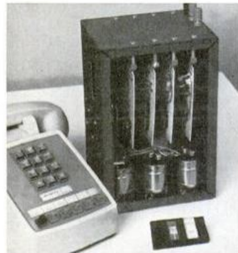
Present version of unit is somewhat bulky, but large-scale integration can put its circuits onto chips, like those in foreground, that will fit inside telephone.
