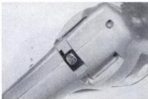
Reversing switch lets you back out screws and nuts—useful in freeing jammed bits.
