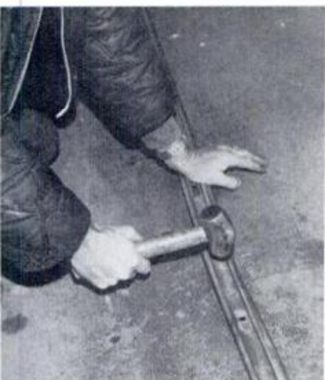
7 Hand sledge is also handy. Make certain work rests on a solid surface.
