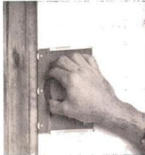
Pad-type edger is kept off stained molding by plastic wheels. You get sharp edge without use of protective tape.
