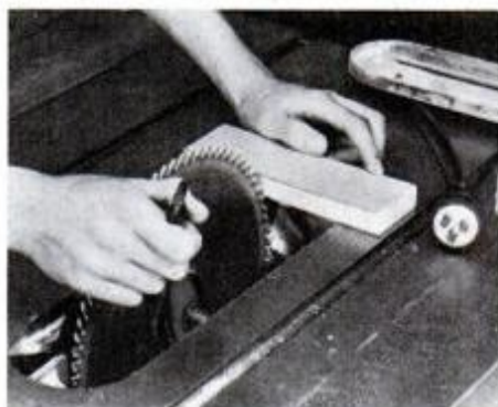
Disconnect power and hold block of wood against teeth to loosen arbor nut.
