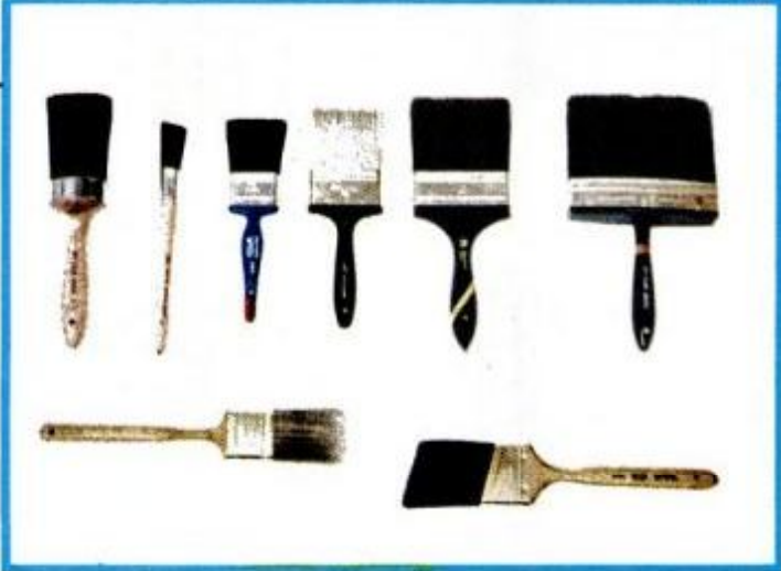
Brushes (left to right): oval varnish, oval sash, enamel, varnish/wall, wall, wall-coating; (bottom) flat and angular sash.
