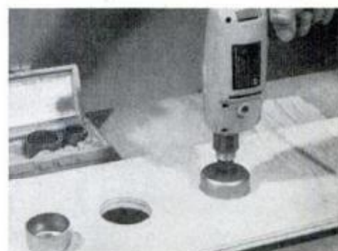
Cut holes up to 2 1/2-in. diameter with a hole saw, slow speed. Pilot bit centers cut.
