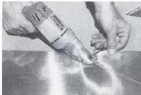
A shear head assembly fits the Milwaukee 1/4-in. drill to precisely cut sheet metal.
