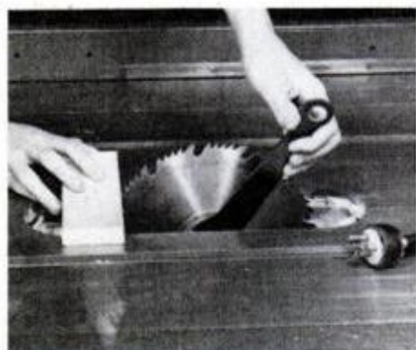
With block of wood against blade teeth at rear, install and tighten the arbor nut.
