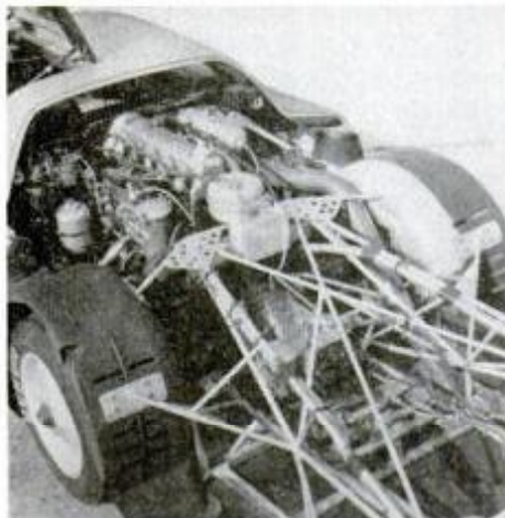
Midships-mounted, five-cylinder diesel is turbocharged for 230 hp SAE net.
