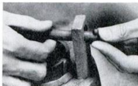
15. Roll handle coil, place it through the support holes and add a pea-sized handle stop near each handle end.
