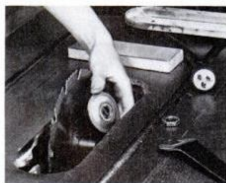
Put new blade on arbor, reinstall arbor washer that's provided with table saw.
