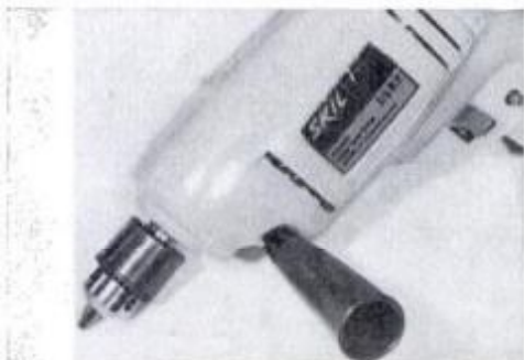
Side handle should be used on any high-torque drill for protection against twist.
