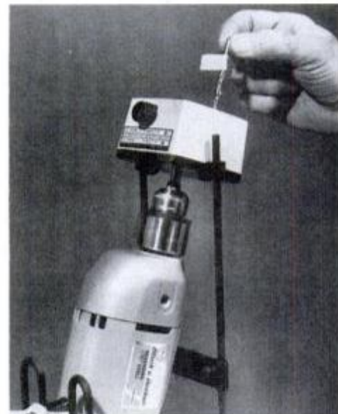
Black & Decker's sharpening attachment lets you sharpen a dull bit quickly.
