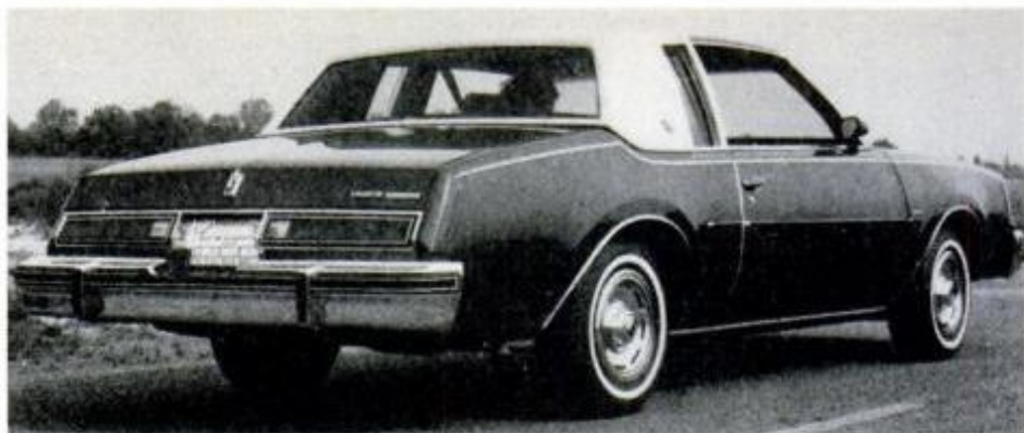
Regal shares GM's A-Special body with Monte Carlo, Grand Prix, Olds Cutlass.
