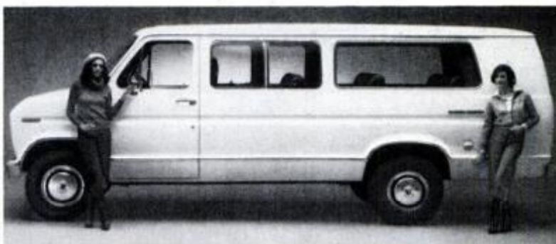
Ford has stretched its Econoline Vans and Club Wagons. Super Van and Super Wagon (above) have 14-foot cargo floor, can seat 15 passengers, carry 5025 pounds or tow trailers weighing 10,000 pounds.
