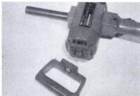
Four-position D-handle on this heavy-duty drill gives the user maximum tool control.
