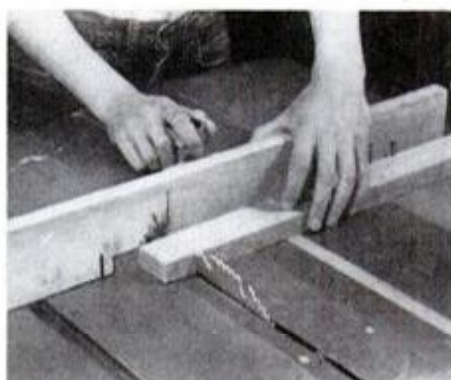
Always use the miter gauge when cross-cutting—never crosscut freehand.
