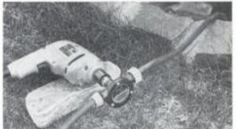
Drill pump is useful for draining plugged sinks. Never use it on volatile liquids.
