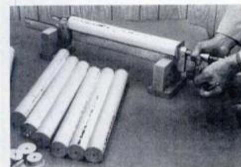
Press plugs into pipe ends using a bar clamp, or tap the plugs in with a mallet.
