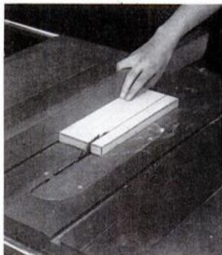
When using a rip fence to rip boards wider than 3 in., hook your last two fingers over the fence as shown above. For cutting narrow stock, see below.
