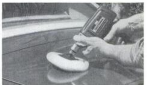
Swivel-jointed polishing pad and bonnet flexes to 30° angle, follows contours.
