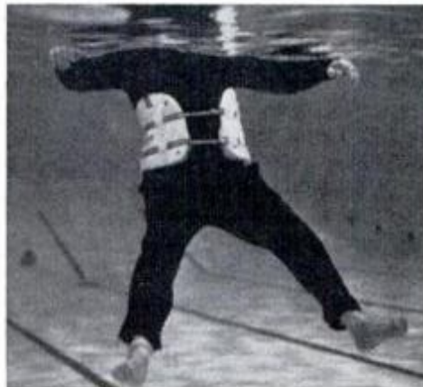
Foam belt pad protects thorax from cold, keeps head high, is worn under clothing.
