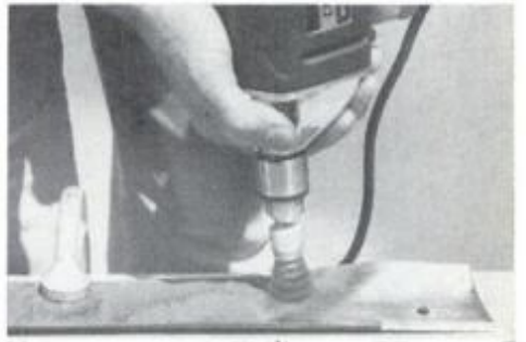
Rugged, twisted-end cup brush quickly removes rust, scale and carbon from steel.
