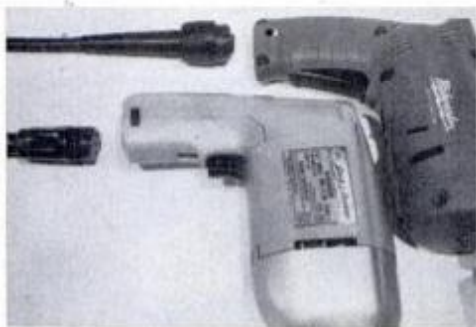
Some drills have detachable cords that are stored conveniently in your tool chest.
