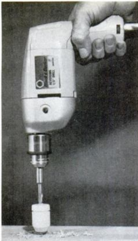
Plastic collar tightens at any position on the bit to control depth of the hole.
