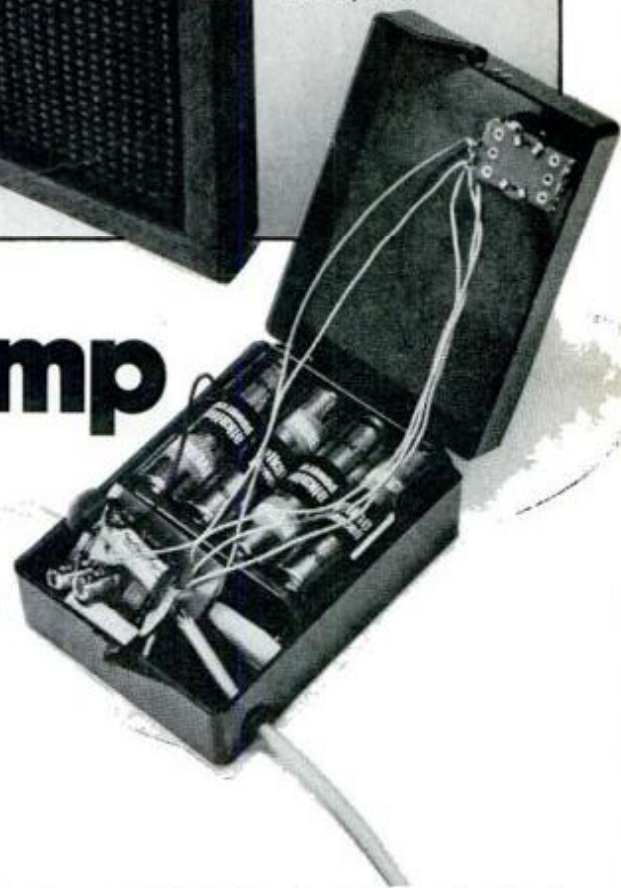
Hooked up to the tuner output of a small AM/FM portable radio and driving two Poly-Planar foam speakers (here encased in grille cloth and a simple wood frame), the booster amp gives clear sound at surprisingly high volume levels. The amplifier itself is on the small circuit board inside the box below—batteries take up most of the available space.
