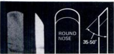
Round-nose chisel can be used for coves and the like in spindle turning, for concave cutting in faceplate turning (bowl interiors). The tool is used with a scraping action; a sharp one produces a very smooth cut. Sizes from 1/4 to 1 in.
