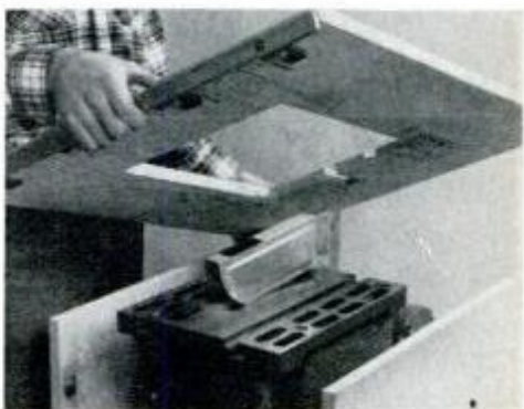
Use 1 1/2-in. No. 8 fh wood screws to fasten table to base. Countersink heads to prevent workpieces from being snagged.
