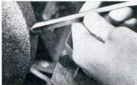
Gouge bevel can be ground as above or as in photo at left. Watch bevel carefully.
