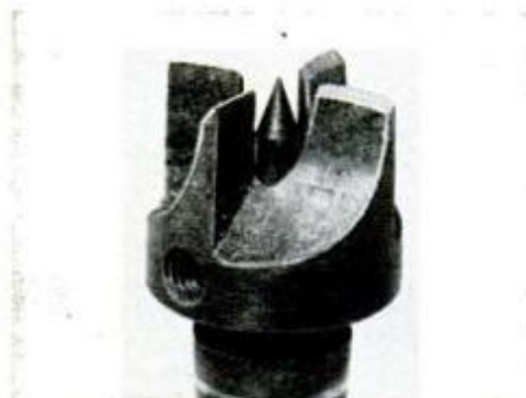
Drive center fits into headstock spindle, turns the work driven between centers.
