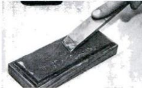
To whet skew, pour oil on stone, keep bevel in full contact, use figure-8 motion.
