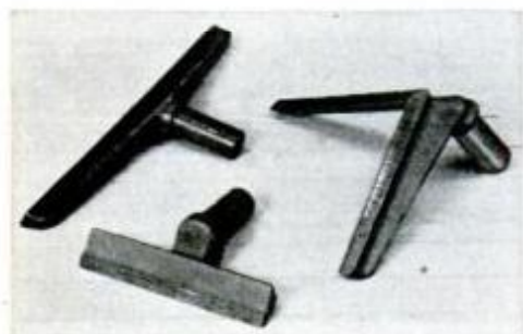
Toolrests come in various sizes, shapes. Shown are 6- and 12-in., and right-angle.
