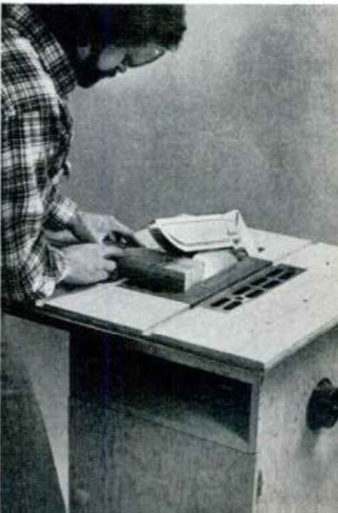
Use 1 1/2-in. No. 8 fh wood screws to fasten table to base. Countersink heads to prevent workpieces from being snagged.
