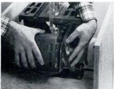
Motor is suspended by drive belt—and allowed to slide or pivot on rod supported by two eyebolts fastened to saw bottom.
