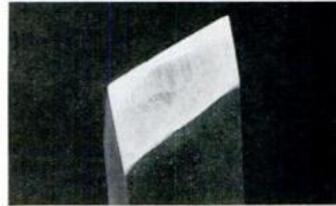
When "wire" forms on the edge, turn the skew over and whet its second bevel.
