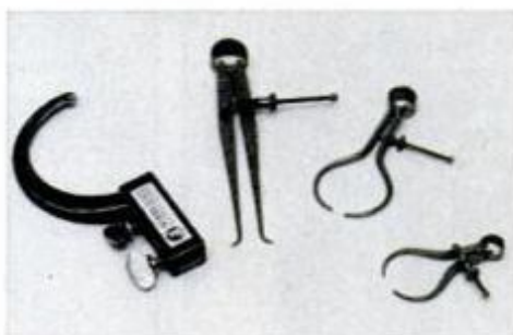
Assortment of inside and outside calipers is needed to check diameter of work.
