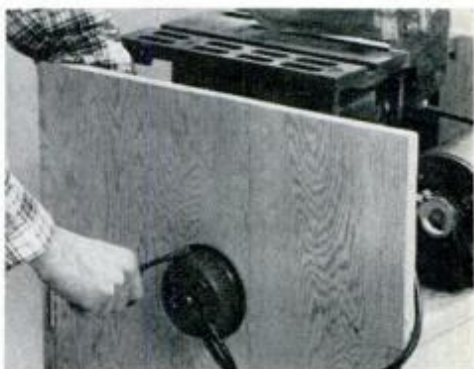
Locate switch within easy reach—but not where it can be bumped and accidentally turned on while making adjustments.
