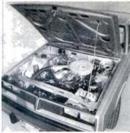
Silent Shaft MCA-Jet engine has hemi-head; counters pollution, vibration.
