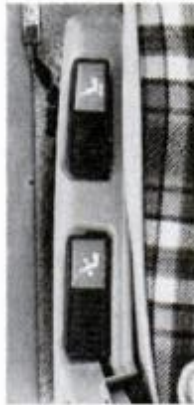
Optional overhead console (above) on Challenger and Sapporo contains big interior light plus reading spotlights, digital liquid crystal display (LCD) clock. The levers located beside the driver's seat (left) are remote releases for trunk lid and flap door over the fuel-tank filler neck.
