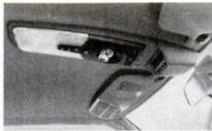
Optional overhead console (above) on Challenger and Sapporo contains big interior light plus reading spotlights, digital liquid crystal display (LCD) clock. The levers located beside the driver's seat (left) are remote releases for trunk lid and flap door over the fuel-tank filler neck.
