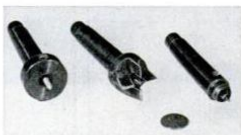
Screw (left), drive and spur centers; the first is for small faceplate work.
