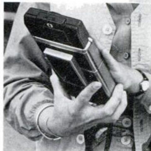
Sonar unit adds about 1½ inches to length of folded camera, is powered by flat battery in SX-70 film pack.
