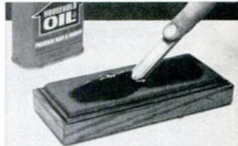
To whet the gouge, pour oil on oilstone, stroke the gouge using a circular motion.
