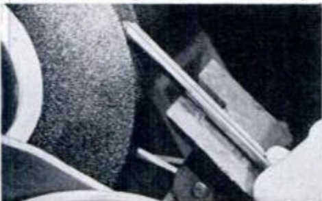
To restore cutting edge to correct angle, grind tool on grinding wheel with true face.
