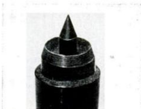
Cup, or dead, center is used at tailstock to support the outboard end of spindle.
