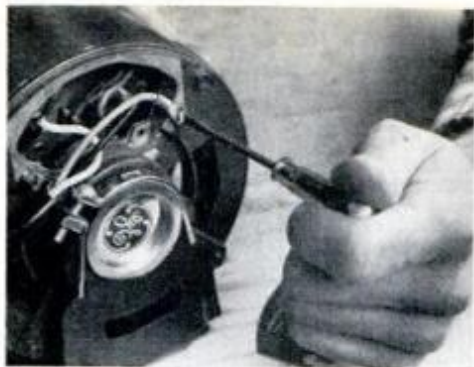
Attach black and white wires to leads (either wire to either terminal). Secure green (ground) wire to cover plate screw.
