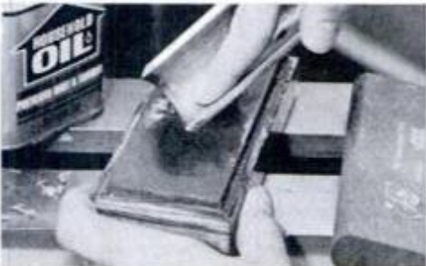
As gouge is moved in circular motion, rotate the beveled edge from left to right.
