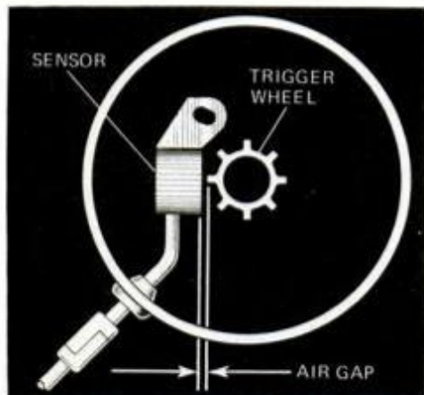
Air gap adjustment between sensor and trigger wheel of the International system.
