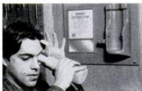
Author demonstrates emergency eyewash bottle—a precaution in addition to goggles—which quickly flushes out particles.
