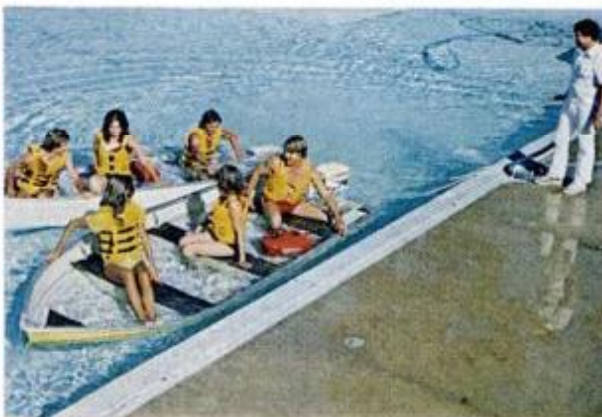
As boats start to sink, starter batteries would have been drowned out, fuel tanks begin to float, righting tendencies of hulls become more sluggish. Boats without under-gunwale flotation tend to roll more.
