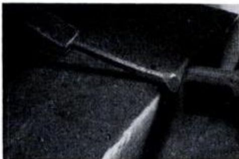
3. Curl the button by extending it over anvil edge, hammering as you move it.
