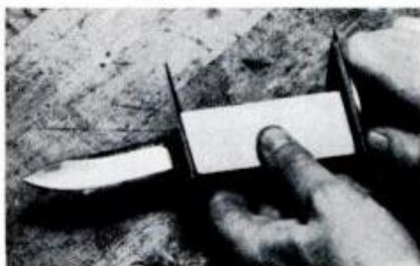
Knife is assembled with handle between spacers, and nut tightened to check fit.
