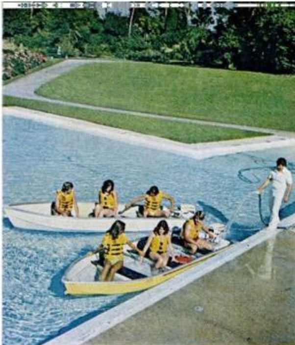
Under controlled conditions, in the Cypress Gardens Aquarama pool, identical 14-foot hulls with 15-hp outboards are flooded with a fire hose while stability of top and bottom flotation is compared.
