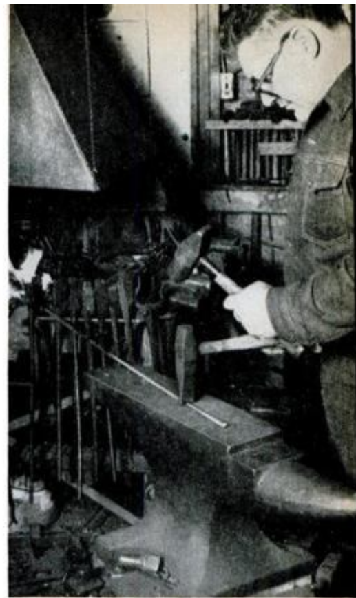
Kayne cuts steel with cross peen hammer and chisel, striking it on both sides.
