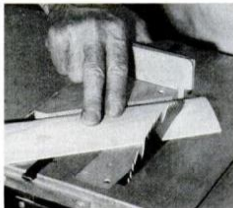
The 45° angle block makes mitering door or window casings quick and easy.
