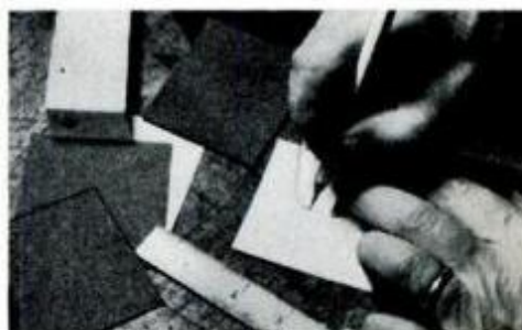
Spacers are selected to fit against nickel silver hilt, butt nut, and cut for tang.
