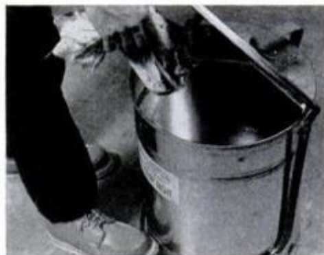
Container for oily wastes confines highly combustible material until it can be safely removed from the shop and left out for trash pickup.
