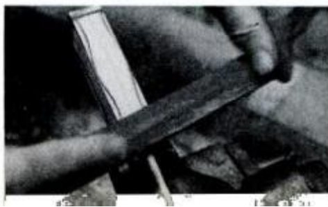
Blade, taped for protection, is clamped in vise for rough shaping of the handles.
