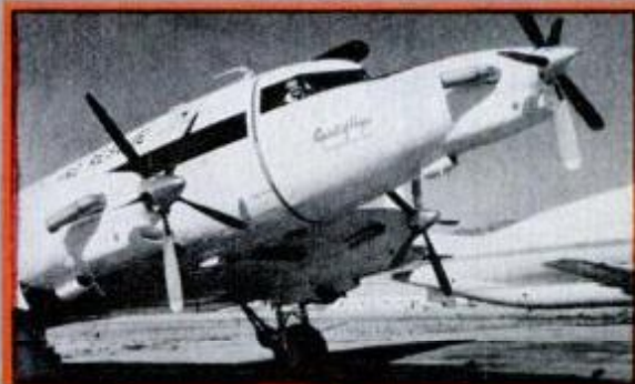
Lined up to unload (top), C-47s (cargo versions of DC-3) played major role in famed Berlin Airlift in 1948, breaking Russian blockade of city. Above, a DC-3 lives on as a sleek, new trimotor turboprop.
