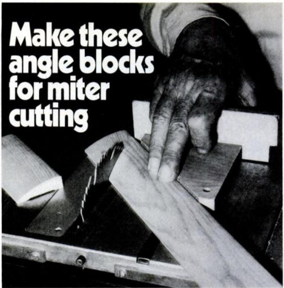
Angle blocks save time, assure accuracy. Blade guard is removed for photo clarity.
