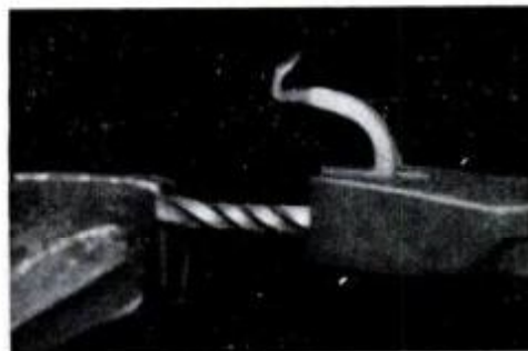
6. Heat twist area to cherry-red. Hold with vise and tongs; pull as you twist.
