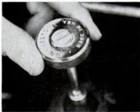
Thumb-wheel ratchet is for tight places.
