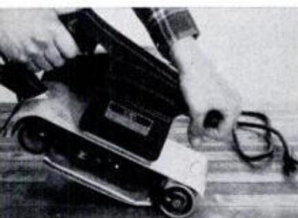
Front pulley is pressed against bench to release tension on belt to be removed.
