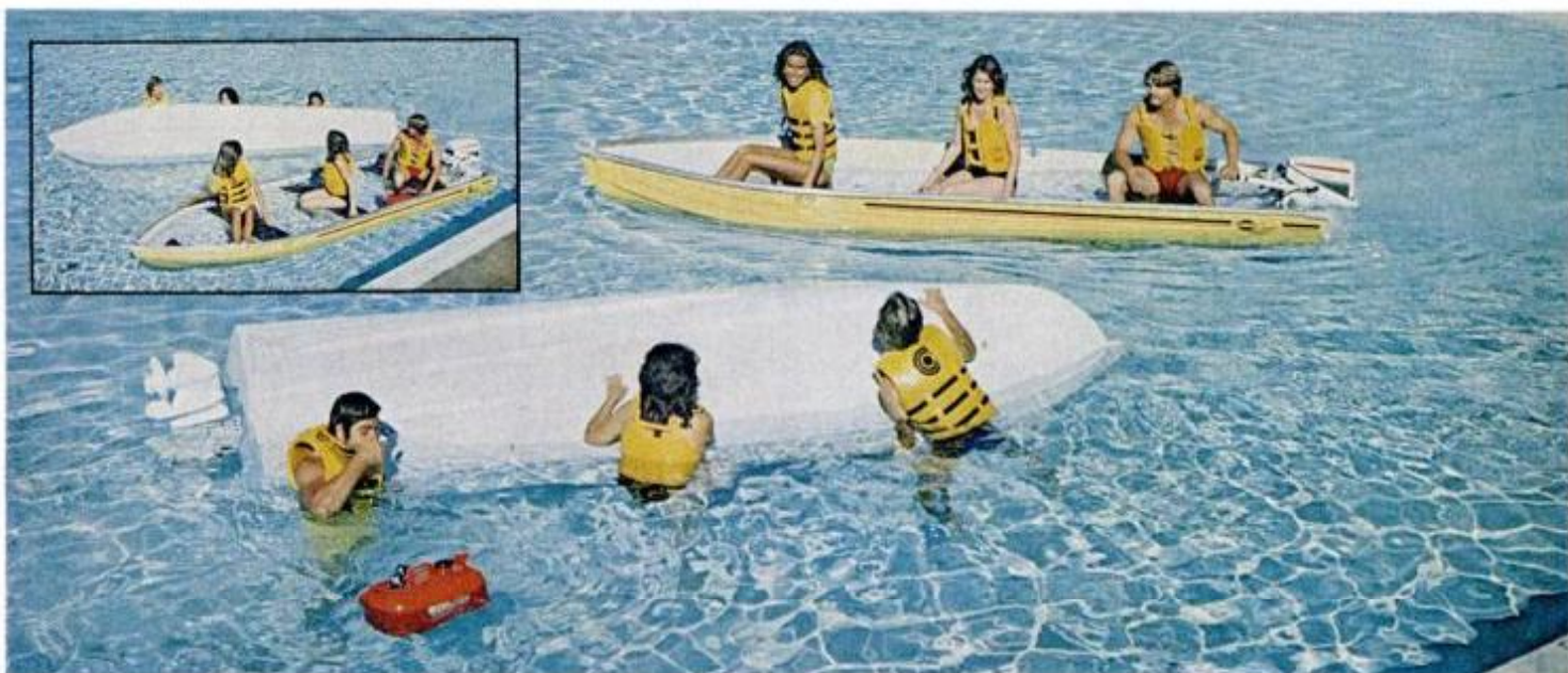
Conventional flotation boat (inset) starts to capsize; can't be kept upright. It won't sink but drowns engine, makes poor raft.
