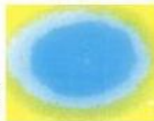
Ordinary Spray Gun Oval pattern hard to control. Misting and extreme feathering require extensive use of drop cloths and masking.
