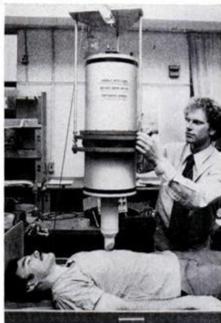
SQUID zeroes in on weak magnetic field.
