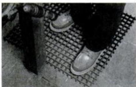
Antifatigue mats placed at work stations are great leg savers—especially if your shop has a concrete slab floor.
