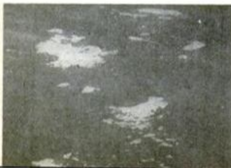
FINE BLISTERING, FLAKING. Bare spots appear; may be due to surface moisture.
