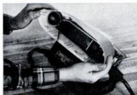
New belt is slipped over both pulleys, arrow on inside must point to the front.
