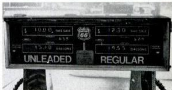
Electronic gasoline pumps are gradually replacing the older types of pumps designed to read out the price and gallons mechanically.
