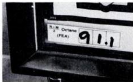
Posted octane number, or antiknock index, is average of Research and Motor octane numbers; must be on all pumps.
