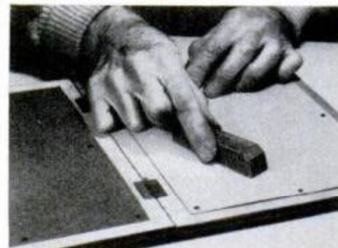
Open the sanding book and rub your work-piece back and forth on the desired grit.
