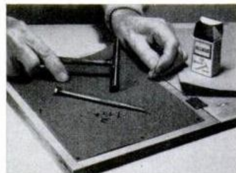
Fasten sandpaper to the plywood with upholstery tacks or 1/4-in. staples.
