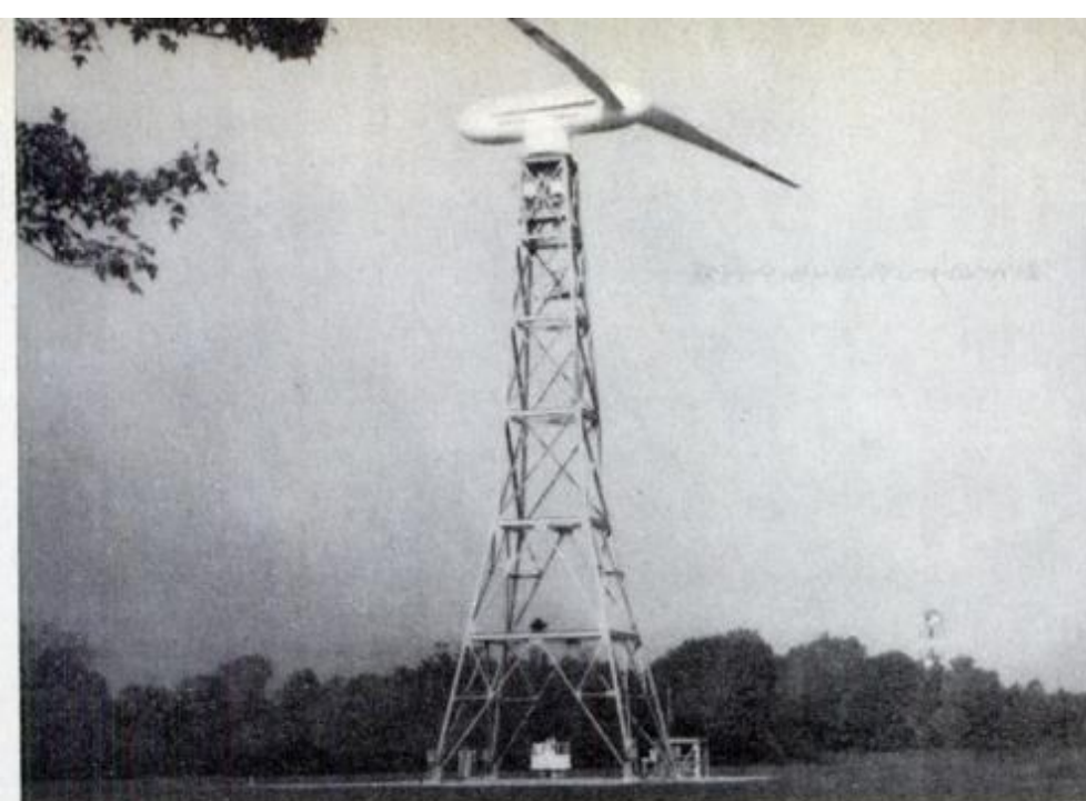
Simple tail-aimed Dunlite windmill is made in Australia and sold here by several U.S. companies. It has electrical output of 2 kilowatts in 25-mph wind.
