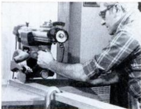
14 To cut the long notch at top, clamp 2x4 to table, support outboard end.
