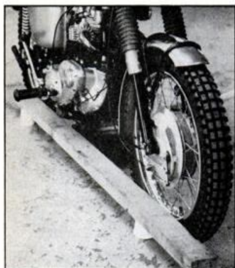
Wheel alignment can be checked with any one of several methods including boards.
