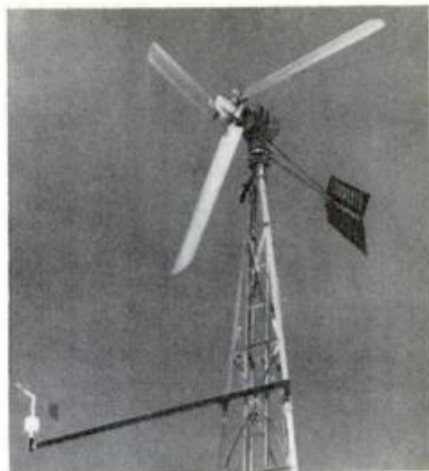
Simple tail-aimed Dunlite windmill is made in Australia and sold here by several U.S. companies. It has electrical output of 2 kilowatts in 25-mph wind.
