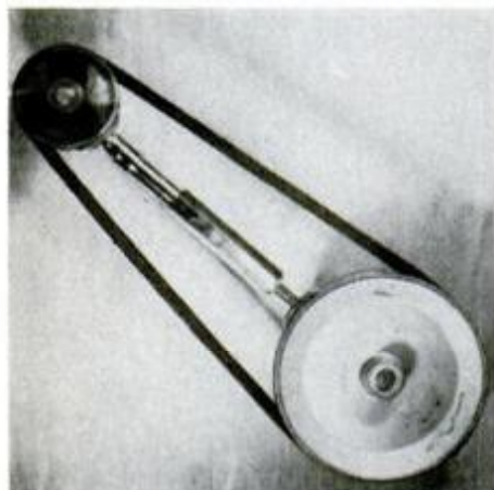
Belt tensioner works like a screw jack.
