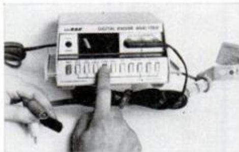
Engine analyzer, this one a digital type, offers many functions in one instrument.
