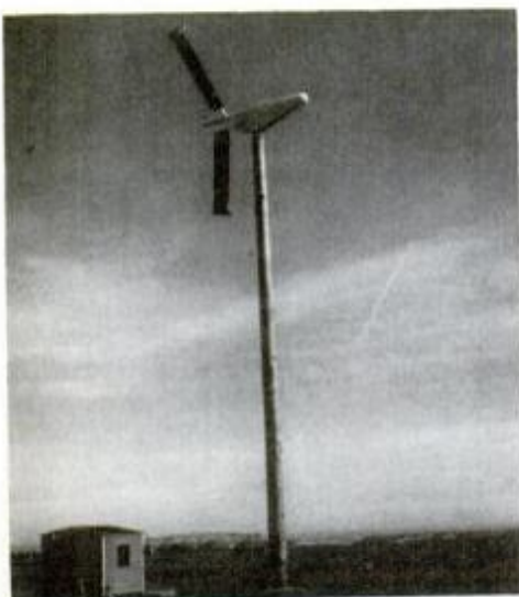
Grumman's Windstream-25 is one of several commercially available windmills designed for private use. It has a rated output of 15 kilowatts in 26-mph wind.
