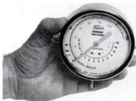
Vacuum gauge is an essential diagnostic tool. Large dial face is easy to read.
