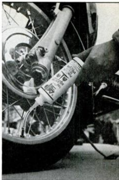
Squirting in a charge of tire-balancing fluid is a quick way to improve balance.
