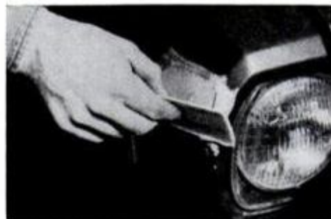
Fill in wrinkles with a body filler after preparing the surface thoroughly.
