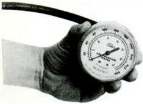
Compression gauge pinpoints conditions inside your engine—and it's easy to use.
