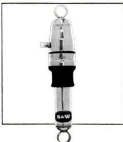
Fine control of rear suspension is achieved with air-adjustable shocks.
