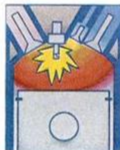
Ignition and combustion phase.
