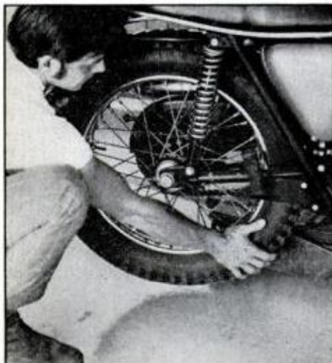
Wheel bearings are checked by rocking wheel and determining amount of play.
