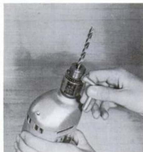
Next, use chuck key that comes with the tool to tighten bit securely in chuck.
