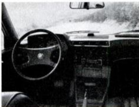
Instrumentation includes readout panel for levels of most fluids under the hood.
