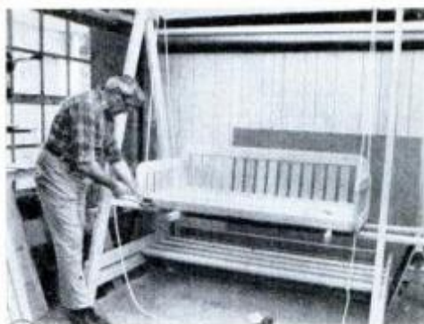
17 Prop seat on horses to install rope, push knots in counter-bores.
