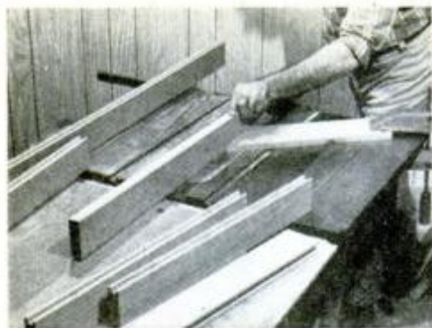
1 Top and bottom rails for back and sides are grooved to receive slats.
