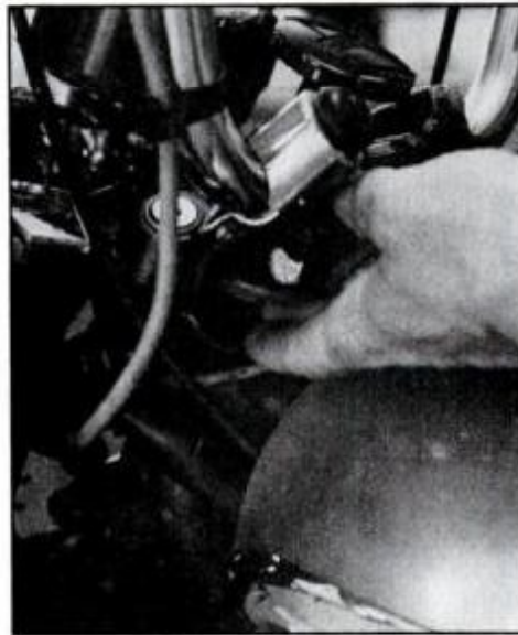
Another method for checking head bearings is with front brake on (see text).
