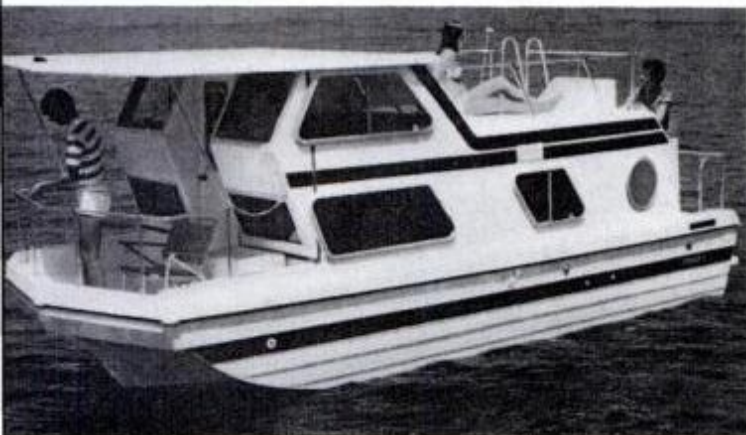
Outboard motor or stern drive push Steury's 23-foot T523 five-sleeper afloat; 8-foot beam allows trailering ashore.
