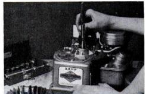
12 Points are gapped following instructions. Parts are then reinstalled.
