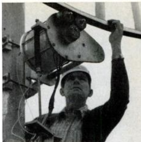
Rim-driven generator is feature of "bi-cycle windmill" under study at Oklahoma State University. Rotor is shaped like a bicycle wheel with rim connecting blade tips. Advantage: Rim travels much faster than hub, drives generator at high speed.
