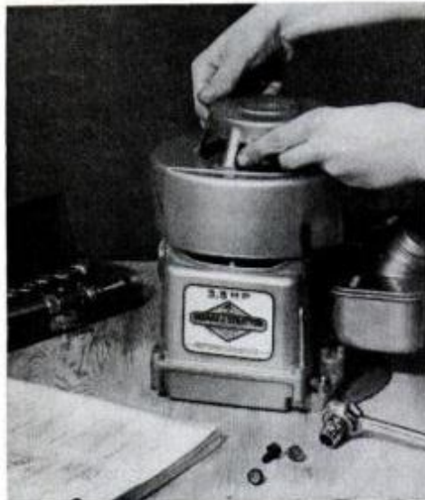
8 To gap points, follow book sequence. Start by removing cover.
