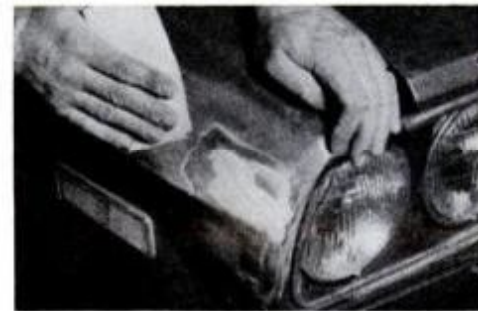
Sand the repaired area as smooth as possible with a fine grade of sandpaper.
