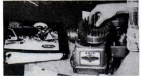
11 Flywheel is lifted off to expose the points in B&S engine.
