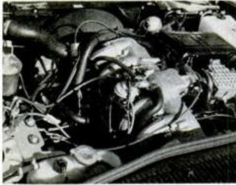
Fuel injection hardware is apparent on the 733i's in-line, overhead-cam Six.
