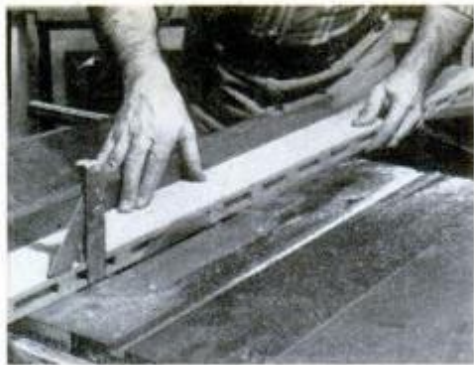
3 After glue dries, trim the rails slightly using a smooth-cutting blade.
