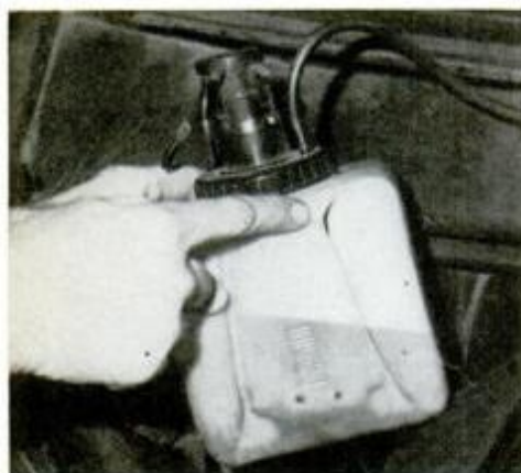
When windshield cleaning-fluid reservoirs crack, try patching before replacing.
