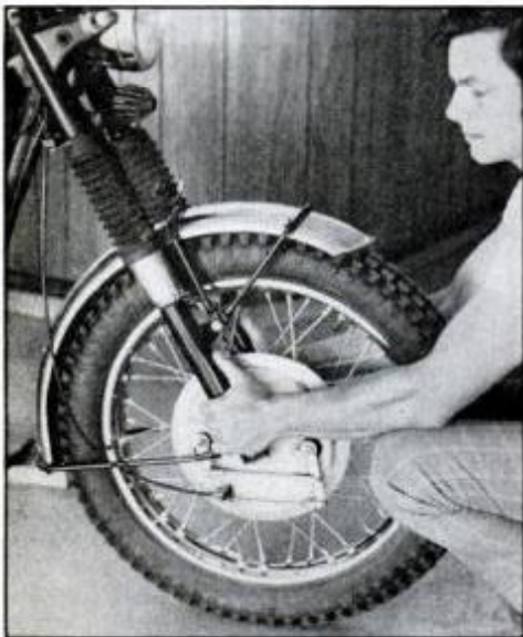
Steering-head bearings and fork-leg bushings should be checked for looseness.
