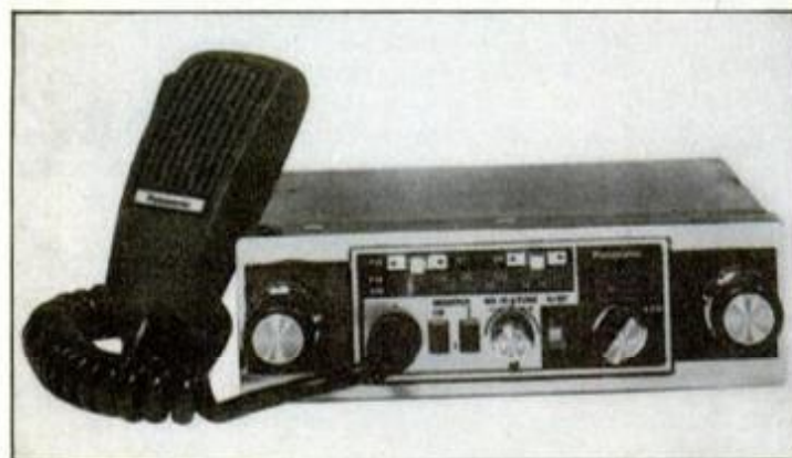
Monitor feature on Panasonic CR-B4700 interrupts AM or FM stereo radio whenever there's a signal on channel you've chosen.
