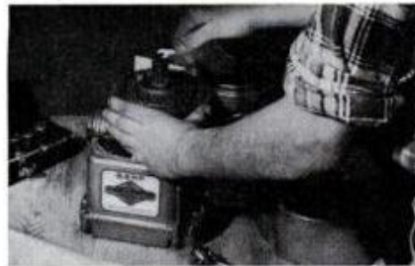
9 Next, mesh screening comes off so that the flywheel is exposed.
