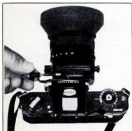
Turn knob to shift lens off optical axis. Scale on top gives an accurate guide.
