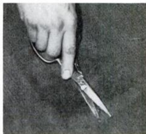
9. Use a long needle to intertwine yarns at seams; clip carpet fuzz near the patch.
