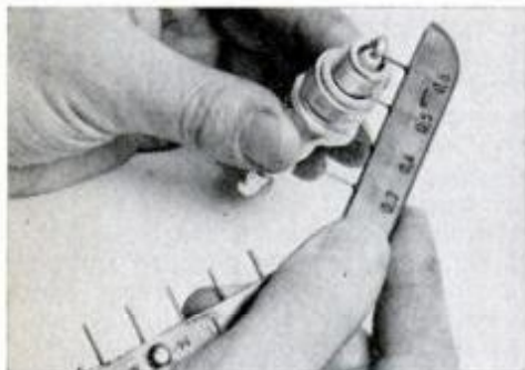
Check and set sparkplug gap. A gauge in your garage and your car is a good idea.
