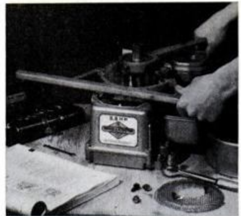
10 Book illustrates technique for using tools to remove the flywheel clutch.
