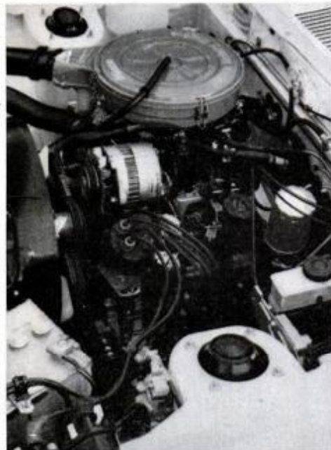
The RX-7 Wankel-type rotary engine, designated the 12A, has undergone many design refinements to achieve goal of better mileage and longer life for a rotary.
