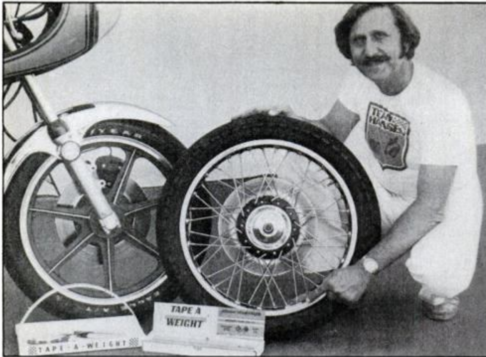
Balance weights with adhesive backing make tire and wheel balancing easier than ever. These Tape-A-Weights are especially easy to use on cast-alloy wheels (left).
