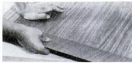
Next, bend cutoff portion up—that is, against the decorative surface as here.
