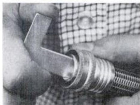
Male and female couplings are secured to hose by screwing ferrule into opening.
