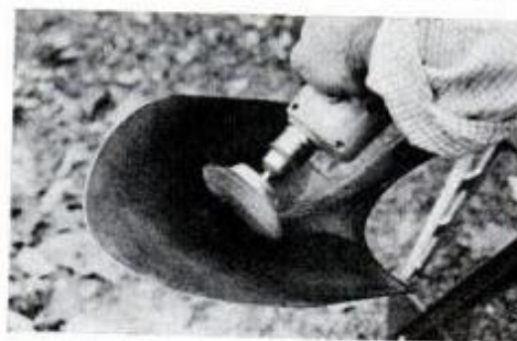
Wire cup brush, chucked in drill, is an easy way to remove rust from shovel.
