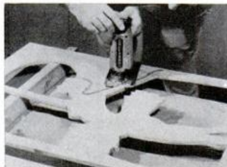
To minimize vibration damage, the hands and feet of this figure will be cut last.
