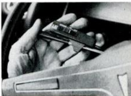
Engagement switch mounts on stalk, is preferably about \frac{3}{4} inch from the end.
