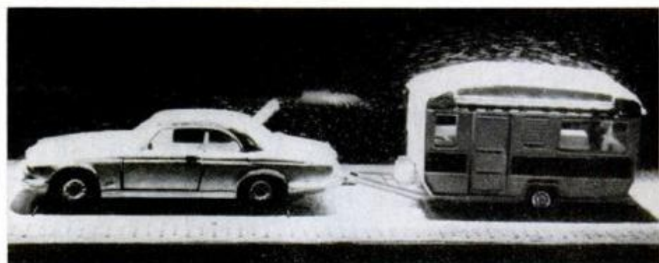
Sedan "pulls" house trailer underwater in special tank. Bubbles trace the "airflow."
