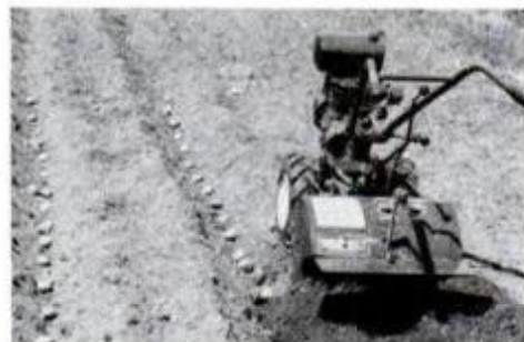
Wings which attach to the furrower can be used for hilling and making raised rows as well as covering seed in furrow.
