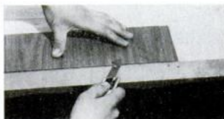
Use hook part of blade to dress newly cut edge; blade back can also be used.
