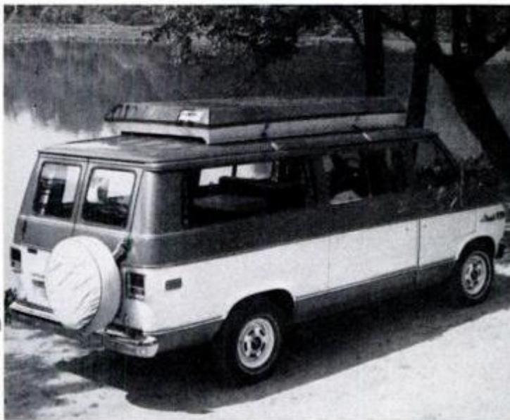
Vans and large station wagons can increase space without cutting top or sides with the Jutter, from J.C. Industries, Cherry Hill, N.J. A detachable 125-pound package mounts on the roof and opens into 4x8-foot sleeping loft and 8x8-foot room with roll-down sides.
