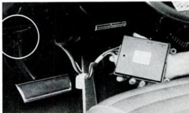
Under-dash work includes installation of disengagement switch to brake pedal arm (detailed at left) and disengagement switch anchor (not visible); connection of wires to main harness. Regulator (hand-held) is compact, easy to position.
