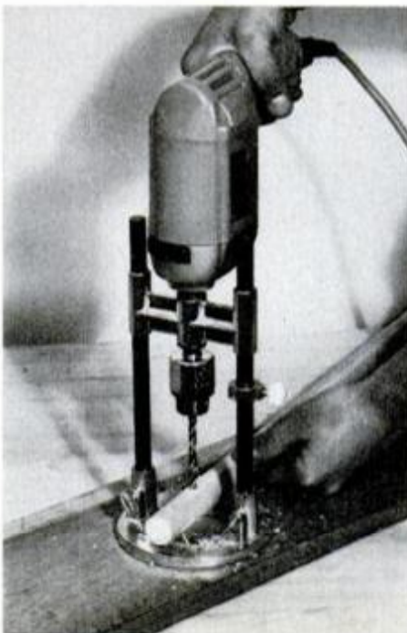
Depth of bore is determined and assured by locking wingnut. V-blocks mounted on Portalign's base make it a snap when you have to bore round stock accurately.
