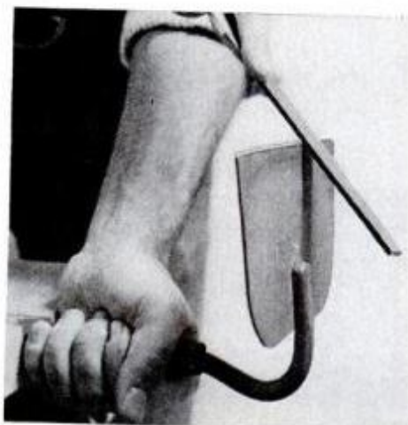
Properly beveled edge increases hoe control by helping it bite into the ground.
