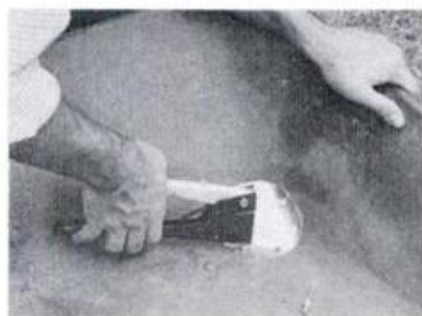
Rivet tool makes awkward patching easy. Use standard, medium-duty Pop rivets.
