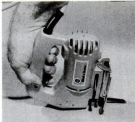
For plunge cut, use short, stout blade. Pivot saw into wood as it reaches full speed.
