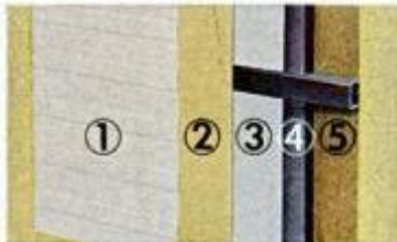
Vacubond™ 1. Prefinished aluminum 2. Wood backing panel 3. Block foam insulation 4. Steel framework 5. Interior panel
