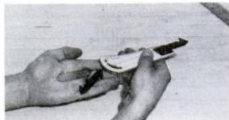
Five blades come with the cutter. They store conveniently in the handle.
