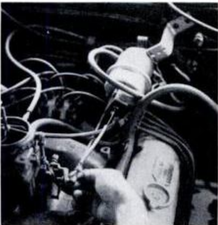
Servo is mounted on firewall and its cable is secured to throttle linkage.
