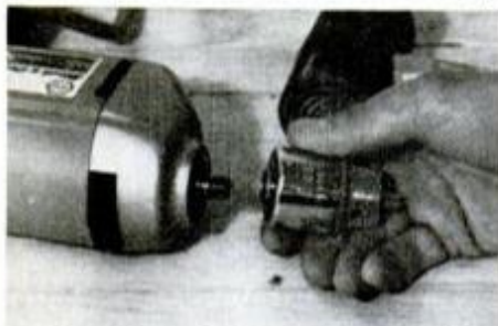
Depth of bore is determined and assured by locking wingnut. V-blocks mounted on Portalign's base make it a snap when you have to bore round stock accurately.
