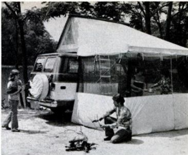
Vans and large station wagons can increase space without cutting top or sides with the Jutter, from J.C. Industries, Cherry Hill, N.J. A detachable 125-pound package mounts on the roof and opens into 4x8-foot sleeping loft and 8x8-foot room with roll-down sides.
