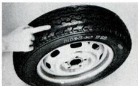
Deep, wide grooves in tread of Kléber V12 radial give water an easy escape route, minimize chance of hydroplaning.
