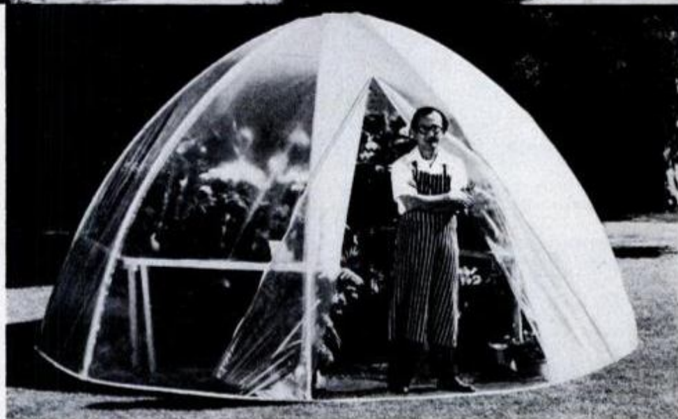
The portable Gro-dome by Botanical Environments requires no foundation. A pea-gravel floor cover is suggested. The dome has a PVC frame with polyethylene glazing. It can be assembled without tools. Cost of a 13-ft.-dia. dome like one above is $100.
