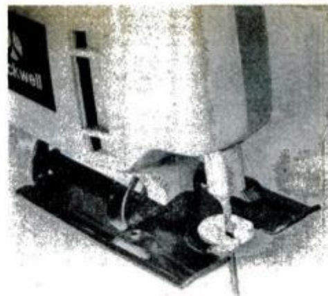
Base insert surrounds blade and reduces splintering of plywood veneer along cut.
