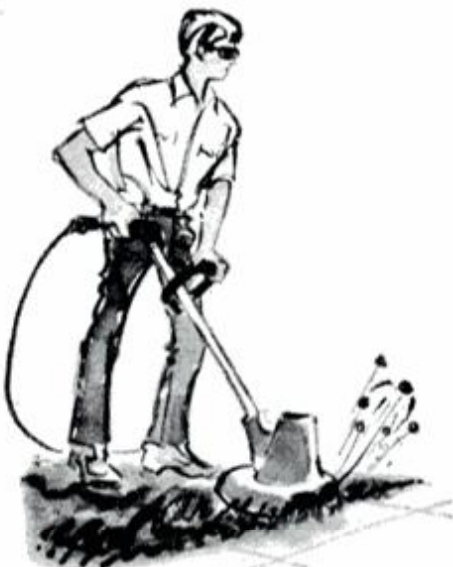
Power edgers kick up debris and throw it hard. Clear the area before you start.
