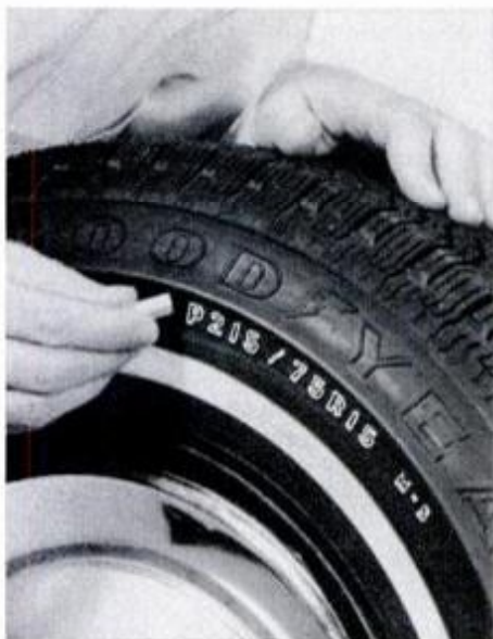
New metric marking on tire sidewalls shows section width in millimeters (215), but gives wheel diameter in inches (15).
