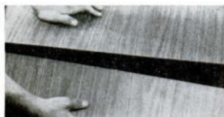
Cantilever piece over edge of bench and break off waste with downward snap.
