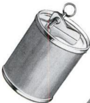
The "stun" grenade (left) has proved effective in immobilizing terrorists during an assault. A laminated paper cylinder with sheet-metal ends, it contains TNT flakes. After pin is pulled, grenade explodes in 4½ seconds.
