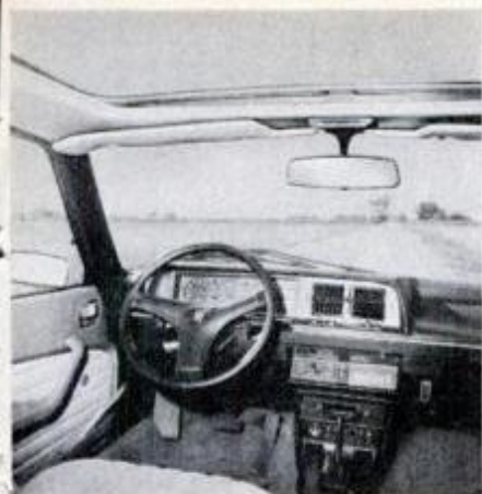
Instruments include tach. Some owners don't like right-side turn lever.
