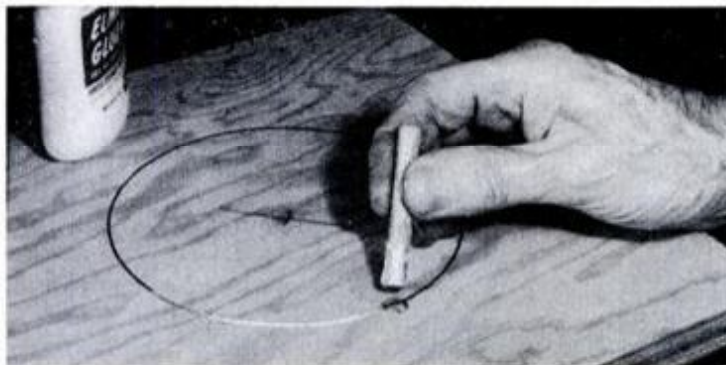
Insert the saw blade into the hole and cut until clear of it. Then plug hole with a length of 1/4-in. dowel and white glue.
