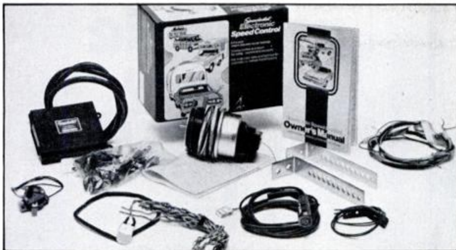
Parts of Speedostat Electronic Speed Control kit are laid out before work begins.
