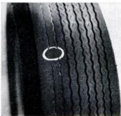
When tire tread is worn so wear indicator spans two adjacent ribs (painted circle), you must replace it. Life of this tire was shortened by running too long with wrong camber, causing the uneven wear.
