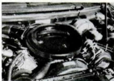
Twin-cam V6 delivers 88 bhp, has different valve timing right to left.
