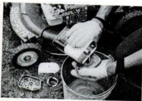
To get better performance from mower engines, wash clogged foam air cleaners.
