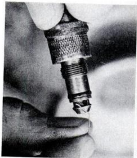
Use fine wire and kerosene to clean debris from the grooves in sprayer nozzle.
