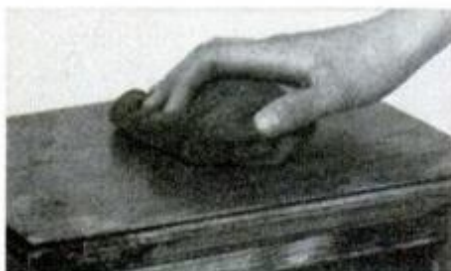
When dry, sealer is rubbed lightly with 00 steel wool to remove any roughness.
