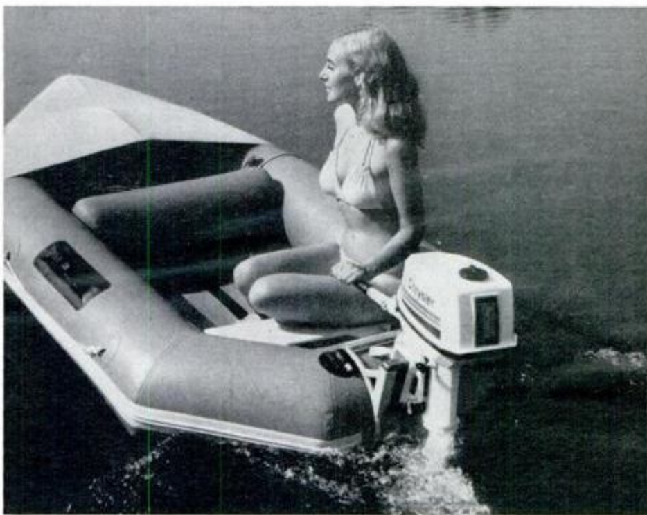
Trolling up to planing speeds is possible with a larger mini mounted on a flat-bottomed craft. Chrysler's Six (above) also comes in long-shaft sailboat models.
