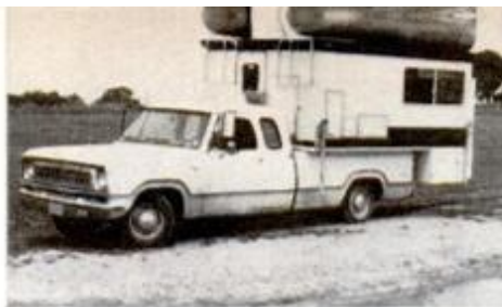
Ready for the road, the afloat-ashore RV only gives away its dual purpose with the four pontoons secured on camper roof.
