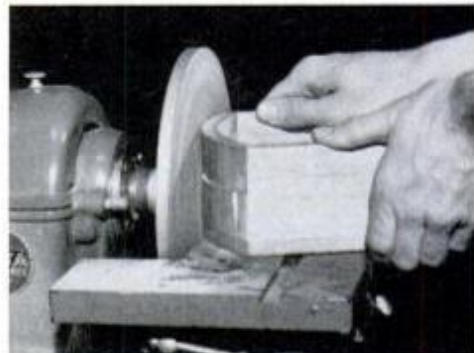
Next, use disc sander to remove saw marks, smooth curved cabinet front flush.
