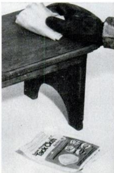
Final preparation step is to wipe all surfaces with a commercial tack cloth.
