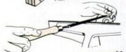
When sharpening a hand saw, make sure the file is level as the stroke is made.
