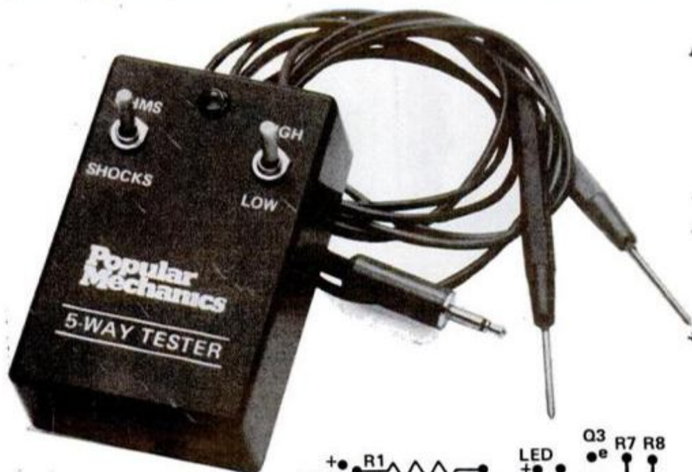
Setup to test appliances: one probe connected to ground, other touching conductive parts of plugged-in appliance. Handle with care until you're sure appliance is safe.
