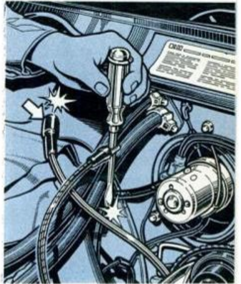
Improvised probe (see text) is best way to discover current leakage from cable.
