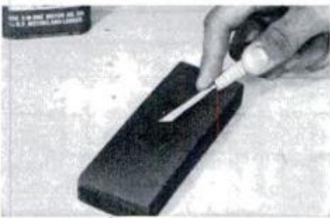
To finish cutting edges, hone on an oilstone. See notes on sharpening in text.
