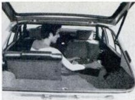
Split rear bench folds in halves so one passenger can ride beside cargo.
