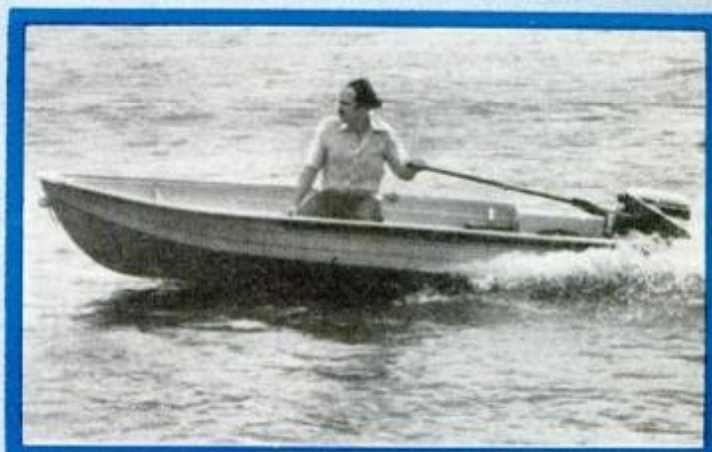
Gilco outboard handle extends 27 to 38 inches, lets driver sit forward. Fits Johnson, Evinrude, Mercury, Chrysler, Clinton, Eska, Suzuki, Honda, Mariner, most Volvo Penta twist-grip units.
