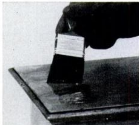
Then level the varnish with the brush by using strokes across the grain.
