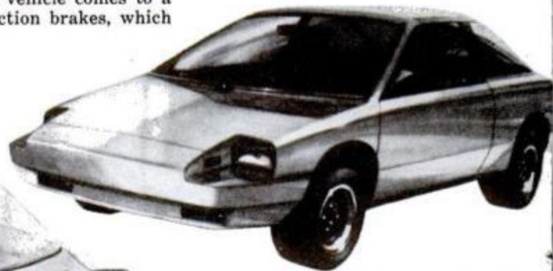
New four-passenger flywheel electric boasts sleek, spacious design and Garrett powerplant (top), with performance that's comparable to piston-engined family-size automobiles.
