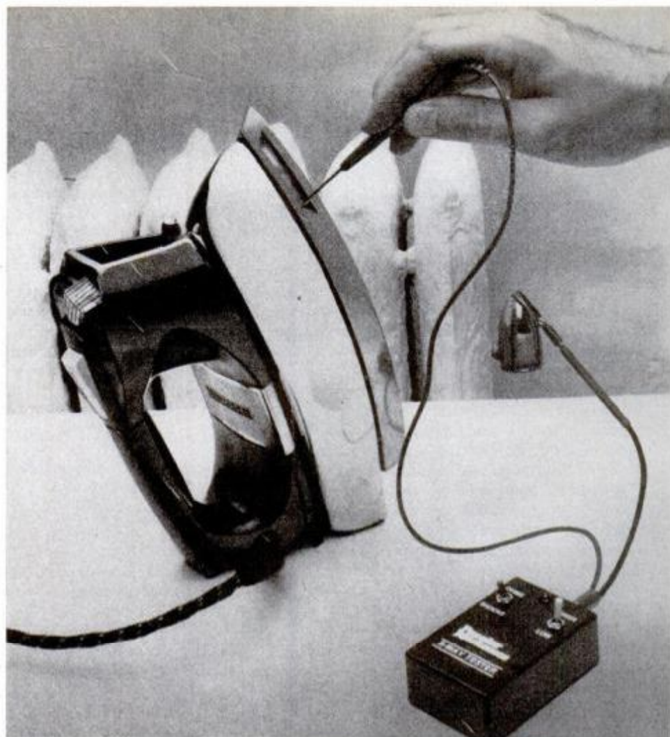
Setup to test appliances: one probe connected to ground, other touching conductive parts of plugged-in appliance. Handle with care until you're sure appliance is safe.
