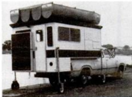
Firm level ground along shore is needed for quick-change from camper to houseboat. Wheels are lowered, body jacked.
