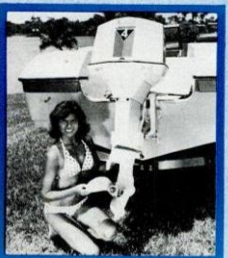
Metal flake finish styles the OMC Silver Streak SST propeller, called a bass boat bow-lifter that reportedly levels ride of 140-hp motors at speeds over 55 mph.
