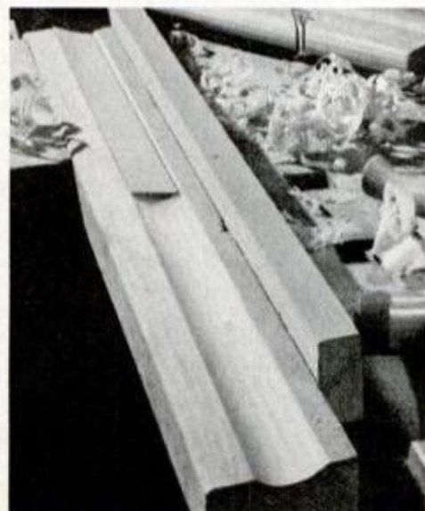
Caul, hollowed with rounding plane, will insure bond of veneer glued to molding.
