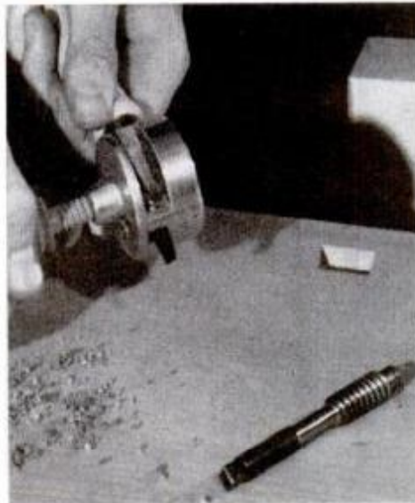
Wood screw on knob is threaded with woodcutting die, holds mirror at any angle.
