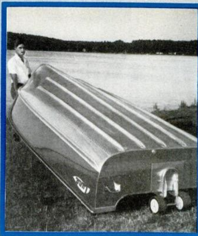
Clamping on a transom like an outboard motor, the Cosom Loner Boat, a 9-pound $33 accessory, allows one person to turn over and launch or haul out a light hull like a big wheelbarrow.
