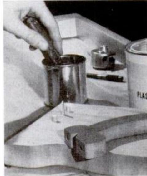
Uprights are glued, doweled and screwed to base. See text for alignment procedure.
