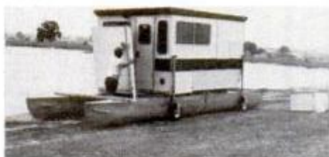
Cross-member braces are secured across four pontoons to hold them together and act as cabin foundation. Decks hinge.
