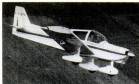
Tri-Z (above) makes it three in a row for Canadian kit-producer Chris Heintz. As name implies, it is three-place version of original two-place Zenith and single-seater Mono-Z (see text for source). At left are two Fikes in formation, the latest (foreground) a two-seater with 85-hp Continental and low-aspect-ratio wing said to prevent stall and spin. Cost: about $3500. Plans: $37.50, W. J. Fike, Box 683, Anchorage, Alaska.
