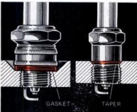
Gasket on plug at left should be seated tightly; tapered seat needs no gasket.
