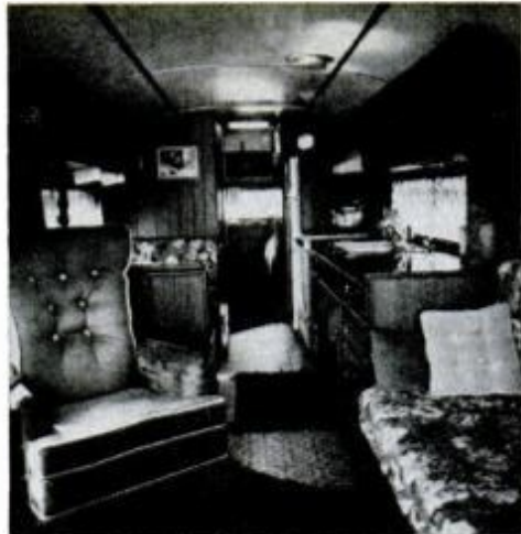
Most converted buses, like this GMC, put bedroom aft, galley and bath amidships.
