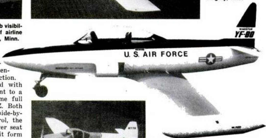
First military jet fighter to turn up among homebuilts is this half-scale Lockheed YF-80 (above), later to become famous USAF F-80 Shooting Star. Kits to come from Windstar. At left: Two-seater Emerald with 125-hp Lycoming and 1000-f.p.m. climb rate.
