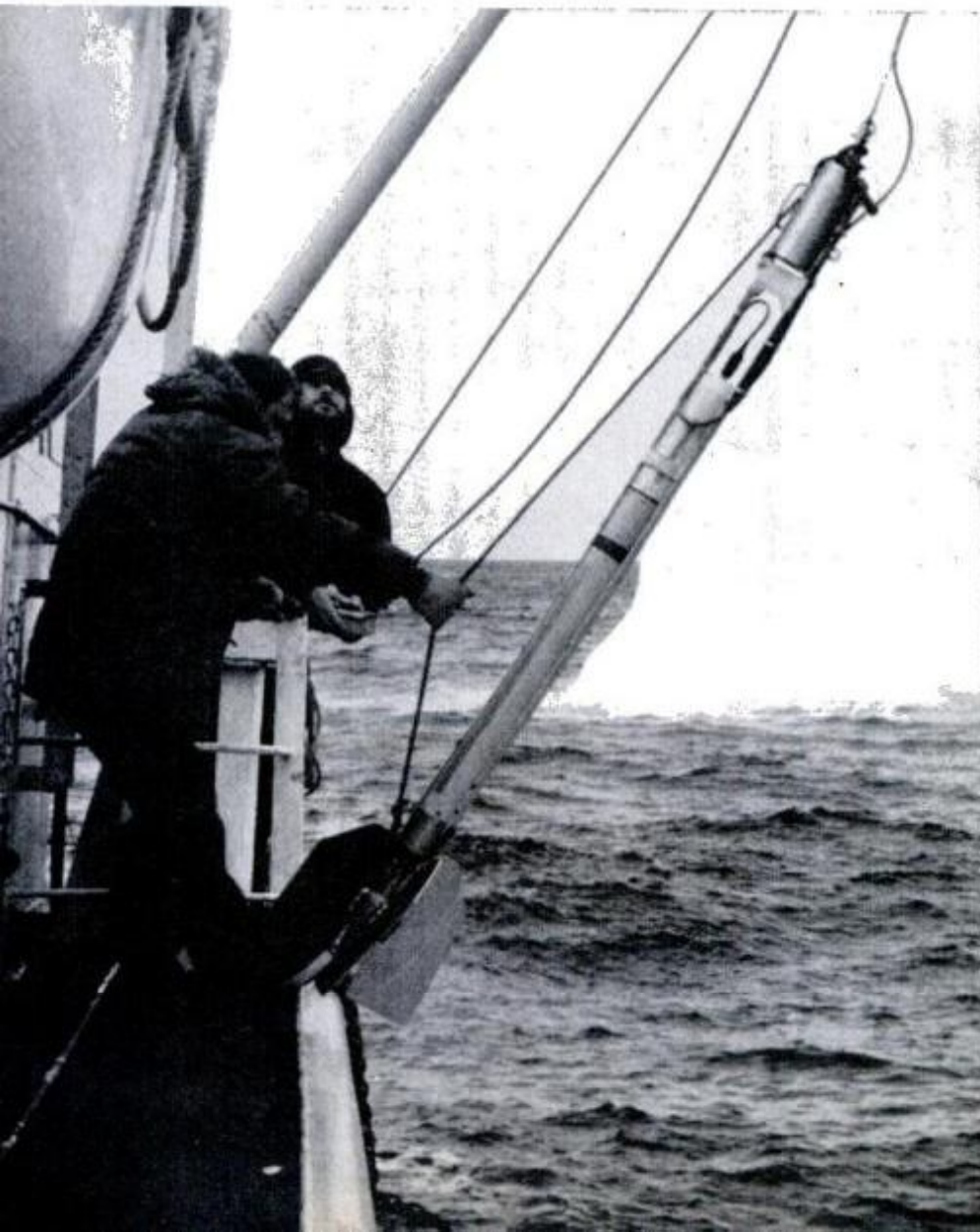
Torpedolike side-scanning sonar device is retrieved (left) after being used to determine draft of iceberg looming up dead ahead. Above, a crew change takes place between Orkney Shore and her supply ship by way of modern-style breeches buoy. Note rough seas. Below, mile-long tow hawser holds berg on massive winch.
