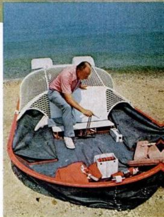
With controls back (top) and rear buckets aimed forward, hovercraft backs up rapidly. Removal of the front cowl (above) reveals battery box and controls.
