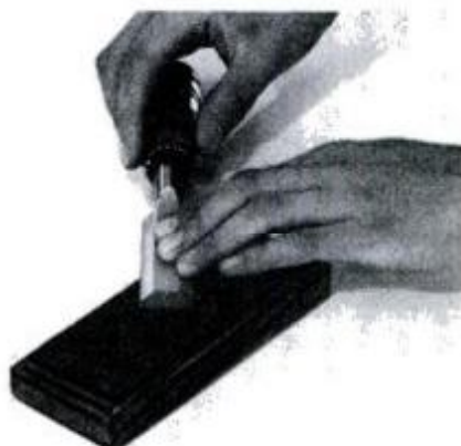
To chisel a dado, alternately work from both edges, start with bevel side down. Rotate chisel and use paring cuts to assure accurate depth throughout groove.
