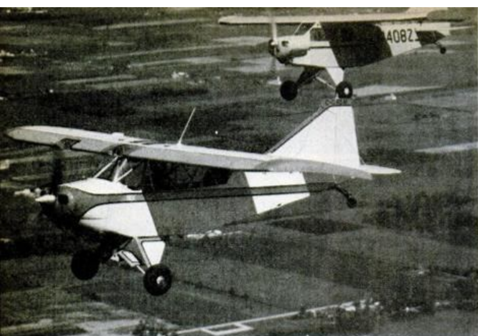
Tri-Z (above) makes it three in a row for Canadian kit-producer Chris Heintz. As name implies, it is three-place version of original two-place Zenith and single-seater Mono-Z (see text for source). At left are two Fikes in formation, the latest (foreground) a two-seater with 85-hp Continental and low-aspect-ratio wing said to prevent stall and spin. Cost: about $3500. Plans: $37.50, W. J. Fike, Box 683, Anchorage, Alaska.
