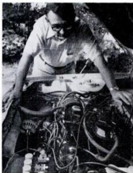
Ohc, 1.7-liter Four, VW-designed and supplied, is laid out transversely.
