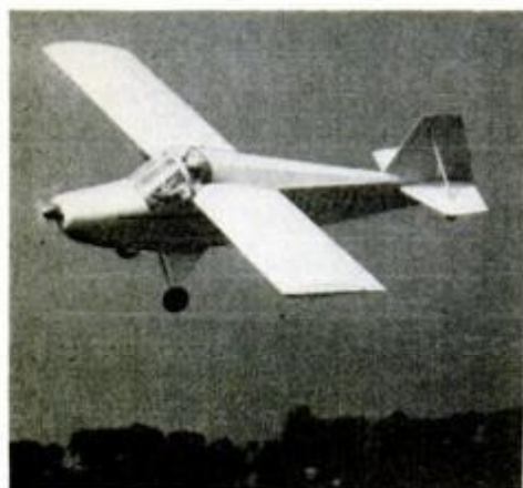
Shoulder-wing design gives superb visibility above and below, is work of airline captain Bert Sisler, Bloomington, Minn.
