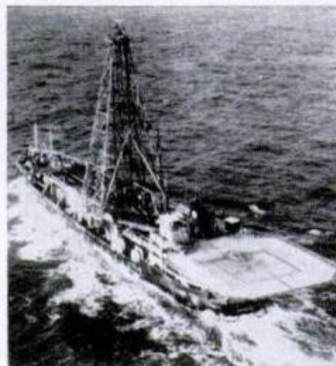
Oil-drilling ships are more often used in northern iceberg-infested waters than fixed platforms since they can be moved in an emergency. Tower amidships is a drill derrick. Note helicopter pad astern.
