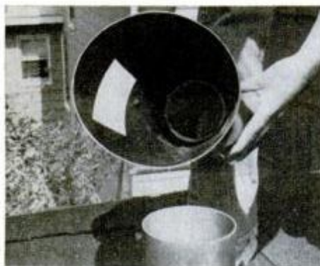
Inner ring enters stack for positive hold.
