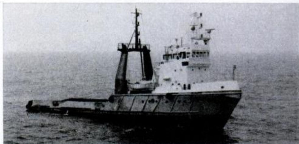
Typical tow-ship used in Newfoundland is M.V. (Motor Vessel) Orkney Shore. Note four-sided pilothouse for viewing in all directions. There are even dual controls
