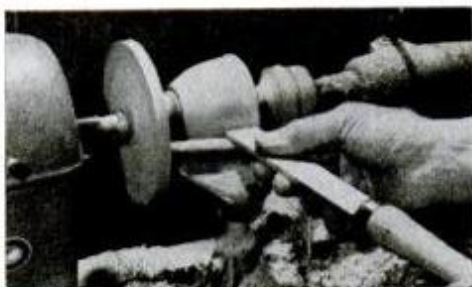
Use round-nose and skew chisels to finish concave and convex curves respectively.
