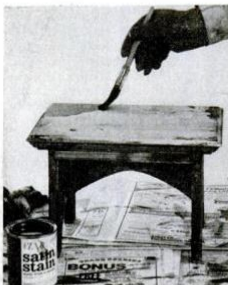
Working just one surface at a time, put on oil stain with bristle brush or rags.
