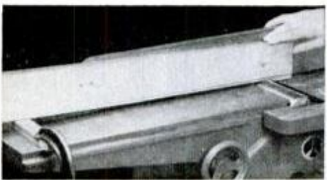
For short tapers, place taper start over knives; use a block to support front end.
