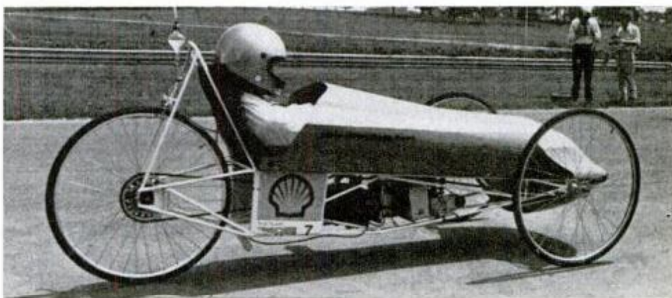
All contestants used three-wheel tricycle design permitted under rules, but could not agree on best arrangement. Most put single wheel in front (upper two photos) to simplify steering; a few went to dual front wheels (bottom photo) for better stability. Placing third, Finnish entry (top) employed unusual gas-steam hybrid drive giving 814 mpg. University of Wales tried hard with flashy drop-snoot affair (center), managing 564 mpg. Famed Hawker-Siddeley aircraft maker hit neat 699 mpg with sporty "roadster" (bottom).
