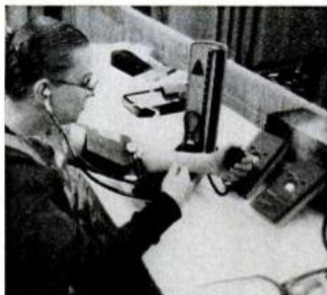
Sphygmomanometer (blood pressure tester) with electronic readout, also demonstrated at AMA convention, enabled visitors to try it out on themselves. Many did.
