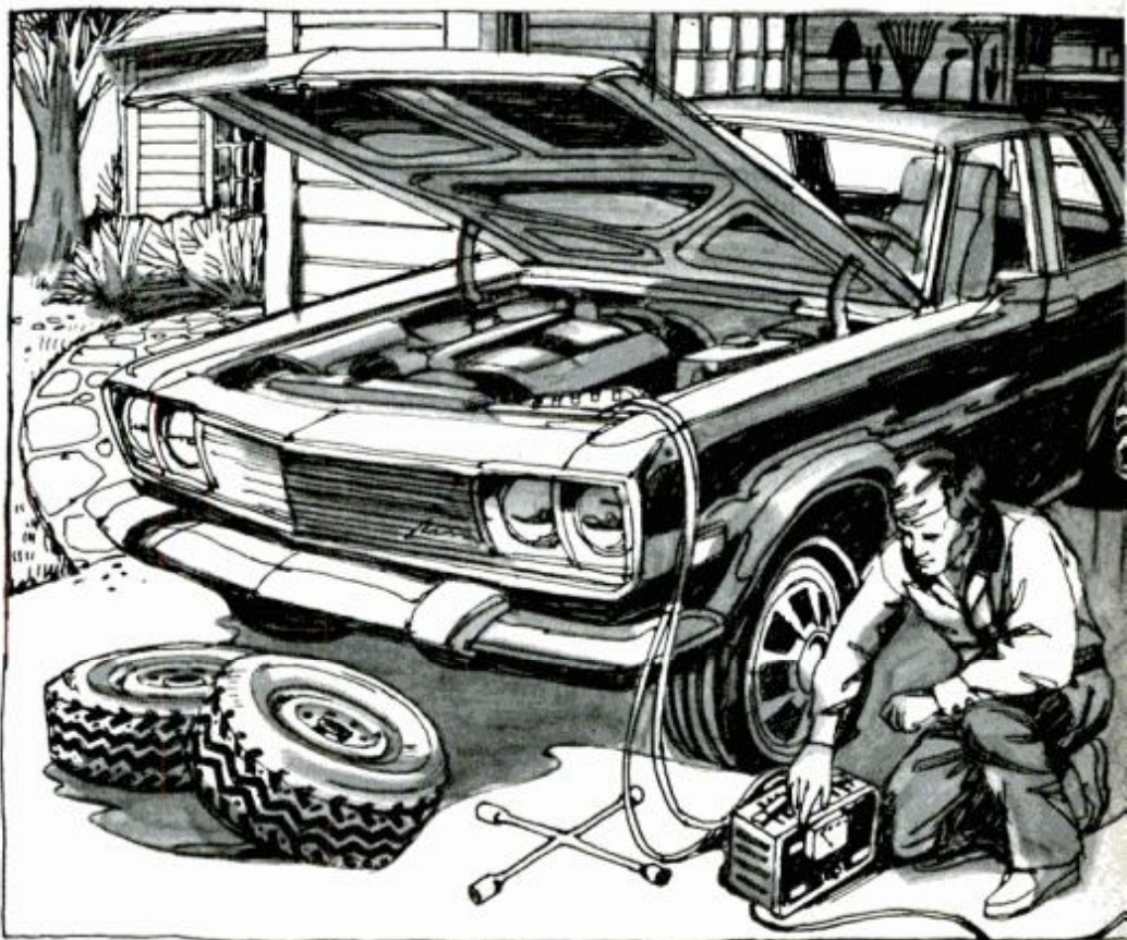
Use charger, if necessary, to bring your battery up to full charge for winter starting.
