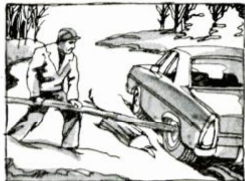
16. Stuck car can be levered up slightly using sapling with an appropriate fulcrum.
