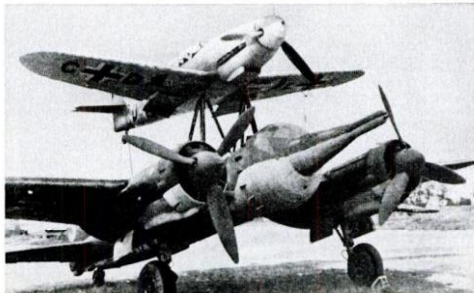
An unmanned Junkers 88 (bottom) helped up by a Messerschmitt 109, was a German composite. The JU88 actually was a four-ton bomb. The 109 unhooked at target and left.
