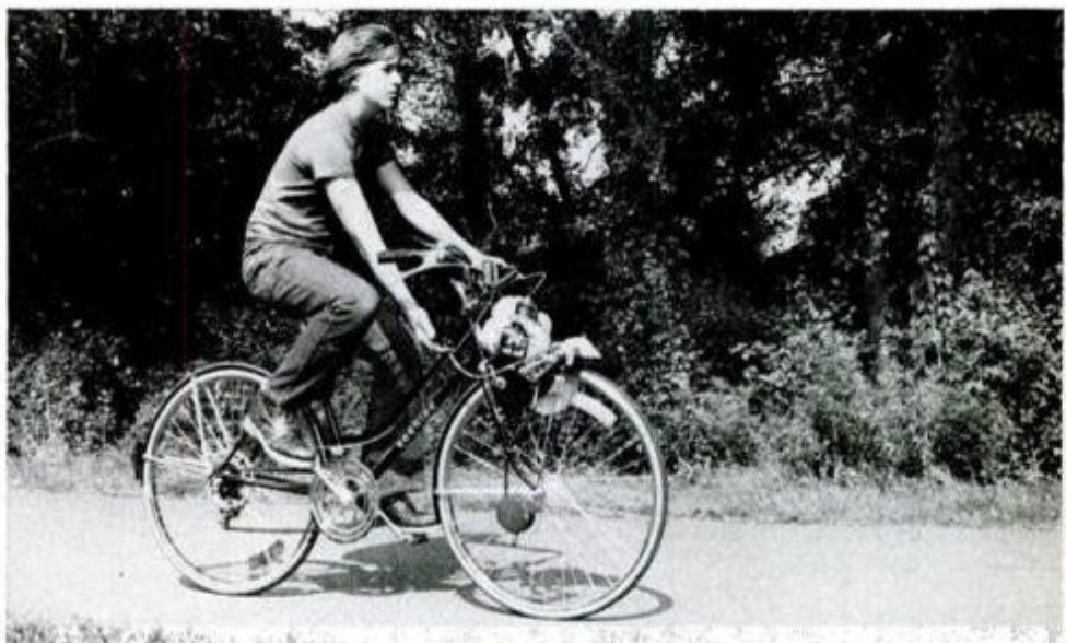
To start the BikeBug, lift the engagement lever which lowers the rubber drive roller against your front tire. Engine starts with throttle at idle; choke is automatic.
