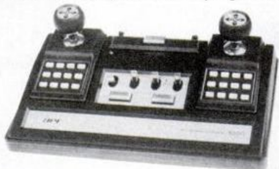
APF M1000's lift-out remote controllers have both joysticks for action and keypads for question-and-answer games.
