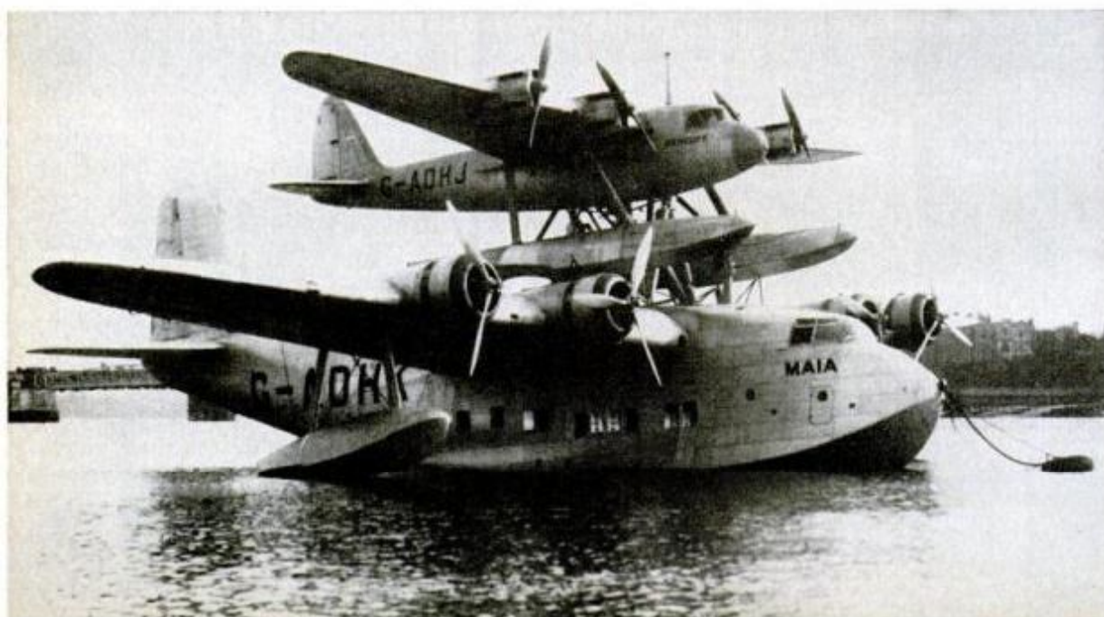
Britain's Short-Mayo composite used a "mother" flying boat, Maia , to carry smaller, heavily loaded seaplane Mercury , on takeoff and part way on trip to increase range of little plane on ocean flights.
