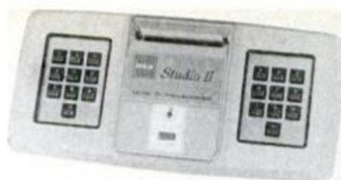
With RCA's Studio II control, keys mean directions of motion as well as numbers.
