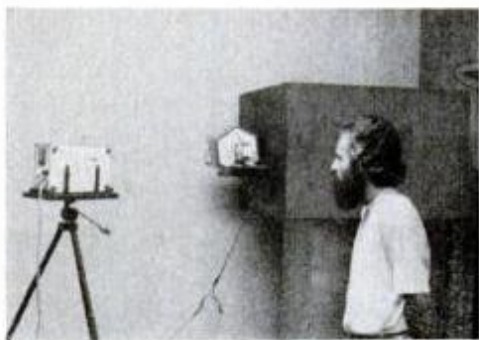
Co-inventor Rudy Manheim with display setup: low-power (2-mw.) laser at left, drum carrying six 70-mm holograms at center, box of optics at right. Viewing window is located at end of box opposite the drum.
