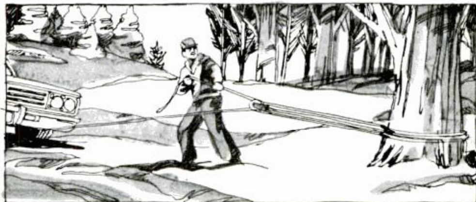
15. Block and tackle may move car just enough to give tires a fresh bite.
