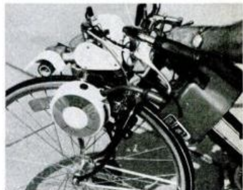
Fill fuel tank with liter of gas/oil mix (25:1) and then get ready to ride!
