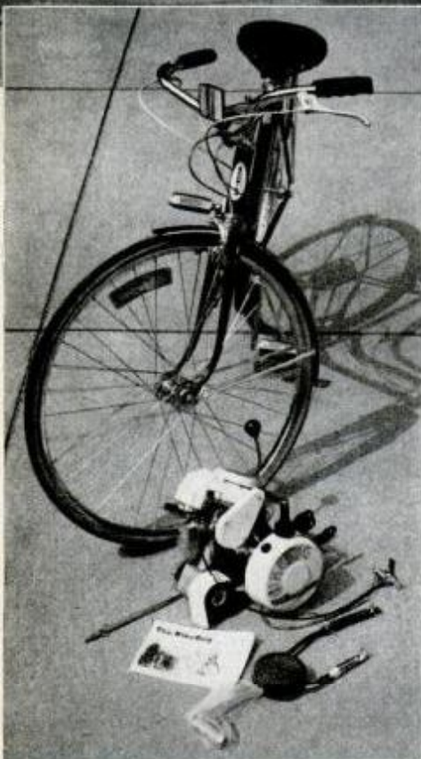
BikeBug engine from AquaBug International mounts on Schwinn Suburban 10-speed in a few steps (see facing page).
