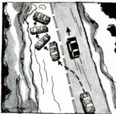
13. Passing spins occur when drivers move out from dry lane to icy passing lane.
