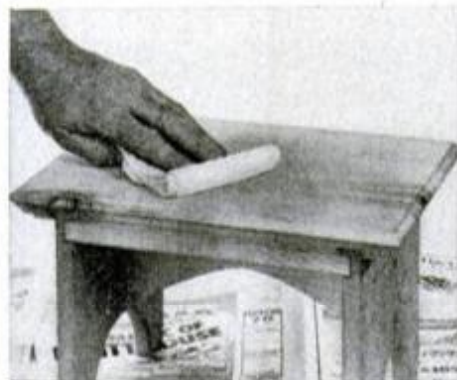
Tack cloth wiped across all surfaces picks up minute particles of dust.
