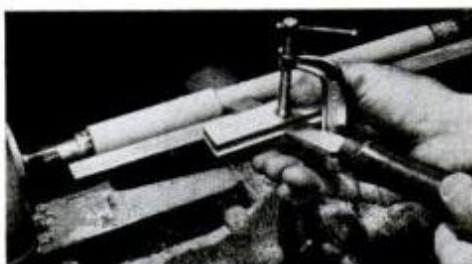
Jig helps turn a post accurately and parallel. Notched block holds skew chisel at proper angle; toolrest is fitted with 3/4 x 3/4-in. straight-edged aluminum angle.
