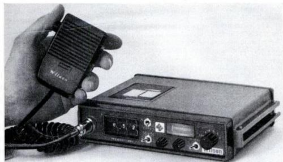
Front-panel switches help to select 800 channels on this new Wilson WE-800 model.
