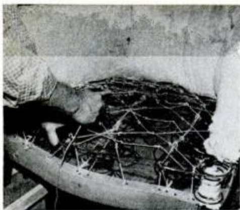
4 Cut weak twine and begin rebuilding of the chair by retying the springs.
