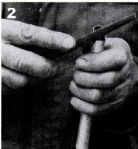
Then cut the extension length needed from the spare rod and file off burr.
