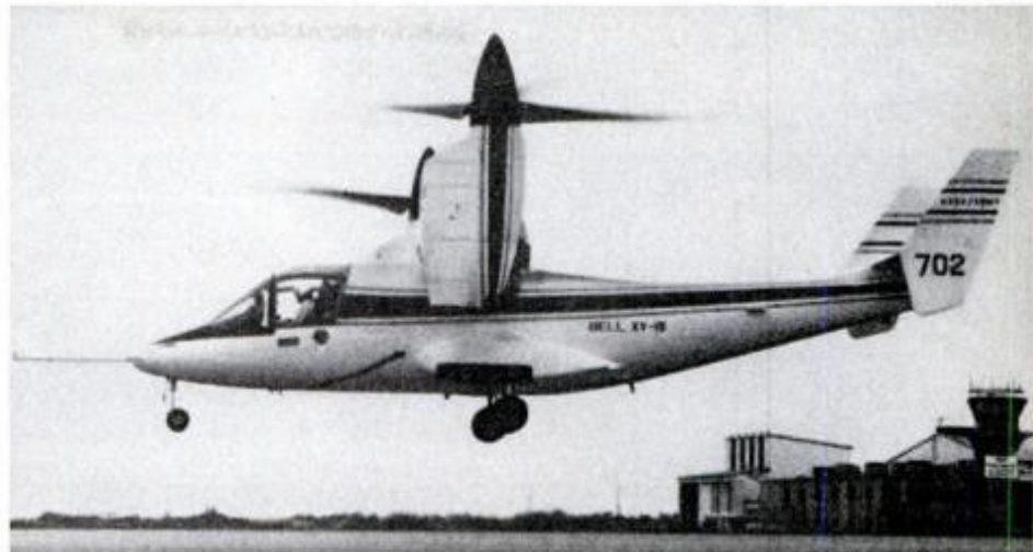
First hover flight for test aircraft. Tilttable engines pivot for horizontal flight.
