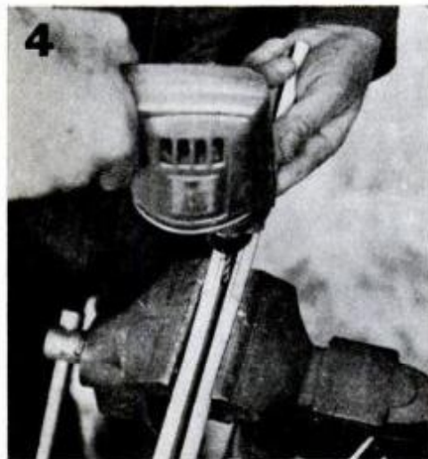
Drill through splice and rod and through splice and extension for fasteners.
