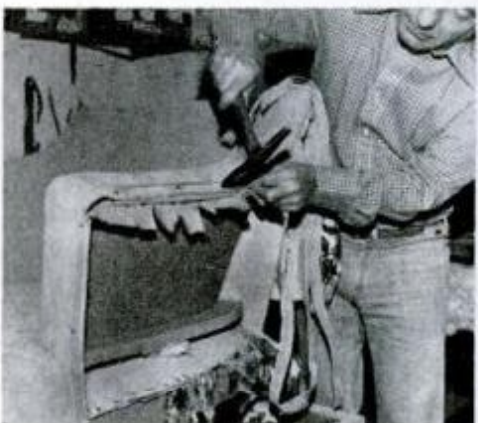
23 Following the chair contour tack welt-ing on the outside of the arm.
