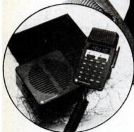
Microcomputer controls all operations in Texas Instruments single-sideband CB (left, above).
