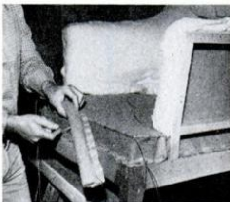
9 Fox edge sewed to the burlap is used to cushion and round the seat edge.
