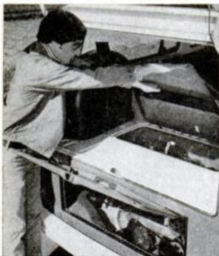
Despite doors top and rear, engine and battery aren't too accessible.
