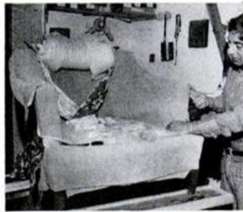
18 Fit fabric over the inside of arms. Note 6 in. of extra fabric at top.
