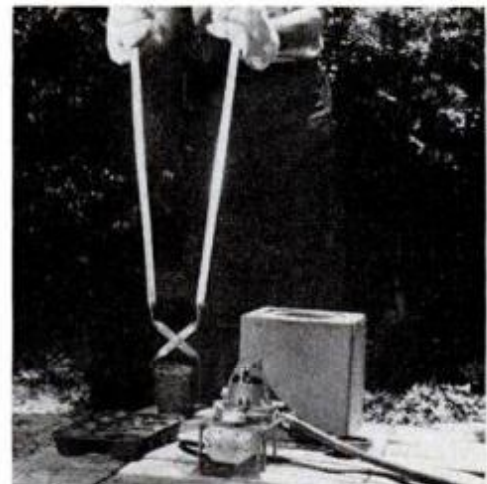
Use large tongs to remove crucible full of molten metal from the furnace.
