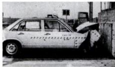
In 31-mph barrier crash, hood folds, and does not slice through the windshield.
