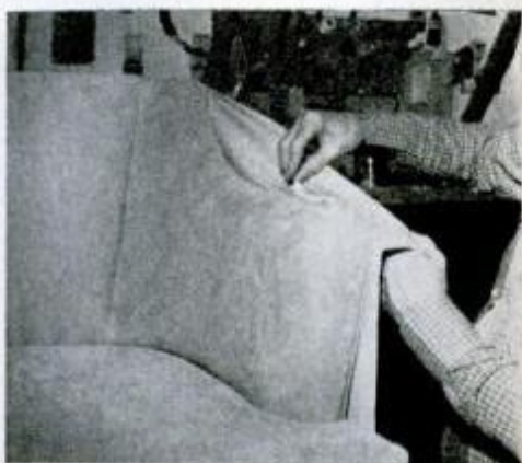
24 Position fabric for outside of arm. Chalk the contour inside the fabric.
