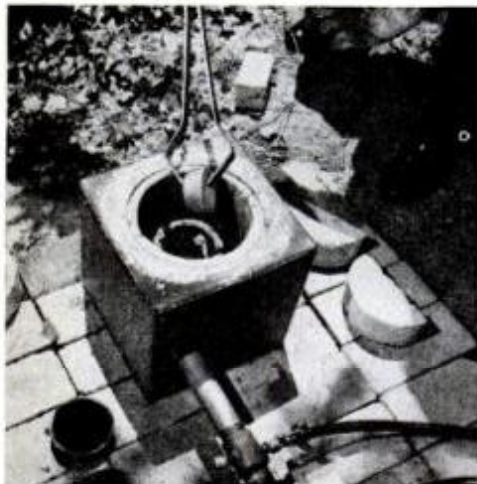
When the crucible is glowing brightly use tongs to put in an ingot of metal.
