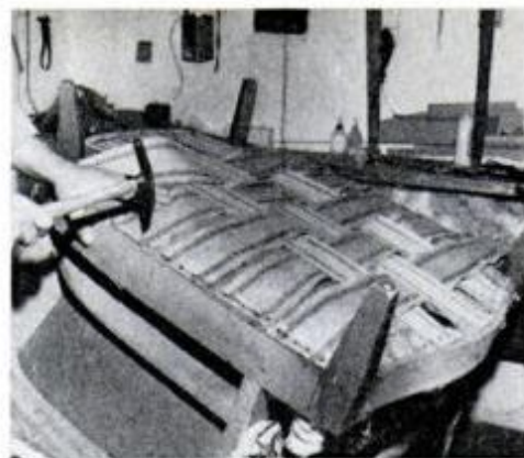
6 With a tack hammer and tacks attach webbing to the bottom of the frame.
