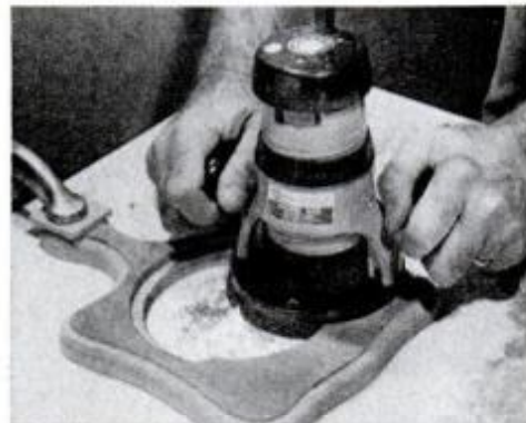
The rabbet where the dial rests is made with a router and a rabbeting bit.
