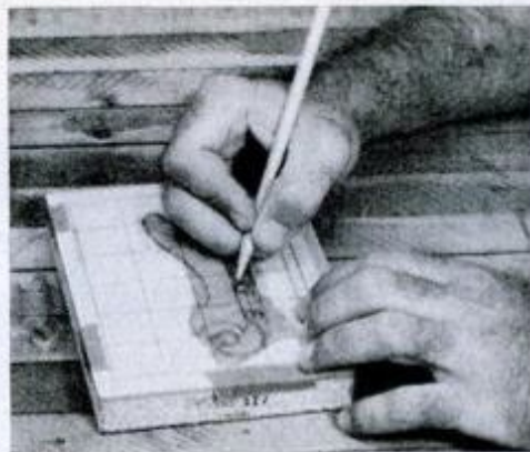
Tape the pattern on the block and go over the design lines with a hard pencil.
