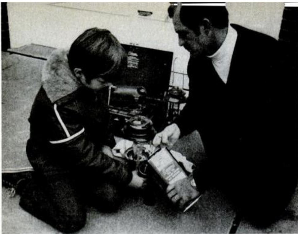
Outdoor equipment in all grades lends itself to blackout situations. Coleman's deluxe two-burner takes 11-inch pans. Two-mantle lamp (rear) has 220 candlepower.
