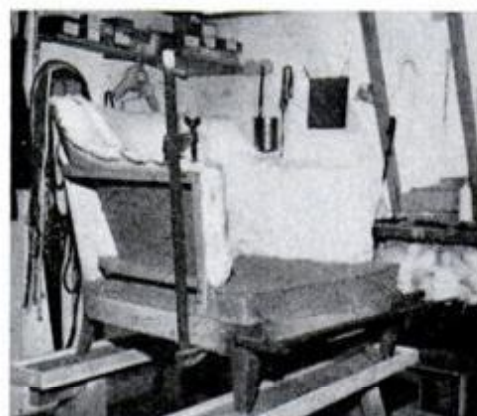
10 If the frame needs repair, glue and clamp it to insure a strong bond.
