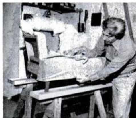
14 Smooth the new fabric over the chair seat and into the proper position.
