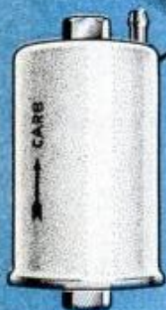
In-line fuel filter is shown above. It's in fuel pump-to-carb fuel line (right).
