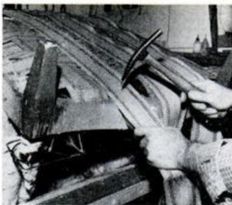
5 Weave jute webbing on chair bottom. Pull it taut with webbing stretcher.
