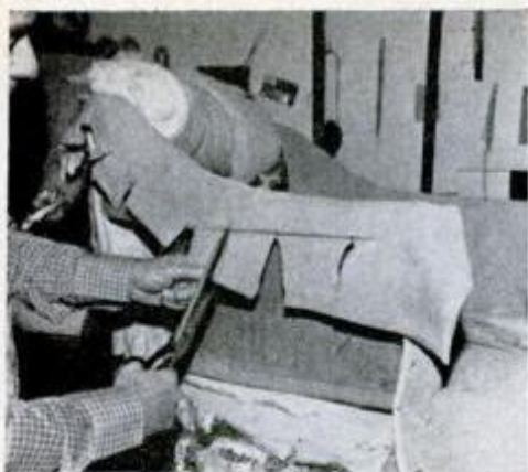
19 Cut the arm fabric up to the frame at stress points to avoid wrinkles.
