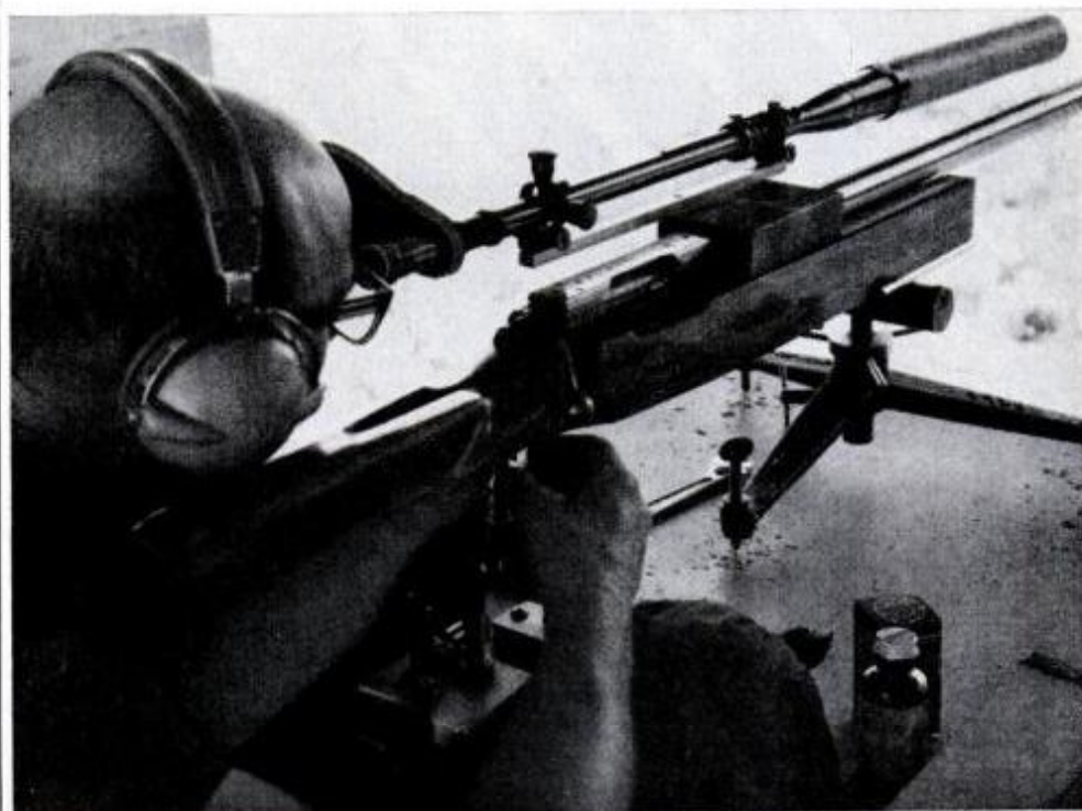
Massive bench-rest model can be held by sandbags, mechanical adjustable supports as shown, or elaborate return-to-battery mounts that return to aim-point after recoil.
