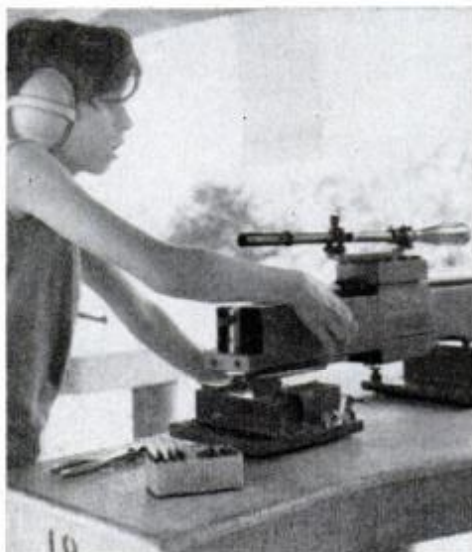
Heavy weight and small caliber of bench-rest rifle (above) dampen recoil and make unnecessary shooter's shoulder support.
