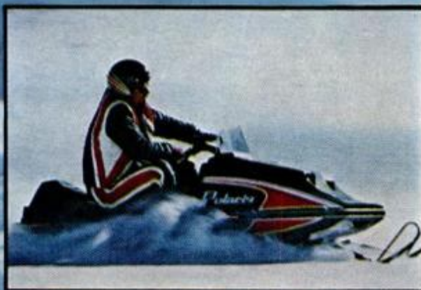
Liquid cooling is reported to give snowmobiles more even temperature control, better performance, quiet operation. Polaris TX-L 340, developed from racers and top of nine-model line, has it.
