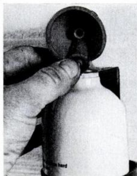
Charge is checked by pushing green button; it pops out (right) if still good.
