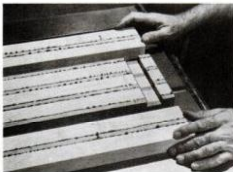
Three sections are glued up using hidden nail points to keep parts from slipping.
