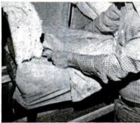
17 Position the seat fabric by the pull strips at the chair back.
