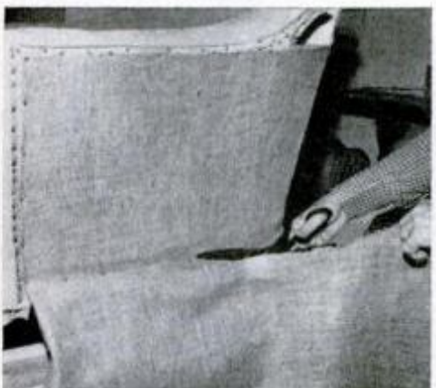
25 Tack cotton topped with burlap to the outside of arms and chair back.
