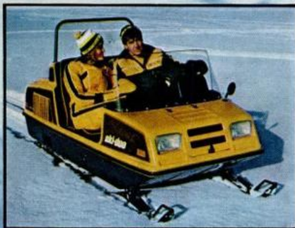
For side-by-side snow sport, Ski-Doo Elite has a different look, heated handlebars, reverse gear, liquid-cooled rear-mounted engine, twin tracks. (You can even order monograms.) Price: $3995.
