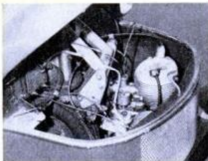
Single-cylinder engine that powers '47 Bond Minicar pivots with the front wheel.
