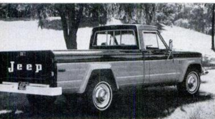
A straightforward workhorse with a capability for customizing, the Jeep J-20, like the Wagoneer, has a standard 360-c.i.d. V8 engine and choice of AMC's 401 V8 for its four-wheel drive.
