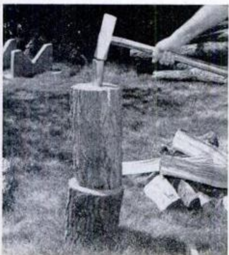
Use a splitting wedge and heavy sledge to halve large logs. Do wear eye goggles.
