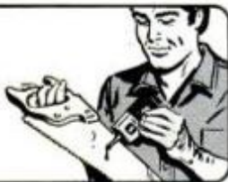
A one-piece plug-in version of the auto electrical system tester is made by taping or gluing the cigaret lighter plug onto the back of a smaller 0-1 milliamp. meter.
