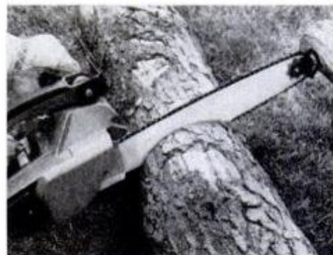
The antikickback device on this bar tip prevents accidents if object is touched.
