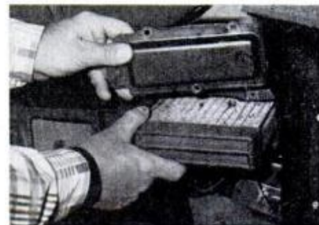
Heater core pulls out as if it were a drawer; it makes service simple.
