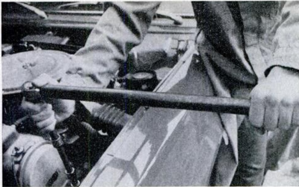
A "cheater pipe" is the best way to get additional leverage. It's important for the pipe to slide all the way over the handle to the ratchet as shown here.
