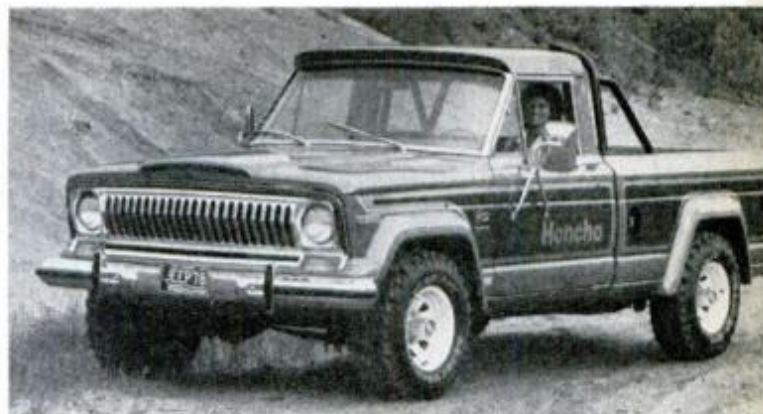
Jazzed-up Jeep version of the J-10 four-wheel drive, high-styled Honcho pickup features name on side, body stripes, cargo-bed roll bar, 258-c.i.d. standard engine or 360 V8 option.
