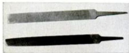
Taper file narrows toward its point (end); a blunt file tapers in thickness only.
