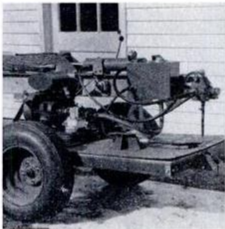
A two-wheel trailer makes a good bed for the splitter and lets you tow it as well.
