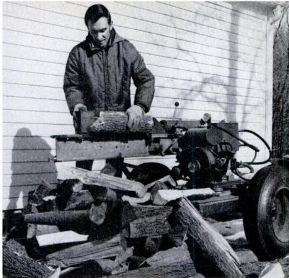
Move lever to split the log, remove the split halves and toss them on the pile.
