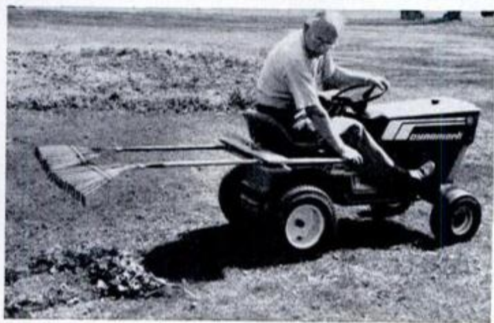
Homemade "power rake" speeds springtime cleanup of twigs and leaves. Handle clears fender of mower to permit dumping.
