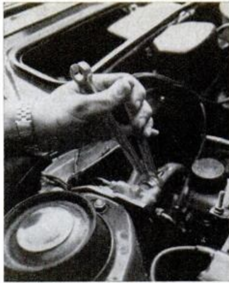
Tubing wrenches are used in pairs and are squeezed together to loosen nuts.
