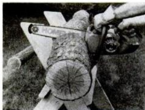
. . . then touch chain to log. Keep bumper in contact with the log as saw penetrates.
