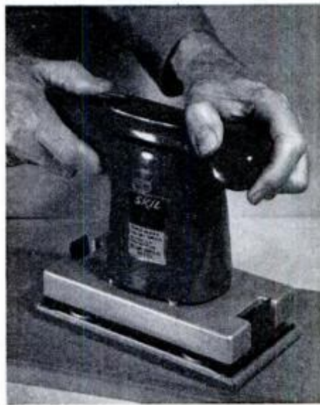
Sander utilizes strong spring clamps at both ends of pad to hold abrasive paper.
