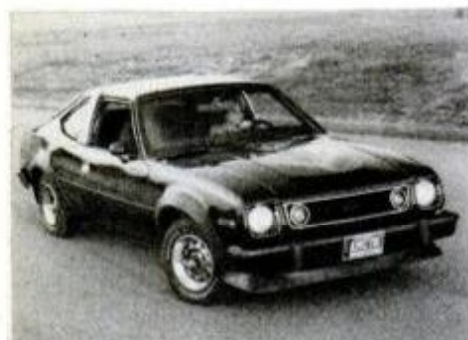
Racy AMX has four-speed manual transmission standard, new instrument panel.
