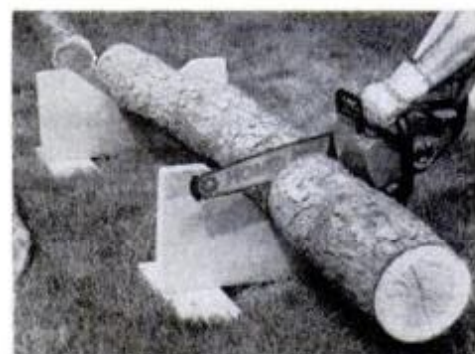
When using cradles, release the throttle as soon as the chain cuts through a log.
