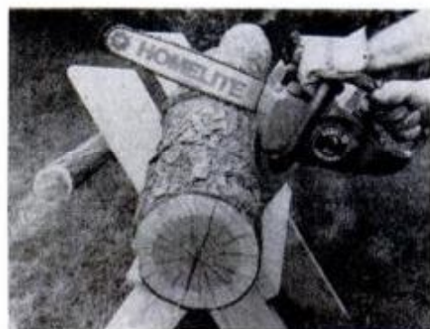
Start cut with saw bumper against log, bar tilted upward. Open throttle totally . . .
