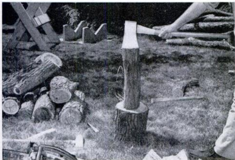
Split small logs with an ax. Keep your legs out of the line of swing.
