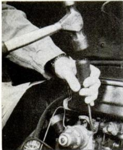
Tapping screwdriver while turning often will loosen tight slot-head screws.
