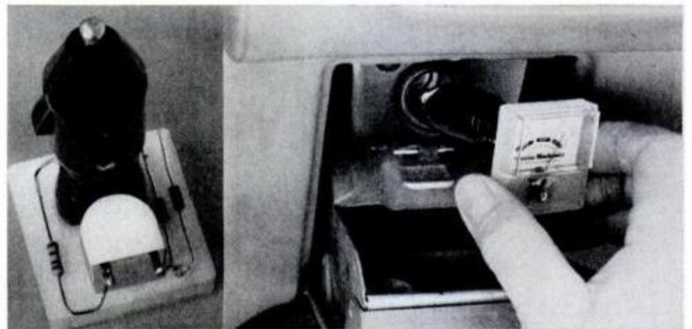
A one-piece plug-in version of the auto electrical system tester is made by taping or gluing the cigaret lighter plug onto the back of a smaller 0-1 milliamp. meter.
