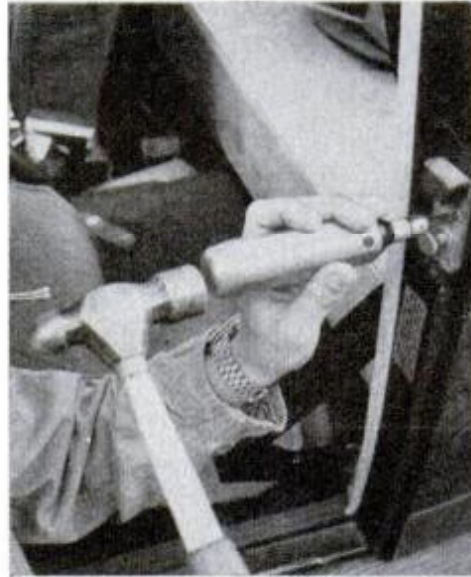
Impact driver will work when twisting and tapping won't loosen tight screws.
