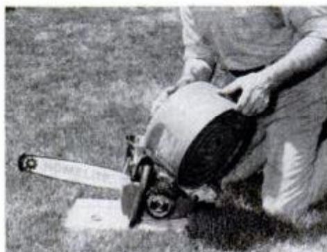
Fuel your chain saw at a distance from the work area so spills won't be a danger.
