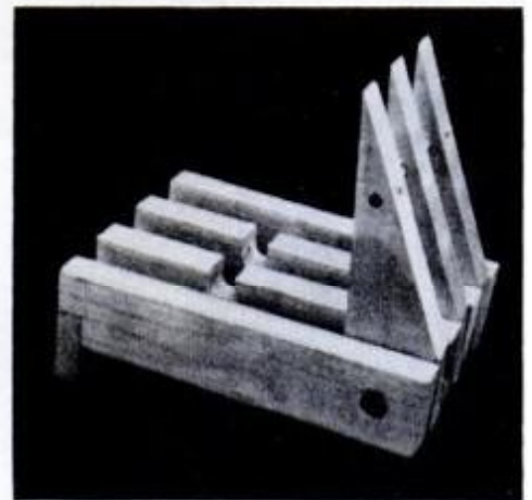
Time for an oil change? Ramps make it easier to slide under your car and work. They fold for easy, compact storage.
