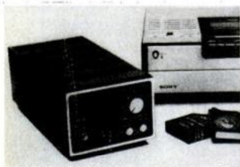
Sony PCM (pulse code modulation) peps up sound in Betamax video recordings.
