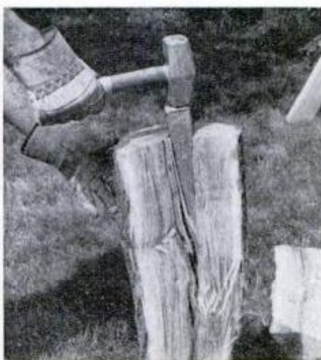
One-hand sledge (maul) is easier to use when splitting the log in quarters.
