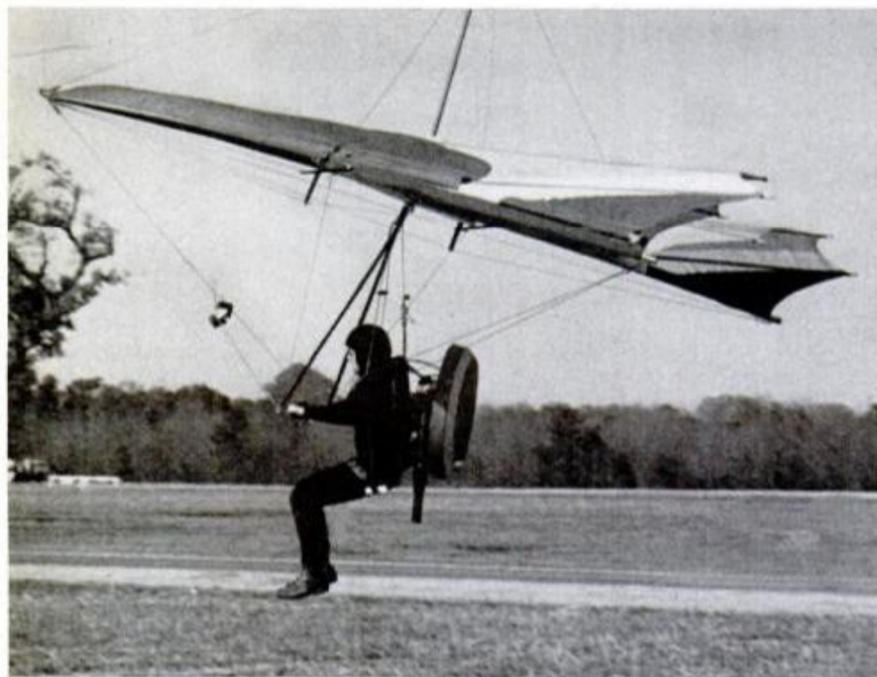
Flying wing, called 49er, is handiwork of Craig Catto of Cupertino, Calif. Unlike Jensen design on preceding page, it has no tail. Engine has hand throttle plus kill switch to cut power.
