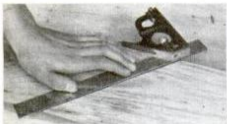
Versatile combination square performs many functions, including this more familiar one—the marking of a miter cut.
