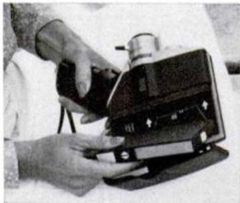
Polavision Instant Movies film cassette slides into back of battery-run camera.
