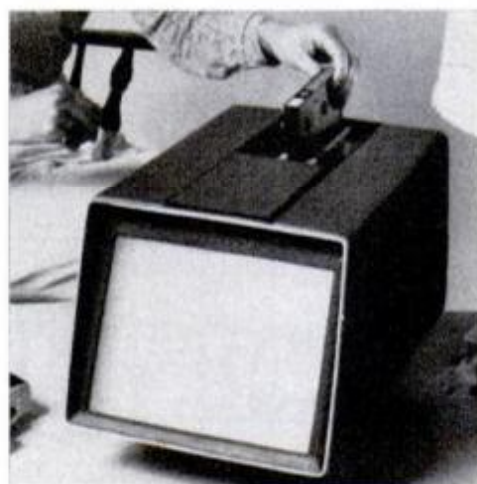
Instant film is never removed from its box. After exposure in the camera, the cassette drops into projector for rewind, developing and playback in 90 seconds.
