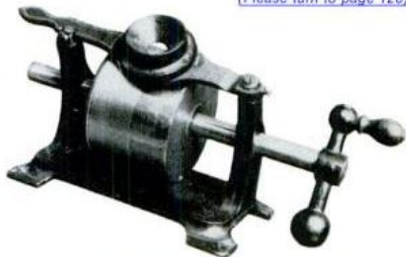
Edison's first phonograph of 1877 still lacked the sound-amplifying horn. On this machine he recorded Mary's Little Lamb .
