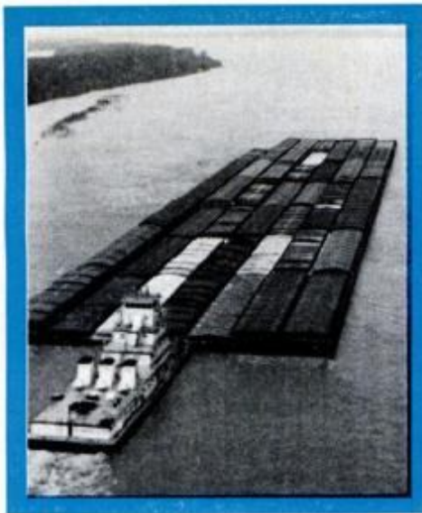
A 48-barge tow plowing upstream is a rig that the riverboats must reckon with.
