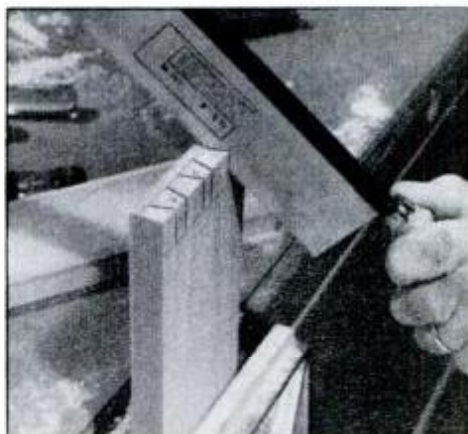
For half-blind doves, cut tails; then saw pins at upward angle as far as possible.
