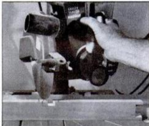
Set the saw arm at the required angle; then make passes with an elevated blade.
