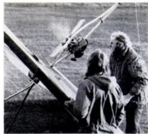
Twin-tube kingpost mount was devised by Terry Sweeney to allow adding engines to flex-wing Rogallo-type hang gliders.
