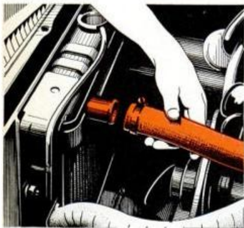
Radiator upper hose delivers hot coolant from the engine to the radiator.
