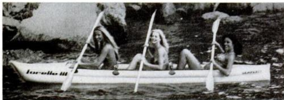
Inflatable canoe for two or three paddlers, the Forelle III by Semperit-Leisure America, Fort Lauderdale, Fla., is a 33-pound 13-footer for touring, cruising.
