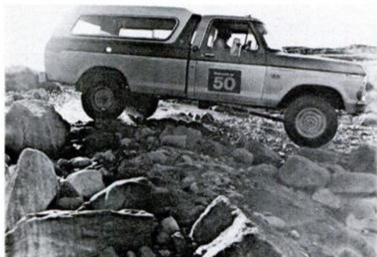
Shocks on the rocks. In rugged Alaska, the toll on shocks can be brutal. Sudden twists can misalign their spindles permanently.
