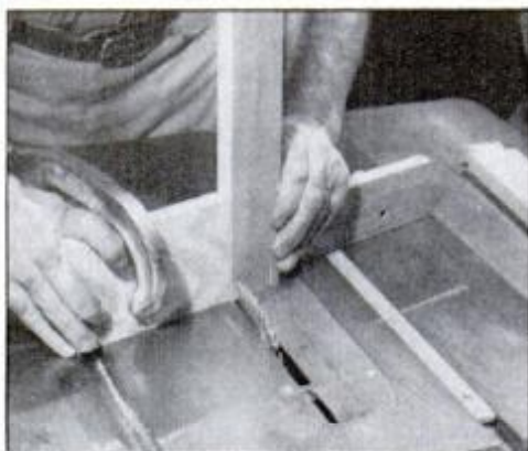
With a high stop block, set miter gauge at right then left angles for first pin cuts.
