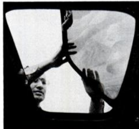
Flip-up sunroof option tilts up at rear edge or it can be removed completely.
