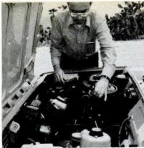
Easy service features include translucent reservoirs to quick check fluid levels.
