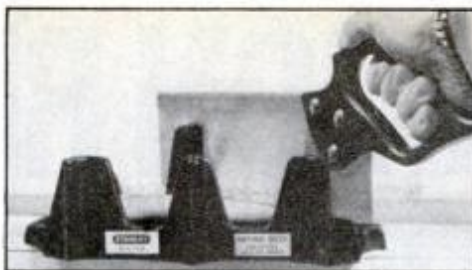
Inexpensive plastic miterbox gives 45° and 90° cuts with reasonable accuracy. For rigidity and best results, holes are provided for fastening box to workbench.
