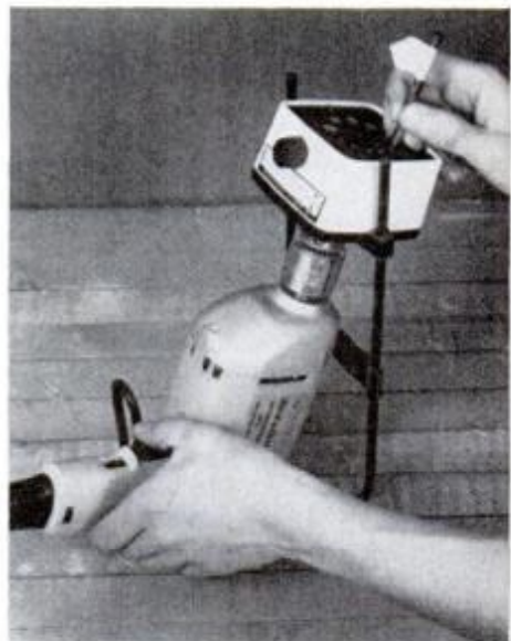
Tape flag indicated bit position: It's rotated 180° to sharpen second edge.
