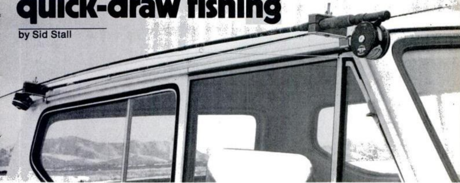
Clamping blocks attached to rain gutter hold set-up rods securely but allow quick removal for instant fishing action.
