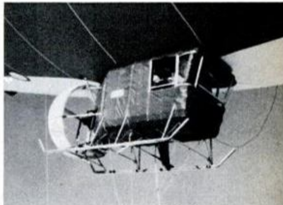
Delta-shaped "flying wing" at top is one-man prototype of much larger Dynairship shown on following page. Ship has actually flown, indicating combination of gas and wing lift could work. At left is Raven's two-man, 120-foot hot-air "sport" craft powered by 65-hp VW engine with steerable prop mounted behind gondola (above).
