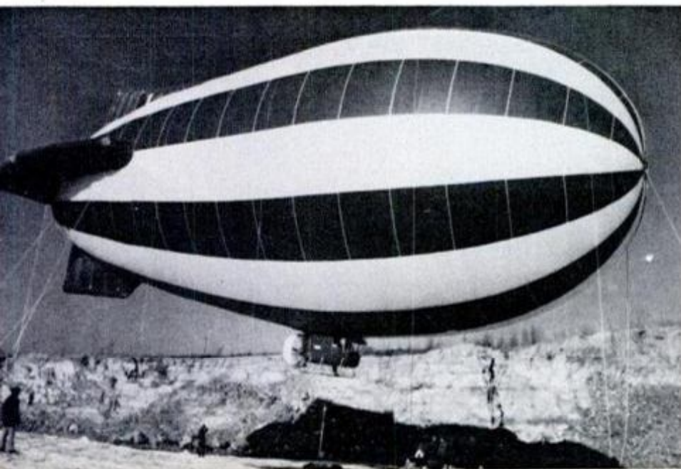
Whimsically painted Cameron D-96 above, a British import, is a hot-air balloon also prop-powered like the Albatross at left and Raven below. The big scoop hanging down behind the gondola directs ram air into the bag to help maintain nonrigid envelope shape. Craft accommodates two, is 95 feet long, has a speed of about 11 mph. You can pick one up, delivered in the United States, for $39,500—less tax and dealer prep.
