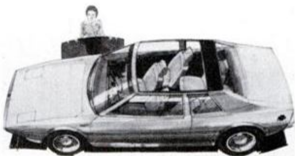
Staggered seating arrangement of the Triplex design is shown at left. Each passenger gets full legroom with this layout. View above shows large glass area and removable Targa-style roof of bronze glass.
