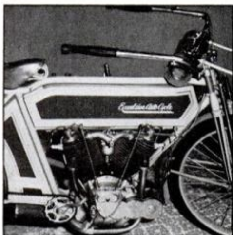
Good as new: The 1921 Norton (top left) belongs to Al Signman; the 1931 Henderson in-line Four (above left) is Leon Blackman's; the 1914 Pierce Arrow (top right) has a one-cylinder, four-cycle engine—with no gas tank, it stored fuel in hollow frame; 1912 Excelsior Auto Cycle (above right) is two-cylinder, four cycle, pedal-start.
