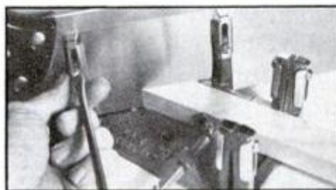
Depth stops on a combination miterbox and clamp move up to contact the back-saw rib. Capacity of the $24 unit ranges up to 2 in. wide and 1 3/4-in. deep.
