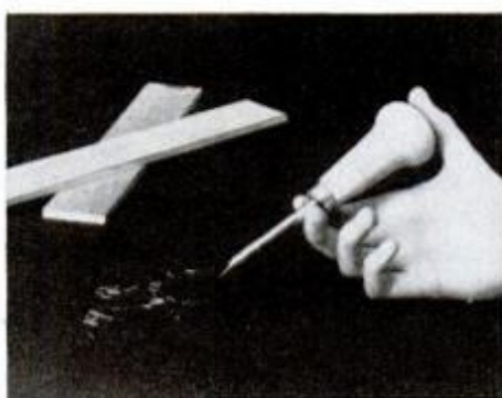
Comfortable-to-hold pusher has magnetized tip for easy pickup of small brads.
