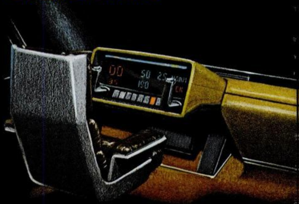
Command console for driver seats him behind a picture-window windshield and facing a control panel where digital readouts display miles an hour, distance remaining to campsite, miles per gallon, time and distance run, estimated time of arrival, engine temperatures and pressures on demand, gas tank levels and programmed route numbers. Pushbuttons adjust climate control, lights. Control handles can replace steering wheel.
