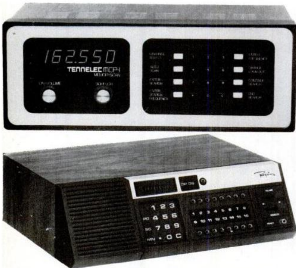
The Touch, a new-signal-searching VHF-UHF scanning monitor by Regency (above), silently listens to 15,357 radio channels. It will alert you automatically if the National Weather Service sends a severe weather warning. Tennelec MCP-1 (top) also searches out uncharted signals, plays them for you, stores them in memory, recalls on command. These new digital synthesized receivers need no code book or crystals.
