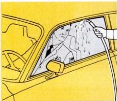
Water leaks can be tough to find; best way is to use a garden hose to soak the car.
