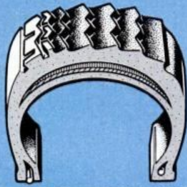
FEATHERING DUE TO MISALIGNMENT OR SEVERE CORNERING
