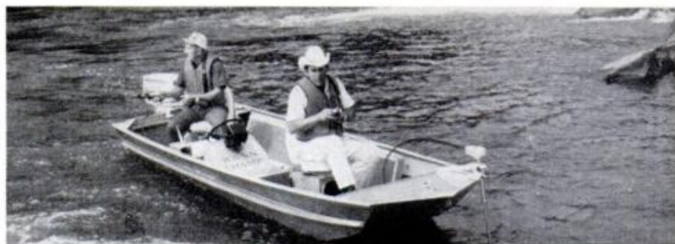
B.A.S.S. Champ afloat shows aluminum hull with modified-V design that allows soft, safe but fast ride with only 35 outboard horsepower pushing the light rig to 35 mph.
