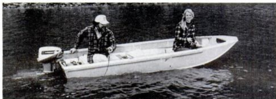
Newest from Grumman, the 3.8 (meter) model meets the latest level flotation requirements and takes a 10-hp motor. The aluminum hull has V-form with strakes.
