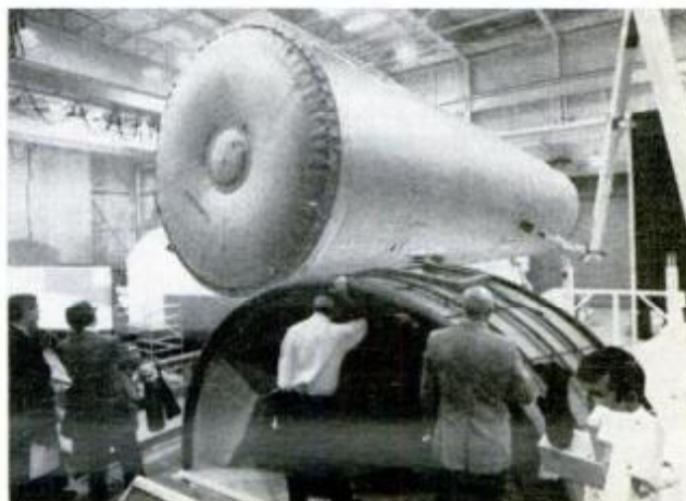
Inside Building 9-A at Houston, scientists use a 60-foot inflatable bag (below) to simulate a payload in order to check operation of a prototype manipulator that will be mounted on Shuttle.
