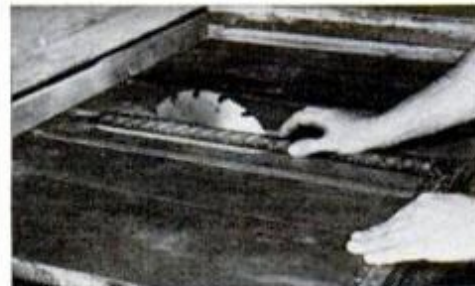
Check blade trueness with framing square; turn blade by hand with saw unplugged.
