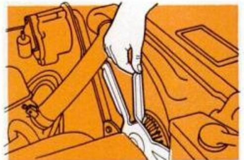
Newer cars use fans with clutches; test to make sure clutch is working properly.
