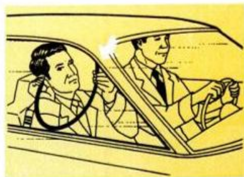
Wind noise, too, can be hard to pinpoint; use section of hose as an aid in the job.
