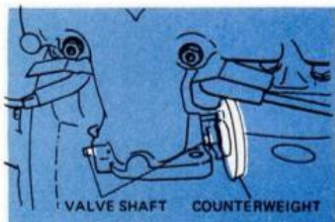
Manifold heat-control valve is lubricated at valve shaft points shown here.
