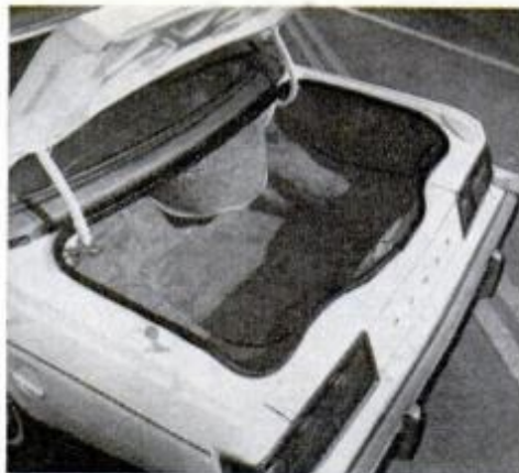
Trunk space with space-saver tire is 16.3 cu. ft. for the coupes and 16.6 cu. ft. for the four-door sedans.
