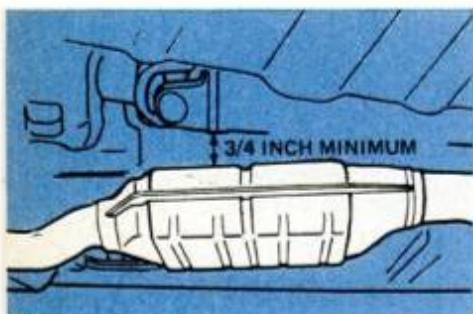
Catalytic converters get hotter than mufflers: position to spec.
