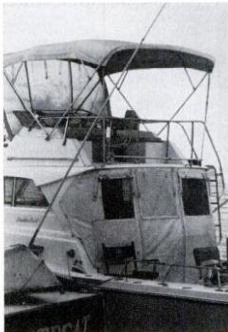
Bimini Top over the flying bridge and a plastic windshield give sun and spray protection; canvas below encloses cabin.
