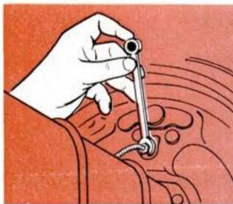
Hydraulic-brake-fluid leak may be fixed by tightening brake line.
