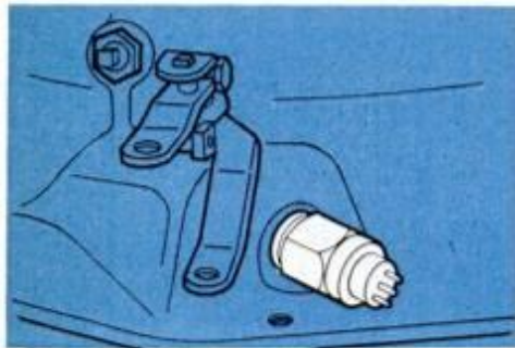
Neutral start switch prevents starting when automatic transmission is in gear.
