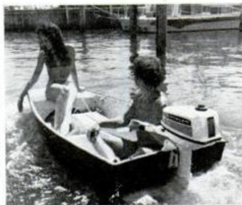
Larger inflatables have transom mounts that can carry an Evinrude 2-hp mill.
