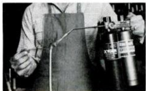
BernzOmatic torch brazes a copper pipe and fittings. Cost is about $40.
