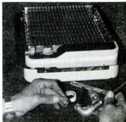
Quick-disconnect fittings make permanent gas line (and chance flexing) unneeded.
