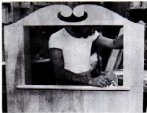
The stage (above) is planed smooth. A notch is sawed into the ledge (below) for the hinge attaching the side panels.
