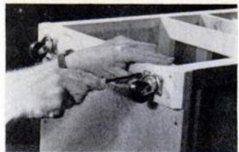
Screw-on casters make your worktable mobile. They're held on firmly by being mounted into 3/4-in. stock. Use long screws and glue to anchor the stock.
