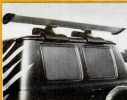
Even awnings are being styled up by Carefree of Colorado. Firm's Indy Spoiler Awning mounts on the back of a van as an air foil and scoop but opens to offer camping shade.
