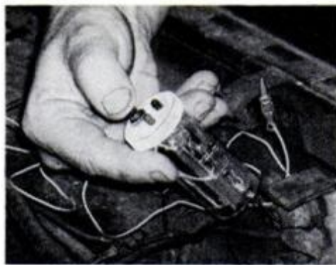
Is that wire hot? Ground? Nowhere? Press the button, and an LED will tell you.
