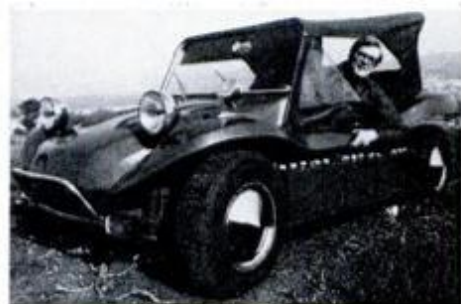
Paul Howes's homebuilt costs 4 to 5 cents a mile to operate—1 for electricity, 3 to 4 for batteries.
