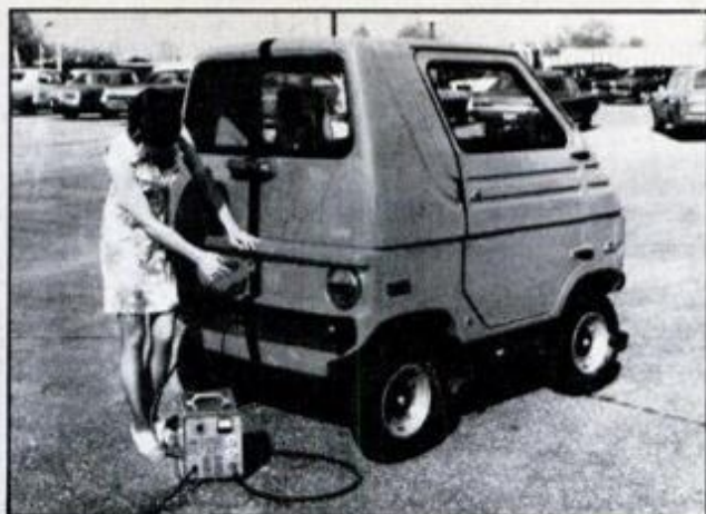
Elcar 2000 is a two-passenger electric car from the Elcar Corp. in Elkhart, Ind. The power pack is a bank of eight batteries that slide out on a tray which is suspended under the chassis. Car is plugged in for recharge as shown above.
