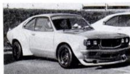
RX-3 coupe racing version spins out over 250 hp with 9500-rpm redline.
