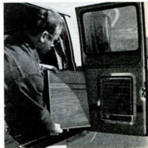
Installed heater, inset away from latches, can have panel covering when not in use.
