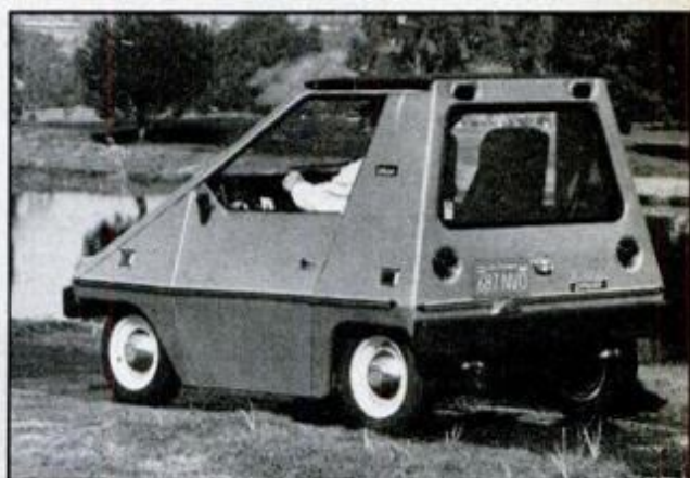
Citicar is a wedge-shaped, two-seater electric from Sebring-Vanguard in Florida. Shown here is Chester E. Jones' 1975 Citicar that he uses every day around his home in Walnut Creek, Calif.
