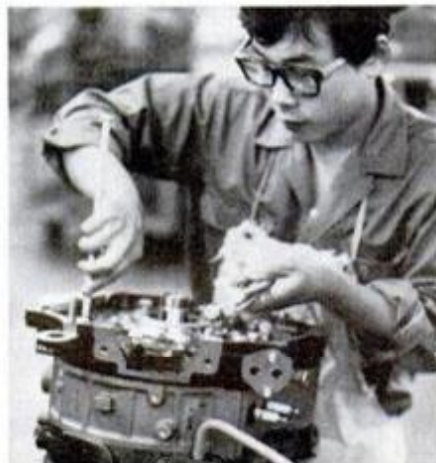
Two-rotor Mazda engine is assembled at Toyo Kogyo's Hiroshima factory.
