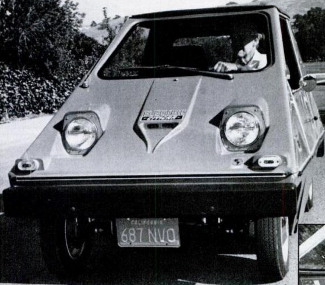
Batteries of Jones' Citicar are under seat. His '75 model uses six; newer models, eight. This is his second electric. The first was an old Goggomobil that he converted to electric. Only problem he's had with his Citicar was dragging front disc brakes. He fixed the problem with rubber bands!
