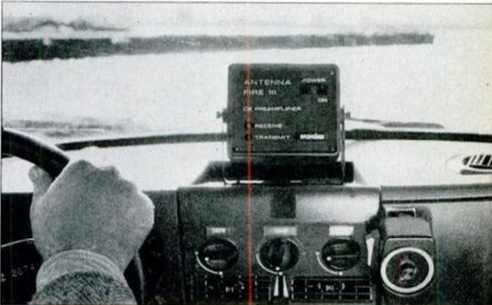
Mike at right has a tuning dial; the antenna preamp atop dash boosts weak signals.
