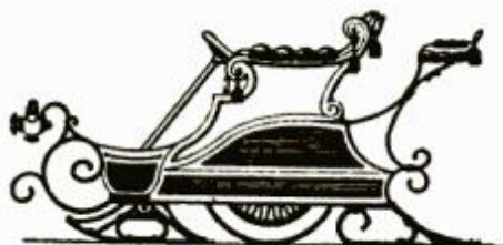
1902 Fancy car for snow and ice sported runners, center drive wheel and carriage-like contours.
