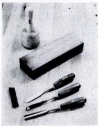
Tools used are (from bottom): straight gouge, bent gouge, skew chisel, mallet, slipstone.
