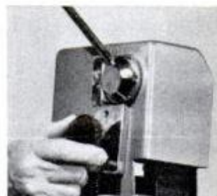
Strong spring won't let belt-tracking adjustment shift during belt change.
