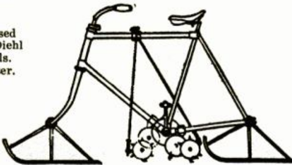
1902 Runners replaced wheels on winter "velocipede." It used pedals and gears to drive spiked discs.
