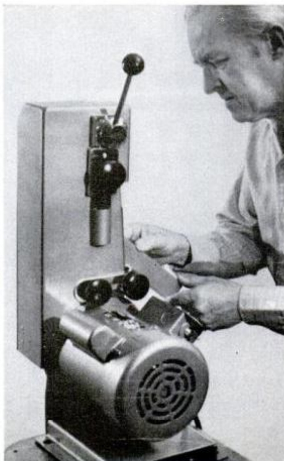
Single-phase ½-hp motor drives 2x36-in. belt 4500 f.p.m. Workrest tilts and locks at any angle, can be adjusted by hand.
