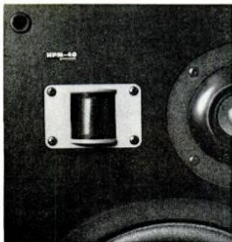
Pioneer tweeter is unique, piezoelectric type. Plastic half-cylinder shown here flexes with signal to produce sound.
