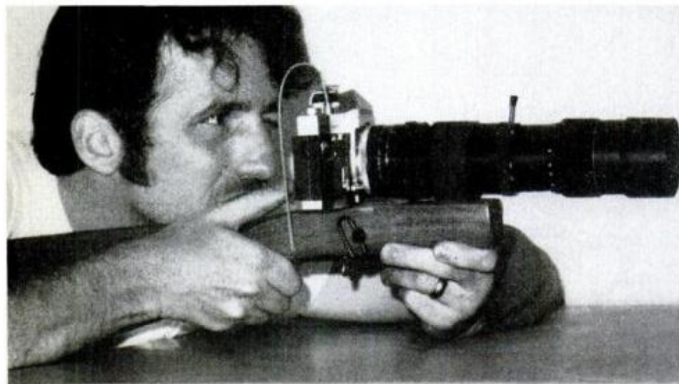
Screw and mounting plate , inserted from under stock, hold camera by tripod hole.
