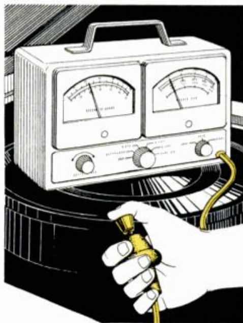
5 Remote starter switch makes it possible to crank the engine while working under the hood.
