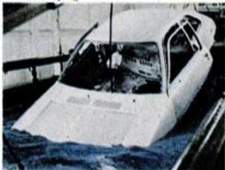
Our electro-dip priming process: part of our Improved Corrosion Protection Plan for '77.
