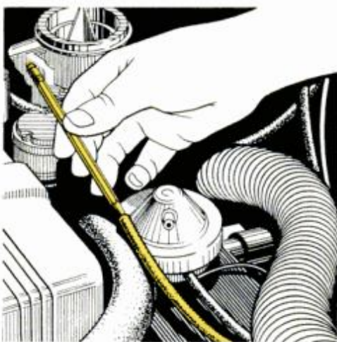
7 Hoses to vacuum advance must be plugged (you can use pencil) before setting ignition timing.
