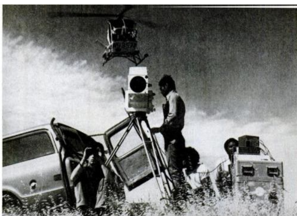
Laser ranging devices (right) are part of the new arsenal of earthquake-prediction equipment. They can detect minute changes in land formations. Scientists can "read" quakes on seismometer printouts.
