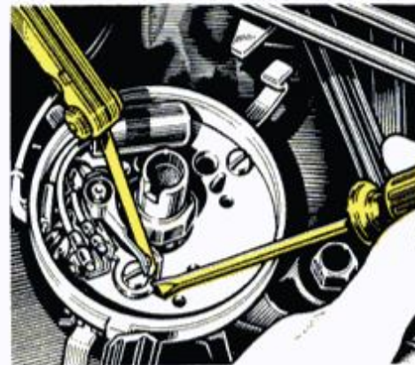
12 Point gap can be set accurately by means of the adjustment notch in the point assembly.
