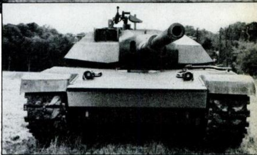
The two XM-1 prototypes—General Motors (top) and Chrysler—have low silhouettes, good stability, speed near 50 mph.
