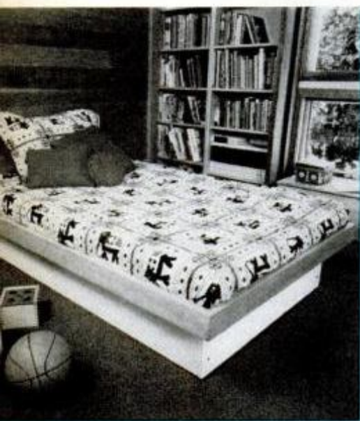
You can build this simple platform bed for about $50, including the foam mattress. The solid platform is surrounded by pine rails, mitered at the corners and reinforced with 5/4-square kiln-dried strips. The support platform is made of plywood and painted to suit. Pull out the eight carriage bolts and the bed will store flat.
