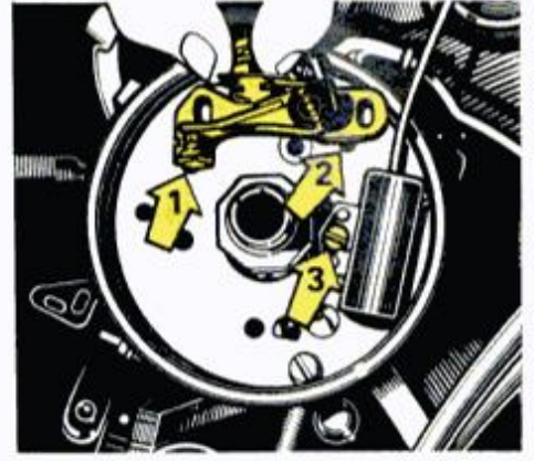
7 Remove distributor point assembly held at mountings (1) and (2). Note condenser mounting screw (3).
