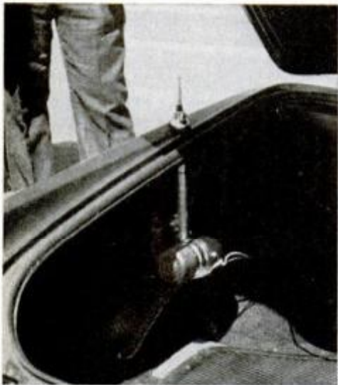
Retract your antenna and it won't attract thieves—or vandals, either. This model, from Tenna, is center-loaded. Many makes of retractable antennas are available, some of them doubling as antennas for ordinary AM and FM car radios.
