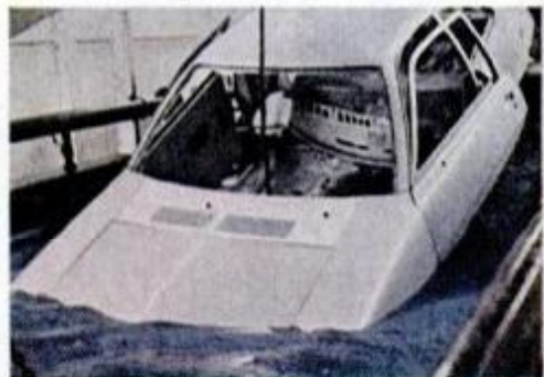
Our electro-dip priming process: part of our Improved Corrosion Protection Plan for '77.
