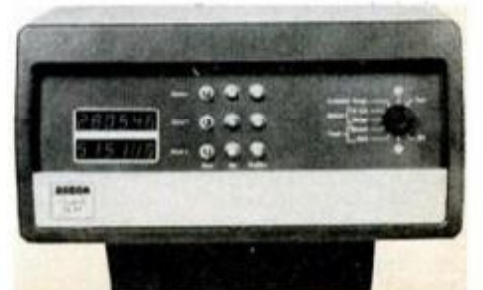
Loran C is an expensive fishing aid, but can give skipper instant pin-point position by measuring radio waves from two stations. Decca DL91 is $4995.
