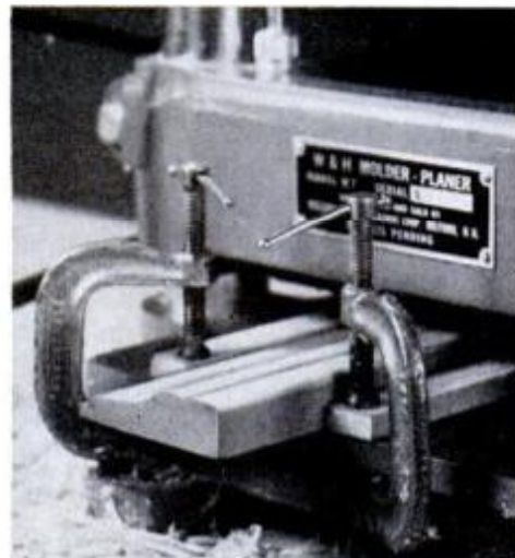
Alignment strips clamped to base keep stock passing straight under twin molding knives. Cutter head turns at 7000 rpm, requires 1-hp motor and 5-in. pulley.
