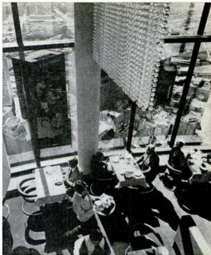
Unusual rooftop restaurant , more than 700 feet high, slowly revolves to give diners a spectacular, ever-changing view of Atlanta's skyline. Its floor is so perfectly supported on friction-free bearings that only two ¾-hp motors are needed to turn it. Restaurant is one of 12 in luxury-loaded hotel.
