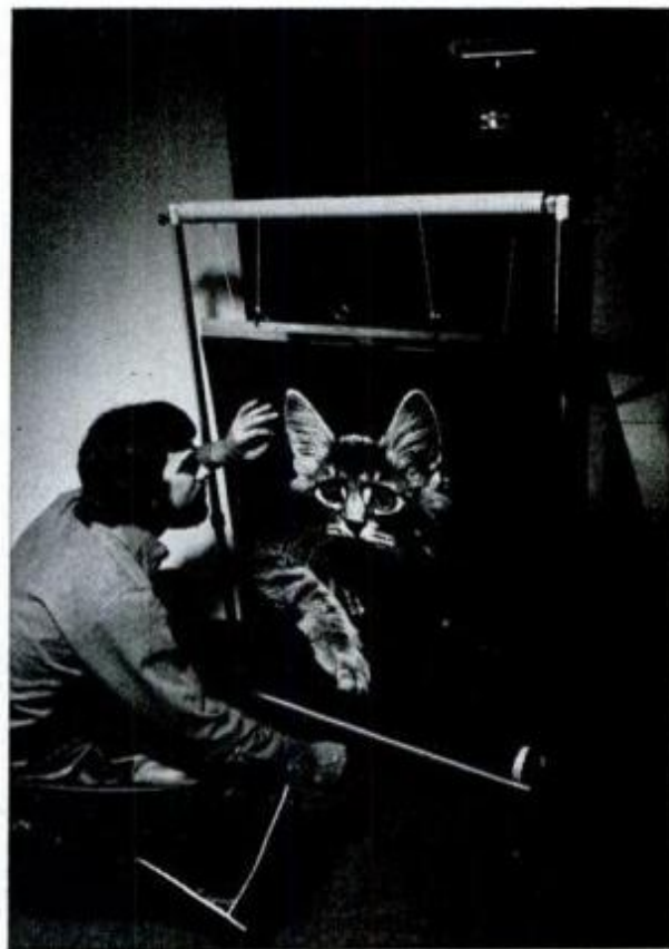
Big Dipper is expensive ($119), but its crank system makes it easy to roll the paper through the chemicals evenly.
