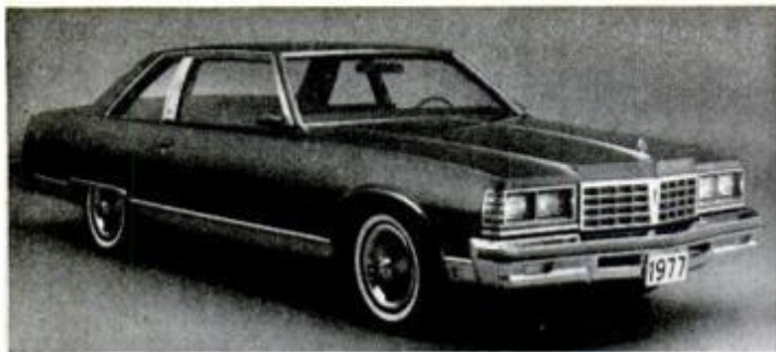
Pontiac Bonneville two-door hardtop coupe is on a 115.9-inch wheelbase. Overall length is 213.8 in.; width, 75.4 in.
