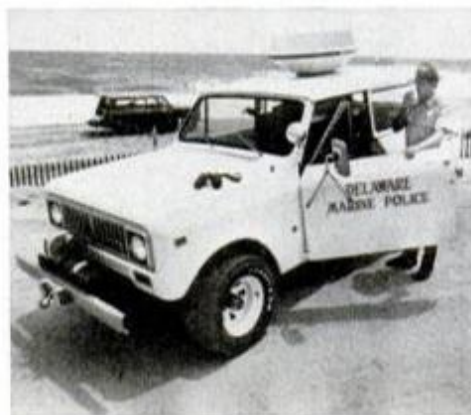
Onshore offshore patrol is provided along Delaware coast with International Scout II's roof radar that locates fishing boats up to 12 miles out in the Atlantic.
