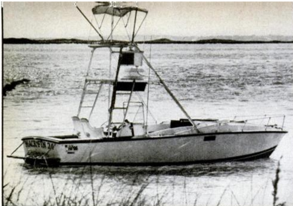
Biggest fishing rig for regular trailering may be 24-foot Blackfin with 30-mph Caterpillar V8 diesel, from Karanda Marine, Fort Lauderdale, Fla.
