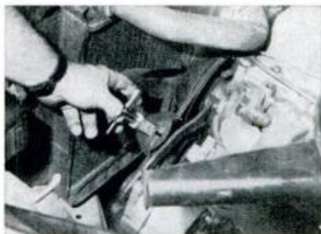
Belt tension is best checked using the type of tension gauge shown here.
