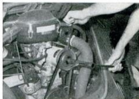
Pulley nut is loosened on VW while screwdriver is wedged to hold pulley.
