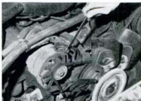
Bracket with curved slot is most common arrangement for belt-tension adjustment.
