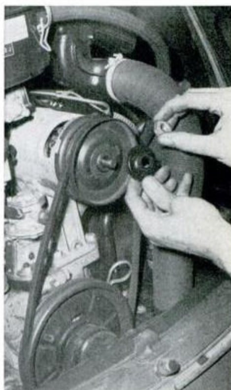
Pulley halves are separated to remove belt with unique arrangement on Beetle.
