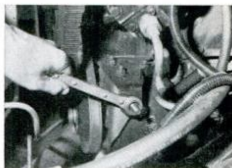
Studnut adjuster on power steering pump is tensioning device on some Fords.
