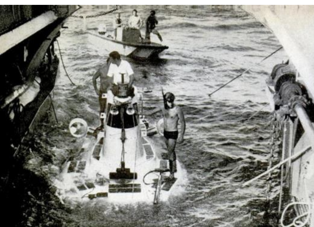
Back from dive, Alvin is carefully guided into stern well of mother ship Lulu for retrieval in a cradle (left). Above, a technician checks diving weights—stacks of steel plates each weighing 230 pounds—that can be released to control buoyancy.
