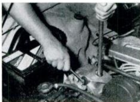
Pilot hole for the pry bar, as used on Chevette, is accurate and convenient.
