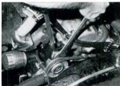
Adjuster is turned to tension idler pulley as seen here on the Dodge Colt.
