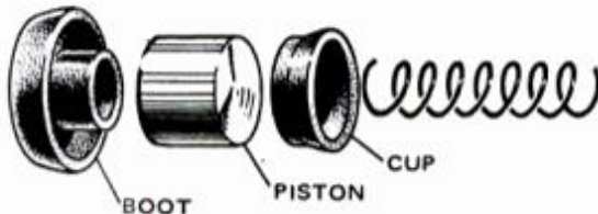
Exploded view 1: Typical brake cylinder (wheel cylinder) has two boots, pistons and cups, plus a common spring, cylinder housing and bleeder screw.
