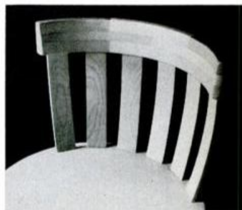
Close-up view of chair-back rail shows an interesting effect of laminated segments.
