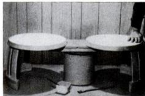
To glue top rail to slats, apply level support, then glue and press it into place.
