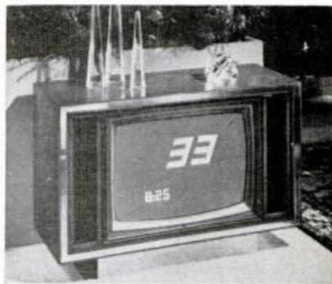
Digital keyboards and readouts zip you from one station to another as fast as you can push two keys. Some sets have on-screen readout, visible only when tuning.
