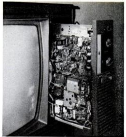
Works in the drawer of the latest, large-screen Quasar sets are all on one, big "Super Module." Panasonic and JVC follow similar, modular-building approaches.
