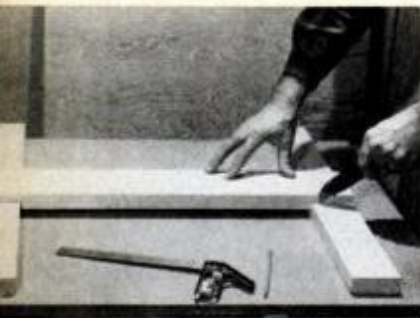
tion upright on base, and mark mating lap with knife blade for accuracy.
