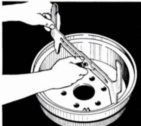
8. Drum-to-brake-shoe clearance gauge is set to measure inside diameter of drum.
