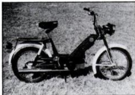
Jawa Babetta gets 130 mpg; fuel tank holds .8 gal.; ignition is transistorized.
