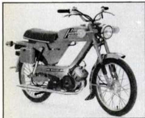
Jawa Babetta gets 130 mpg; fuel tank holds .8 gal.; ignition is transistorized.
