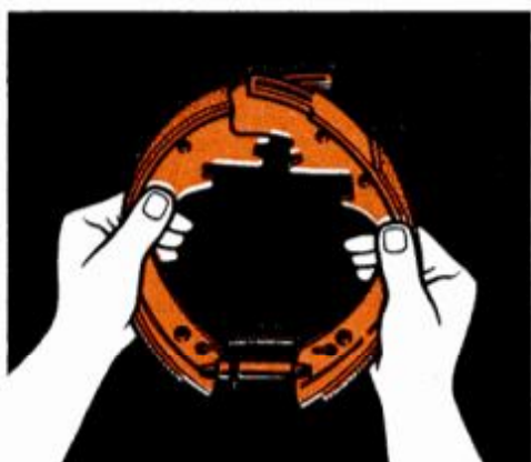
13. Separate shoes by relieving tension on the adjusting spring.
