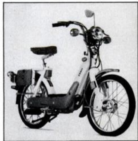
Jawa Babetta gets 130 mpg; fuel tank holds .8 gal.; ignition is transistorized.
