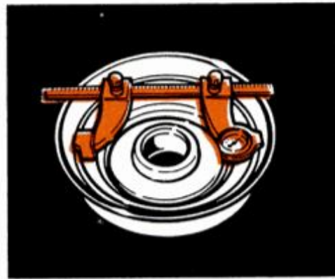
5. Brake drum is checked with micrometer for wear, out-of-roundness, taper.
