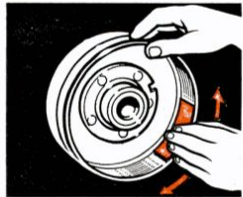
2. Lightly buff drums that are in good condition with emery cloth.
