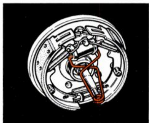
7. Use clamp to hold wheel cylinder boots in place to prevent fluid leakage.
