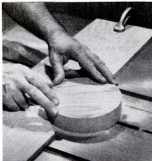
Saucer-like cut in the underside of a wood disc is made by rotating work over saw blade. V-notched board is clamped to table so it positions disc directly over blade.
