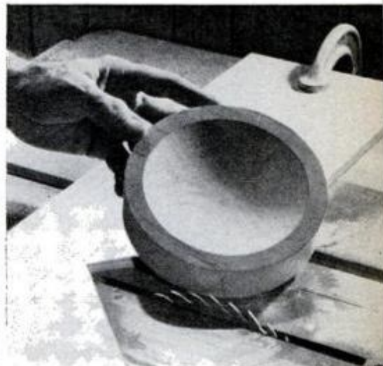
Saucer-like cut in the underside of a wood disc is made by rotating work over saw blade. V-notched board is clamped to table so it positions disc directly over blade.
