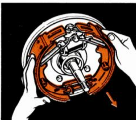
12. Assembly of brake shoes, adjusting screw and spring is removed.
