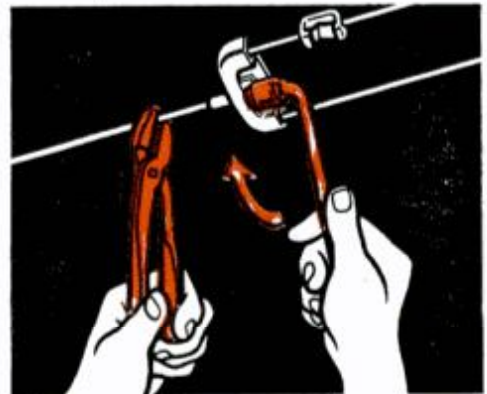
1. Parking brake cable tension is released by loosening adjusting nut.
