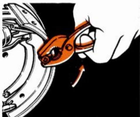
9. Hold-down springs are compressed and cups rotated to line up with pins.
