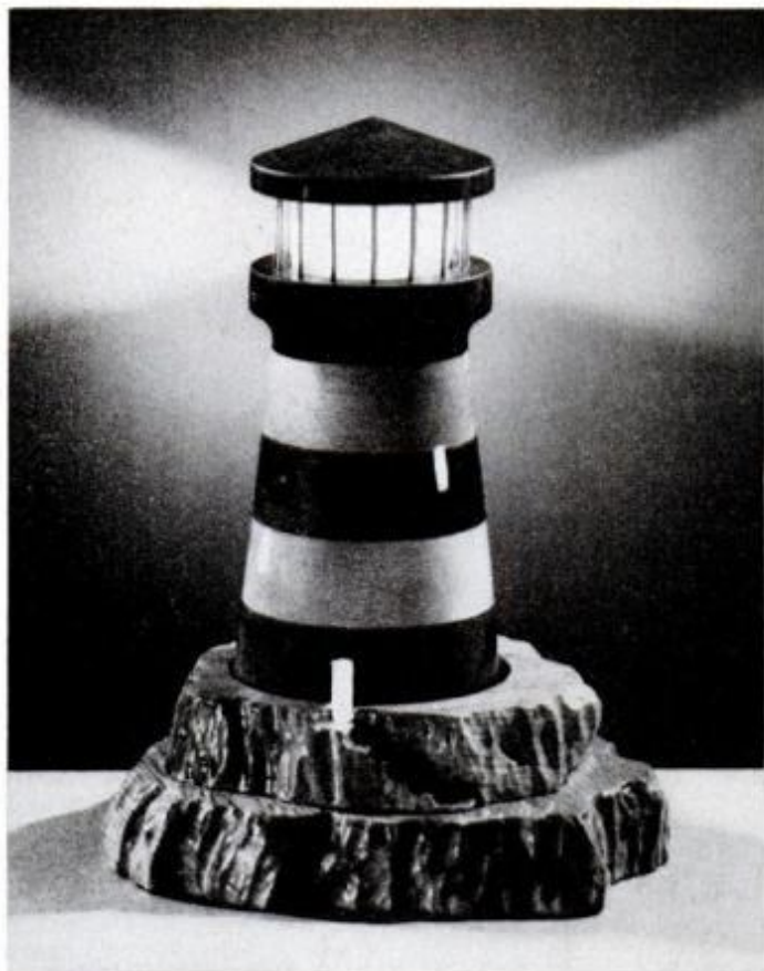
Socket well and the top recess both are turned after base is glued and fastened to faceplate of the lathe. The lamp cord is passed through hole drilled in side of the base.
