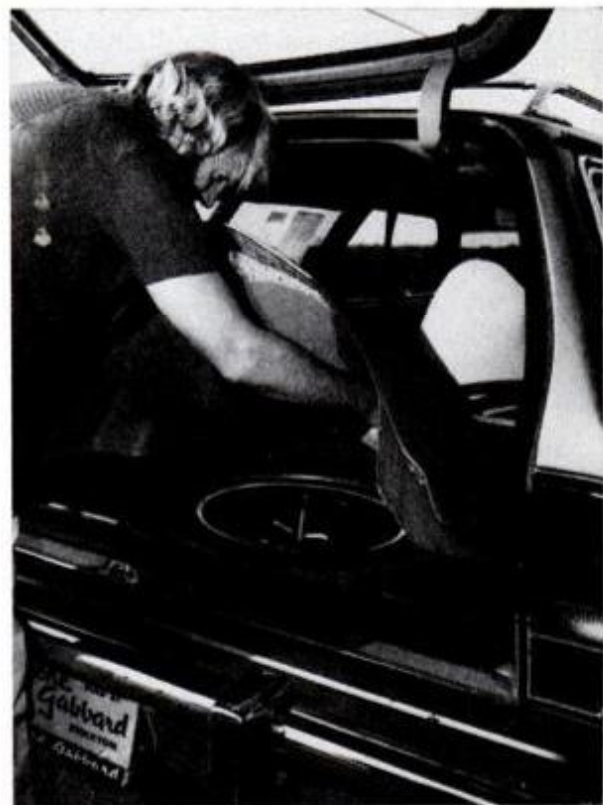
Spare tire lies flat under floor of station wagon and is covered by carpeting. Owners are mostly happy with wagon, but some want to see four-door version.
