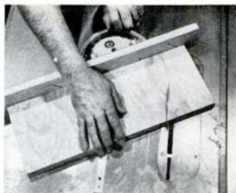
When parts are cut individually from separate pieces, the first cut is made with the work held in position shown above.
