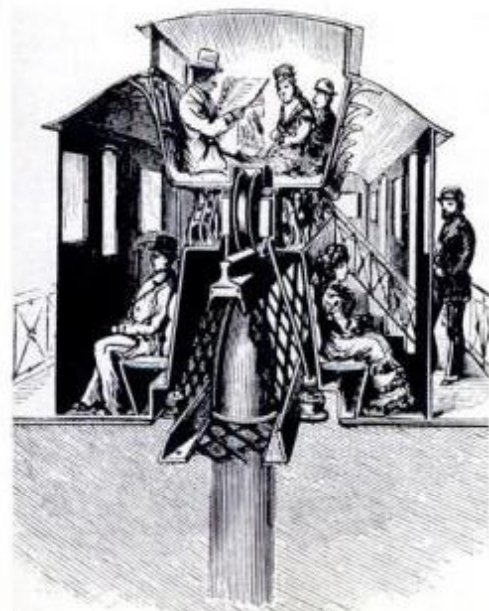
Prismoidal Railroad that carried Centennial visitors to a nearby restaurant was one of America's first monorail experiments.
