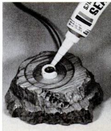
Exposed socket terminals and wires are coated with a layer of silicone rubber.
