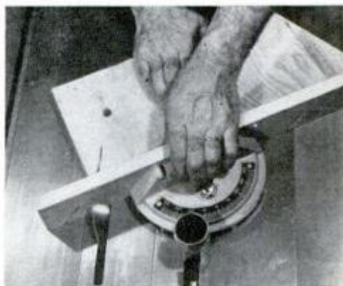
To make second cut, miter gauge is turned around and used backward in the table. Same miter-gauge setting is used.
