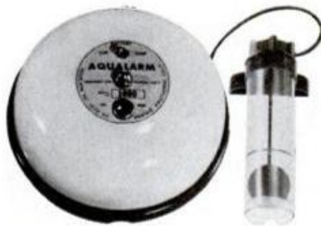
Bilge alarm is triggered by rising water which pushes up float to activate bell.
