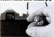
A round sewing-machine bobbin used as a finger grip adds leverage to cheap cable releases that lack wing-type finger holds. Just slip the camera end of the cable through the bobbin so the bobbin forms a flange for the plunger.—Grace B. Weinstein.
