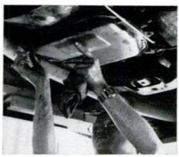
11. Replace the pan using a cork or a neoprene gasket, and don't use any adhesive on the gasket. Run up a couple of bolts to hold the pan while you align the gasket, and then tighten all bolts in a crisscross pattern to prevent any warping of the pan.
