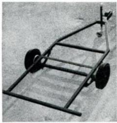
Welded frame is made from 2-in.-square steel tubing. Optional electric or surgetype brakes are not required by law in most states, but do provide extra safety.
