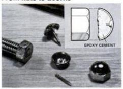
If you are in a bind for some acorn nuts, you can make your own by cementing the tops of nickel-plated upholstery nails to regular nuts. Simply cut off the nail shanks and fill the heads with epoxy.
