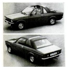
The latest German Opel, for Europe only, is a convertible that's based on the Kadett sedan. It's Opel's first convertible since 1955. The Aero is not a true convertible, of course, but it is an open car using the Targa approach: The roll bar remains in place, the top roof panel is removable and the soft rear panel folds down.
