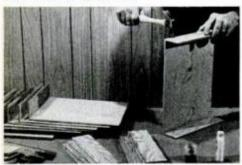
Assemble trays with glue and %-in. (20ga.) brads, being careful to drive them straight. Cut parts from flat plywood.
