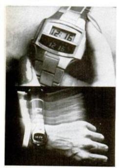
Battery savers: Longines G-II (top) has liquid crystal daytime display, pushbutton LED for night. Pulsar AutoCommand (above) lights when you flick your wrist.
