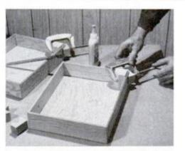
Protect outside corner with a notched 90° block when gluing and clamping pivot blocks in right front corners of trays.
