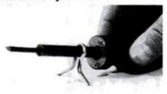
A large cotter pin bent as shown and forced over your soldering iron will provide a handy two-legged stand that's always there when you need it. -Ken Patterson
