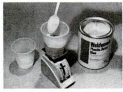
Glues which require mixing with water should be proportioned very carefully for best results, A postal scale will be useful for weighing the components.
