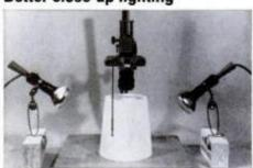
For shadowless close-up lighting of small objects, use a plastic lamp shade around the subject as a lighting tent. It will diffuse illumination evenly, withstand the heat of your photo lamps and leave a hole for the camera to shoot through.
