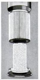
The outer hiter: a 6 foot phenoiimpregnated cellulose element. The inner filter: a fiber strand more than 60 feet long, wound on a steel core. Your oil goes
