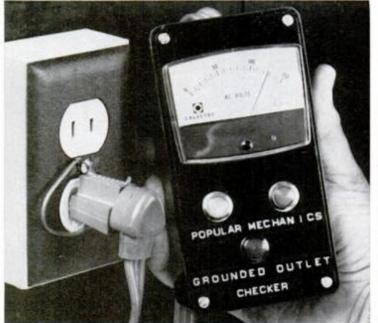
Tester measures line voltage and checks outlet wiring (see table below). Designed for three-wire grounded outlets, it can also check three-wire adapters used in two-wire outlets; here, yellow light shows that "ground" screw isn't really grounded.
