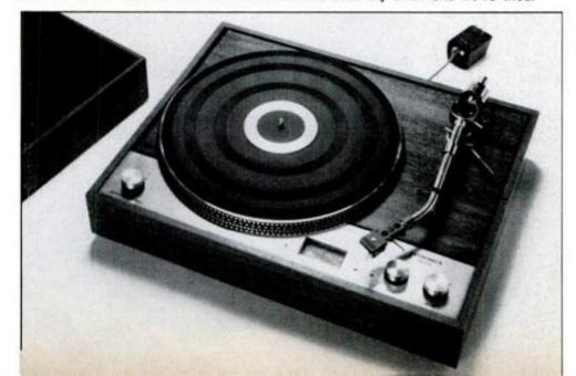
wheels and belts and gears designed to transmit the motor's power to the platter that turns the record, while reducing the motor's 1800-rpm speed to the record's speed of 45, 78 or 33½ rpm. That tradition seems to be ending, for the two unique turntables shown here have none of those parts. Instead, their motors drive their platters directly.
