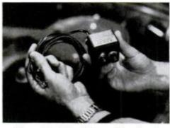
The principle of operation is simple: The Stop-Thief leads replace the 12-volt hot wire from the coil to the distributor. There's a thermal circuit breaker which will blow in a couple of seconds if someone should start the car and the unit is set in the on position.
