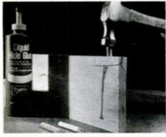
This hammer test shows how trapped glue at bottom of hole can cause work to split when clamping pressure is applied. Always plane a flat on dowels.
