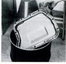
10. Clean the transmission pan thoroughly in solvent before you put it back on the transmission body.
