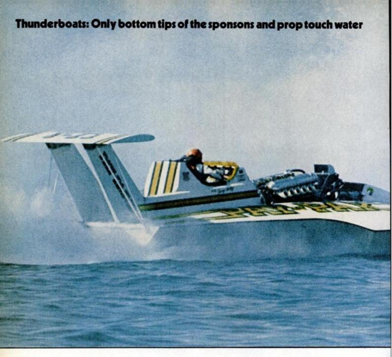
steering has to be by means of one or more submerged rudders. Competition is held on a two-and-a-half or three-mile oval course. This effectively eliminates the jet-powered rockets that can approach 400 mph in a straight line but could never complete the first turn. Airfoil adjustments that could be changed by the driver during a race are not allowed. Part of the skill of designing and driving an unlimited, in fact, is to keep it from turning into an airplane—and the disaster that follows.
