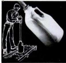
Filled with concrete and fitted with an iron-pipe handle, a ½-gal. plastic jug makes a fine lawn and fill tamper that weighs almost 13½ lbs. Use second jug for funnel. Let soupy mix set and cure two weeks.
