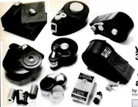
Film loaders and accessories include (clockwise from upper left): Premier, Prinz 66, Western, Watson, unbranded model, Prinz standard. In front row are empty cartridges, bulk film and new Whitehead Cinek self-loading spools still in pilot production stage.
