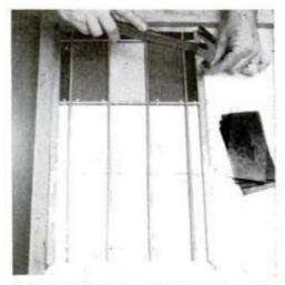
8. L-shaped cleats nailed to wood workboard hold the window along two sides and assure squareness. Tap each section of glass firmly into channels of leads with hammer and wood block. Nails hold the border and inside leads for soldering.
