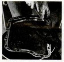
Old gasket should also be scraped away from the transmission pan.
