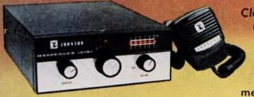
Clearly an improvement! Bright ruby red LED readouts let you read signal strength, transmitter power and modulation precisely ... at a glance! All solid-state, it's completely reliable regardless of temperature, dust or humidity. Solid-state metering—exclusive in the Messenger 123SJ.
