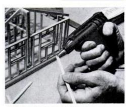
Hot glue from an electric glue gun provides quick gluing for many do-it-yourself projects and hobby crafts. You'll find it handy for gluing parts of models.
