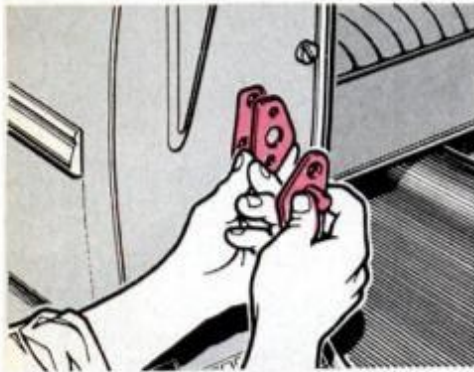
Realigning a car door will require an adjustment to the door striker plate.
