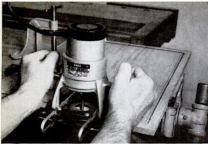
Clamp tabletop securely to workbench when routing groove for ebony cock beading. Square corners carefully with wood chisel.
