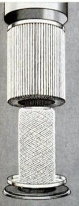
The outer filter: a 6 foot phenolic impregnated cellulose element. The inner filter: a fiber strand more than 60 feet long, wound on a steel core. Your oil goes through both approximately once every 30 seconds!
