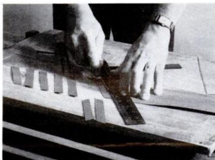
Use a veneer knife to slice the veneer 60° to the grain. Arrange veneer pieces on strip of veneer tape, then glue to table edges.
