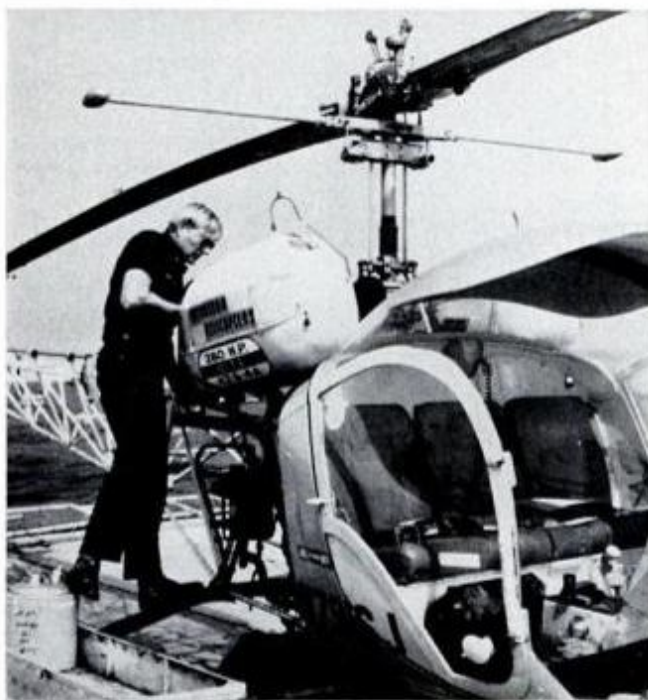
Some of the Petroleum Helicopter company's birds are based on rigs and platforms in the Gulf. To service them, mechanics are flown from PHI's Morgan City base. The man shown is working on a Bell 47G-4A. The Morgan City layout (also shown), said to be the world's largest commercial heliport, has 46 pads. The air really hums here during the early morning "rush hour."
