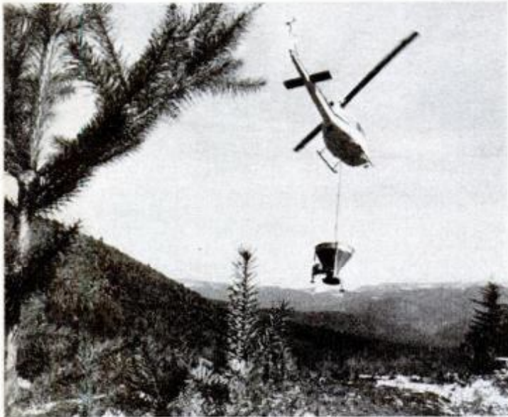
Fertilizing by air speeds process of promoting good forest growth, is one of latest techniques in advanced tree culture. At top, a chopper leaves a swirling white trail as it spreads growth-giving nutrient over young forest at treetop level. Lower photo shows large spreader hopper slung below helicopter that holds and releases 3500 pounds of fertilizer per load.
