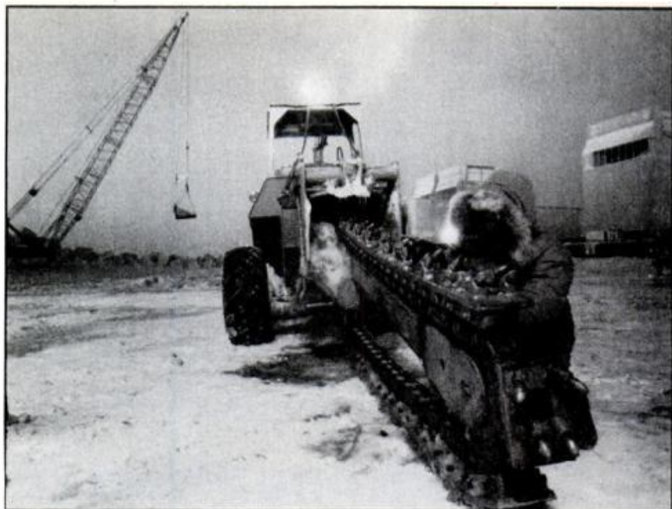
Ice chewer-upper is this Bunyanesque version of a portable chain saw. Mounted on a vehicle the size of a D9 Cat, it can slice a fast trough through ice or permafrost.
