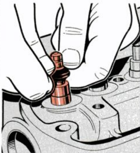
New seals installed over valve stems may be necessary if you're burning oil.
