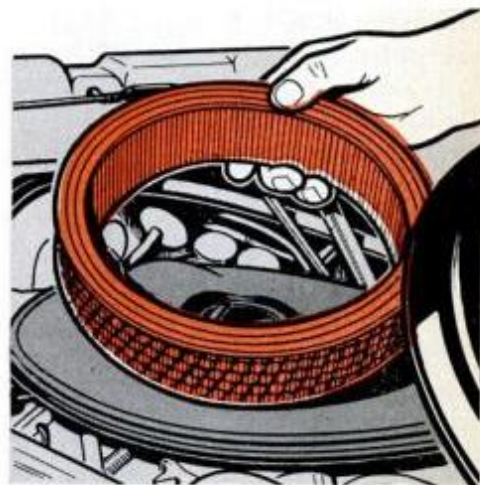
Air filter should be checked if black exhaust smoke indicates too-rich mixture.
