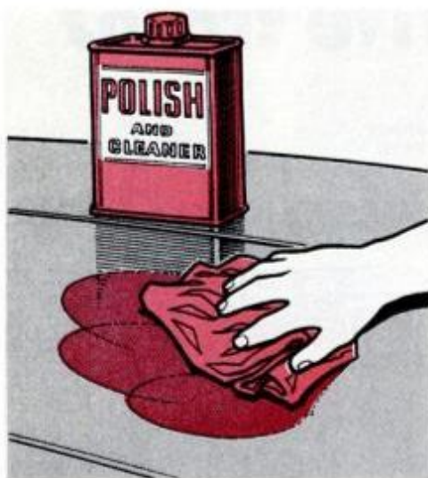
Cleaning and polishing removes dead paint and lays down protective finish.
