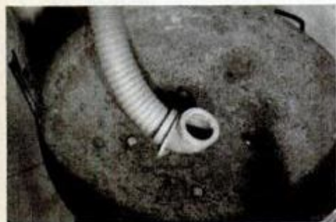
Fasten 90° pipe elbow to bottom of grill with U-bolt; it saves cutting large hole.
