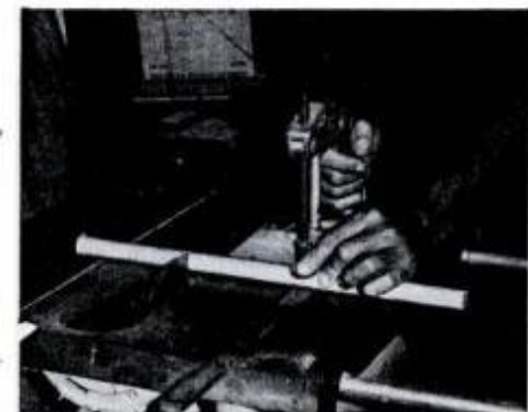
First cut divides \frac{3}{4} -in. birch dowel into 5\frac{1}{2} -in. length for the popper plug bodies.
