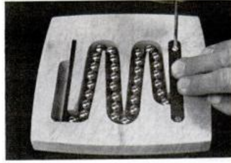
6. Fit ball-release spring in right-hand channel and nonrelease spring in left.
