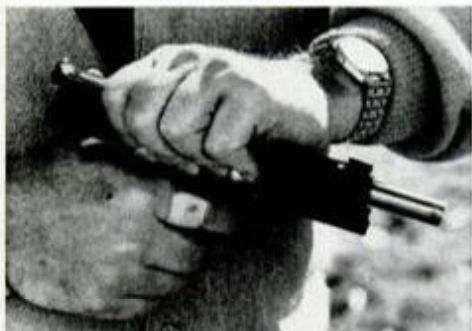
Safe handling , essential to all shooting, is demonstrated as Blankenship holds the hammer in cocked position while releasing slide so hammer can't fall forward.
