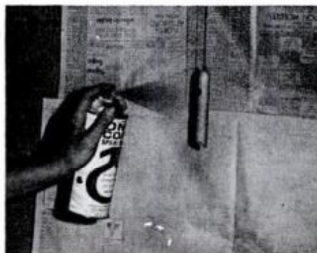
Plugs are painted with a number of coats. One or two treble hooks are then added.
