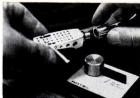
Cartridge heads on most of our turntables were mutually interchangeable type shown. AR, BSR, Garrard and Philips had different, but still detachable cartridge mounts.
