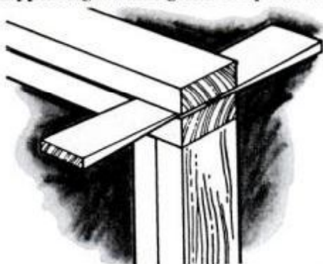
Shim from both sides. This will help to keep the board level and stable.
