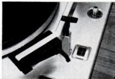
Stylus force gauge of Philips was a scale whose platform was the tone-arm rest.
