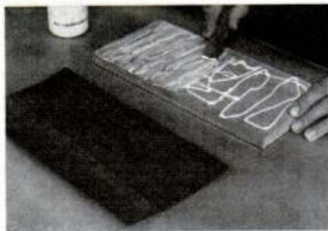
1. Spread white glue over top of the 3/4-in. base and cover with walnut veneer.
