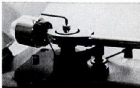
Antiskating adjustments were mostly either string-and-weight type (near side of tone arm above) or weight-and-lever type (rods visible behind tone arm below). I found no difference in performance—even with AR, which had no antiskating.
