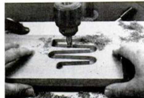
5. Rout 1/2-in.-wide ball channels in the base with drill press at high speed.
