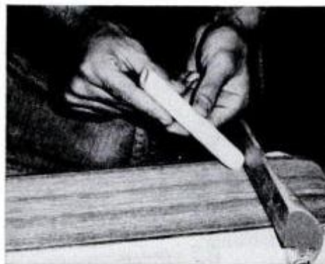
Head and tail ends are rounded on a belt sander, shaft smoothed with hand sanding.
