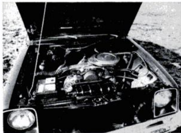
Chevette's 1.6-liter ohc Four has cast-iron block, 60 bhp, peaks relatively quickly with standard 4.1 axle.
