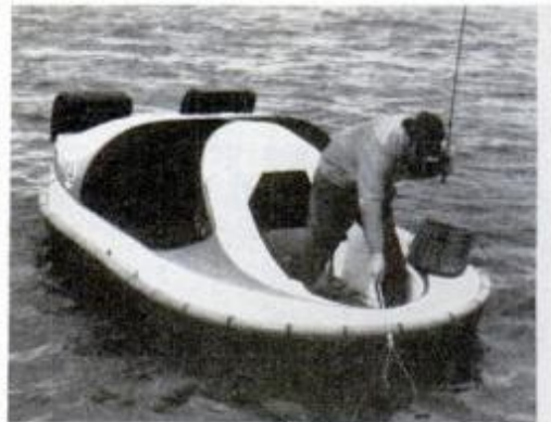
Afloat and ashore , the Neova 2 Hovercraft rides on air at a reported 35 mph with VW engine. Plans are sold by Neoteric Engineering, Terre Haute, Ind.
