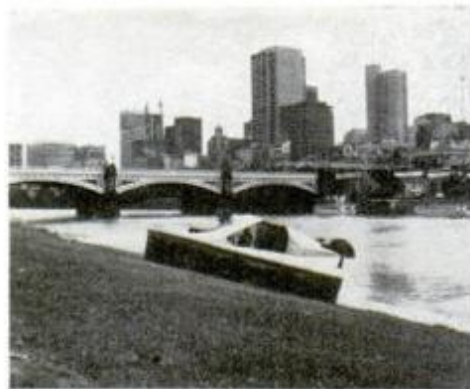
Afloat and ashore , the Neova 2 Hovercraft rides on air at a reported 35 mph with VW engine. Plans are sold by Neoteric Engineering, Terre Haute, Ind.
