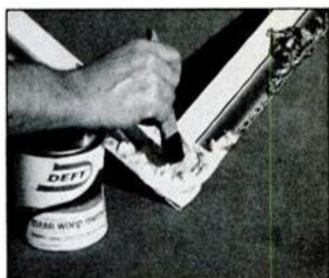
9. Coat new overlay with clear sealer (Deft), wipe frame with a lacquer thinner, then spray entire frame with a gold paint.
