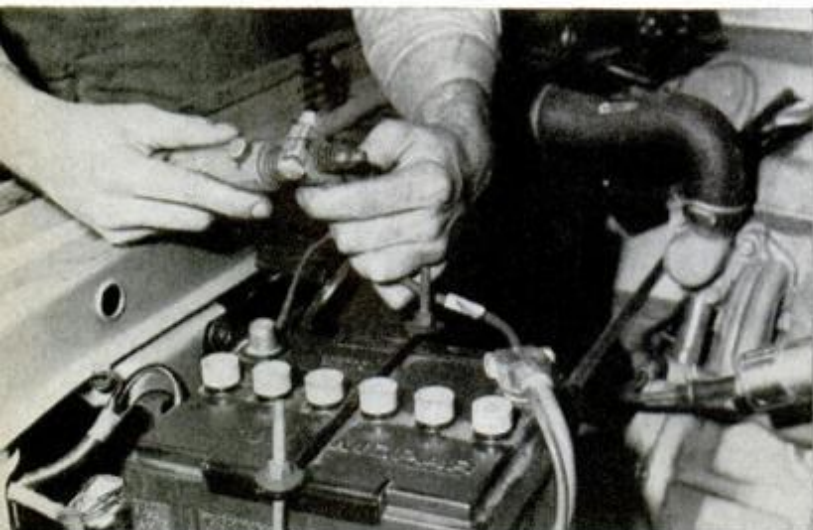
Battery terminals and cables that are dirty or not tight cause most no-start problems. Use wire brush tool to clean terminals (as shown above) and posts.
