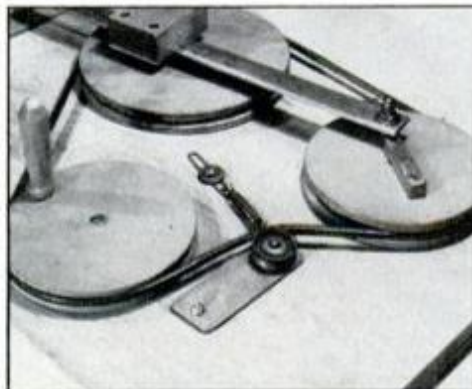
Spring-loaded idler pulley keeps belt taut, slip free. Belt dressing also helps.
