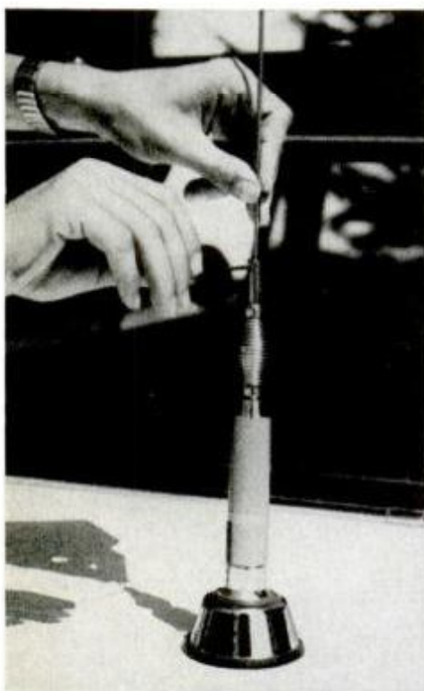
Matching antenna involves minor length adjustments (top) using SWR meter like this Radio Shack model (below) as guide.
