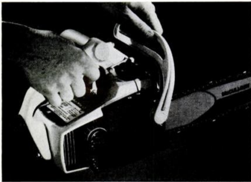
Cutaway view shows how braking lever mounted ahead of top handle tightens steel band around clutch drum when moved forward, stopping chain instantly—a "brakethrough" in reducing kickback.
