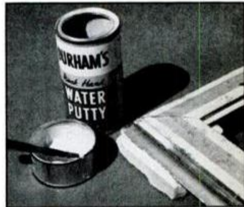
6. Place filled mold right side up under face side of the frame corner, press down frame into wet putty to force out excess.
