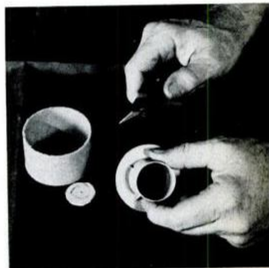
Flanged hose connector is made from plastic cap off spray-paint can. You cut away the outer shell and center of the top.
