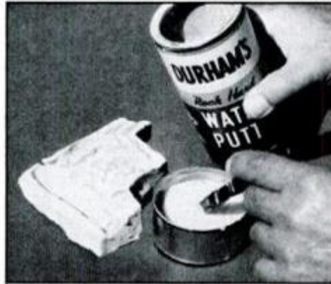
5. Pour water-putty mixture into inverted mold level with top. Mix putty until it reaches the consistency of thick cream.
