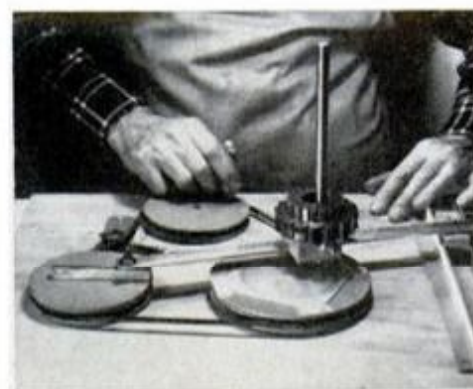
Added weight (milling cutters) on stylus arm lets diamond cut brass deeper.
