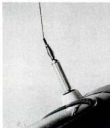
Gutter mounts include screwdriver-locking type (this one with built-in flip-over to clear obstructions) and temporary clip-on; both from Antenna Specialists.
