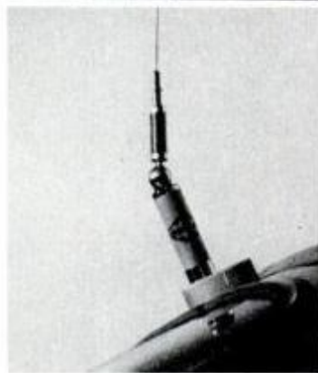
Hatchbacks can take regular trunk-mounts like this Radio Shack one (top), but angle may be wrong; one solution is to bend it (center) or use Hustler's ball-mount (above).
