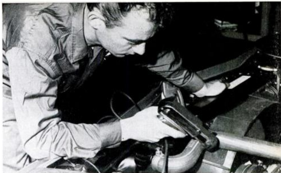
Time ignition system. If timing cannot be set, suspect the distributor, assuming that breaker-point dwell is set correctly.
