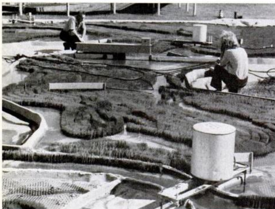
A tidal model of New York Harbor (top) is used to study navigation, shoaling and environmental problems. During the 1973 flood, the Mississippi Basin model (above) was reactivated to predict flood problems. A new model (right) of the diversion structure was built and a quick-fix found for the failing wing-wall abutment protection shown at the top of the photo.
