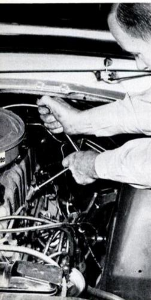
Remove sparkplugs. Check wide gap, electrode deposits, worn electrodes, damage.
