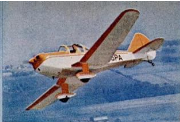
Canard-winged VariEze is a mini version of its famous bigger brother, the VariViggen (page 145, March '73). It's shown here fitted with special auxiliary fuel tank in rear seat just before setting world distance record. For more, see article that follows.
