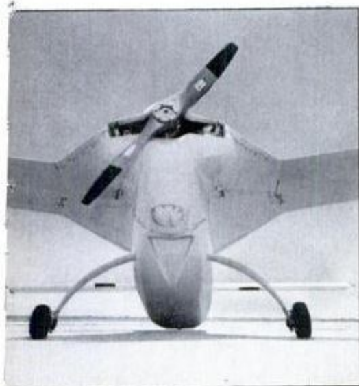
Rear view shows pusher prop and wide-bodied fuselage that flares into wings. Fuel tanks are housed in these thick wing-root sections so they take up no space inside craft itself. Bow-shaped main landing gear strut is single piece passing straight through the fuselage. This eliminates separate struts, simplifies mounting, lessens impact strain on airframe attachment points. Engine is 62-hp VW, giving a 185-mph cruise speed.
