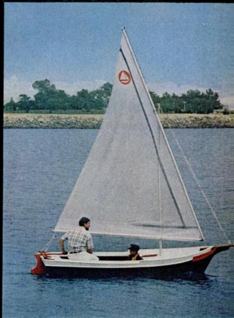
Sailing workboat lines rendered into a 13-footer in plywood, the Mini-Indy by Peter Stevenson has the character-boat look of a Chesapeake Bay skipjack.
