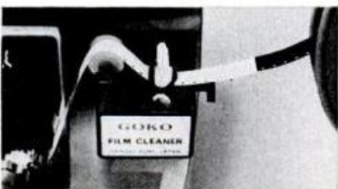
Film cleaner helps protect edited film against dirt which can cause scratches.
