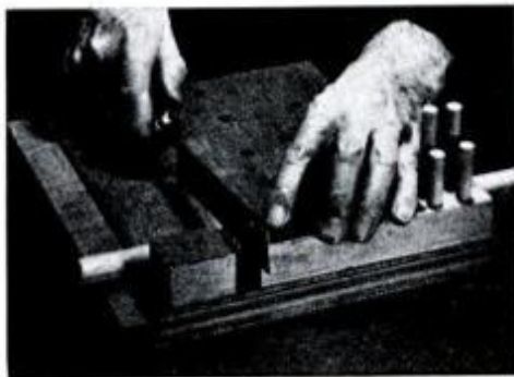
When sawed through gap in a cleat, both parts of workpiece are firmly supported.
