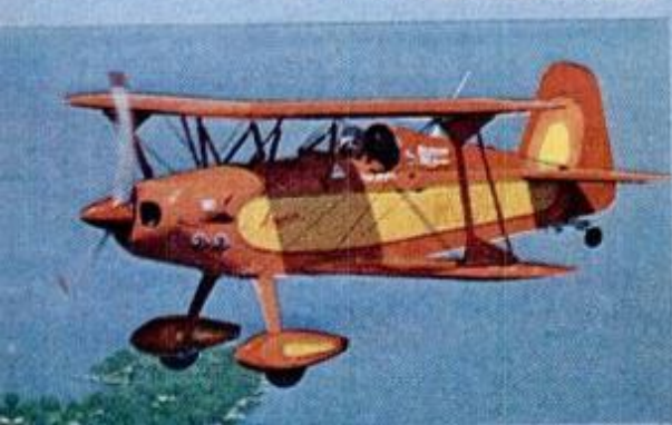
Colorful Acroduster I (above) is versatile new competition aerobatic bi-winger you can build from a kit. Wings have symmetrical airfoil for inverted flight, incorporate four ailerons, give roll rate of 240° per second. Top speed is 195 mph with 200-hp Lycoming engine. Wingspan is 19 feet; length, 15 feet, 9 inches. Fuselage and tail are aluminum; wings, Dacron-covered wood. The kit is $5500 from Stolp Starduster FORB-43R1 Twining, Riverside, Calif. 92509.
