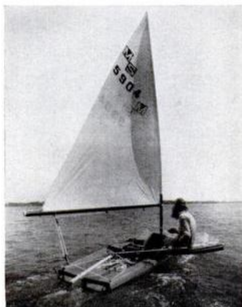
For high-performance sailing , MiniSprint Mark II, imported by KMS Marine Ltd., has open self-bailing transom, sliding seat.
