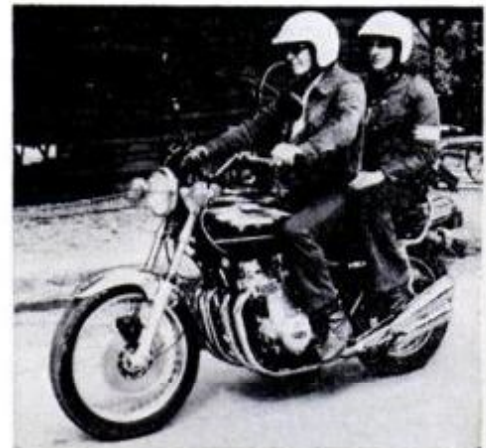
Kawasaki KZ900, quickest of superbikes, has 76 hp at 8500 rpm, weighs over 500 pounds. Quarter-mile times are between 12-13 seconds. Fuel tank holds 4½ gal.
