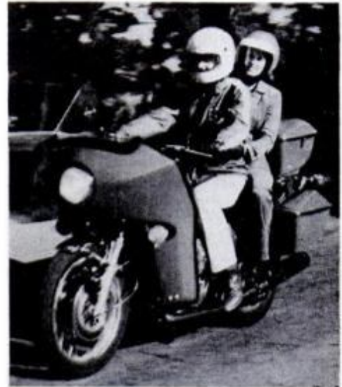
Suzuki 750 is water-cooled, two-stroke triple that weighs in at 550 pounds. In full touring trim, as shown here, it's closer to 600 pounds. Fairing makes long-distance touring much less fatiguing.
