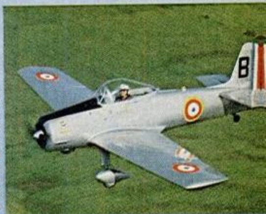
Two low-cost, low-wing monoplanes are the Hauscat (right), patterned after Grumman Bearcat and Mono Z (below), a single-seater version of earlier Zenith (page 162, March '74). Both are VW-powered and cost about $2500 to build. Plans are $125 for Hauscat, Yvan Bougie, 11 Terrasse-Robert, Nitro-Valleyfield, Que.; $130 for Mono Z, Chris Heintz, 236 Richmond St., Richmond Hill, Ont.
