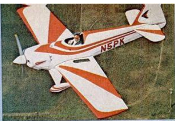
Super Fli (above) is aerobatic single-seater, has been flown by top aerobatic pilots who report good handling. A 200-hp Lycoming provides a top speed of 200 mph, a rate of climb of 3000 feet per minute. Wingspan is 24 feet. Plans and kits expected. Kraft Systems, 450 West California Ave., Vista, Calif.
