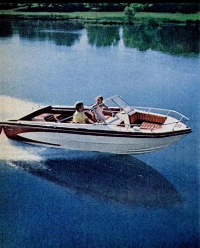
First of the Glastrons to offer bowrider design with a deep-V hull, the new SeaRider V-195 with Merc or Glastron stern-drive, has stern ladder, optional hardtop.
