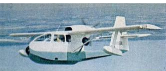
Spencer Air Car (above) is roomy four-place amphibian with 285-hp Continental engine. Wingspan is 37 feet, max. speed 150 mph. Plans $185; kits also available. P.H. Spencer, 8725 Oland Ave., Sun Valley, Calif. 91352. Sporty Namu II (facing page) seats two, does 135 mph with 125-hp Lycoming. Plans available. Peter Bowers, 13826 Des Moines Way S., Seattle, Wash. 98168.
