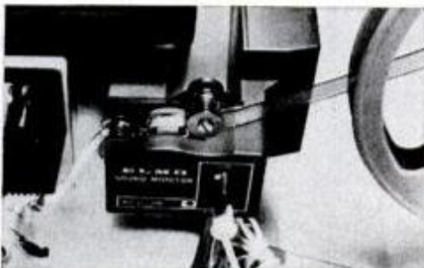
Sound reader attachment is battery powered, has volume control and earphone.
