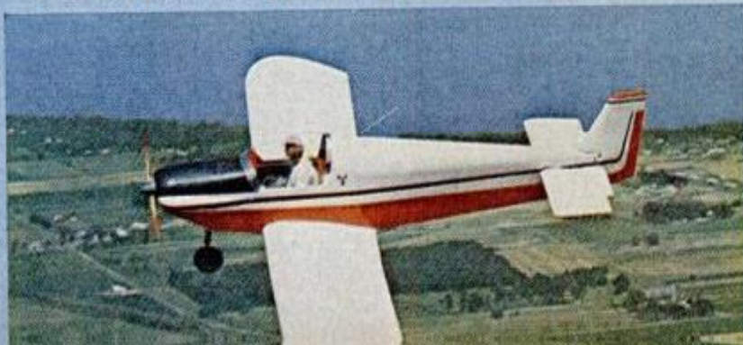
Two low-cost, low-wing monoplanes are the Hauscat (right), patterned after Grumman Bearcat and Mono Z (below), a single-seater version of earlier Zenith (page 162, March '74). Both are VW-powered and cost about $2500 to build. Plans are $125 for Hauscat, Yvan Bougie, 11 Terrasse-Robert, Nitro-Valleyfield, Que.; $130 for Mono Z, Chris Heintz, 236 Richmond St., Richmond Hill, Ont.
