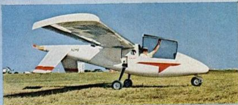
It looks like it's upside down, but it really isn't. The Mini-Imp (below) uses an inverted-V tail and new NASA-designed airfoil for high performance. Takes engines from 60 to 100 hp, is stressed to 9 Gs for aerobatics. Plans $200; kits available. M. B. Taylor, Box 1171, Longview, Wash. 98632.
