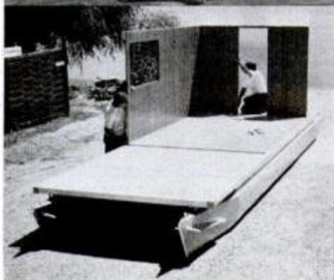
Pioneer from Kayot is called the first do-it-yourself cabin deckboat. Assembly is reported to take two workers four hours. Built on 28-foot pontoons, the 8x24 deck supports a prefab 8x12-foot cabin built with standard tools for budget boating.
