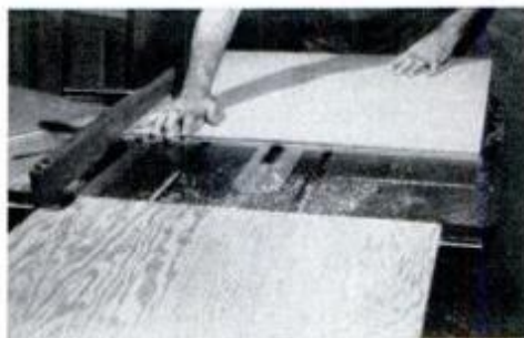
Identical dado cuts are made before moving jig. Outboard work support is must .
