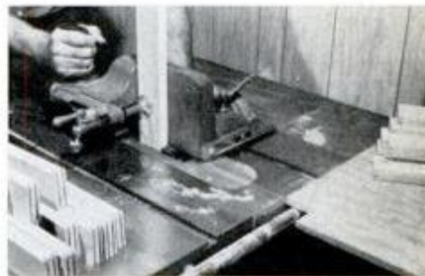
Tenon jig and pair of same-size blades with spacer are used to cut frame tongues.
