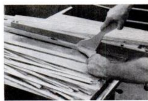
Beveled slats for tambour lid are ripped with sharp blade at 10° angle.
