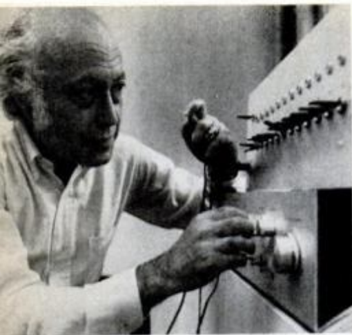
Our test equipment included this Advent speaker switcher, which let us compare all of the speakers at the same sound level, and this Yamaha amplifier.
