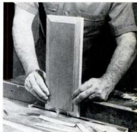
Drawer faces are beveled with saw blade set at 8° angle. Keep hands safe distance.
