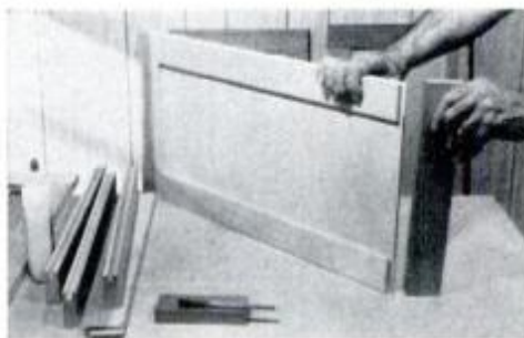
Grooved end members are added to sidepieces after latter are on dust panel.
