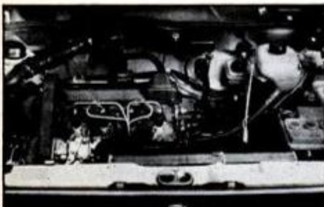
VW Rabbit diesel engine is, like the gasoline engine, mounted transversely.
