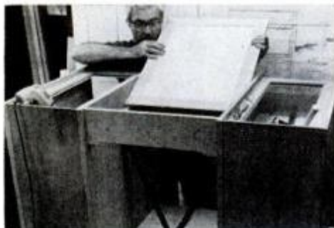
Center frame is set in place without glue, then drilled for screw pilot holes.
