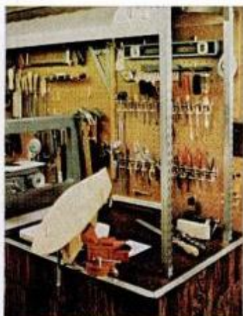
Swivel vise handles large workpieces near the support post.
