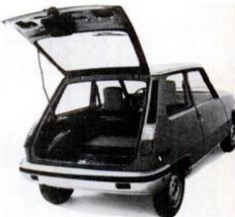
Hatchback up and rear seat folded opens up 31.5 cubic feet of cargo space.
