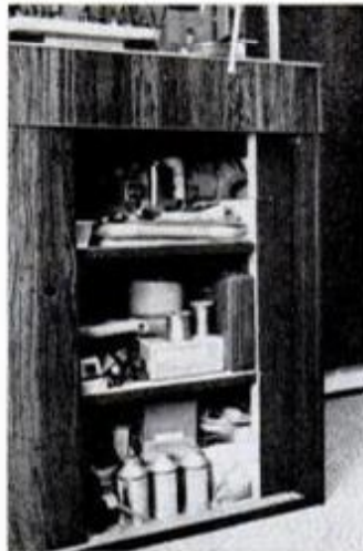
Under-bench area offers plenty of storage space for Shop-Vac and full set of attachments (left), model-building supplies (right). Sliding doors are 1/4-in. paneling running in commercial door tracks.
