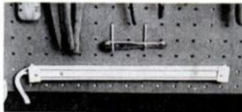
Wiring setup uses existing wall outlet behind bench to provide accessible power for tools through four-outlet, surface-mount box and continuous-outlet strip at other end of bench.
