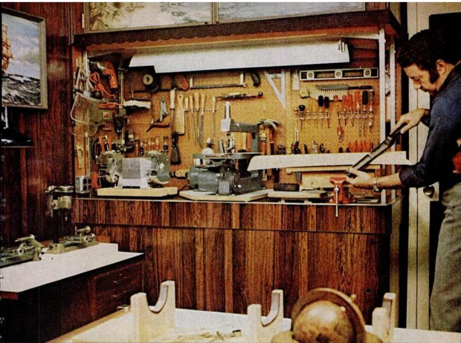
Compact shop includes everything Iken needs for modelmaking, as well as for furniture repairs, other light maintenance chores. Here he shapes a ship-model hull with a Surform tool.
