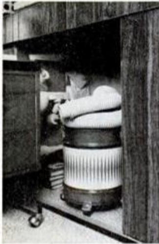
Under-bench area offers plenty of storage space for Shop-Vac and full set of attachments (left), model-building supplies (right). Sliding doors are 1/4-in. paneling running in commercial door tracks.
