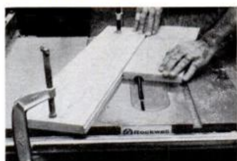
Pencil trays are made by passing stock at 75° angle across 10-in. blade.
