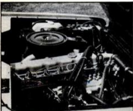
International Scout diesel engine is a six-cylinder in-line, displacing 198 cu. in.
