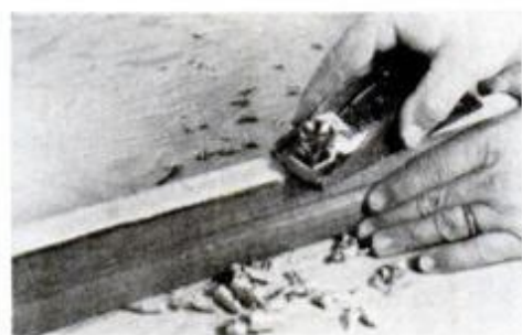
Rough saw cut is smoothed off with block plane to reshape tip and achieve straight right-angle edges with bottom ski surface.
