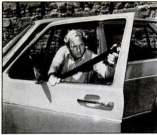
Rabbit's seat belts , once adjusted, automatically drape across chest, need no buckling or unbuckling. But clasps break easily.
