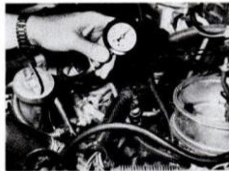
Pressure gauge is connected to the valve to take a reading of fuel-system pressure.
