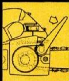
Chain Brake in engaged position, chain stopped in milli-seconds.
