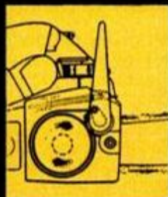
Chain Brake in disengaged position, chain running.
