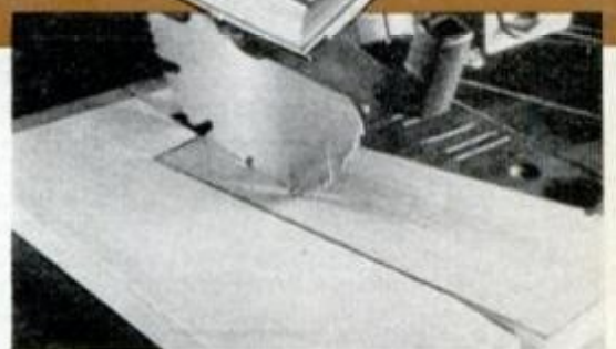
Simple homemade jig permits cutting tapered pieces on the radial arm saw.
