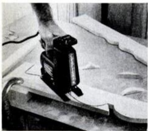
After holes are bored, curves in top and bottom members are cut with sabre saw. With dowel bars in place, ends are added.
