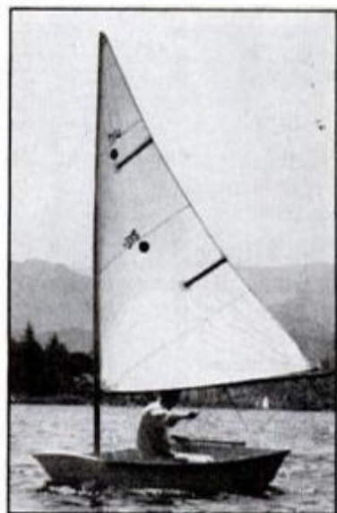
Eight Ball for beginner builders, this 7-ft., 10-in. sailing pram is $8 for Glen L plans, $45 for sail, plus cost of two plywood sheets. At about 75 lbs., it cartops easily.
