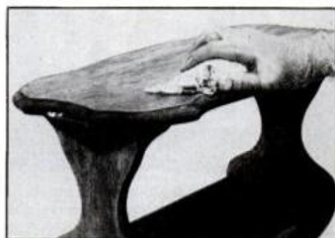
Wet toweling (or steel wool) and water is used to rub off remover and residue. Piece is then flushed clean with a hose.
