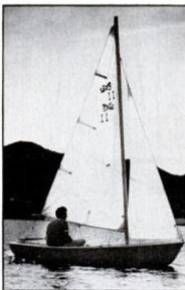
For sailing, rowing, motoring with outboard, 11-foot Glen L 11 is home-built from $15 plans in fiberglass over wood-strip sandwich core. Rigs as sloop or cat.
