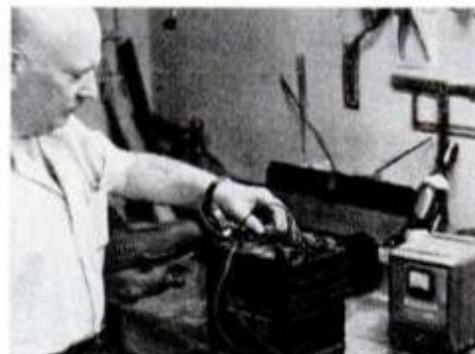
Battery charging is done by Ralph Dankner. Trickle charging extends battery life.
