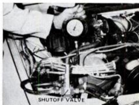
Pressure and counterpressure are checked with special gauge and shutoff valve.
