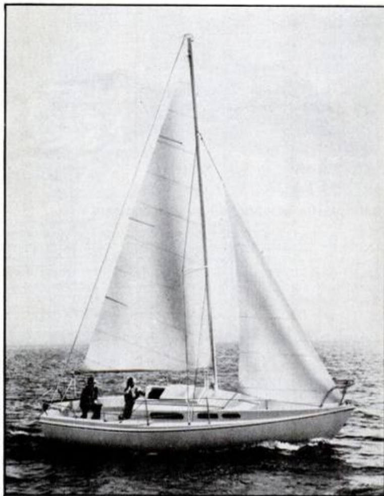
Luger Tradewinds, new 26-footer that is trailerable, sleeps five, has one-piece hull, deck for easy kit assembly. About $4000 with sails.
