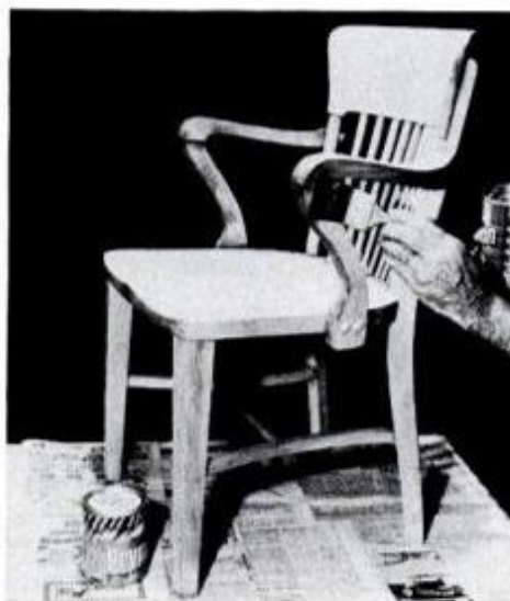
Thorough scraping was done on chair (at right) when it was disassembled for regluing. Disassembly made job easier.
