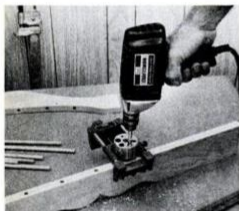
Adjustable doweling jig (Sears) simplifies drilling and aligning mating dowel holes in lower and upper side members.
