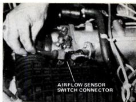
Airflow sensor switch is disconnected for checking the system.
