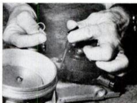
Allen wrench is inserted in airflow sensor, adjusted to lower carbon monoxide.
