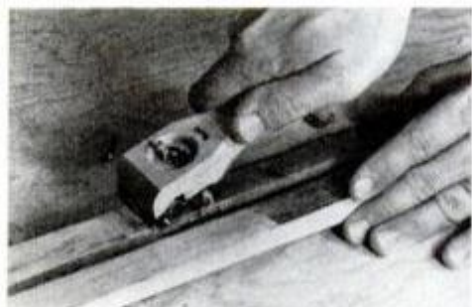
Bottoms are cleaned with sharp furniture scraper until all old wax, base and varnish are removed. Coin edge cleans groove.
