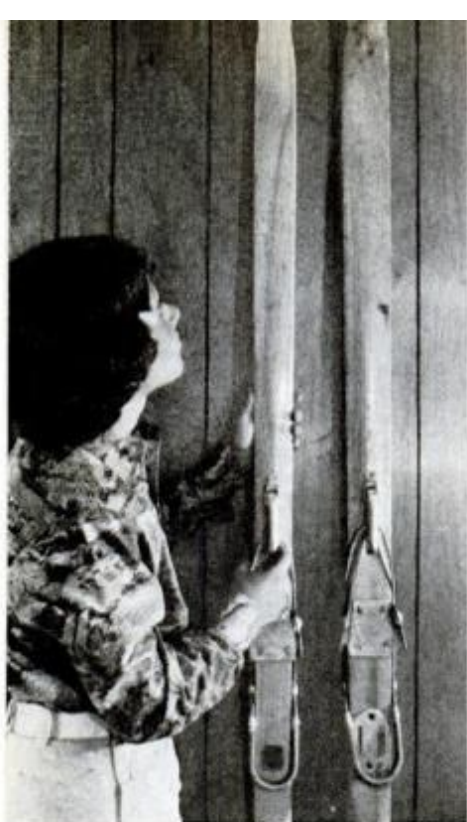
Sleek touring ski (left) for newly popular cross-country, can be trimmed from old Alpine (right) using same bindings.
