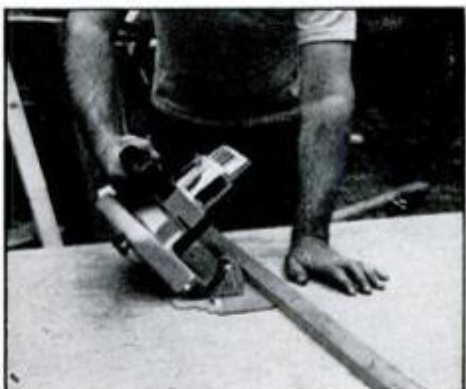
Use a slow feed for bevel cutting because the saw tends to drift away from guide.
