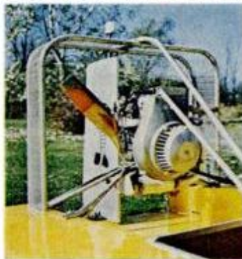
Vertical two-blade prop provides forward thrust; horizontal six-blade prop provides lift.
