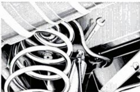
Upper shock mounting is reached with a socket and extension; open end holds nut.
