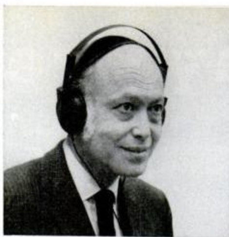
Dual headband on a Yamaha distributes pressure for best comfort. AKG is similar.
