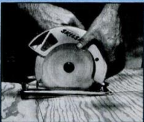
Plunge cut is made by slowly lowering the spinning blade into marked workpiece.
