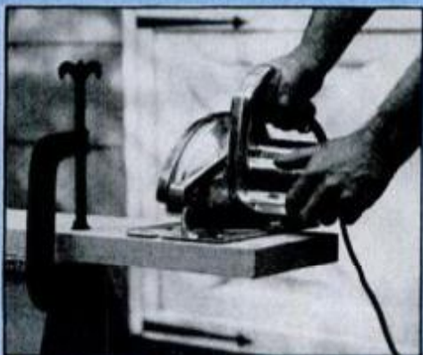
If saw must ride cutoff portion, clamp work securely, hold tool with two hands.
