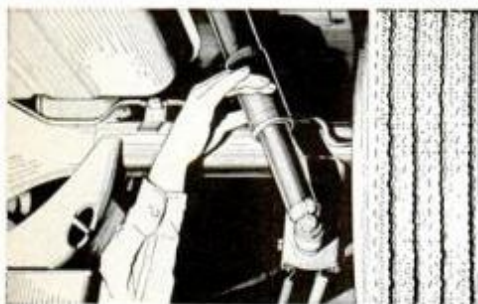
Rubber chamber identifies this rear shock absorber as being the air type.
