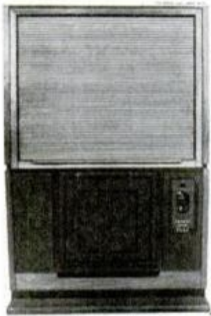
Sony's latest projection TV, its first designed for home use, combines tuning and control circuits, projector and 40-inch screen into one $2500 cabinet (top) that folds when not in use (bottom photo above).
