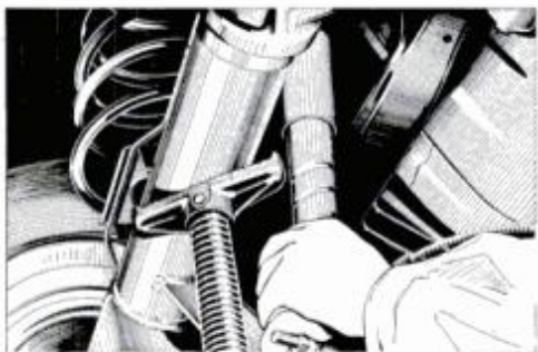
Rear shock absorber can be tested after the lower mounting is disconnected.
