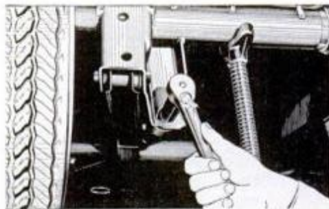
Lower shock mounting is easy to reach, but the nut and bolt are often frozen.
