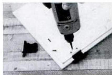
Variable-speed drill becomes screwdriver when fitted with driver bits.
