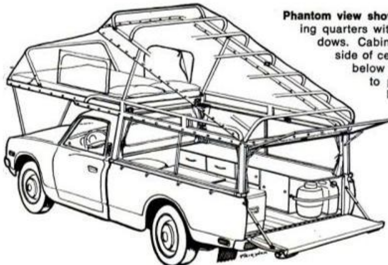
Bed tray slides out over hood to provide upper bunk for two. Canopy framework pivots at rear and rests when closed on permanent side rails.
