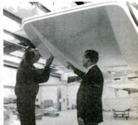
Tunnel bottom slot is pointed out by racing driver-designer Mel Mut, creator of new MonArk tunnel hull.
