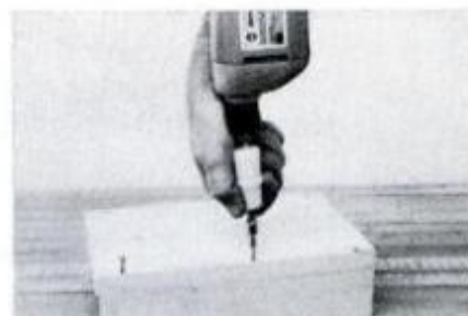
Screwdriver attachment (from Coastal) lets single-speed drill drive screws.
