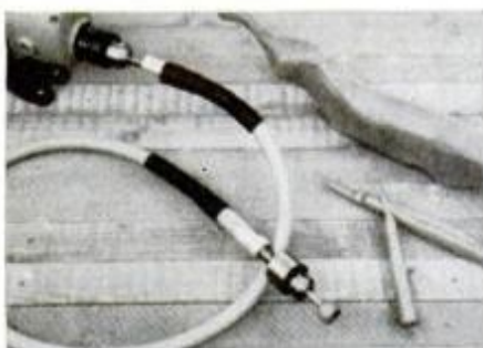
Flexible shaft is perfect for forming, sanding, polishing. Cost: about $13.
