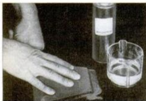
1. Etch glass surfaces by rubbing the two pieces together after sprinkling their surfaces with abrasive and water.
