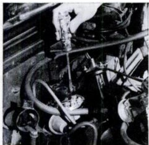
2 Remove distributor rotor; set aside until ready to install light chopper.
