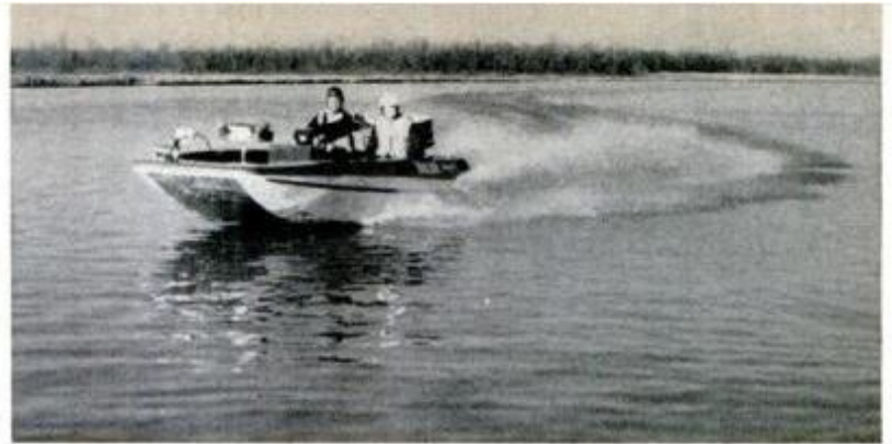
Trailer-mounted outside Arkansas plant, new hull features from stepped-sponson bottom to metal-flake top finish are checked by McClendon and PM's McKeown.
