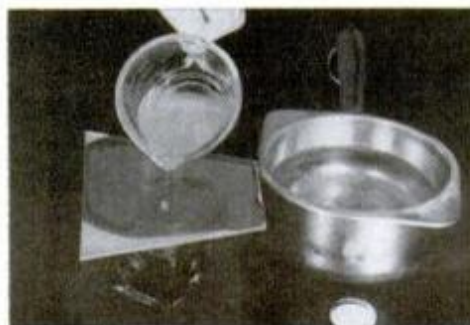
2. Pour melted animal glue over etched glass. The glue should not be overheated and the glass must be level.
