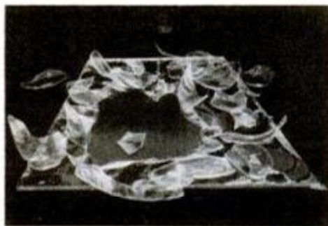
3. As glue dries it shrinks and "shatters" and tears off tiny chips of glass, leaving sculptured-looking surface.
