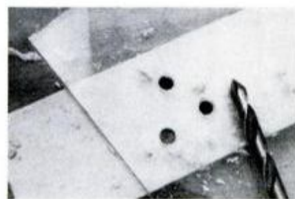
Specially shaped bit is used to bore chip-free holes in sheet acrylics.
