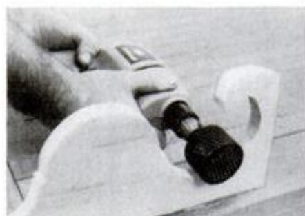
Surform quickly, neatly, removes stock; drill must be steadied with two hands.
