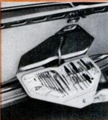
Toolkit is built in trunk lid. Instruments and controls are rationally positioned.
