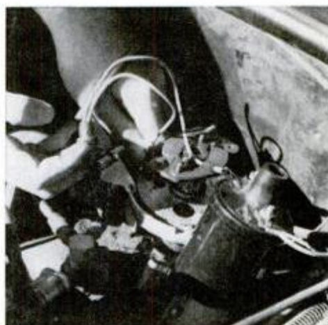
4 Place the trigger light on the distributor plate ready to secure.
