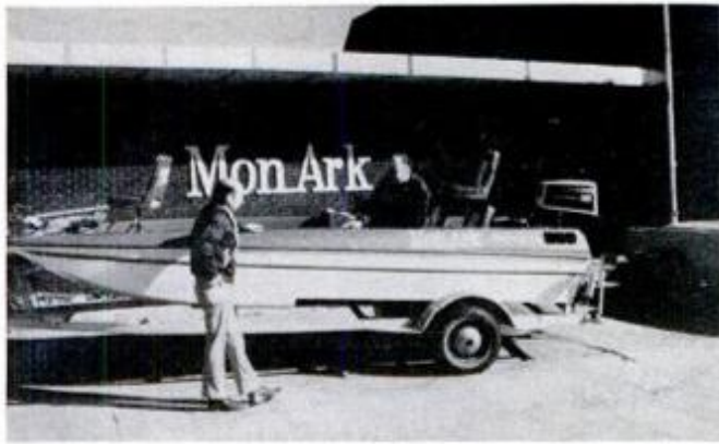
Trailer-mounted outside Arkansas plant, new hull features from stepped-sponson bottom to metal-flake top finish are checked by McClendon and PM's McKeown.
