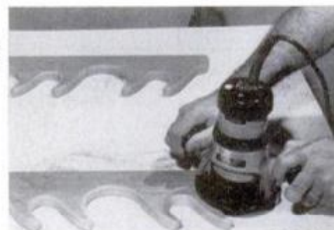
Drop out waste by making a pair of cuts tangent to each hole to create a slot.
