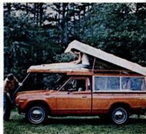
Bed tray slides out over hood to provide upper bunk for two. Canopy framework pivots at rear and rests when closed on permanent side rails.
