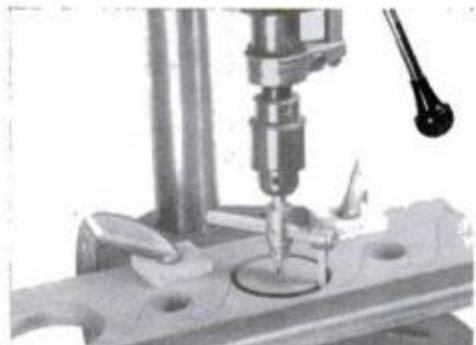
Clamp work securely and keep fingers out of way when using adjustable fly cutter.
