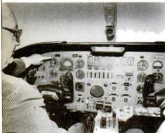
Flasher—back-up for taped-voice warning—is indicated by pilot of corporate jet.
