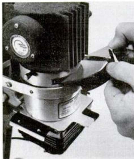
Filter drawers found in many enlargers take inexpensive CP acetate filters.
