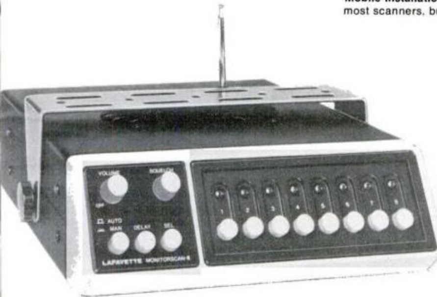
Lafayette Monitorscan DB-8 covers any eight channels on high VHF or low VHF bands, has automatic scan delay (see page 97), costs $150.
