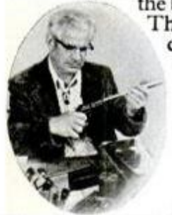
Colt Master Gunsmith checks barrel-chamber alignment.
