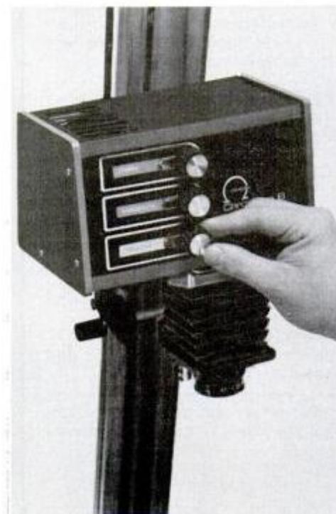
Color heads let you dial in exact filtration wanted; diffuse light to minimize negative spots, scratches and finger marks.
