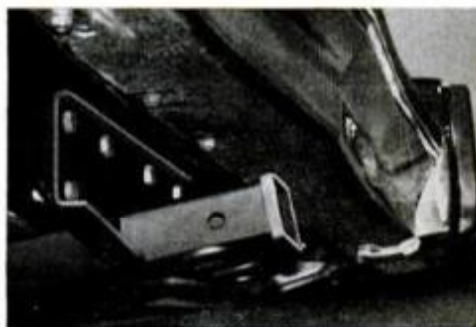
With hitch sleeve behind bumper and tow ball arm removed when not in use, rear impact will not pass from sleeve to chassis.
