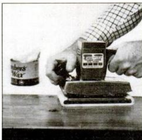
Fitted with a polishing pad , sander brings paste wax to smooth, high luster.
