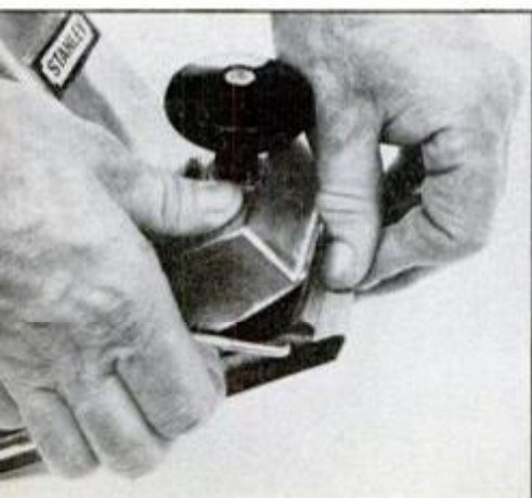
Method of holding sandpaper varies with makers; author liked Stanley's version.
