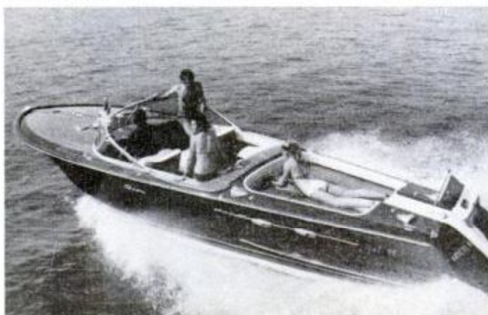
Famous for fun along the French and Italian rivieras, the Riva runabouts, with sunken sun deck and reverse transom, are finished in varnished mahogany.
