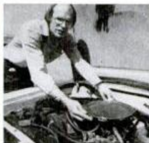
Free-breathing air cleaner installed by author netted him a gain of 4.5 mpg.
