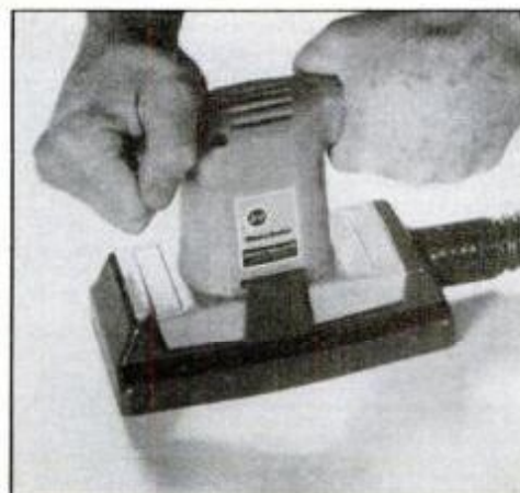
Dustless sanding is possible with vacuum attachment as on Black & Decker model.
