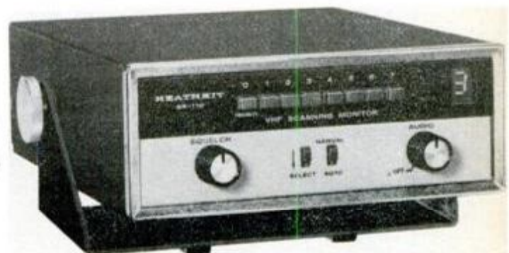
Heathkit 8-channel covers 9-MHz slice of high VHF band, has one priority channel, takes four evenings to build, is $100.
