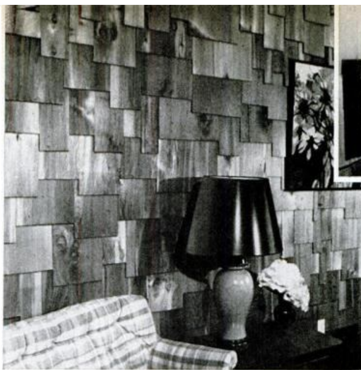
Shingle Interior-Tex 4-ft. panels by Shakertown feature self-aligning backing. You rest back of a panel on panel below, nail or staple it in place and continue application up the wall. Molding is used at the ceiling to complete the job.
