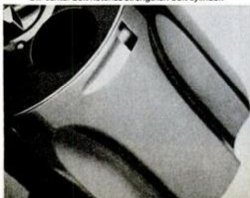
Off-center bolt notches strengthen Colt cylinder.
