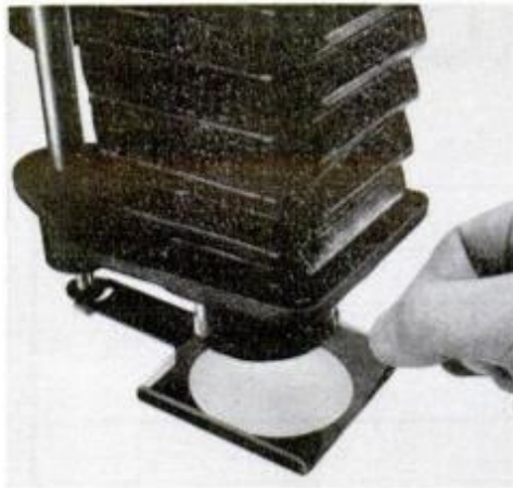
Under-lens filters fit any enlarger—but must be the expensive, fragile CC type.
