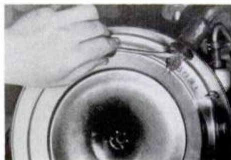
This PCV filter is mesh type.
