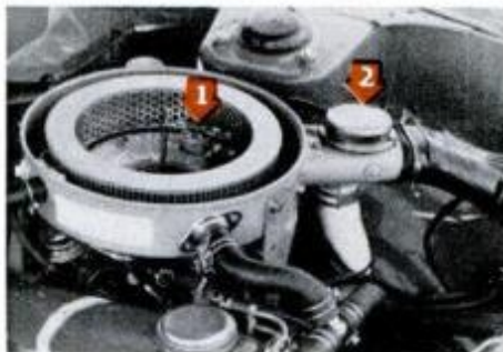
Thermostatically controlled air cleaner parts are: 1. temperature sensor and 2. damper valve.
