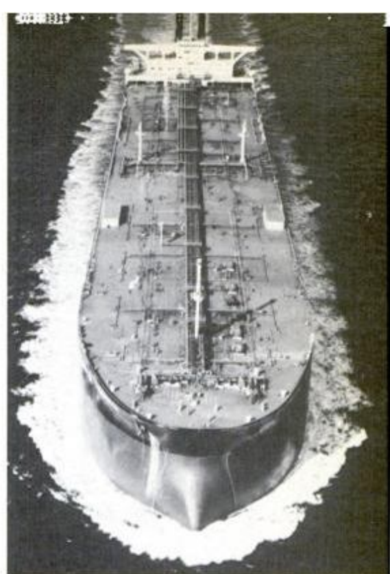
One of largest tankers afloat, Globtik Tokyo weighs 476,025 tons, is 1250 feet long and draws 92 feet when loaded.
