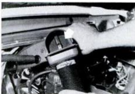
Damper valve is closed on cold engine.
