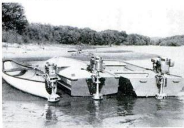
Jet power from outboard? Otterbine four-cycle water jet models come in three shaft lengths and four Briggs & Stratton power heads of 3½, 5, 8, and 10 hp. Snag-free operation is claimed.
