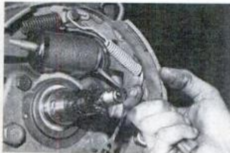
Check wheel cylinders for damage or leaks.
