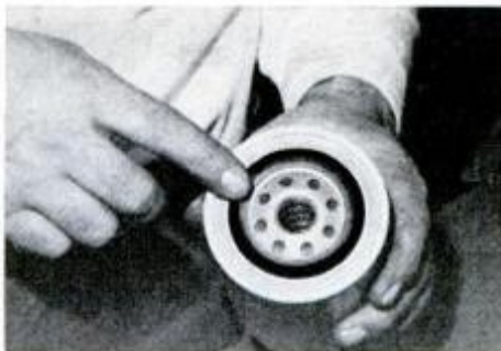
Oil filter gasket should be coated with a film of clean oil before it's installed.
