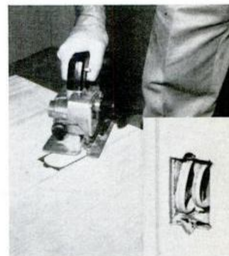
Make plunge cut with sabre saw; complete cutout. See neat accurate fit (inset).
