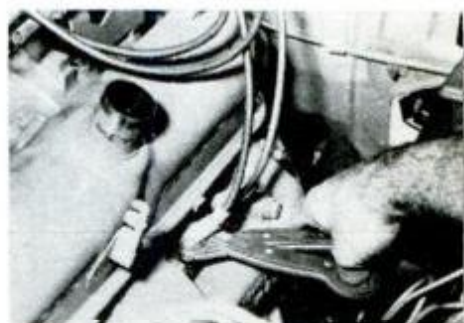
Cable puller prevents damage to cables.
