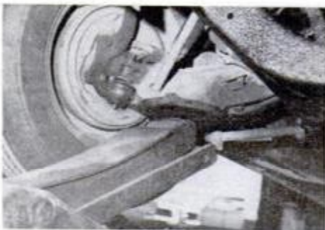
Test ball joints by taking pressure off primary load-carrier, here the lower ball joint of a torsion-bar suspension system.
