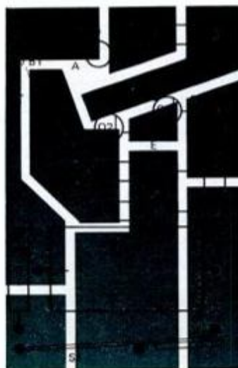
Component-location diagram can also be used as a pattern for cutting copper circuit board.
