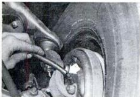
Vacuum hose is slipped over bleed screw at one of the wheels for bleeding system.
