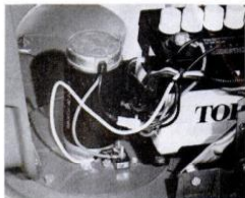
Flip-up cover permits recharging without removing battery from the machine. Motor (right), smaller than coffee can, is surprisingly powerful, spins blade 3350 rpm.
