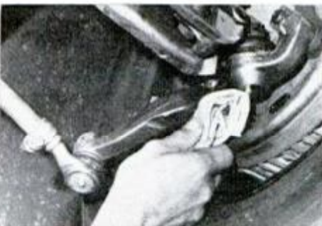
Grease fittings must be kept free of dirt.
