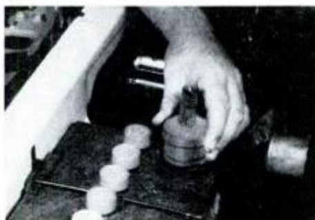
Wire-brush tool makes cleaning of battery posts a flick of the wrist—literally.
