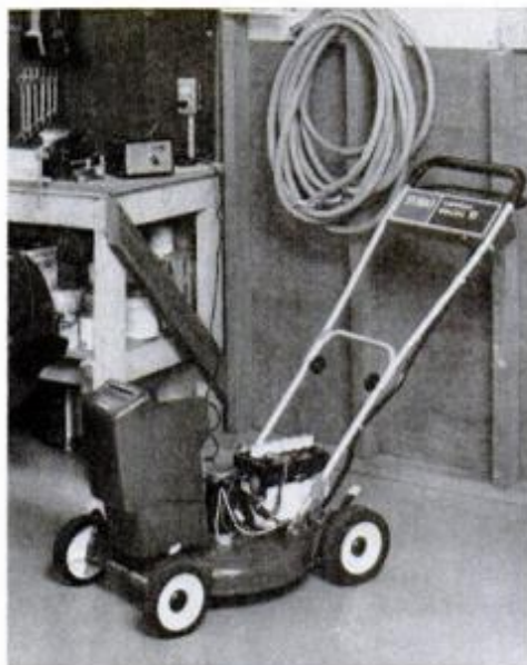
Flip-up cover permits recharging without removing battery from the machine. Motor (right), smaller than coffee can, is surprisingly powerful, spins blade 3350 rpm.
