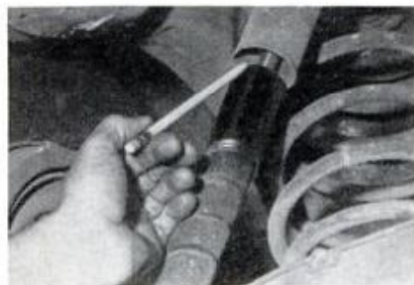
Check shock absorbers for leaks.
