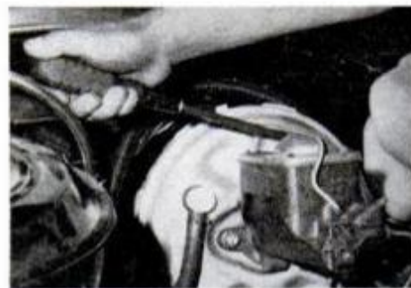
Master cylinder cover is easily removed for checking the level of brake fluid.
