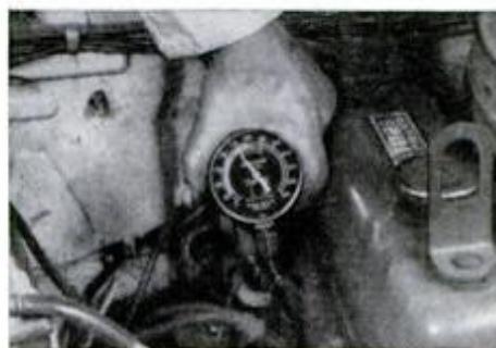
Compression tester is held in sparkplug hole while engine is cranked.
