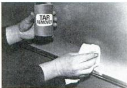
Special cleaners are made for removing tar.
