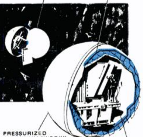
INTERIOR OF BUBBLE PERMITS "SHIRT-SLEEVE" FABRICATION OF COLONY MODULES AT ZERO GRAVITY
