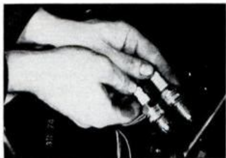
Sparkplug at top is "hotter" than the one below. Note difference in insulator length.
