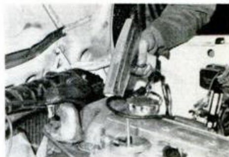
Timing light allows you to make perfect adjustment of ignition timing.
