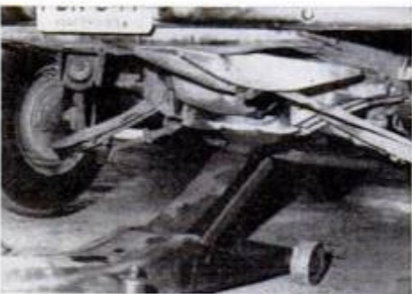
Jack under cross member takes pressure off upper, compression-loaded joint.
