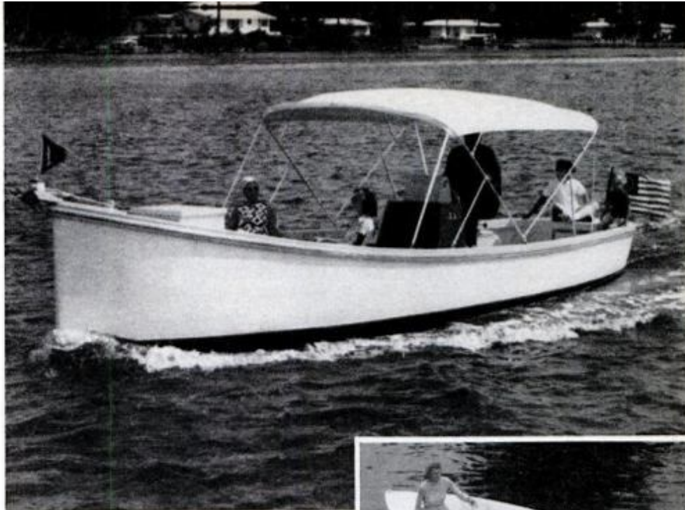
Gliding along without fumes or vibration, Branson Boat Co.'s Electra-30 (above) can cruise 50 miles at 5 knots, 200 at 3. Electra-18 (right) has 36-mile range.
