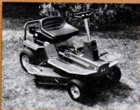
A 6-hp engine provides ample power for Massey-Ferguson's new MF 626 mower. It has 26-inch cutter, adjustable up to height of 3¼ inches.
