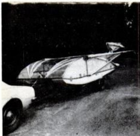
With wings and tail folded, glider can be easily trailered to and from water. Note teardrop shape of fuselage—itsself an airfoil for good aerodynamic characteristics.
