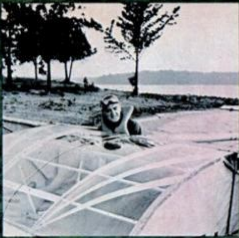
Ready for test flight, author checks out glider's controls. Correct trim adjustment and stay-wire tension are important for proper lift, stability and easy handling.
