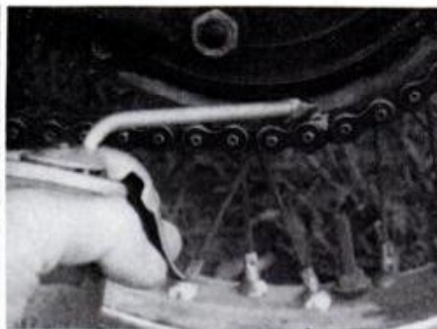
When lubricating chain with nozzled applicator, place tip against the sprocket so oil runs down to the linkplates.
