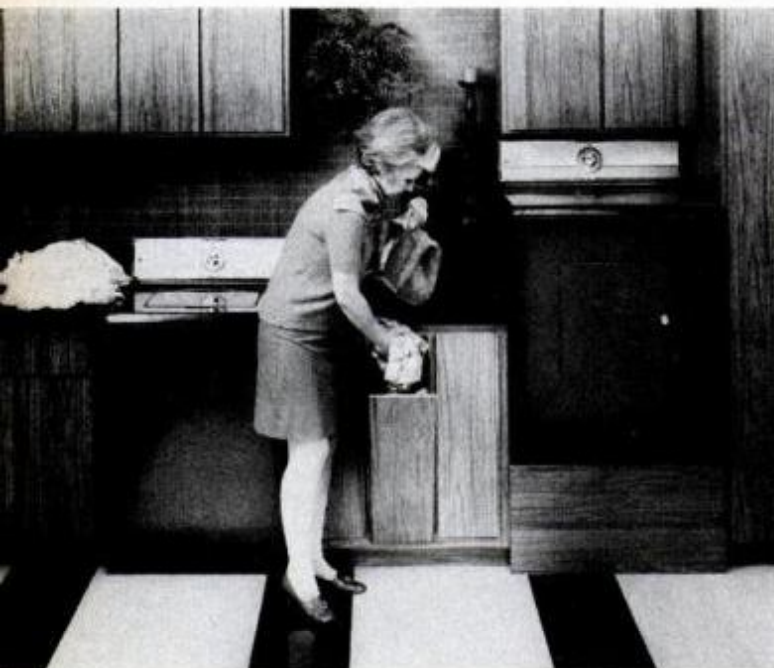
Elevated dryer rests on platform that has roomy storage drawer. Three tip-out bins alongside are for soiled clothes. Plan for making dryer platform is shown at right.
