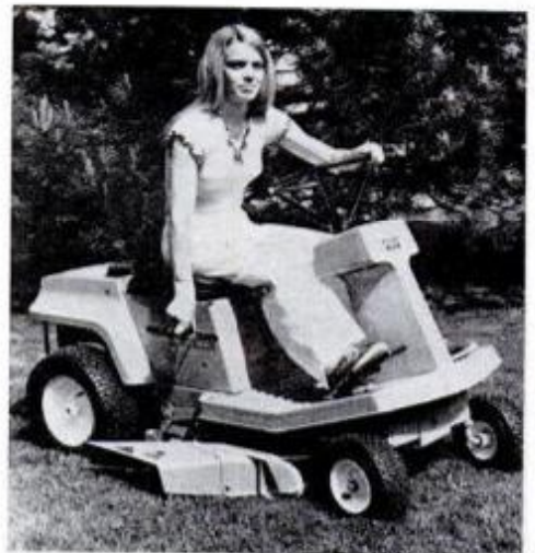
The Bolens 828 has interlocking safety switches hooked up to ignition, seat and brake. It's powered by 8-hp engine.
