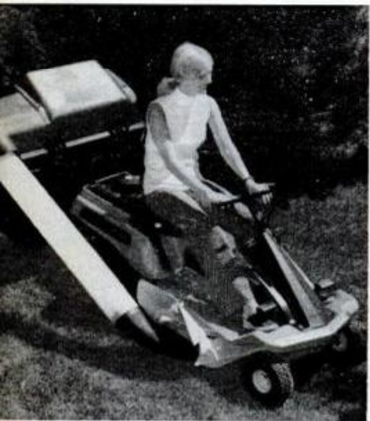
Two standard 20-gallon garbage bags hold clippings collected in the Grass Bagger, which fits most mowers in Ariens line.
