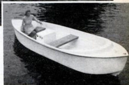
Gliding along without fumes or vibration, Branson Boat Co.'s Electra-30 (above) can cruise 50 miles at 5 knots, 200 at 3. Electra-18 (right) has 36-mile range.
