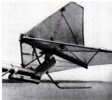
With wings and tail folded, glider can be easily trailered to and from water. Note teardrop shape of fuselage—itsself an airfoil for good aerodynamic characteristics.
