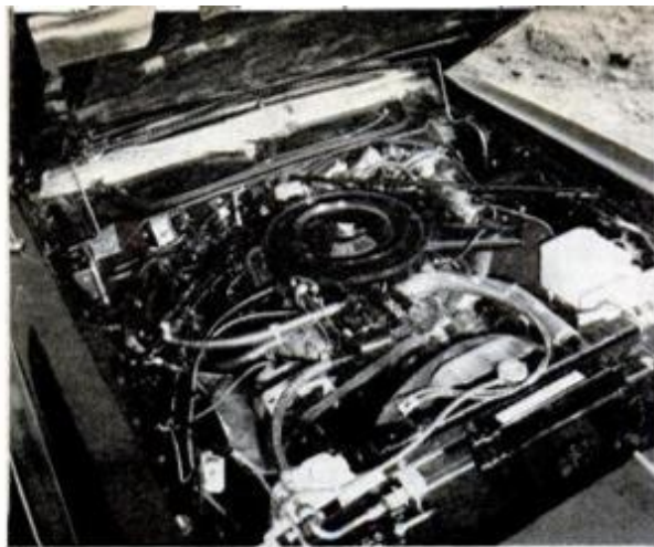
Fuel economy for the 318 and 360-cu.-in. V8 engines is almost the same, averaging about 15 mpg.
