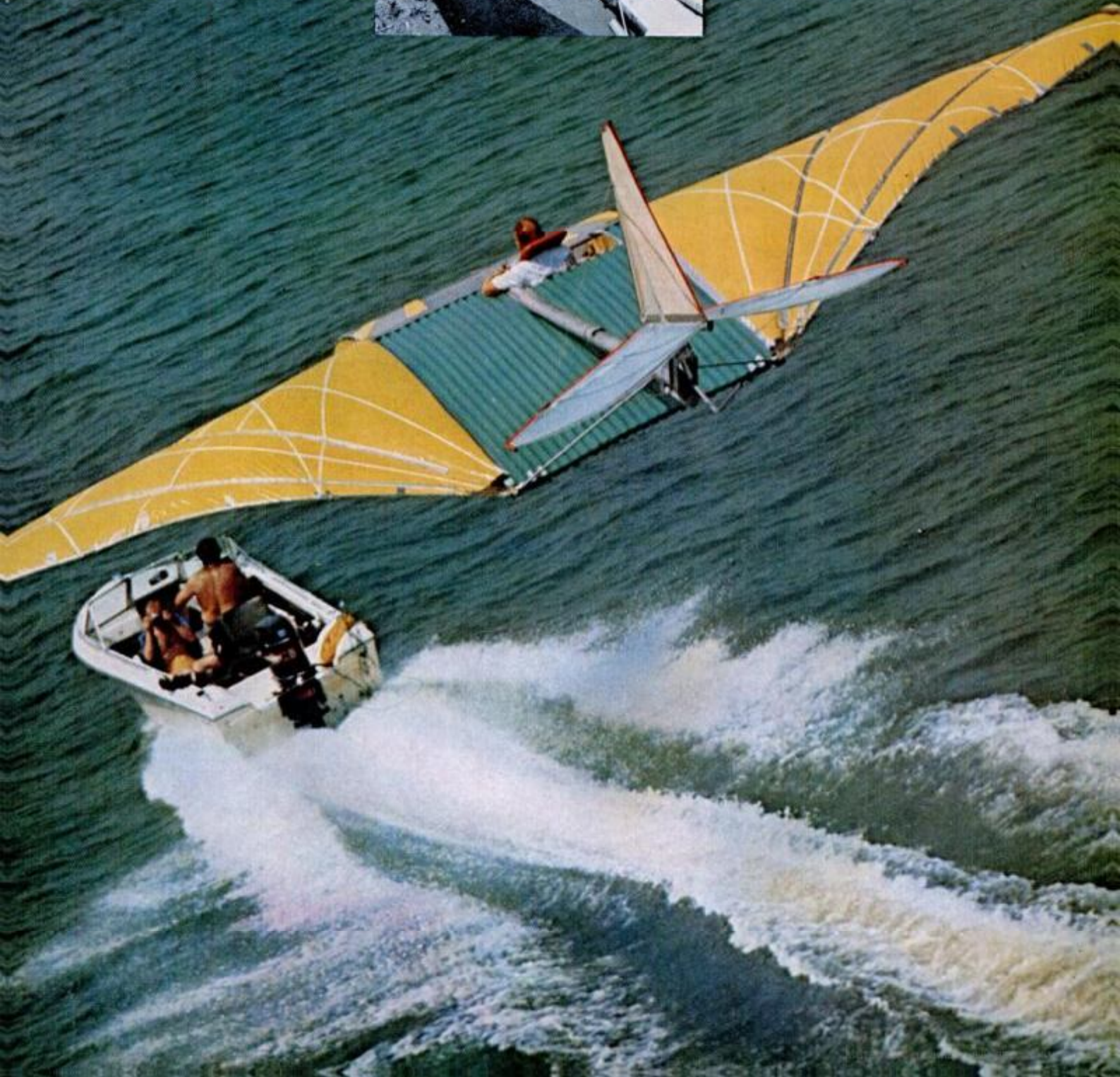
Ready for test flight, author checks out glider's controls. Correct trim adjustment and stay-wire tension are important for proper lift, stability and easy handling.
