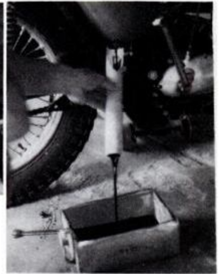
Drain oil from engine after it's at operating temperature. Paper-towel tube prevents splashing.
