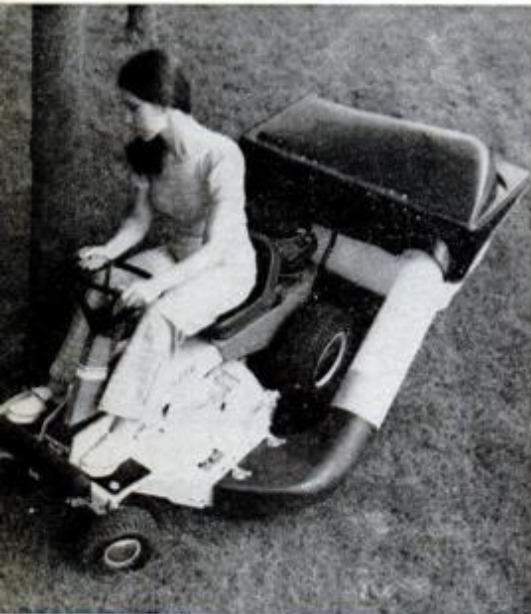
High-volume grass catcher , attached to any of three Homelite mowers, holds five bushels—about 75 pounds—of clippings.
