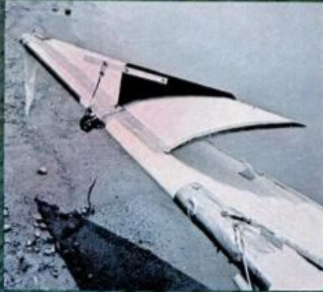
Weighing only 175 pounds, glider is readily carried into and out of water by two persons. Air view below, shot from plane, shows what it's like to soar 60 feet high.
