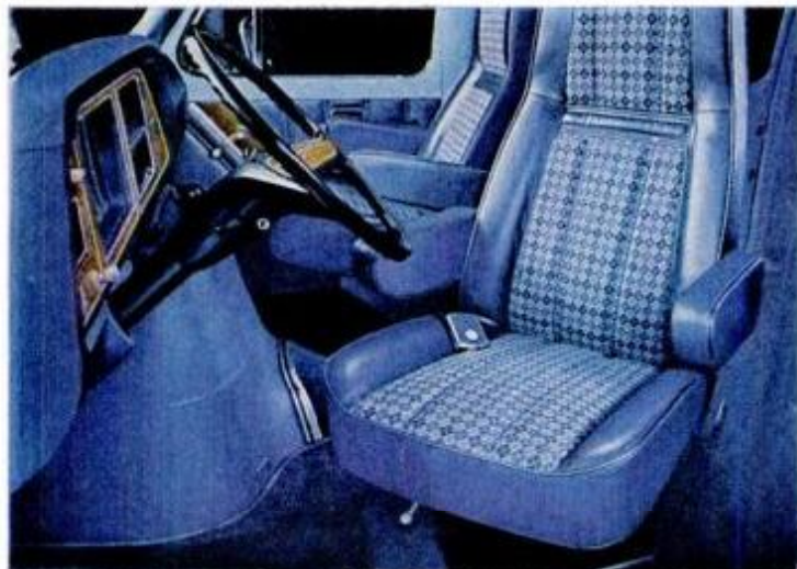
New easy entry. Econoline '75's door openings are taller than last year—wheelhousing is moved forward out of the way. New wide step. Optional Captain's Chairs pivot both ways, have fold-down arm rests.
