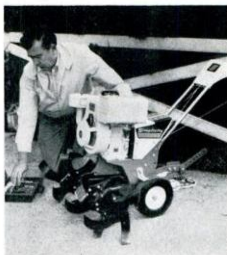
Heavy-duty tiller with rear-mounted tines (upper left) is one of seven models offered by Ariens. Powered by a 7-hp Tecumseh engine, it has two forward, two reverse speeds. The 8-hp Simplicity unit (above) has 35-inch tilling width with tine extensions. The 5-hp Gilson (left) cultivates an area as narrow as 12 inches, a useful capability in a small garden.
