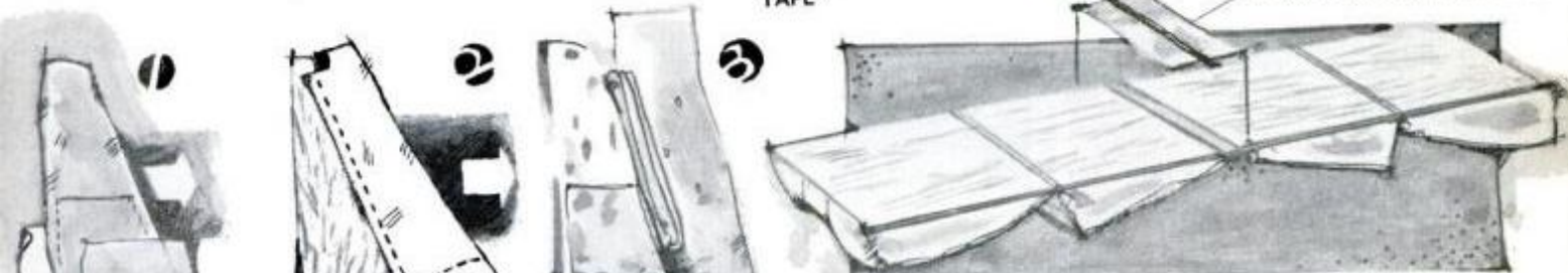
Plywood base of seats is connected to backs with hinges bolted to each, covered piano hinge between front and back. Front seat is hinged to base blocks; back slides aft.
