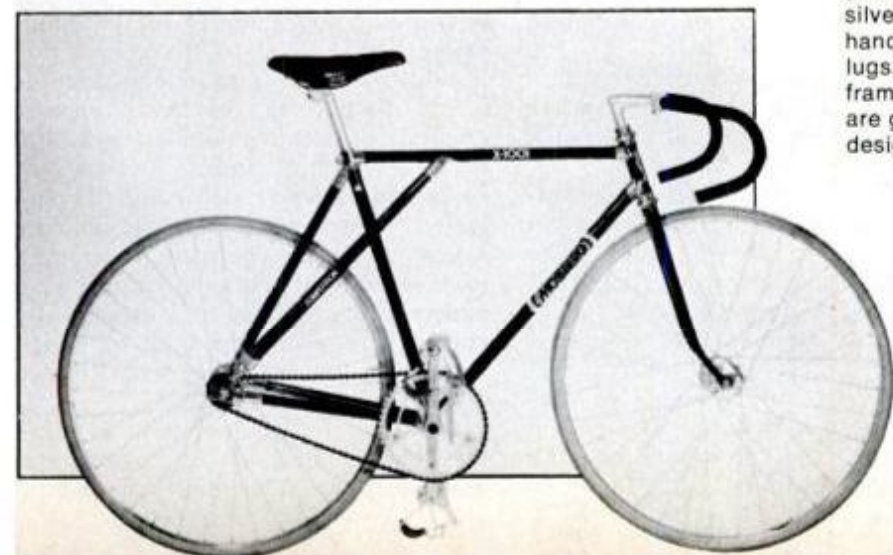
The stainless-steel frame of this Crescent bike will never rust or corrode. Monark-Crescent is in Varberg, Sweden.
