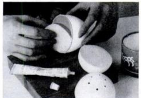
Cut Styrofoam balls in half, glue inside shells. Drills are poked into foam from top.
