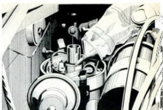
Cam lobe lubrication requires a steady hand: Place one drop on one cam lobe only. Take care not to overlubricate.
