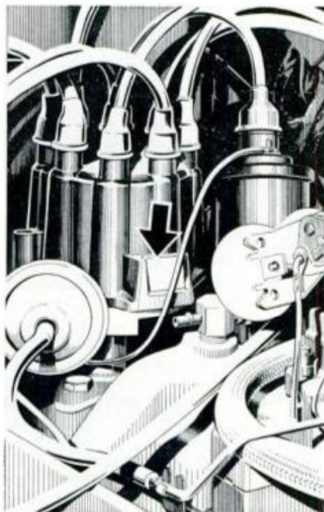
Dwell angle on some cars can be set without removing the distributor top. You open an access door and insert an Allen wrench to make this adjustment.
