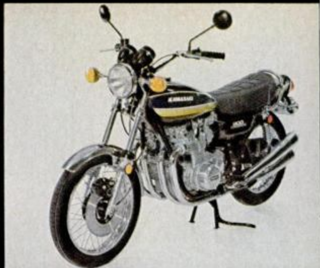
Kawasaki Z-1 is a four-cylinder, 900-cc, double-overhead-cam machine, with positive crankcase ventilation (PCV).
