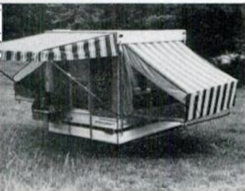
Designed for small-car towing, new Trail Star XL for '75 from Starcraft has 960-pound curb weight, added safety catch on lifter system, 110/12-v. converter.
