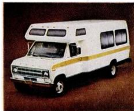
Mini-motorhome chassis. GVW's to 11,000 lbs. Single or dual rear tires. For bodies to 21 ft.
