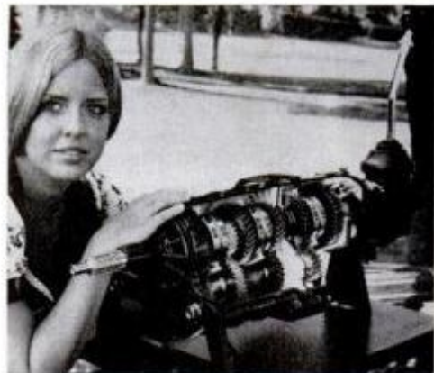
First five-speed mass-produced manual transmission in the United States for passenger cars is Borg-Warner's T50.
