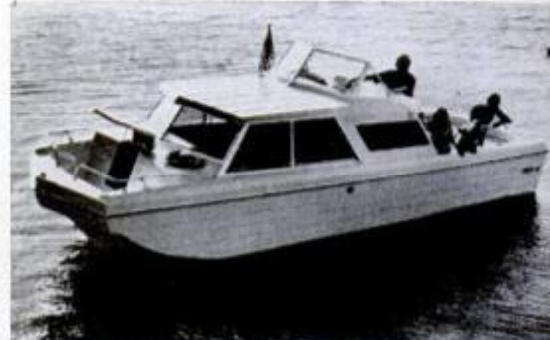
Steury's 23-foot T523 is another tri-hull with 1/0 power that sleeps four. A forward cockpit with guard rail adds safety.
