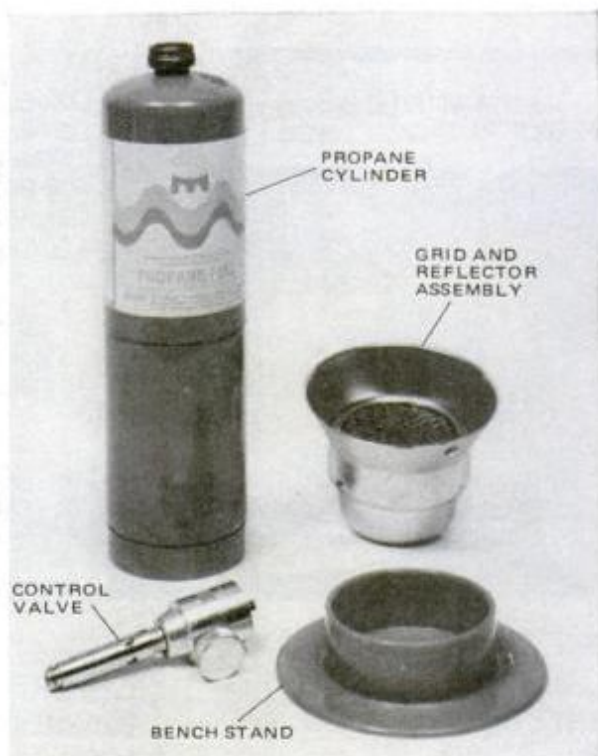
Four items shown at left come in kit for about $26. Head (above) operates on infrared-ray principle.
