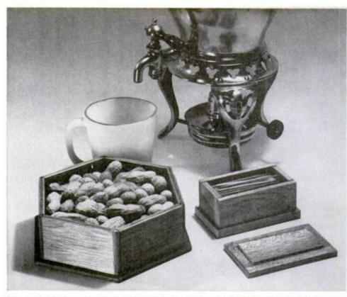
Shapes and sizes of two boxes shown above were controlled by dowel-peg jigs.
