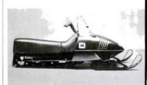
Cross-country racing is target of latest John Deere snowmobile, the high-performance 340/S model. Its increased base length allows the driver to sit forward while running at top speed. About \$1750.
