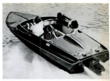
Water-jet speeds to 60 mph came from new Avenger 185 with new MerCruiser Jet 400 rated at 375 hp.
