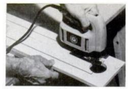
Sabre saw is used to complete parallel cuts to very corners to drop out waste.
