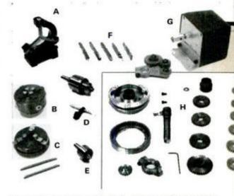
Accessories: A, steadyrest; B, 4-jaw chuck; C, 3-jaw chuck; D, tailstock chuck and key; E, live center; F, tool bits; G, power feed; H, screw-cutting attachment.
