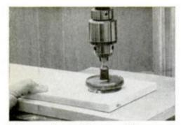
Hole saw is used in your drill press to make circular cut at top of side panels.
