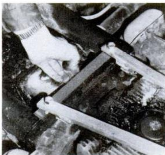
Extension straps bypass the motor area and are positioned after their clamp-bar plate has been slipped over the frame.
