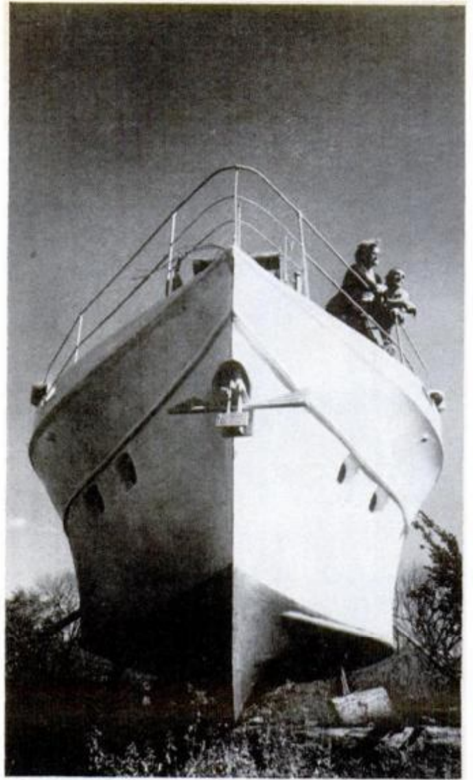
The Cindy-Marie has a 17-foot beam at deck level and is powered with an 85-hp diesel that will drive the yacht at an estimated 10 knots. A 1000-gallon tank will permit the vessel a range of about 3200 miles. The 16-foot-long engine room also contains a shop area and space for photo darkroom. Bow-thruster unit (below), driven by 15-hp electric motor, is another Bill Bodisch "original."
