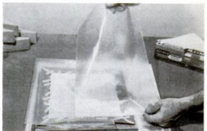
21. Cover face of picture with wax paper to prevent excess glue from sticking paper pad to inlay.
