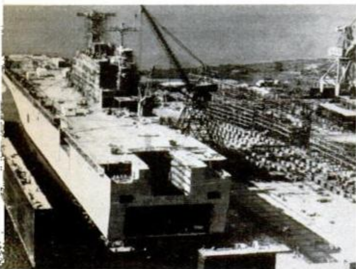
Largest man-made object ever to be moved on land, the first nearly finished LHA is rolled sideways from her construction site (top photo) onto launching platform (bottom photo)—a distance of some 50 feet. The huge vessel, weighing 19,500 tons, is transported on a complex system of wheels and rails. At launching time, the drydock-like platform will be flooded and the ship floated off for completion of outfitting and start of sea trials. The USS Tarawa shown here is one of five such mammoth LHAs scheduled to be built for the Navy during the next two years.
