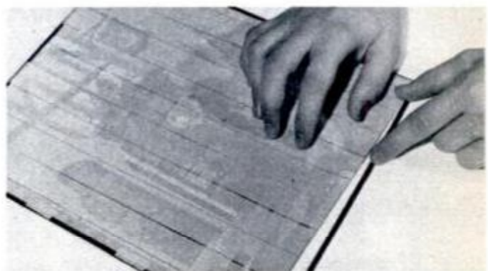
17. Add border strips of contrasting wood to the four sides and miter the corners for a neat fit.
