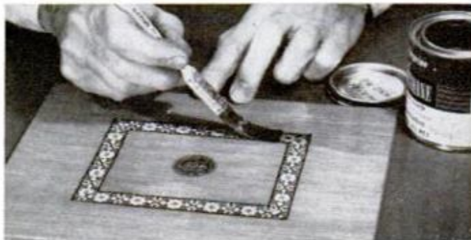
When glue is dry, tape is given two coats of clear urethane finish, finally the rest of the wood surface.
