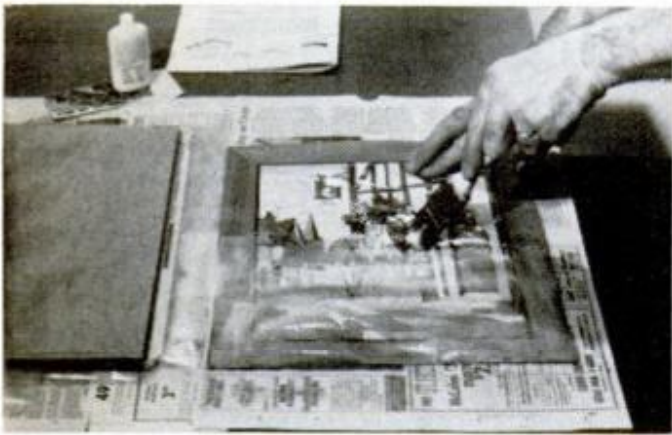
20. Brush white glue on both surfaces. Here the back veneer is already in place on the back panel.
