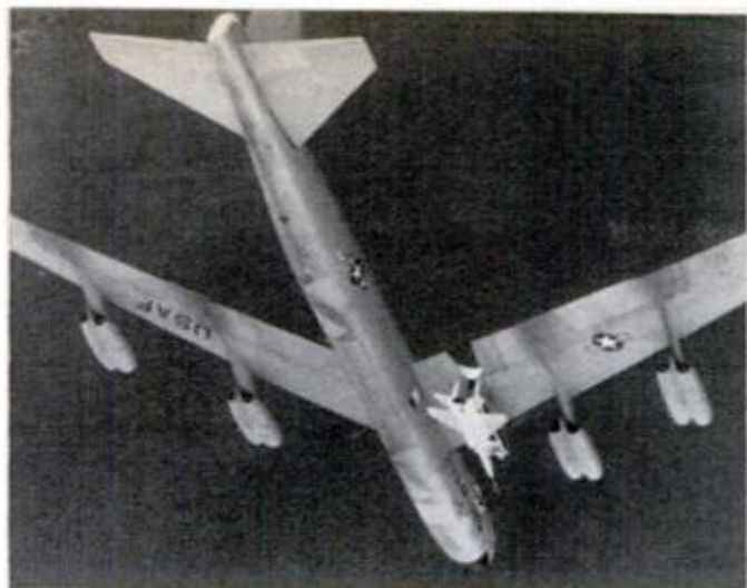
The test vehicle hangs below the big wing of a B-52, which will carry it up to launch altitude.
