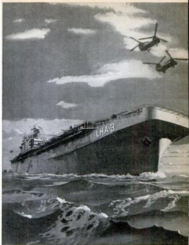
How LHA will go into action is depicted in artist's concept at left, showing simultaneous launching of helicopters from flight deck and landing craft from floodable docking well at stern. Above is bow view.
