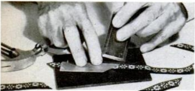
Ends of tape are mitered by holding sharp wood chisel against 45^\circ template and cutting over hardboard.
