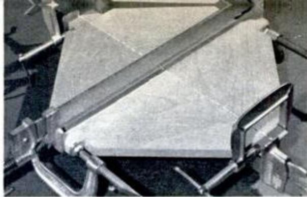
C-clamps are used at corners; bar clamp applies pressure to center area of glued-up work.
