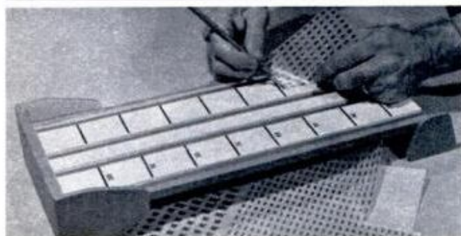
Black charting tape, \frac{1}{8} in. wide, is used to rule lines on track surface (top). Green tape marks wheel channels; press-on numerals make neat numbering job.
