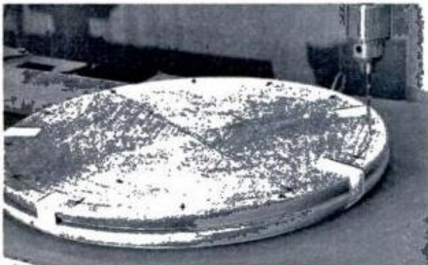
Pilot holes for spindles are drilled in base and ring at same time to assure perfect alignment.
