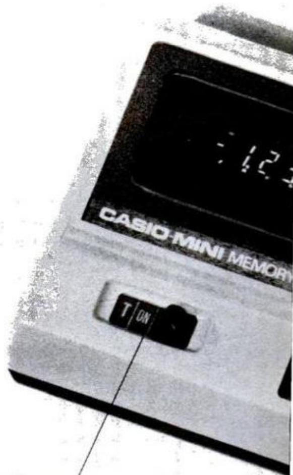
"T" setting on this Casio's on-off switch controls memory. Most calculators with memory use a separate switch
