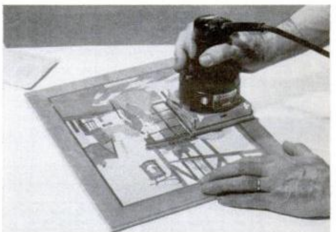
23. Power finishing sander and fine abrasive paper can be used to clean surface if you work carefully.
