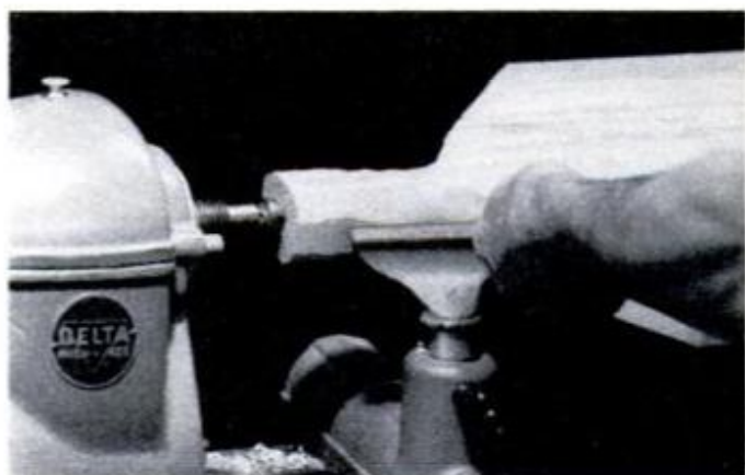
Use ¾-in. gouge, sharply honed, to begin turning handle section round. Keep hands clear of whirring blank.
