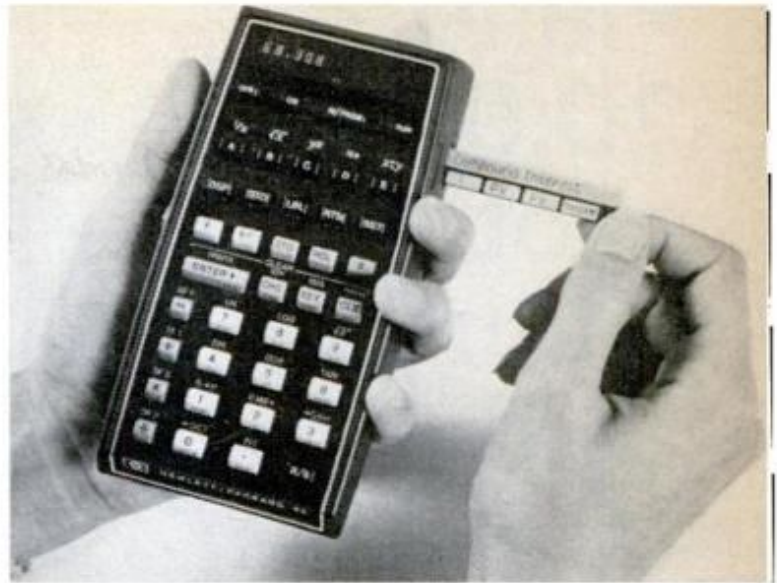
Calculator you can program to perform sequences of operations automatically is Hewlett-Packard's $795 HP-65; 950 premade programs are also available.
