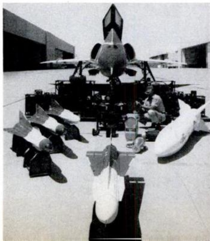
This F-106 is almost a drone. Electronic black boxes can guide it to target and fire its missiles.
