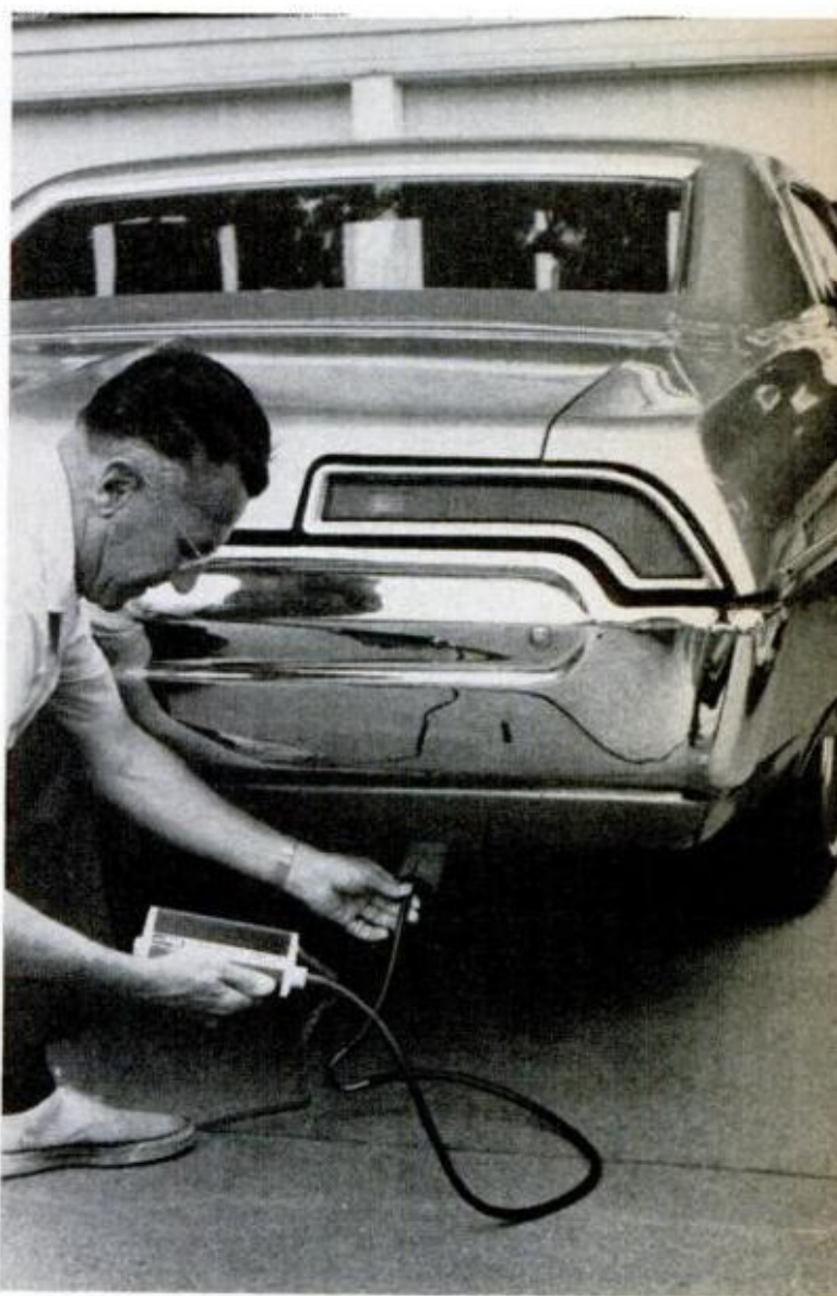
Analyzer probe clips to tailpipe and hose feeds exhaust-gas sample to sensor unit. Sensor produces electrical signal of strength dependent on air-fuel ratio being burned in your cylinders. Signal is conducted to meter circuitry for a direct readout of the air/fuel ratio and of the percentage of carbon monoxide present in your engine exhaust.
