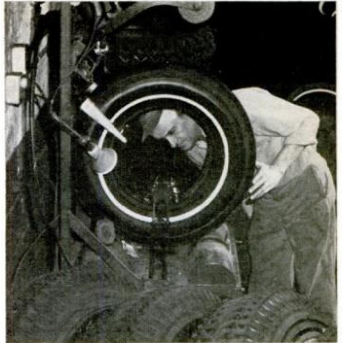
Inspection of retreading operation is done during all stages, plus a final inspection of completed tire.
