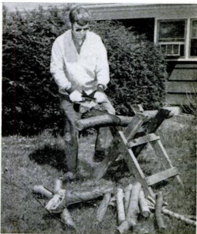
Either trigger can be used, depending upon stance. Use of rear trigger here is easier on right arm.
