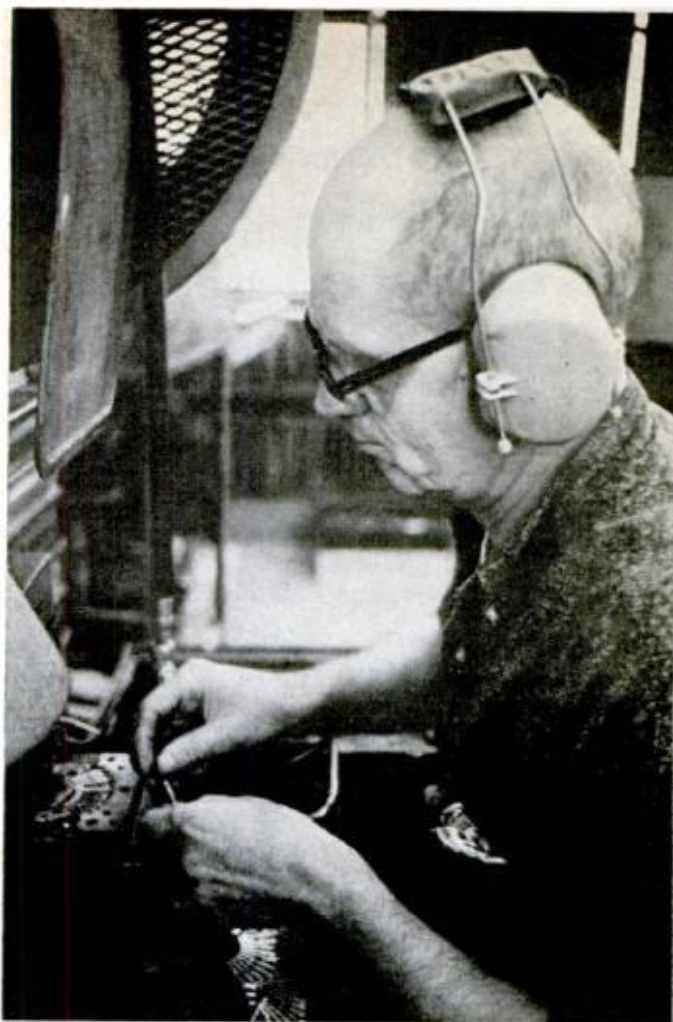
Punch-press operator wears muff-type ear protectors, which reduce sound intensity by up to 40 db. Most industrial plants now require workers to wear such protectors where noise levels approach or exceed 90 db.
