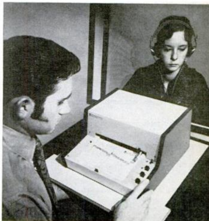
Chart recorder registers hearing acuity at various frequencies with moving pen on graph paper. It's useful for determining type and extent of hearing loss, compares left and right ears on side-by-side graphs.
