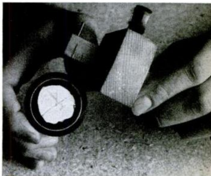
Hole in larger lens cap must be centered carefully and be wide enough to clear movie lens's threads.
