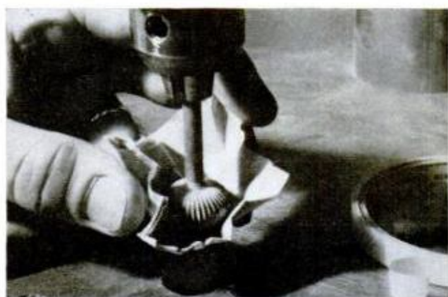
To sand compound in holes wrap abrasive paper on rotary file, tape to shank, chuck in drill press.
