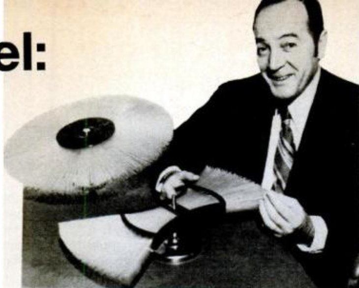
Models of two of the superflywheel configurations that David Rabenhorst (shown) has developed in his lab.
