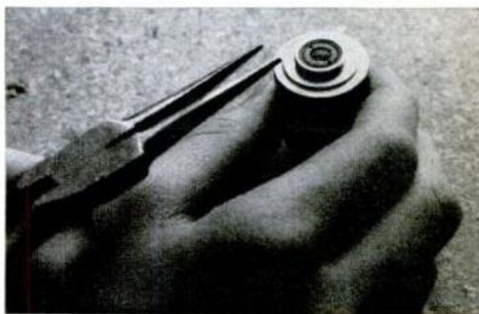
For a right-side-up image, use just the negative front element from a junked 8-mm camera's lens. Unscrew the rear element using a needle-nose pliers as a spanner, then discard.
